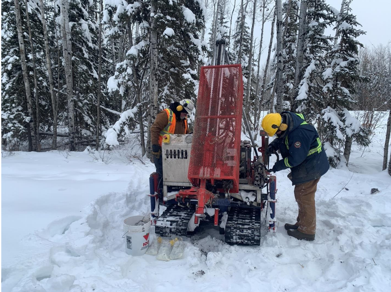
Figure 6. Shock-auger shallow-drilling system used to sample till beneath glaciolacustrine cover in AOI-2.
