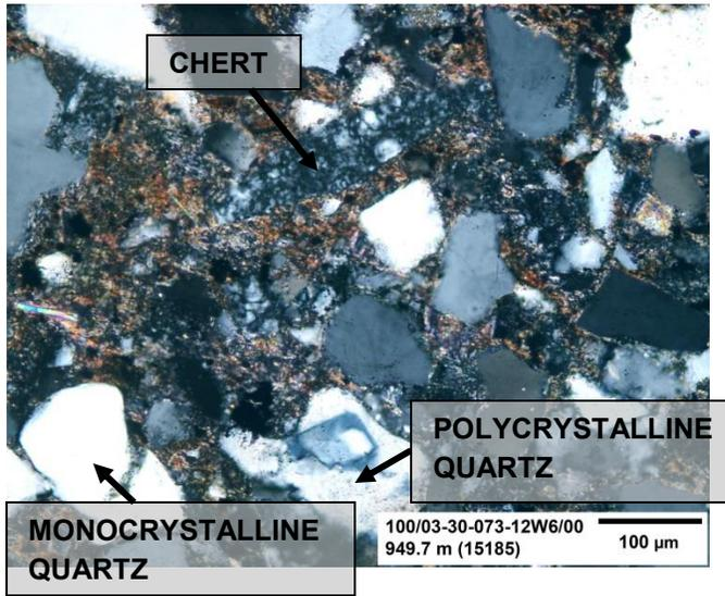
**Figure 94:** This figure is a high magnification image of the sample under cross-polarized light. There are a variety of quartz species in this sample which can only be differentiated with microscopy.
