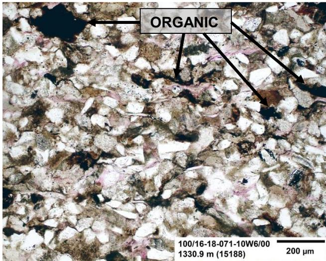
**Figure 104:** This figure is a medium magnification image of the sample under plane-polarized light. Organic components are observed throughout the matrix of the sample. The majority has been identified as amorphous material with some plant material.
