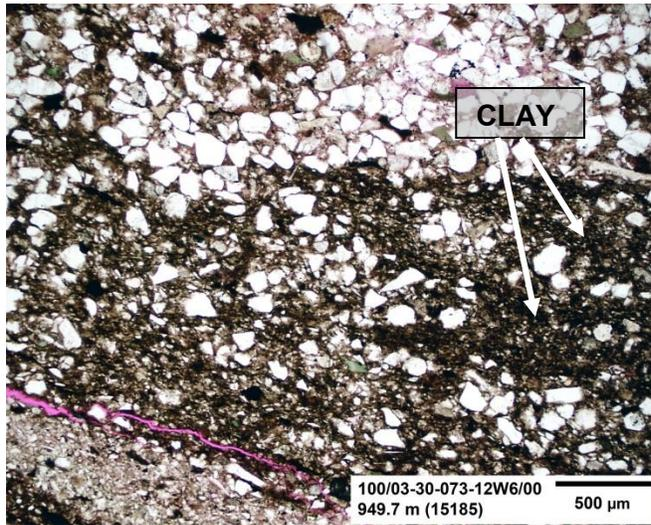
**Figure 91:** This figure is a low magnification image of the sample under plane-polarized light. The overall texture in this image appears immature which is characterized by heterogeneous distribution of clays, subangular grains and silt-sized to sand-sized grains distributed together (moderate-sorting).
