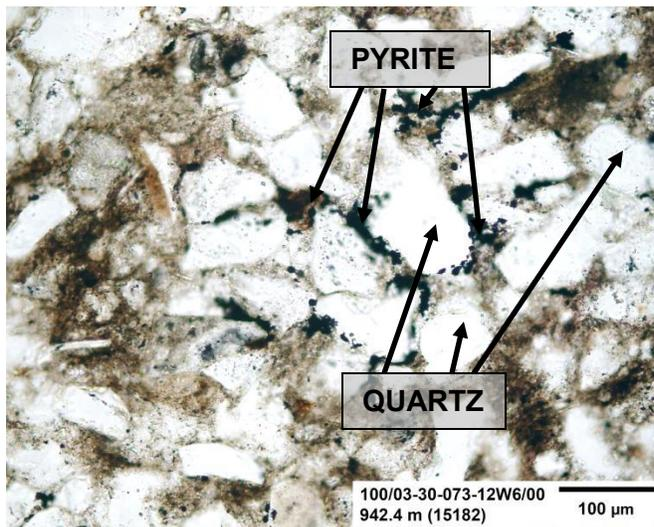
**Figure 89:** This figure is a high magnification image of the sample under plane-polarized light. Quartz grains are identified in the image and are characterized as upper silt-sized, subangular to subround grains. Pyrite is observed partially surrounding these quartz grains.
