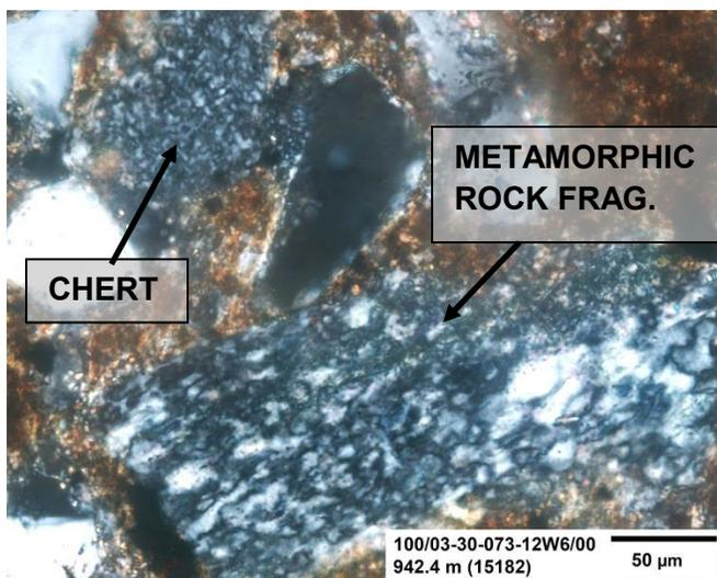
**Figure 90:** This figure is a high magnification image of the sample under cross-polarized light. At first glance the chert and metamorphic rock fragment (MRF) appear texturally similar and can be confused for one another. The distinguishing factor of the MRF is the elongate crenulate quartz crystals that comprise the grain. These sutured high relief crystals are indications that this grain was subjected to compaction forces. The chert grain is characterized by its cryptocrystalline texture.
