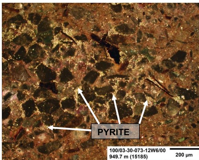
**Figure 93:** This figure is a medium magnification image of the sample under reflected light. Pyrite is observed as the lustrous mineral observed partially surrounding the framework grains in the image.
