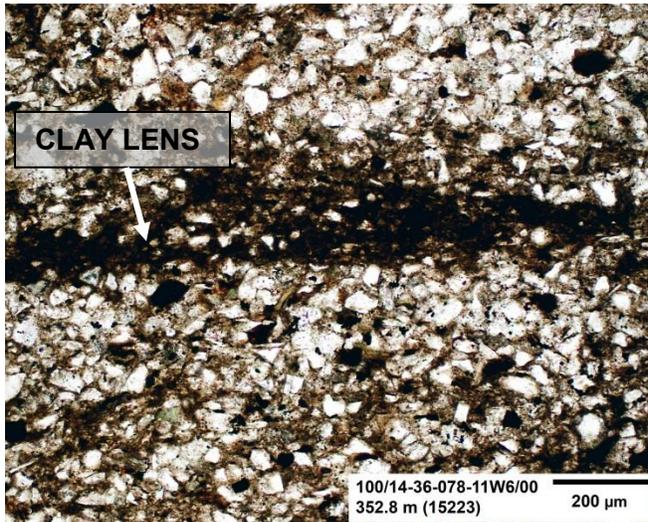
**Figure 118:** This figure is a medium magnification image of the sample under plane-polarized light. Thin clay lenses are observed throughout this sample.
