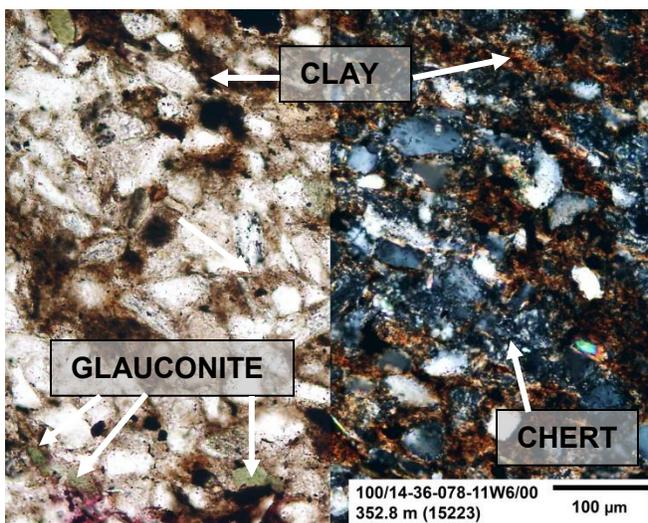
**Figure 120:** This figure is a high magnification image of the sample under both plane-polarized light (left) and cross-polarized light (right). This image shows some of the minerals observed in this sample and are identified as glauconite, chert and clay.
