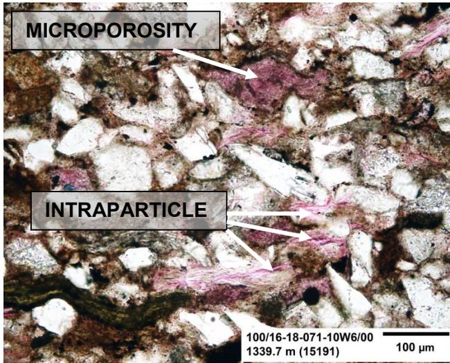
**Figure 112:** This figure is a high magnification image of the sample under plane-polarized light. The two main porosity types are identified in this image. Intraparticle porosity is mainly associated within mica grains. Microporosity is mainly attributed to clays that have replaced secondary porosity.
