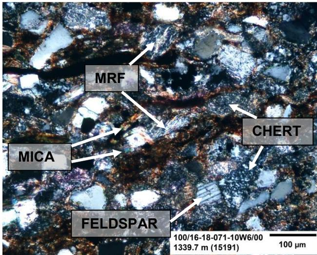
**Figure 113:** This figure is a high magnification image of the sample under cross-polarized light. This image shows the texture commonly associated with beds containing well-sorted, silt-rich grains. There is a large variety of grains observed in this image and are identified as metamorphic rock fragments (MRF), chert, mica and feldspar.
