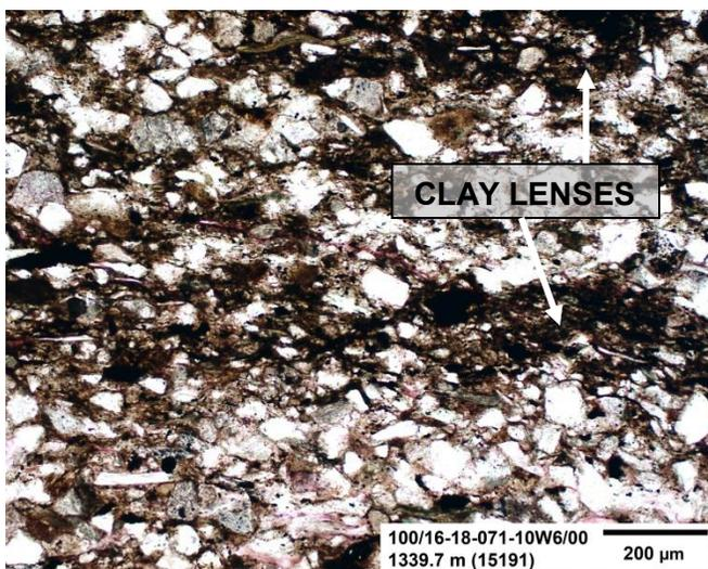
**Figure 111:** This figure is a medium magnification image of the sample under plane-polarized light. Isolated clay lenses are observed throughout the sample contrasting the lighter colored framework grains. Organics are often associated with the clay-rich lenses.
