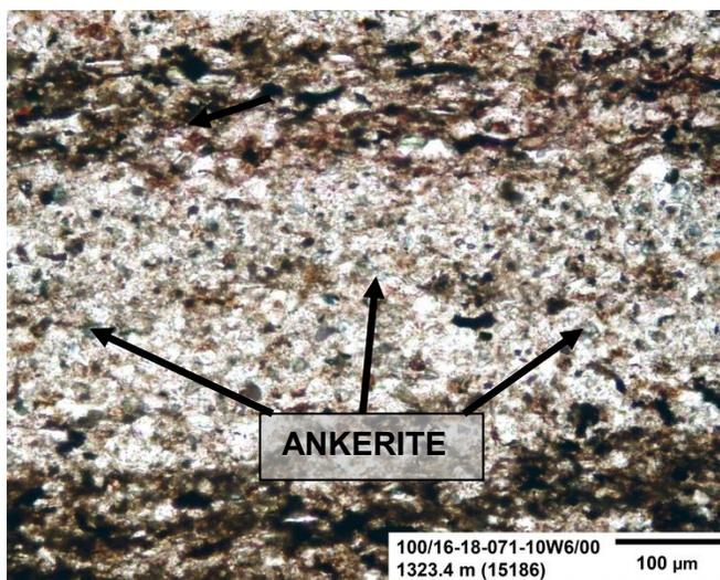
**Figure 99:** This figure is a medium magnification image of the sample under plane-polarized light. This image highlights the beds composed of upper silt-sized grains which are associated with ankerite cement.
