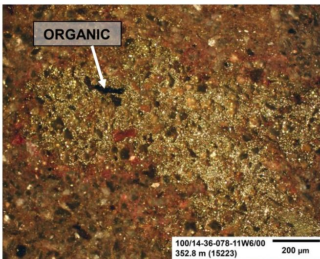
**Figure 117:** This figure is a medium magnification image of the sample, as in Figure 116, under reflect-polarized light. Note the organic fragment associated with the pyrite. Pyrite is highly lustrous and is primarily identified using reflected light.
