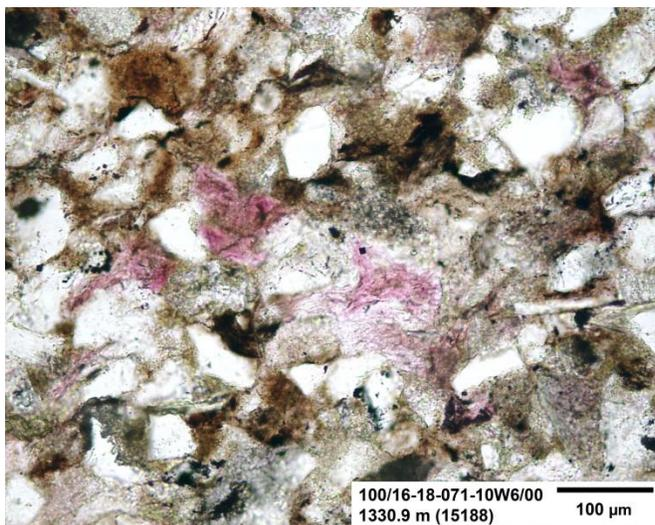
**Figure 105:** This figure is a high magnification image of the sample under plane-polarized light. This is the dominant texture observed in the sample which mainly is composed of quartz, rock fragments, mica, organic material and clays.
