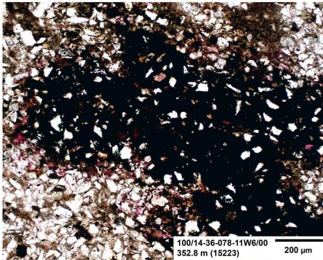
**Figure 116:** This figure is a medium magnification image of the sample under plane-polarized light. Pyrite is observed in concentrated “patches” throughout the sample.
