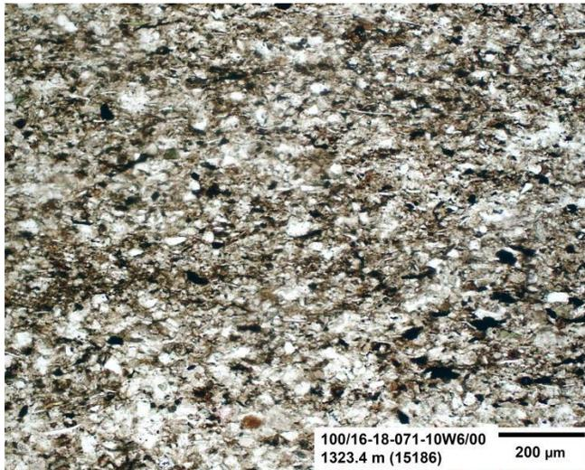
**Figure 100:** This figure is a medium magnification image of the sample under plane-polarized light. The texture observed in this planar bed lacks any structure (e.g. grain gradation) and has the appearance of massive bedding.
