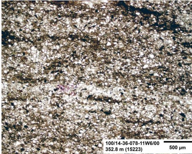
**Figure 115:** This figure is a low magnification image of the sample under plane-polarized light. This sample is composed of silt-sized, subangular to subrounded, well-sorted grains. Clay-rich lenses are observed throughout this sample.
