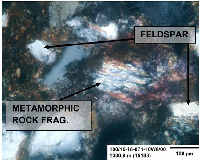
**Figure 106:** This figure is a low magnification image of the sample under cross-polarized light. The metamorphic rock fragment in this image is identified as a micaceous schist. Feldspar grains are also present in the sample.
