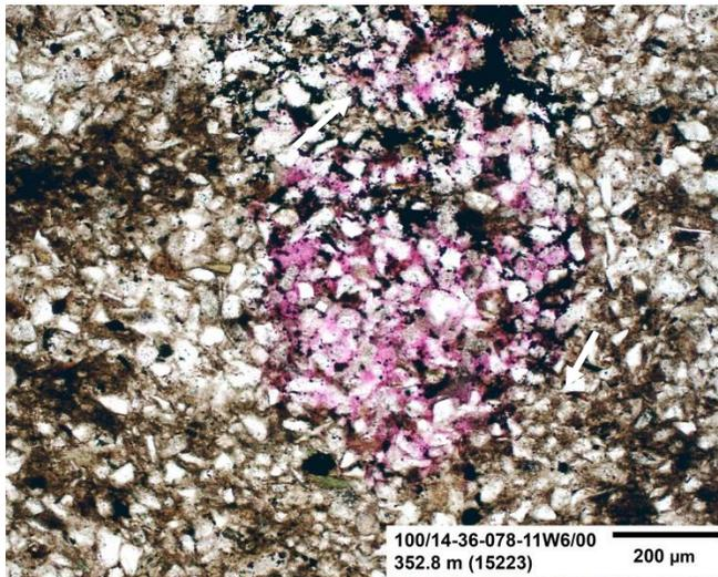
**Figure 119:** This figure is a medium magnification image of the sample under plane-polarized light. This image shows the localized intergranular porosity observed throughout the sample. These localized high porosity zones may lack interconnectivity.
