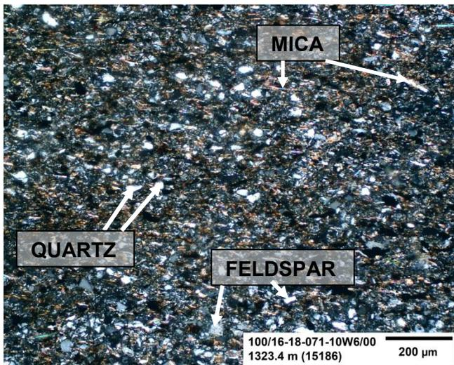
**Figure 101:** This figure is a medium magnification image of the sample, as in Figure 100, under cross-polarized light. Under cross-polarized light distinct properties of certain minerals are more readily apparent. Minerals identified are quartz, feldspar and mica.
