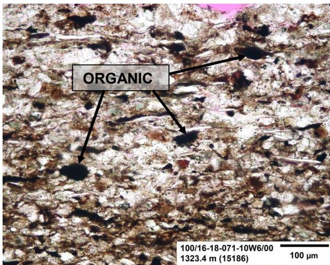
**Figure 102:** This figure is a high magnification image of the sample under plane-polarized light. The organic fragments observed in this sample are identified mainly as amorphous material.
