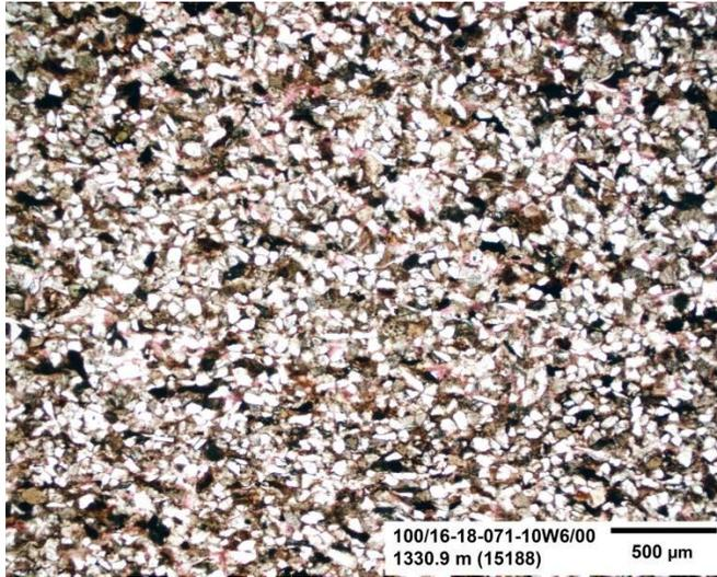
**Figure 103:** This figure is a low magnification image of the sample under plane-polarized light. Note the massive bedding texture observed in this image. The framework grains in this image are characterized as silt-sized, subangular, moderate sphericity and well-sorted.
