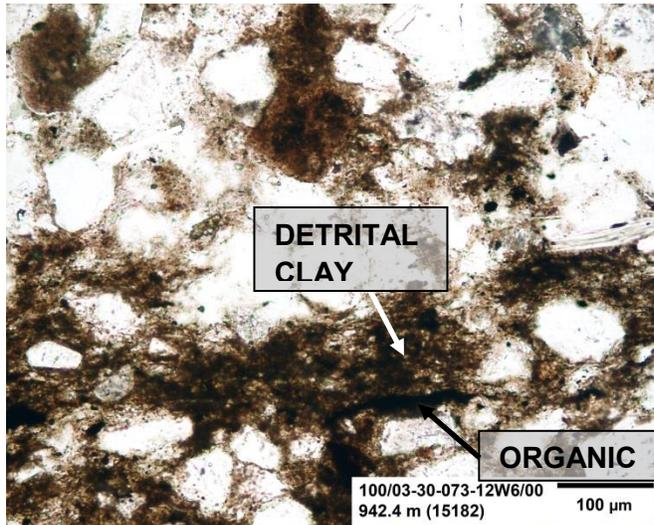
**Figure 88:** This figure is a medium magnification image of the sample under plane-polarized light. The clay lens in this image is composed of detrital clay. Note the elongate organic fragment that has been compacted and incorporated into the clay lens.
