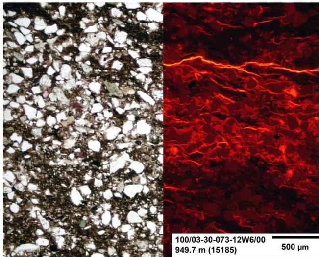
**Figure 92:** This figure is a low magnification image of the sample under both plane-polarized light (left) and ultra-violet light (right). This sample has high fracture frequency, however the majority of the fractures are artificially induced.
