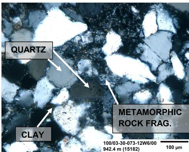
**Figure 87:** This figure is a high magnification image of the sample under cross-polarized light. There is a variety of minerals present in this image and have been annotated (quartz, clay and metamorphic rock fragment).
