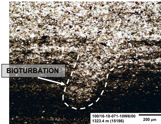
**Figure 98:** This figure is a low magnification image of the sample under plane-polarized light. Note the bioturbation trace that has disrupted the planar beds.
