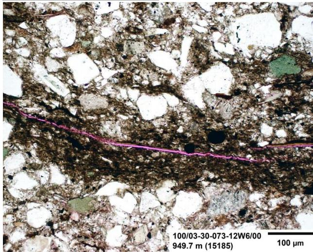
**Figure 95:** This figure is a high magnification image of the sample under plane-polarized light. The brown clay-rich lens in the sample is associated with fracture porosity.
