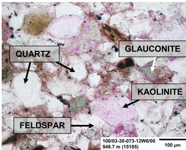
**Figure 96:** This figure is a high magnification image of the sample under plane-polarized light. Quartz, feldspar and glauconite grains are observed in the sample. Authigenic kaolinite is observed replacing the porosity in this image.
