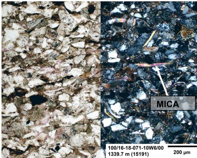
**Figure 110:** This figure is a medium magnification image of the sample under plane-polarized light (left) and cross-polarized light (right). Note the mica grains in the image where some are in excess of 200 microns (fine sand-sized). Comparing these mica grains to the harder framework grains, the micas are found fewer in number but coarser-grained.
