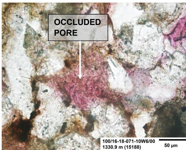
**Figure 108:** This figure is a high magnification image of the sample under plane-polarized light. Note the pore that has been replaced by clays/fines which changes the porosity type from intergranular to microporosity.
