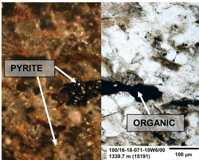
**Figure 114:** This figure is a high magnification image of the sample under both plane-polarized light (right) and reflected light (left). This picture focuses on an organic fragment in the center of the image. Under plane-polarized light the pyrite remains opaque and “hidden” within the organic. Under reflected light pyrite is revealed and can be discriminated from the organic.
