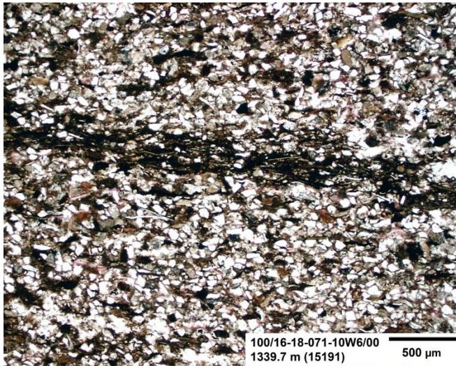
**Figure 109:** This figure is a low magnification image of the sample under plane-polarized light. This sample is composed of silt-sized, subangular to subround, well sorted grains. Clay-rich lenses are observed throughout this sample.
