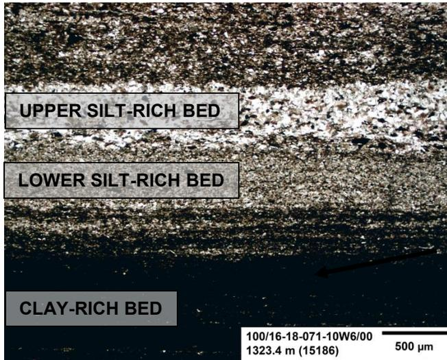
**Figure 97:** This figure is a low magnification image of the sample under plane-polarized light. Each bed in this sample can be characterized by grain-sizes. Individually the beds are well-sorted and form planar beds and thin laminations.
