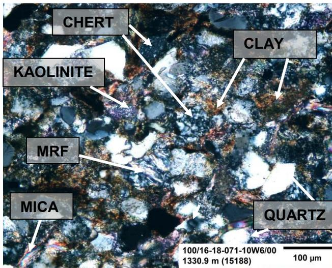
**Figure 107:** This figure is a high magnification image of the sample under cross-polarized light. Quartz, chert and some metamorphic rock fragment (MRF) grains are composed of silica and cannot be differentiated using XRD analysis. Under cross-polarized light these grains can be discriminated from one another. Clay and mica are also annotated in the image.
