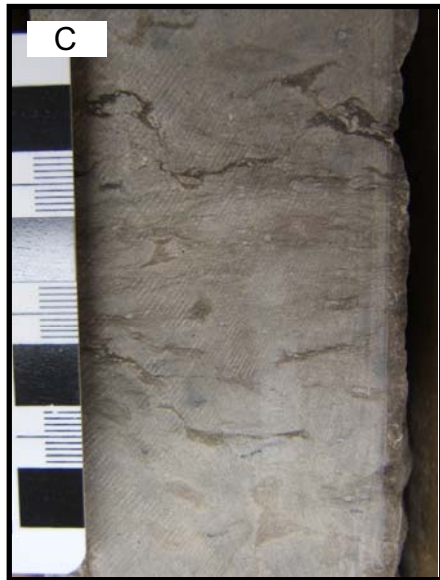
Figure 48. Core and thin section photographs of the Keg River Formation carbonates in the Hansman Lake area. Coarse-grained dolostones (Photo A) with halite-filled vugs change to porous, coarse-grained fossiliferous dolostone (Photo B), which is underlain by a laminated dolomudstone (Photo C). Inter-crystalline and vuggy porosity are predominant and can best be seen in the thin section photograph (Photo D).
