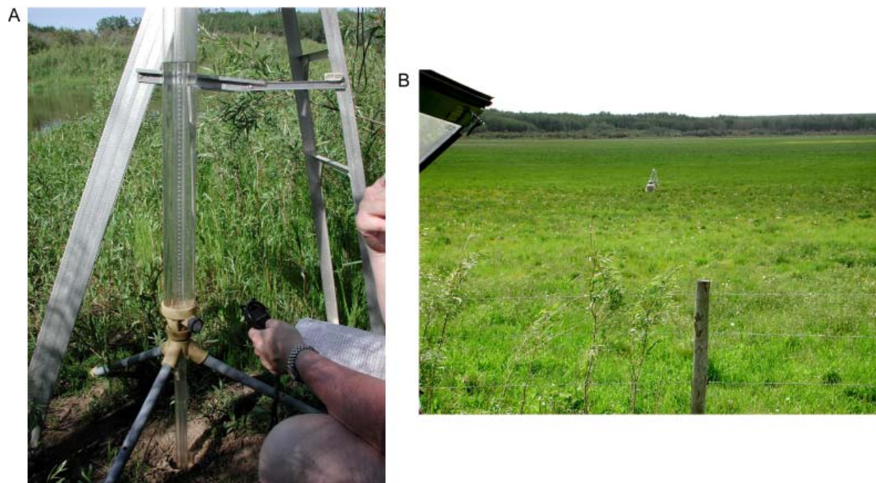
Figure 3.22. Measuring stream-bed and lake-bed permeability in field with Guelph permeameter.
