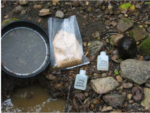
Figure 2. Pre-labelled Kraft paper bags and plastic bottles are used to collect samples of stream silts and stream waters. Flagging tape with a sample site number is used to mark sample sites.
