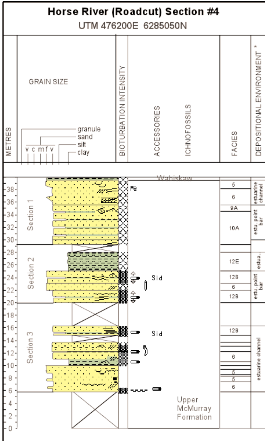
Figure 8.3.6. Schematic representation of the measured Horse River (Roadcut) Section #4 (UTM 476200E, 6285050N). Facies designations as listed in Appendix 2. Vertical scale bars are 1 m in height.
