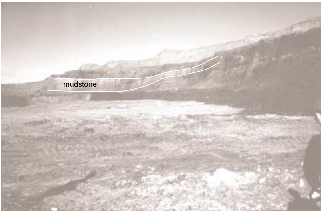
Figure 10.0.3. Mine face displaying muddy abandonment plug within estuarine channel deposits (Suncor Steepbank Mine).
