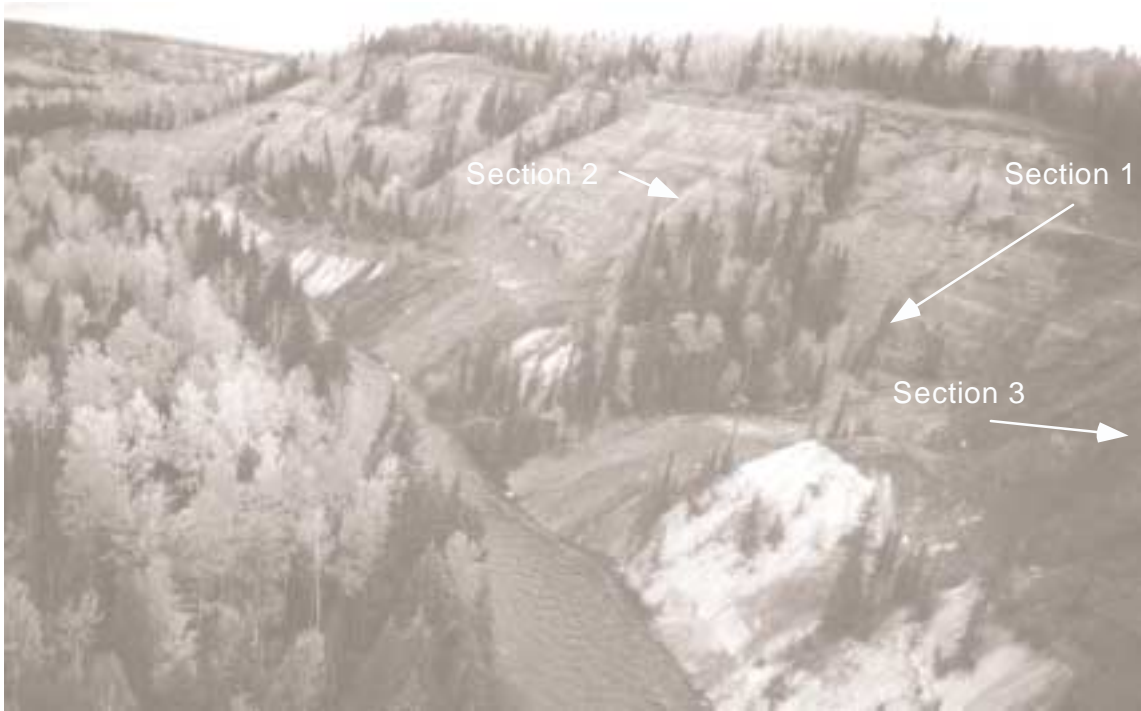
Figure 10.1.4c. Overview of Outcrop #3, showing the Devonian carbonates (white at the base, extending from the lower right corner to the upper left corner of the photo), and McMurray Formation, with access to Sections #3-1 and #3-2 shown by the arrows, Steepbank River.
