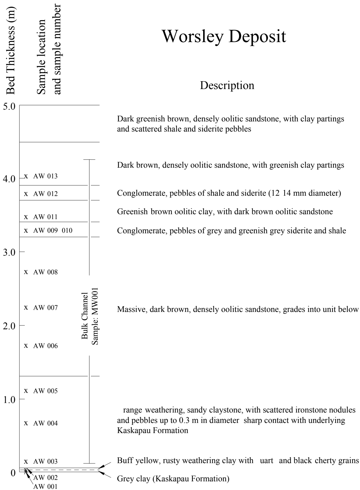
Figure 6. Lithology of the Worsley Deposit (Green and Mellon, 1962 Eccles, unpublished field notes), with sample locations from this study.
