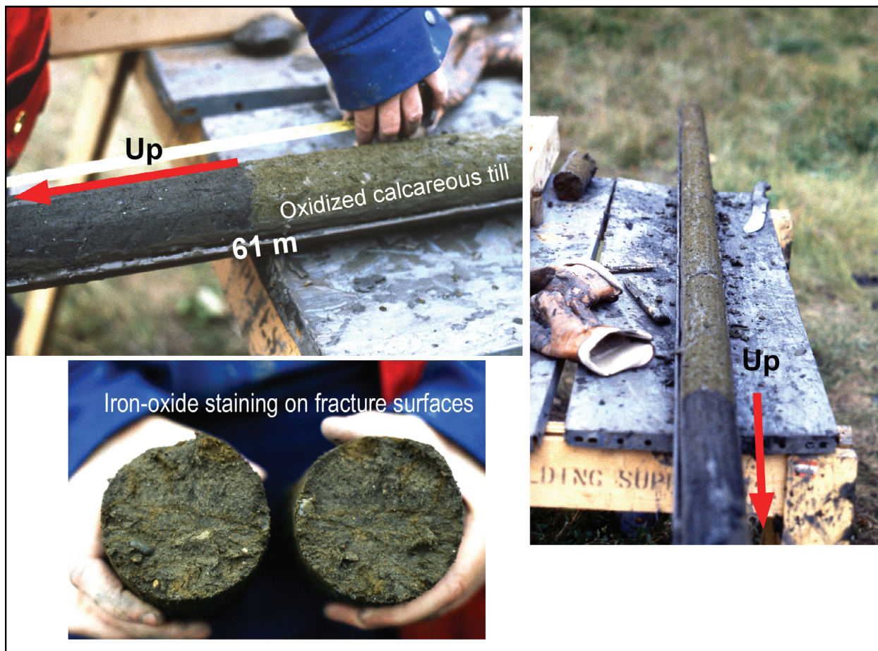
Figure 11. Contact between unoxidized Grand Centre Formation till and oxidized, calcareous Marie Creek Formation till at 61 m depth in borecore WEPA99-1. Both tills are normally magnetized.
