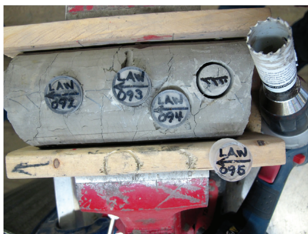
Figure 4. Paleomagnetic sampling procedure: (a) close-up of dry, consolidated sediment archived in core boxes; (b) selecting 7.5 cm diameter representative core segment on which a downhole direction has been marked (WEPA99-2); (c) extraction of 2.5 cm diameter stubs using hand-held drill and circular steel bit (note downhole direction indicated by arrows on wooden cauls and on sediment); (d) insertion of labelled plastic cylinders into stubs of core (WEPA99-2).
