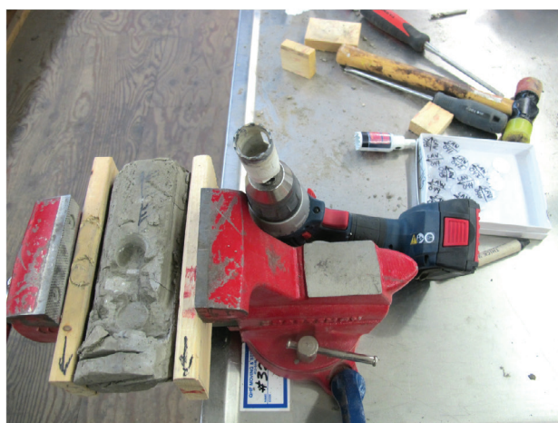
Figure 4. Paleomagnetic sampling procedure: (a) close-up of dry, consolidated sediment archived in core boxes; (b) selecting 7.5 cm diameter representative core segment on which a downhole direction has been marked (WEPA99-2); (c) extraction of 2.5 cm diameter stubs using hand-held drill and circular steel bit (note downhole direction indicated by arrows on wooden cauls and on sediment); (d) insertion of labelled plastic cylinders into stubs of core (WEPA99-2).
