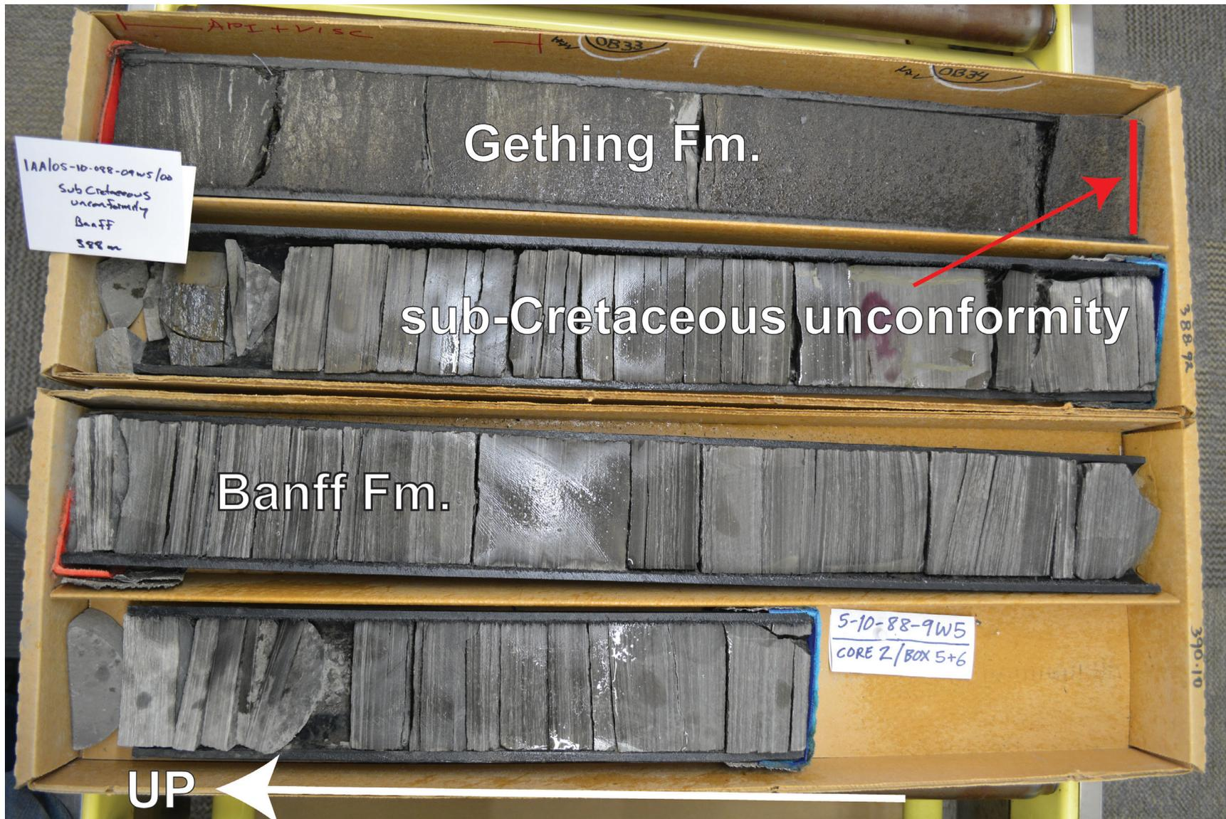
Figure 10. Core photo of well 1AA/05-10-088-09W5/00, with the sub-Cretaceous unconformity surface separating carbonate-rich Banff Formation from overlying Cretaceous Gething Formation argillaceous sandstone.
