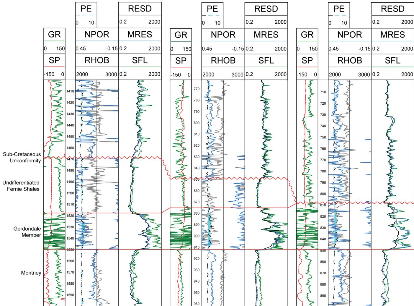
Figure 3. Stratigraphic cross-section (datum=top Montney Formation) with log examples of the Fernie Formation and the sub-Cretaceous unconformity. Log mnemonics are as follows: GR=gamma ray, SP=spontaneous potential, PE=photoelectric effect, NPOR=neutron porosity, RHOB=bulk density, RESD=deep resistivity, MRES=medium resistivity, SFL=shallow resistivity.
