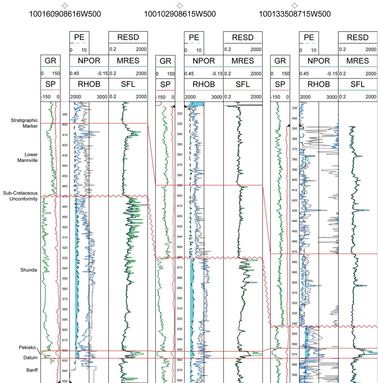
**Figure 6. Stratigraphic cross-section (datum=top Banff Formation) with log examples of the Shunda Formation. Log mnemonics are as follows: GR=gamma ray, SP=spontaneous potential, PE=photoelectric effect, NPOR=neutron porosity, RHOB=bulk density, RESD=deep resistivity, MRES=medium resistivity, SFL=shallow resistivity.**
