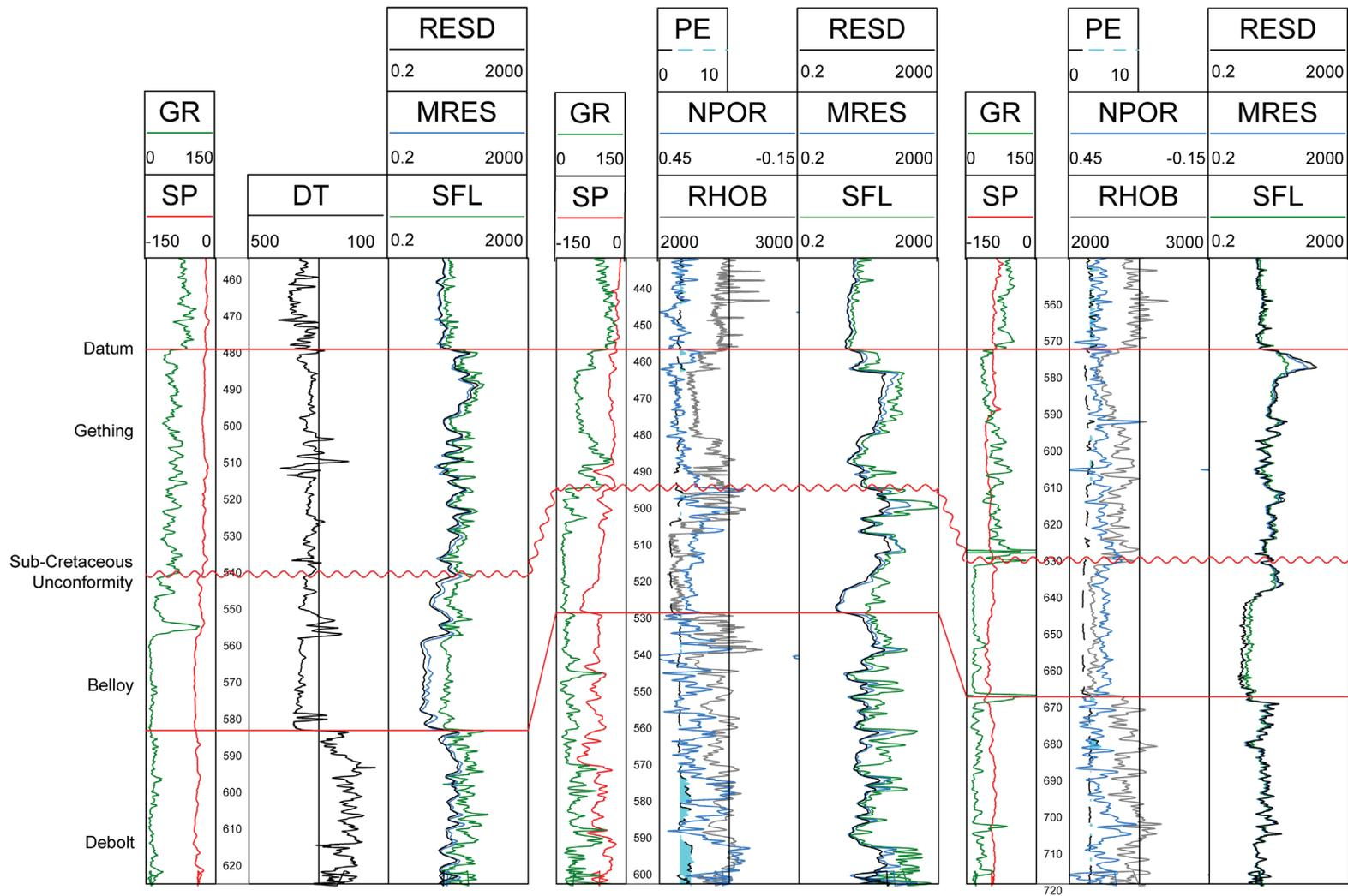
Figure 4. Stratigraphic cross-section (datum=top Gething Formation) with log examples of the Belloy Formation. Log mnemonics are as follows: GR=gamma ray, SP=spontaneous potential, DT=sonic travel time, PE=photoelectric effect, NPOR=neutron porosity, RHOB=bulk density, RESD=deep resistivity, MRES=medium resistivity, SFL=shallow resistivity.
