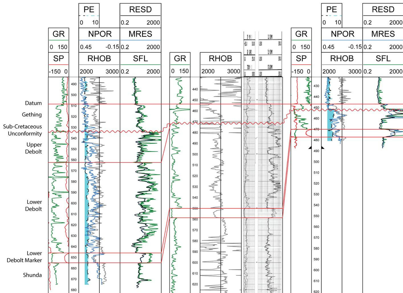
Figure 5. Stratigraphic cross-section (datum=top Gething Formation) with log examples of the Debolt Formation. Log mnemonics are as follows: GR=gamma ray, SP=spontaneous potential, PE=photoelectric effect, NPOR=neutron porosity, RHOB=bulk density, RESD=deep resistivity, MRES=medium resistivity, SFL=shallow resistivity.
