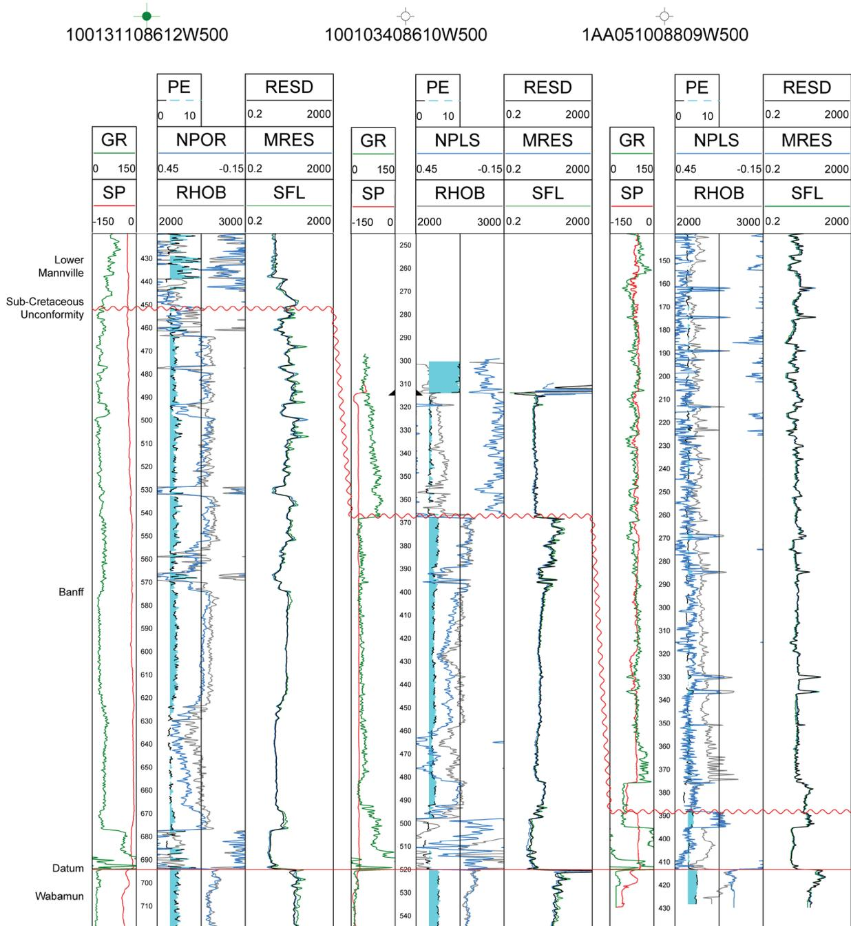
**Figure 8. Stratigraphic cross-section (datum=top Wabamun Formation) with log examples of the Banff Formation. Log mnemonics are as follows: GR=gamma ray, SP=spontaneous potential, PE=photoelectric, NPOR=neutron porosity, NPLS=neutron porosity limestone, RHOB=bulk density, RESD=deep resistivity, MRES=medium resistivity, SFL=shallow resistivity.**
