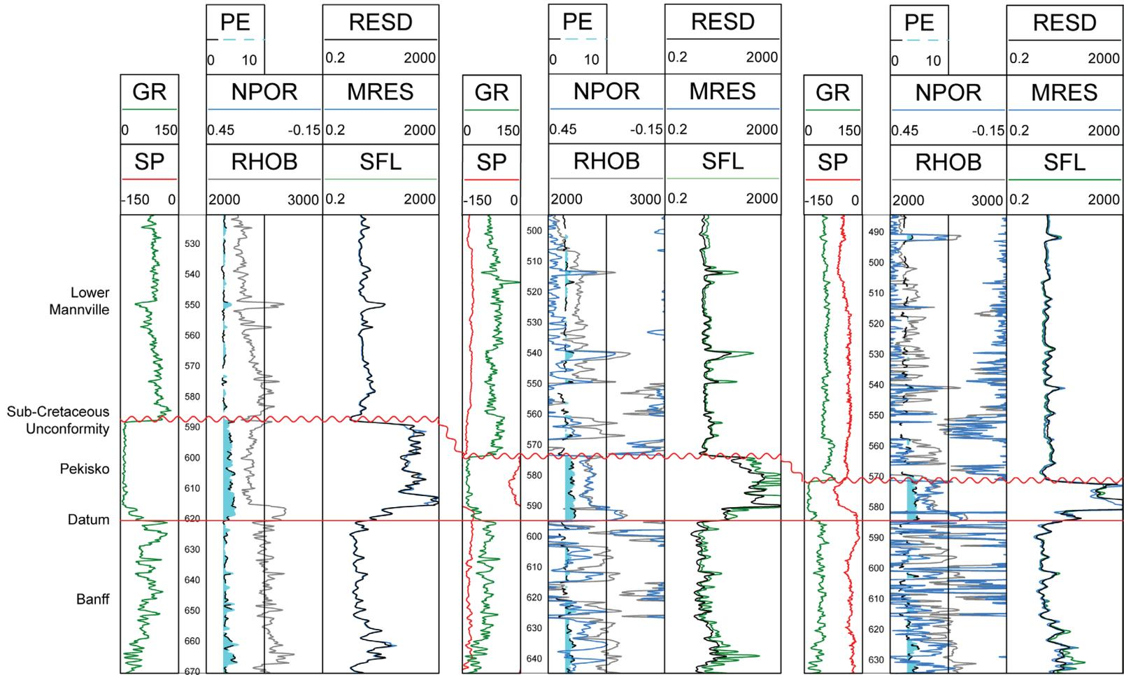
Figure 7. Stratigraphic cross-section (datum=top Banff Formation) with log examples of the Pekisko Formation. Log mnemonics are as follows: GR=gamma ray, SP=spontaneous potential, PE=photoelectric effect, NPOR=neutron porosity, RHOB=bulk density, RESD=deep resistivity, MRES=medium resistivity, SFL=shallow resistivity.
