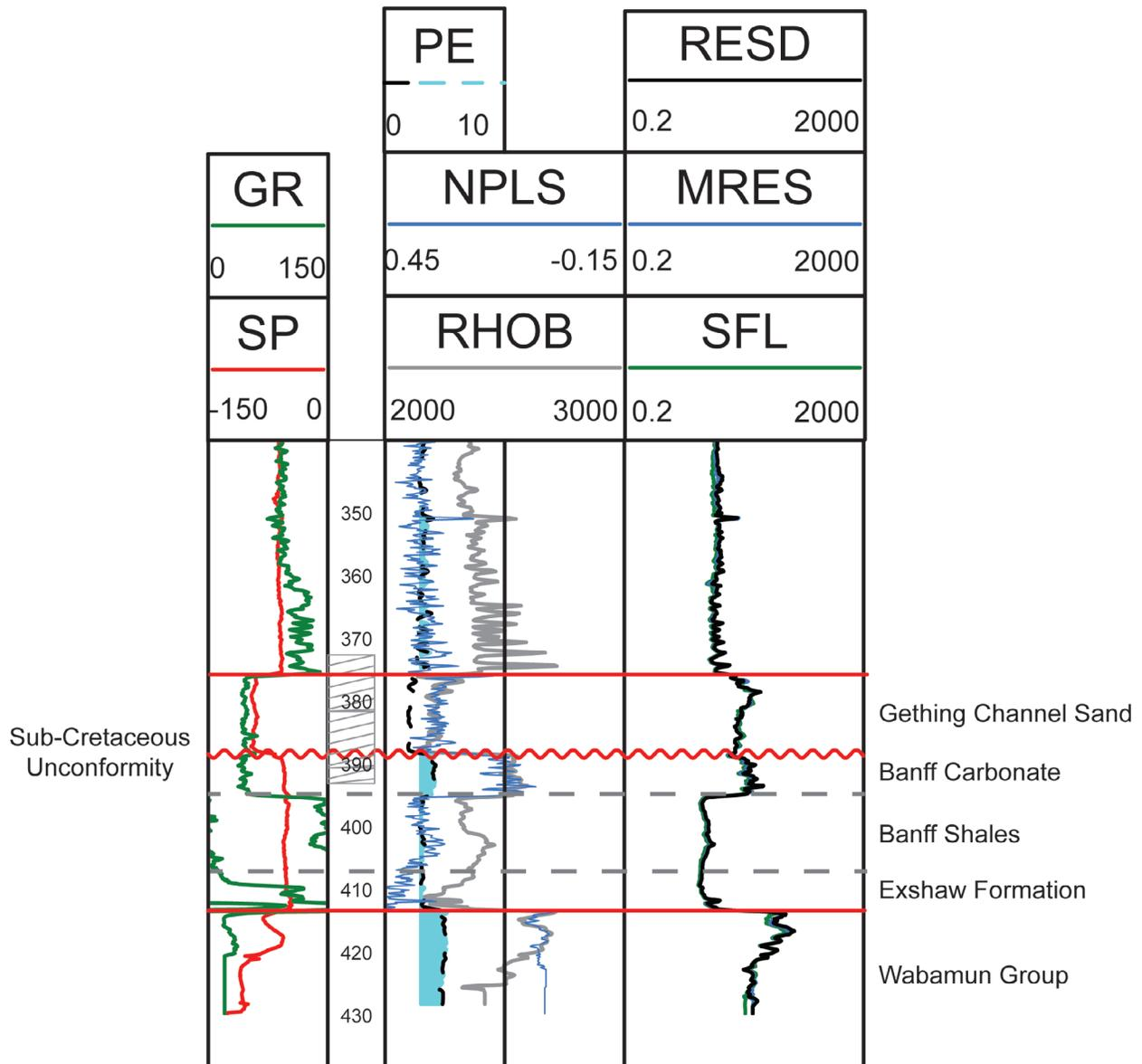
Figure 9. Digital logs of well 1AA/05-10-088-09W5/00, highlighting complexity in picking the sub-Cretaceous unconformity surface. The unconformity is placed at 388 mKB based on distinct changes in PE, RHOB, NPLS, and SP readings. Log mnemonics are as follows: GR=gamma ray, SP=spontaneous potential, PE=photoelectric effect, NPLS=neutron porosity limestone, RHOB=bulk density, RESD=deep resistivity, MRES=medium resistivity, SFL=shallow resistivity.
