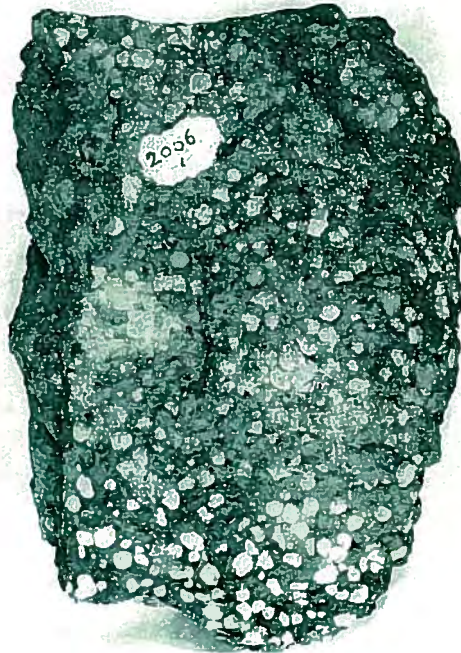
Figure 8—Blairmorite; light colored analcite crystals in a green fine-grained tuffaceous matrix; Crowsnest formation.
