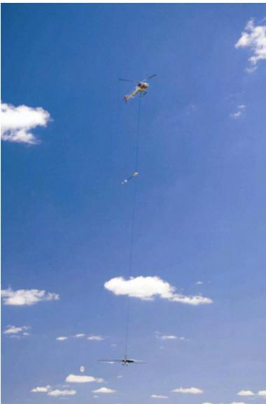
When the secondary field spreads out in space, it is "seen" by a measuring device (a coil receiver) and analysed either separately (as in most time domain techniques) or together with the primary field (as in all frequency domain techniques). The analysis results in products defining the conductivity distribution of the earth, which can be used to map geology.
