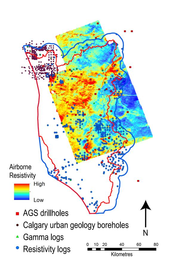
**Data Sources:** Airborne resistivity, historical mapping, historical drilling, borehole logs (AGS holdings, water well drillers, resistivity logs, gamma logs)
