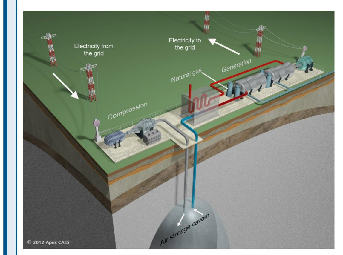
**Figure 2.** Schematic of a CAES facility (from APEX CAES, 2012)
