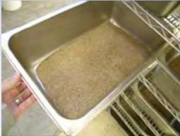
↳ 0.25mm to 1mm are transferred to pre-labeled stainless steel pans and placed in an oven to dry.
