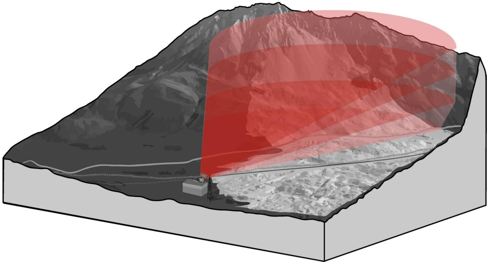
**Figure 2. Overview, as of December 2021, of the primary monitoring equipment at Turtle Mountain, southwestern Alberta. The drawing marks the location of the LiSAMobile system, and the red beam depicts the scanning of the mountain. The light grey area represents the extent of the original 1903 slide. The image is not drawn to scale, and its purpose is to highlight the area LiSAMobile scans.**
