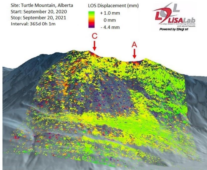
**Figure 7. The line-of-sight (LOS) three-dimensional (3D) displacement map of Turtle Mountain, southwestern Alberta, shows the annual analysis of large block movements near regions A and C, from September 20, 2020, to September 20, 2021 (365 days, 0 hours, 1 minute).**
