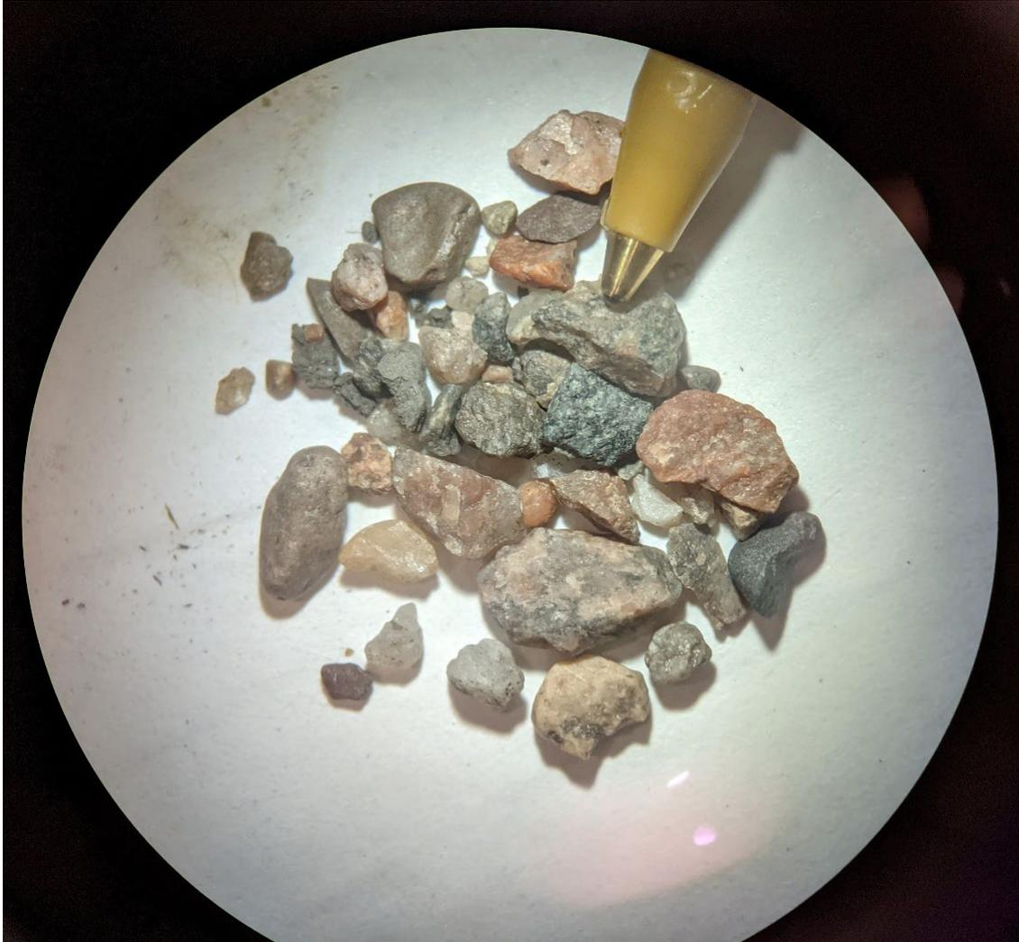
**Figure 22. View through microscope at sample from oil and gas well 10-4-123-2W6 from 290 to 300 ft. (88.4–91.4 m) depth. Note mixed lithologies of angular fragments. Pen tip for scale.**
