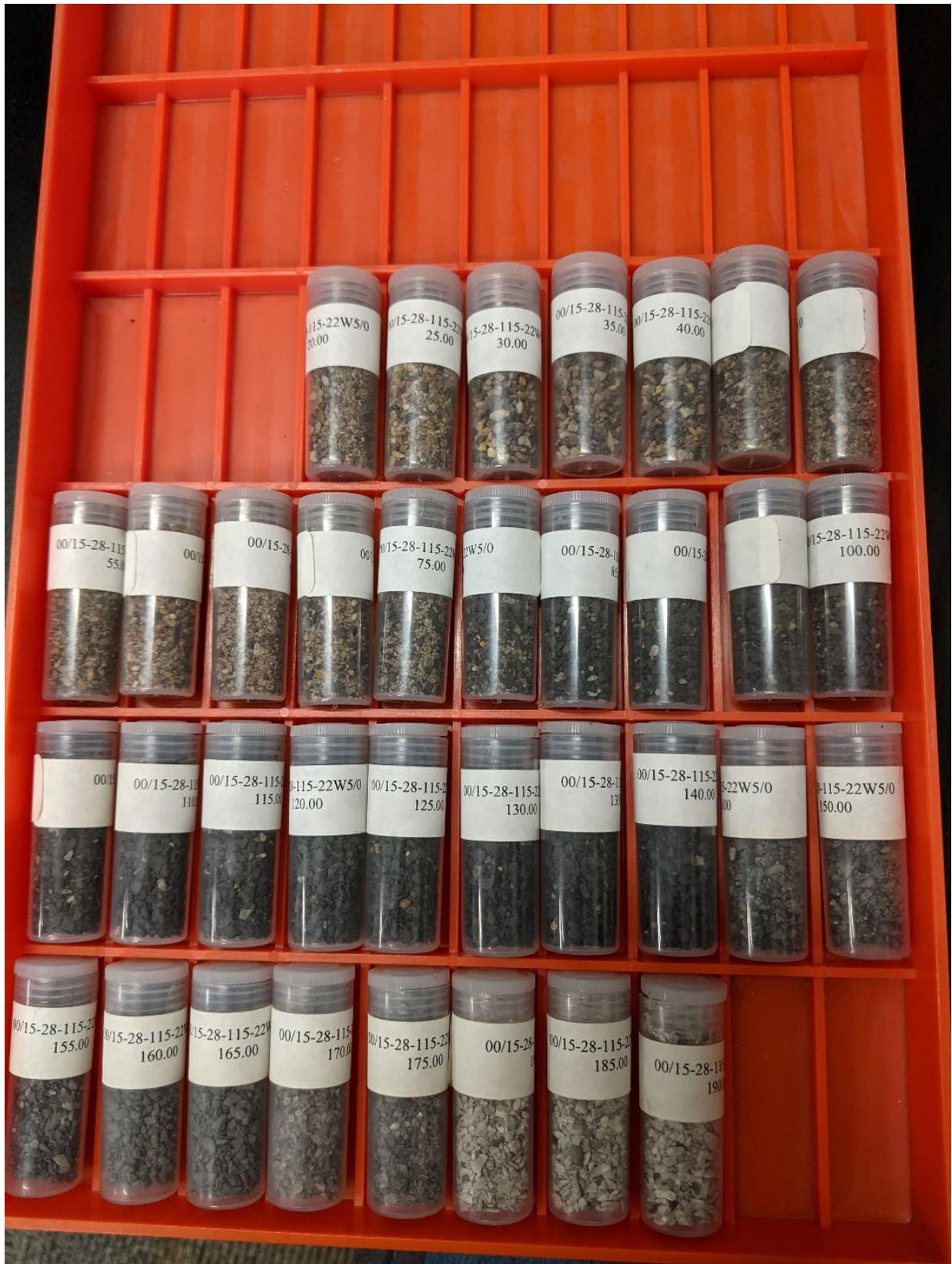
Figure 18. Tray of drill cuttings from oil and gas well 00/15-28-115-22W5/0. Samples from 20 to 195 m depth, each vial contains 5 m depth range.
