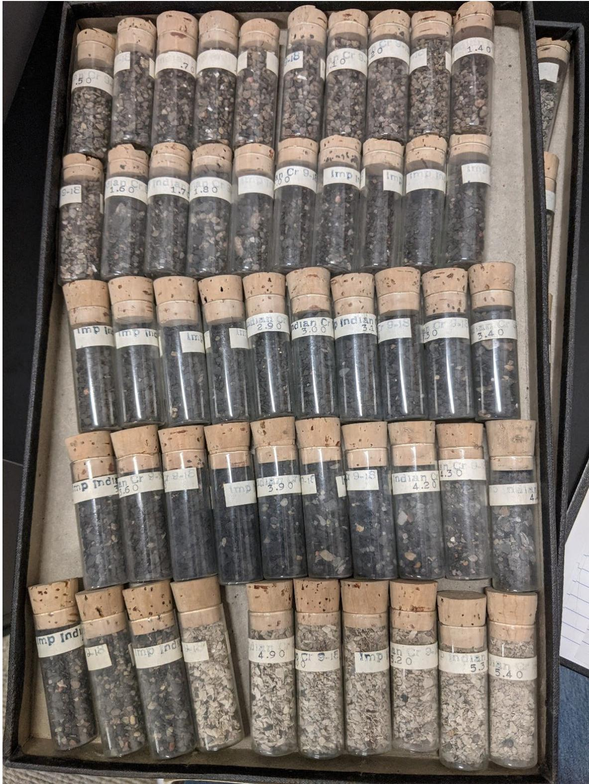
**Figure 24. Tray of drill cuttings from oil and gas well 9-18-118-21W5. Samples from 50 to 550 ft. (15.2–167.6 m) depth, each vial contains 10 ft. (3.0 m) depth range. Bottom right seven vials contain limestone (480–550 ft. [146.3–167.6 m]), top row vials and first vial of second row contain mixed lithologies (50–160 ft. [15.2–48.8 m]).**
