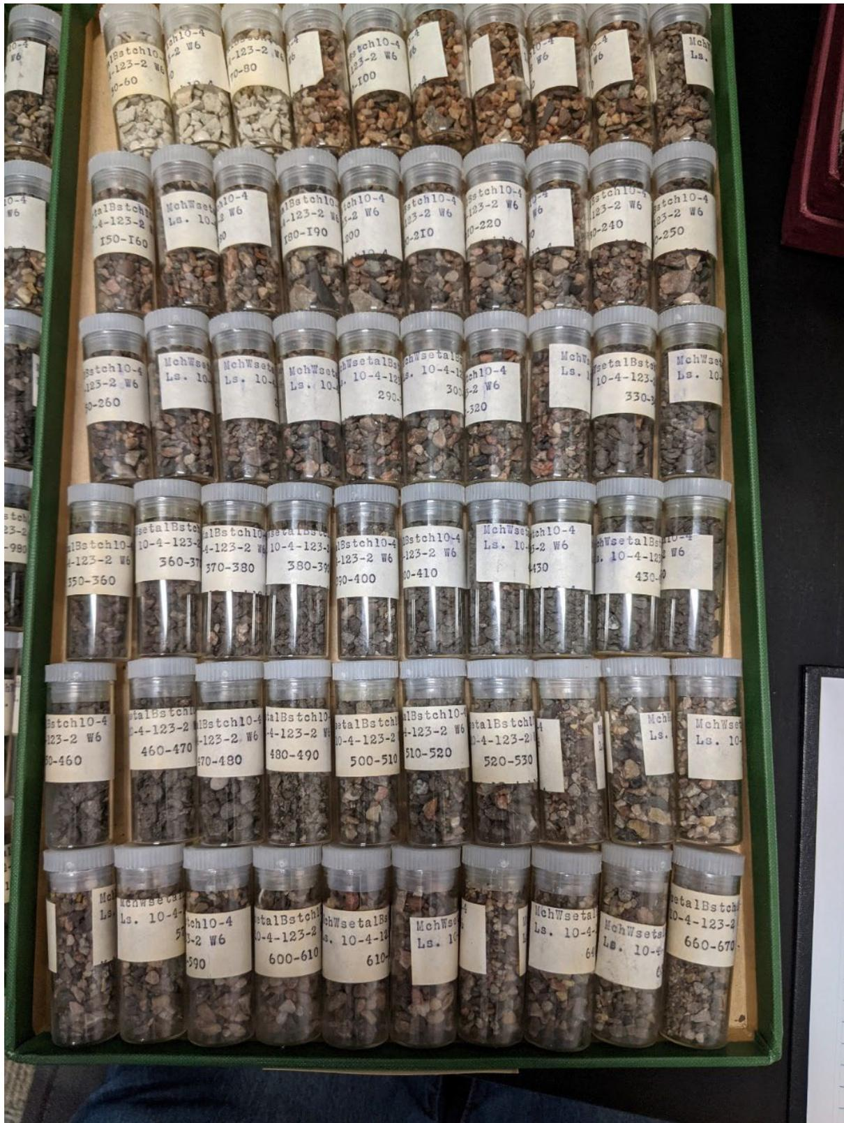
Figure 20. Tray of drill cuttings from oil and gas well 10-4-123-2W6. Samples from 50 to 670 ft. (15.2–204.2 m) depth, each vial contains 10 ft. (3.0 m) depth range. Note first three vials (from top left) contain cement (casing) fragments.
