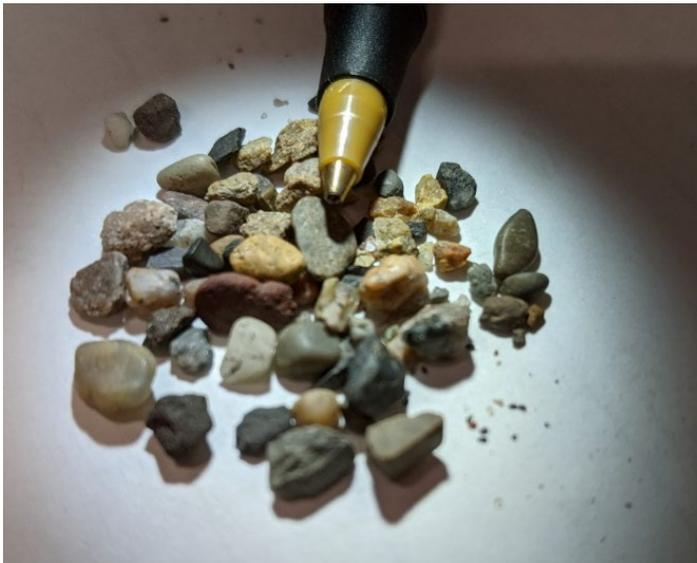
**Figure 4. Rounded pebbles of mixed lithologies from drill cuttings from oil and gas well 10-4-123-2W6 at a depth of 800–810 ft. (243.8–246.9 m). These are interpreted to be of fluvial or glaciofluvial origin.**
