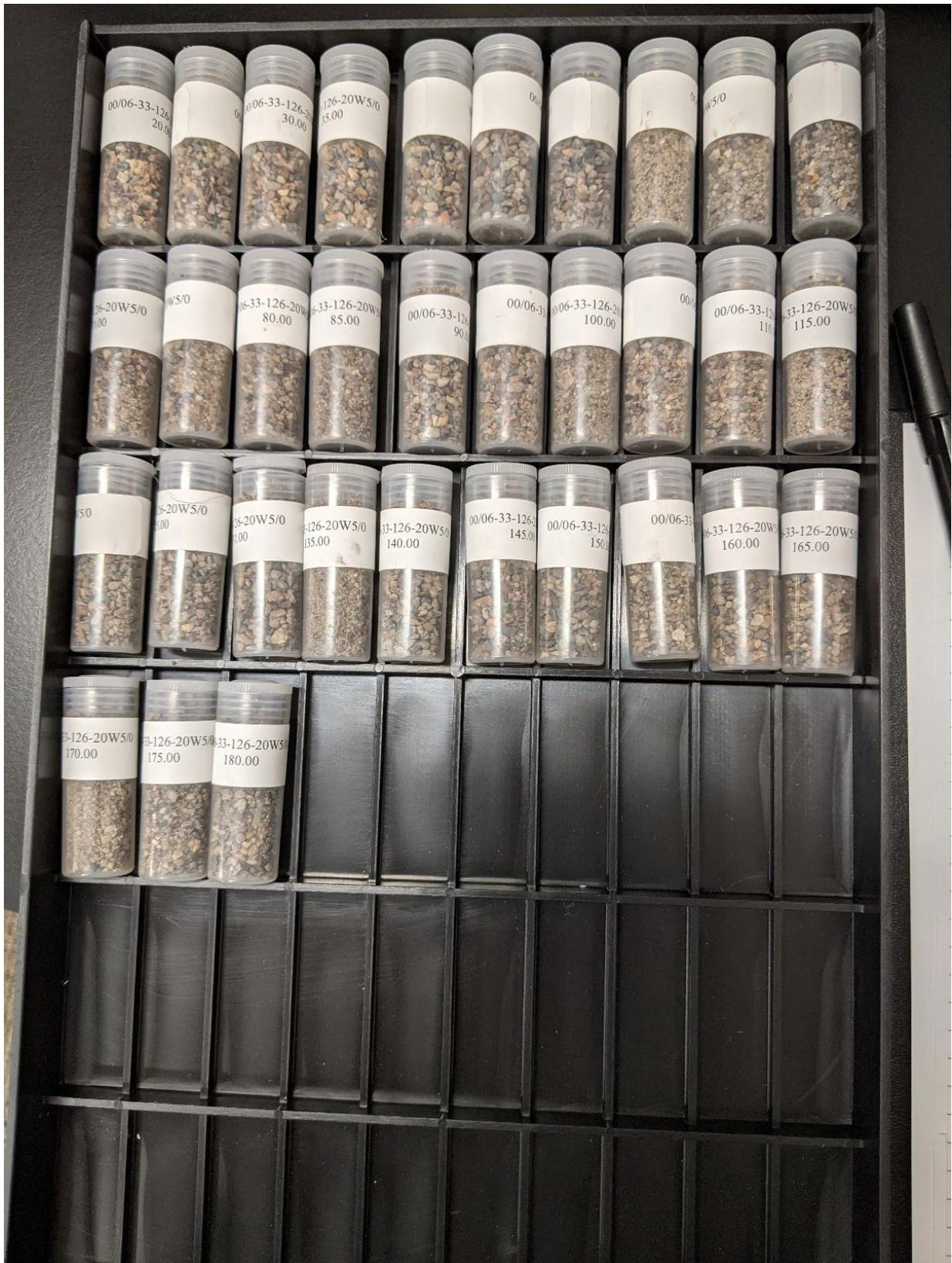
Figure 16. Tray of drill cuttings from oil and gas well 00/06-33-126-20W5/0. Samples from 20 to 185 m depth, each vial contains 5 m depth range.
