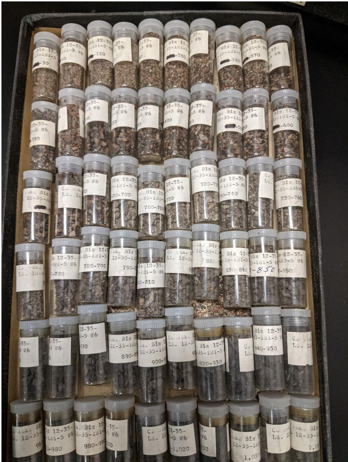
Figure 14. Tray of drill cuttings from oil and gas well 12-35-121-5W6. Samples from 0 to 1060 ft. (0–323.1 m) depth. For depths from 0 to 690 ft. (0–210.3 m), each vial contains 30 ft. (9.1 m) depth range and from 690 to 1060 ft. (210.3–323.1 m), each vial contains 10 ft. (3.0 m) depth range.
