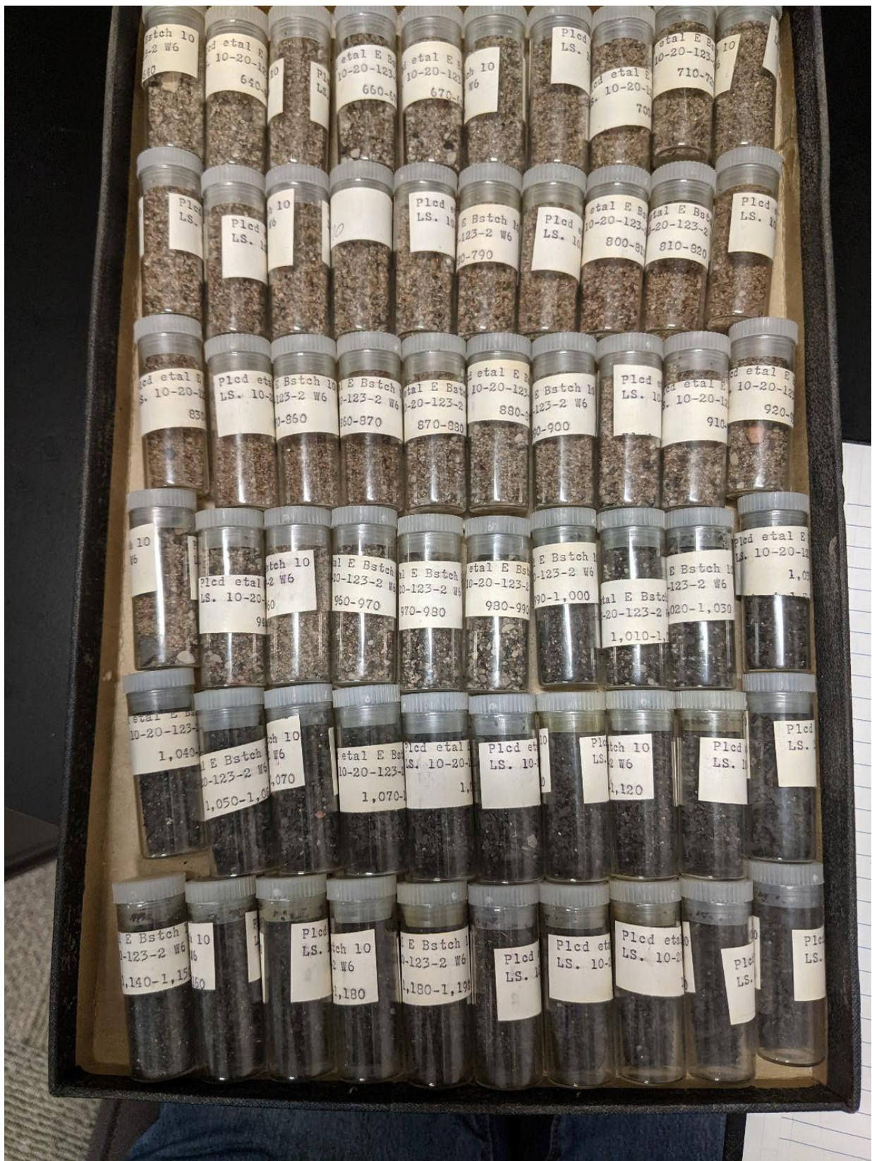
Figure 19. Tray of drill cuttings from oil and gas well 10-20-123-2W6. Samples from 630 to 1240 ft. (192.0–378.0 m) depth, each vial contains 10 ft. (3.0 m) depth range.
