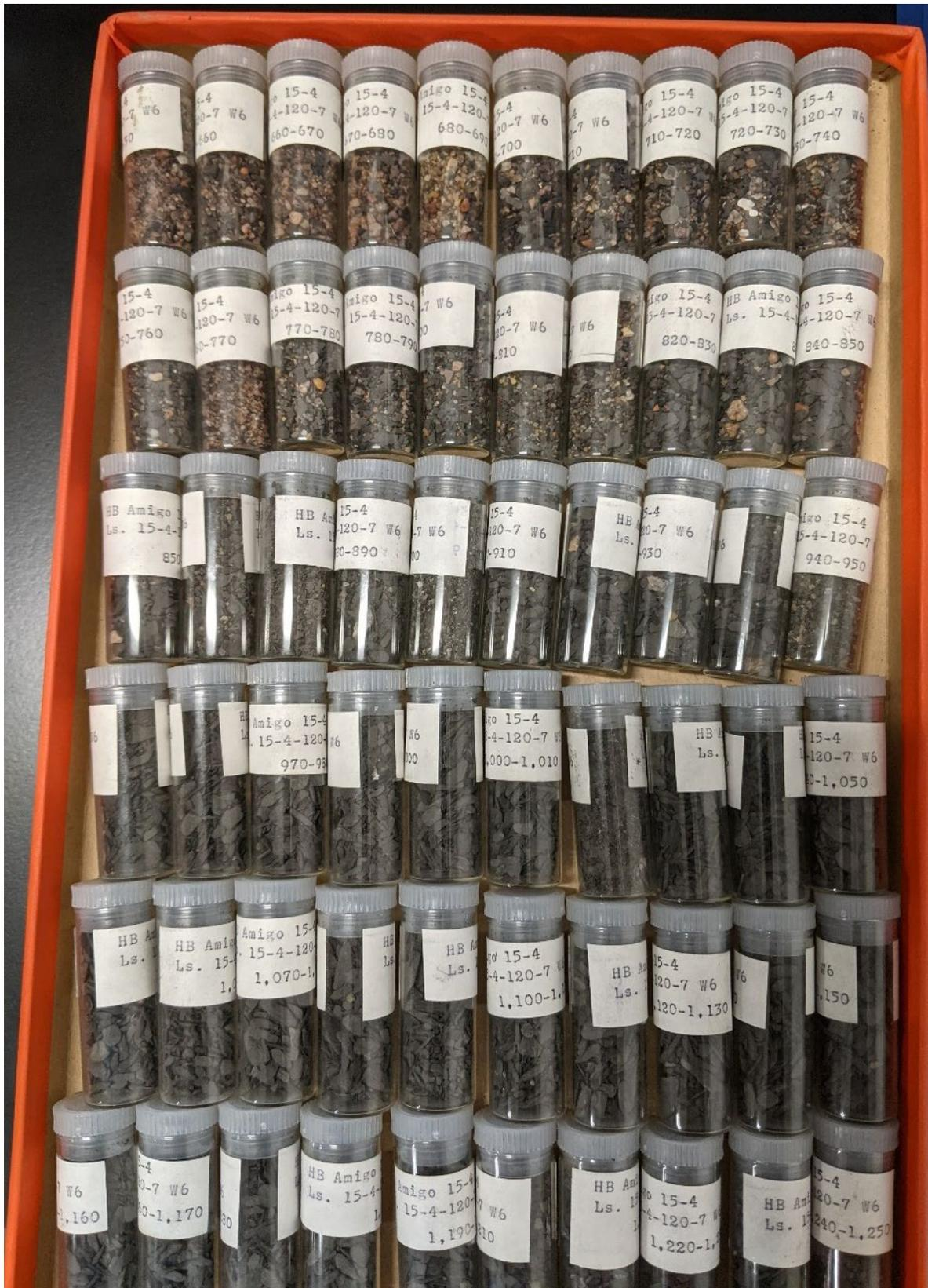
Figure 32. Tray of drill cuttings from oil and gas well 15-4-120-7W6. Samples from 640 to 1250 ft. (195.1–381.0 m) depth, each vial contains 10 ft. (3.0 m) depth range.
