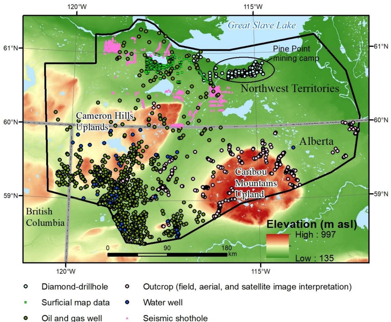
**Figure 3. Location of data compiled from sources to evaluate bedrock topography and sediment thickness. See Utting et al. (2023) for complete list of data sources. Regional physiographic features (Pettapiece, 1986) are highlighted. Elevation data from U.S. Geological Survey and National Geospatial-Intelligence Agency (2010).**
