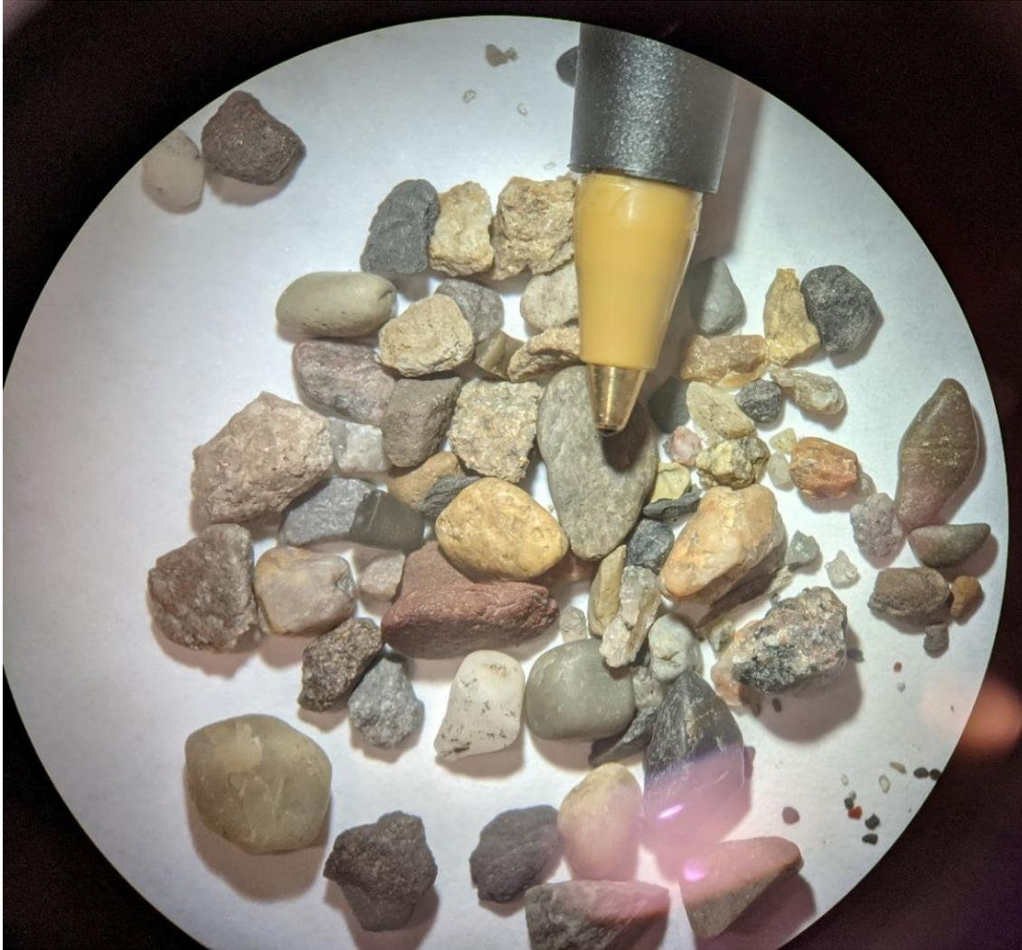
**Figure 23. View through microscope at sample from oil and gas well 10-4-123-2W6 from 800 to 810 ft. (243.8–246.9 m) depth. Note mixed lithologies of rounded to subrounded pebbles. Pen tip for scale.**
