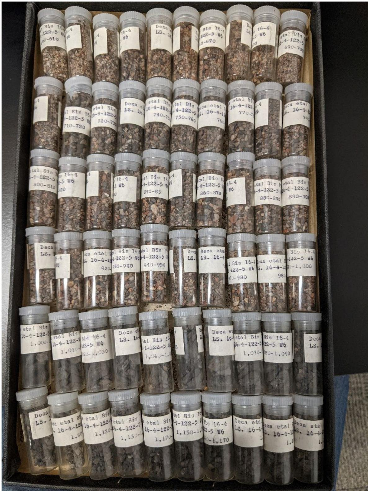
Figure 13. Tray of drill cuttings from oil and gas well 16-4-122-5W6. Darker material in last two rows are shale fragments interpreted as bedrock. The second row contains a higher proportion of shale fragments and is interpreted to be related to a raft (block) of shale. Samples from 600 to 1200 ft. (182.9–365.8 m) depth, each vial contains 10 ft. (3 m) depth range.
