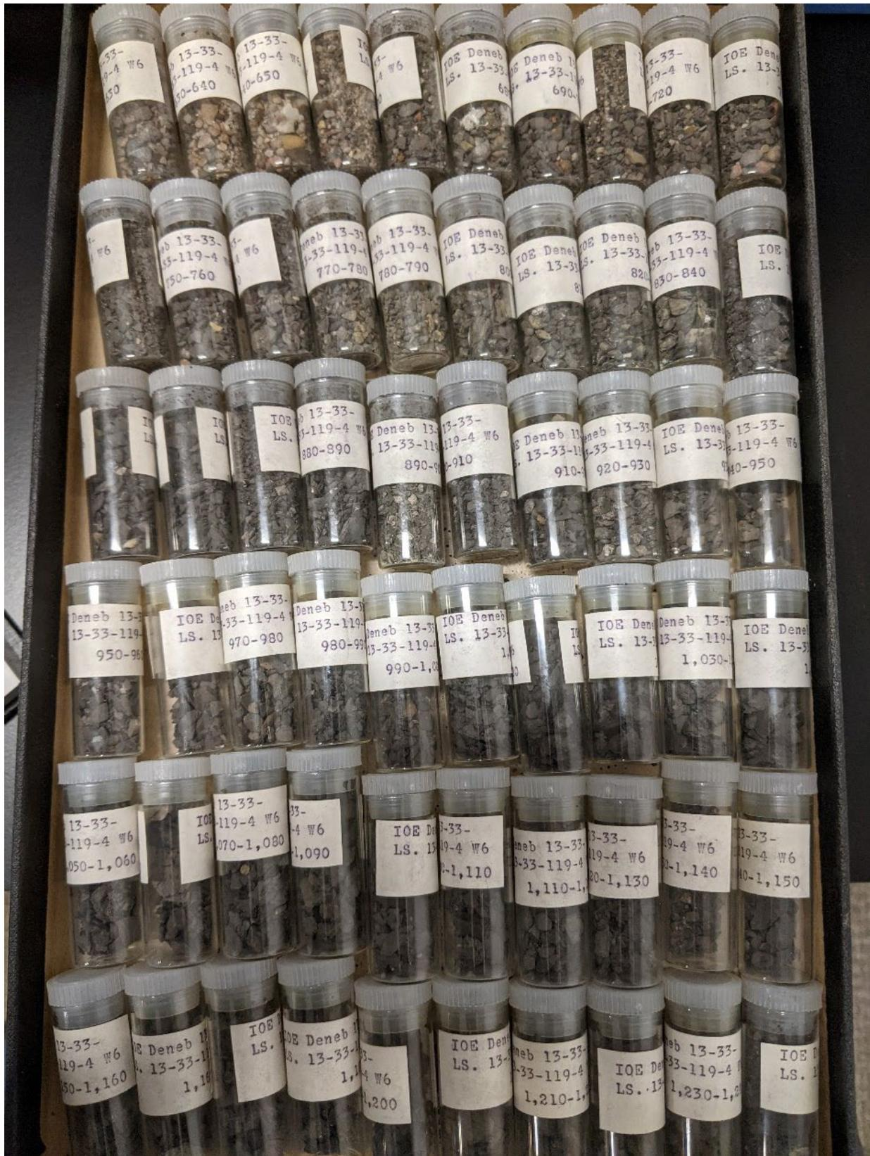
Figure 15. Tray of drill cuttings from oil and gas well 13-33-119-4W6. Samples from 620 to 1250 ft. (189.0–381.0 m) depth, each vial contains 10 ft. (3.0 m) depth range.
