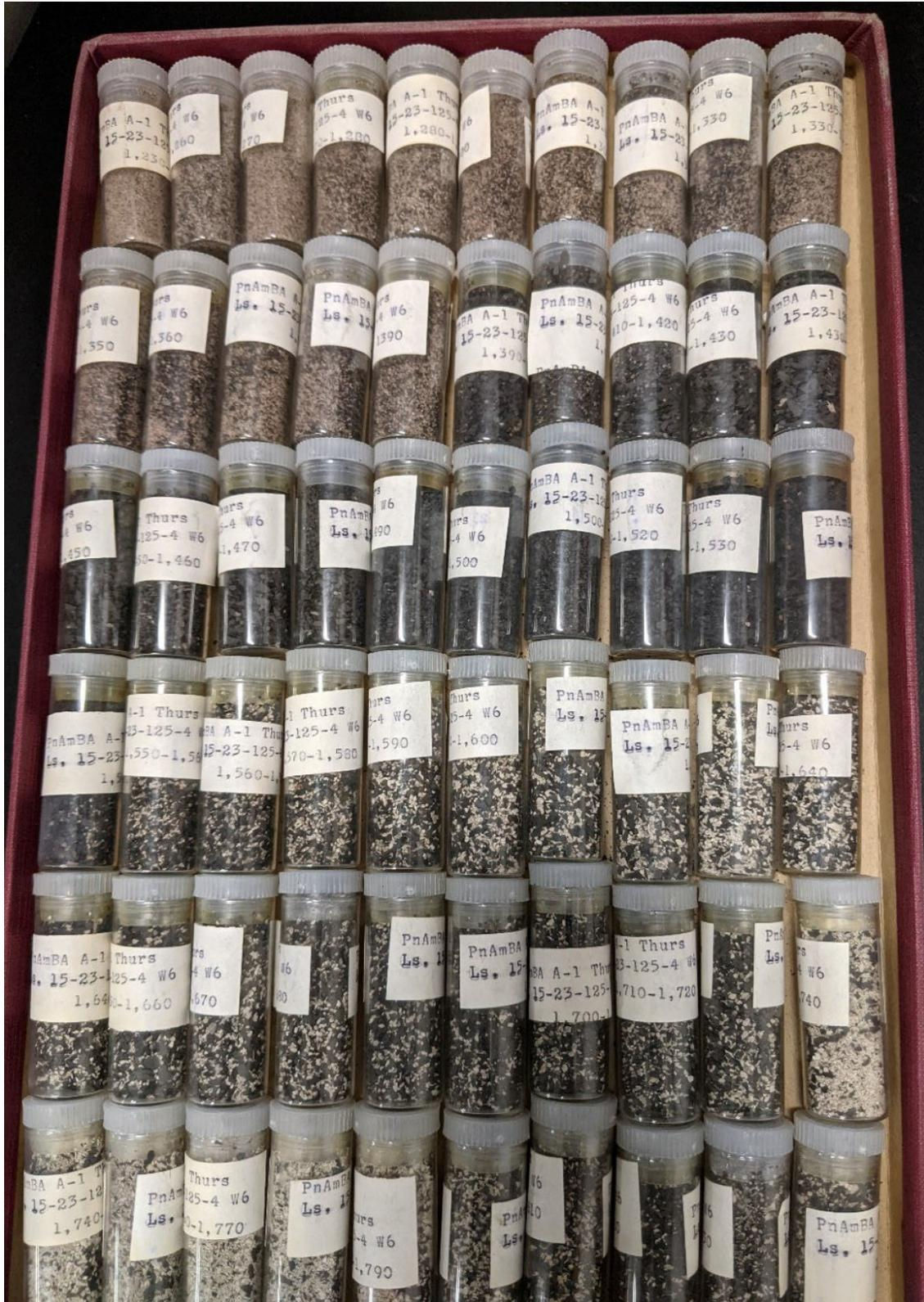
Figure 27. Tray of drill cuttings from oil and gas well 15-23-125-4W6. Samples from 1230 to 1840 ft. (374.9–560.8 m) depth, each vial contains 10 ft. (3.0 m) depth range. Shale encountered at 1390 ft. (423.7 m; dark material halfway in second row). Limestone mixed with shale on the 4<sup>th</sup> to 6<sup>th</sup> rows.
