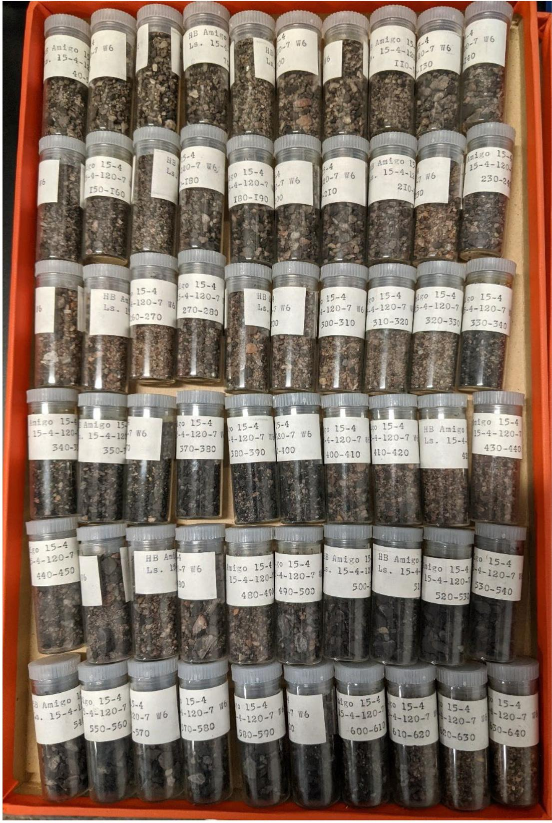
Figure 31. Tray of drill cuttings from oil and gas well 15-4-120-7W6. Samples from 40 to 640 ft. (12.2–195.1 m) depth, each vial contains 10 ft. (3.0 m) depth range.
