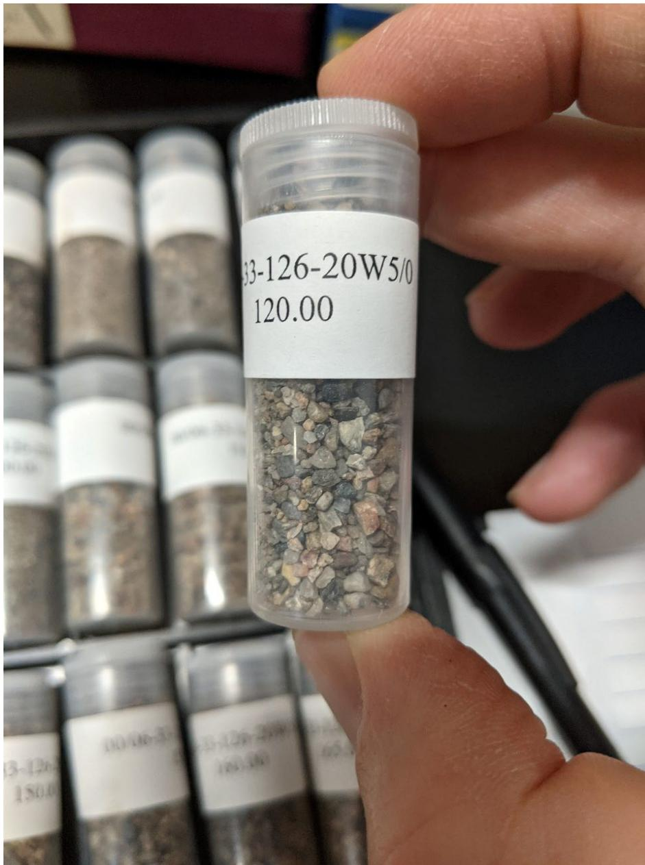
**Figure 17. Drill cuttings from oil and gas well 00/06-33-126-20W5/0 from 120 to 125 m depth, note mixed lithologies and angularity of fragments.**
