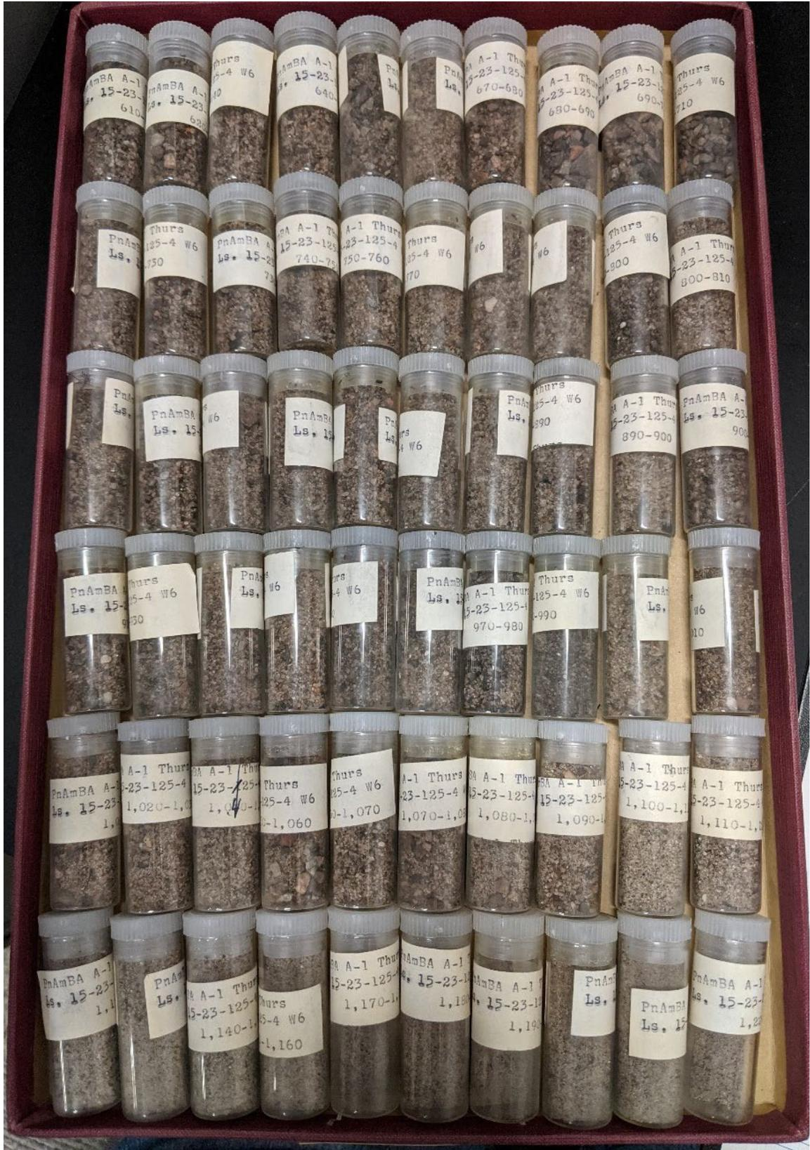
Figure 26. Tray of drill cuttings from oil and gas well 15-23-125-4W6. Samples from 610 to 1230 ft. (185.9–374.9 m) depth, each vial contains 10 ft. (3.0 m) depth range.
