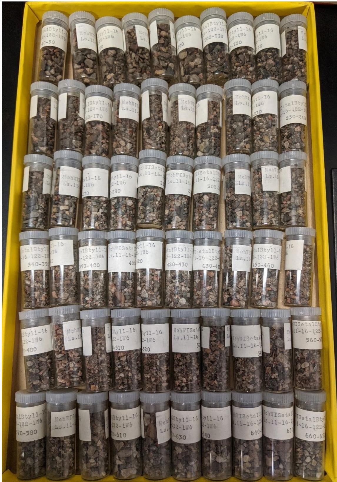
Figure 28. Tray of drill cuttings from oil and gas well 11-16-122-1W6. Samples from 40 to 670 ft. (12.2–204.2 m) depth, each vial contains 10 ft. (3.0 m) depth range.
