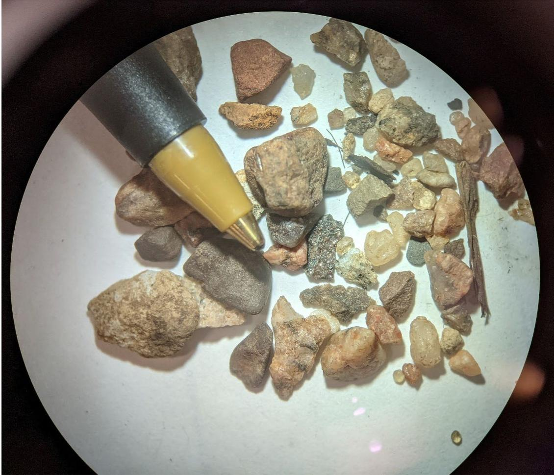
**Figure 21. View through microscope at sample from oil and gas well 10-4-123-2W6 from 100 to 110 ft. (30.5–33.5 m) depth. Note subrounded pebbles of mixed lithologies. Sample includes some wood fragments. Pen tip for scale.**
