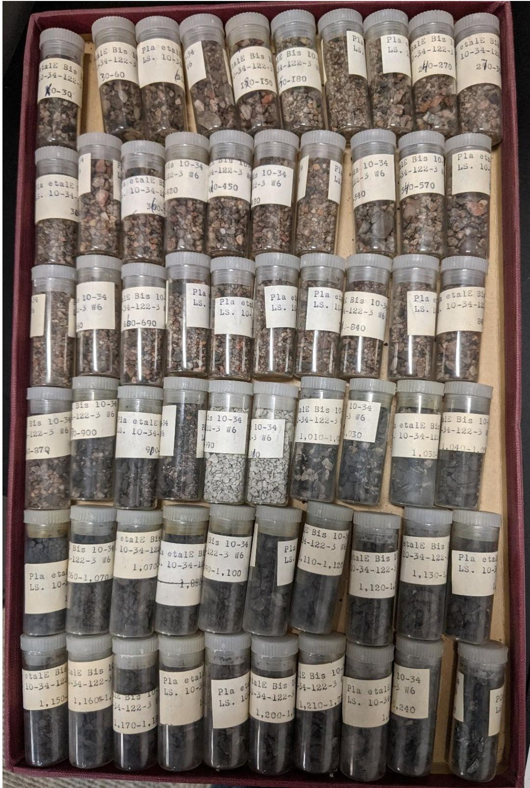
Figure 25. Tray of drill cuttings from oil and gas well 10-34-122-3W6. Samples from 0 to 1250 ft. (0–381.0 m) depth. For depths from 0 to 990 ft. (0–301.8 m), each vial contains 30 ft. (9.1 m) depth range and from 990 to 1250 ft. (301.8–381.0 m), each vial contains 10 ft. (3.0 m) depth range.
