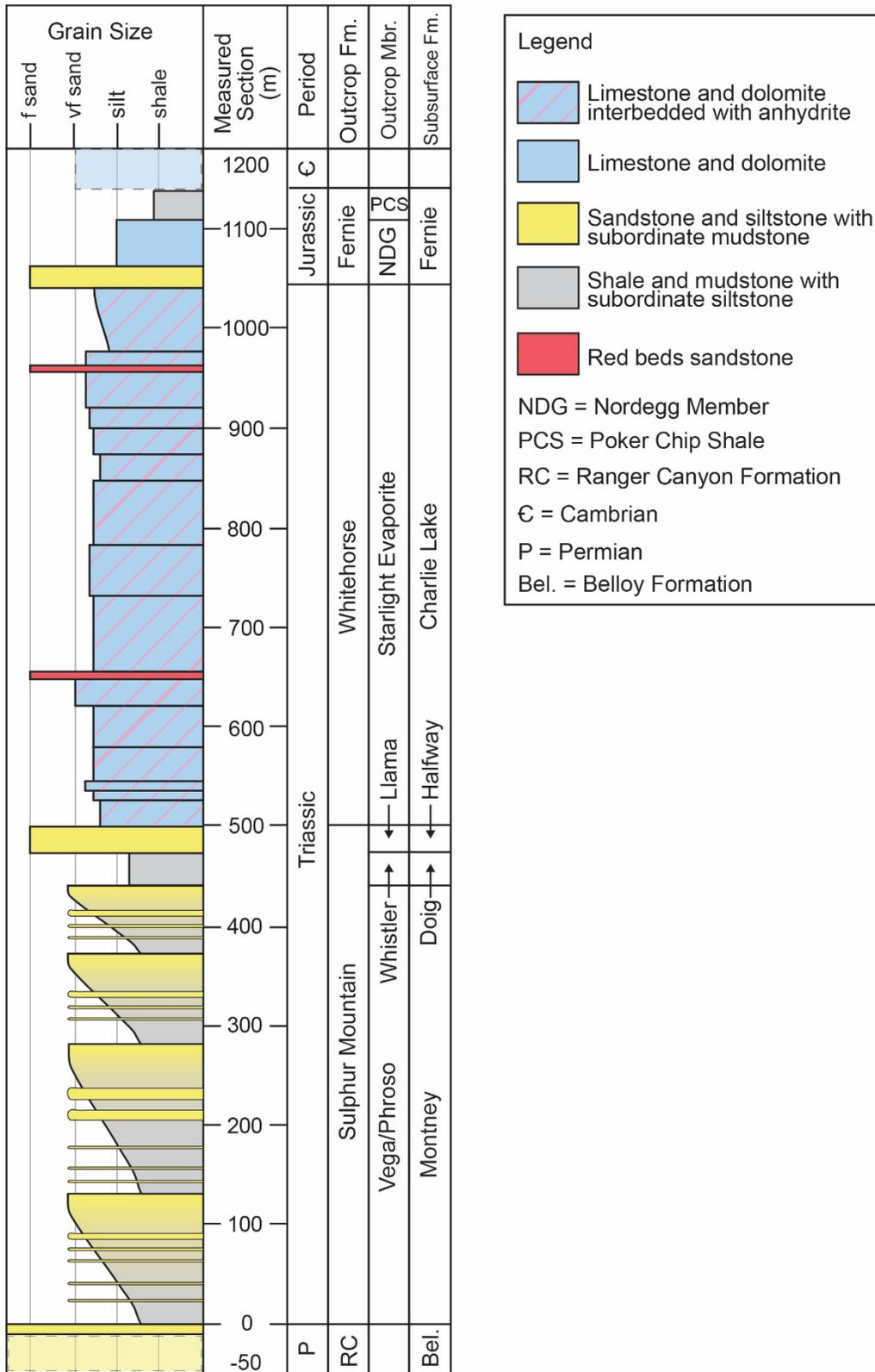
**Figure 4. Stratigraphic log for the Spray River Group at Elliott Peak, central Alberta. Abbreviations: f, fine; vf, very fine.**
