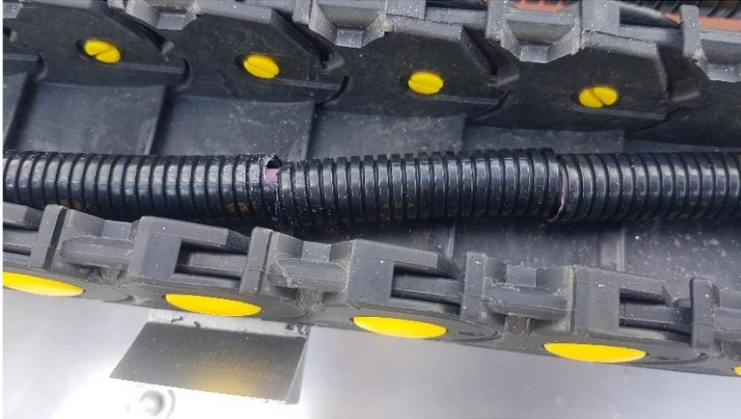
**Figure 3. Damaged chain cable had cut into the data cable causing it to fail.**
