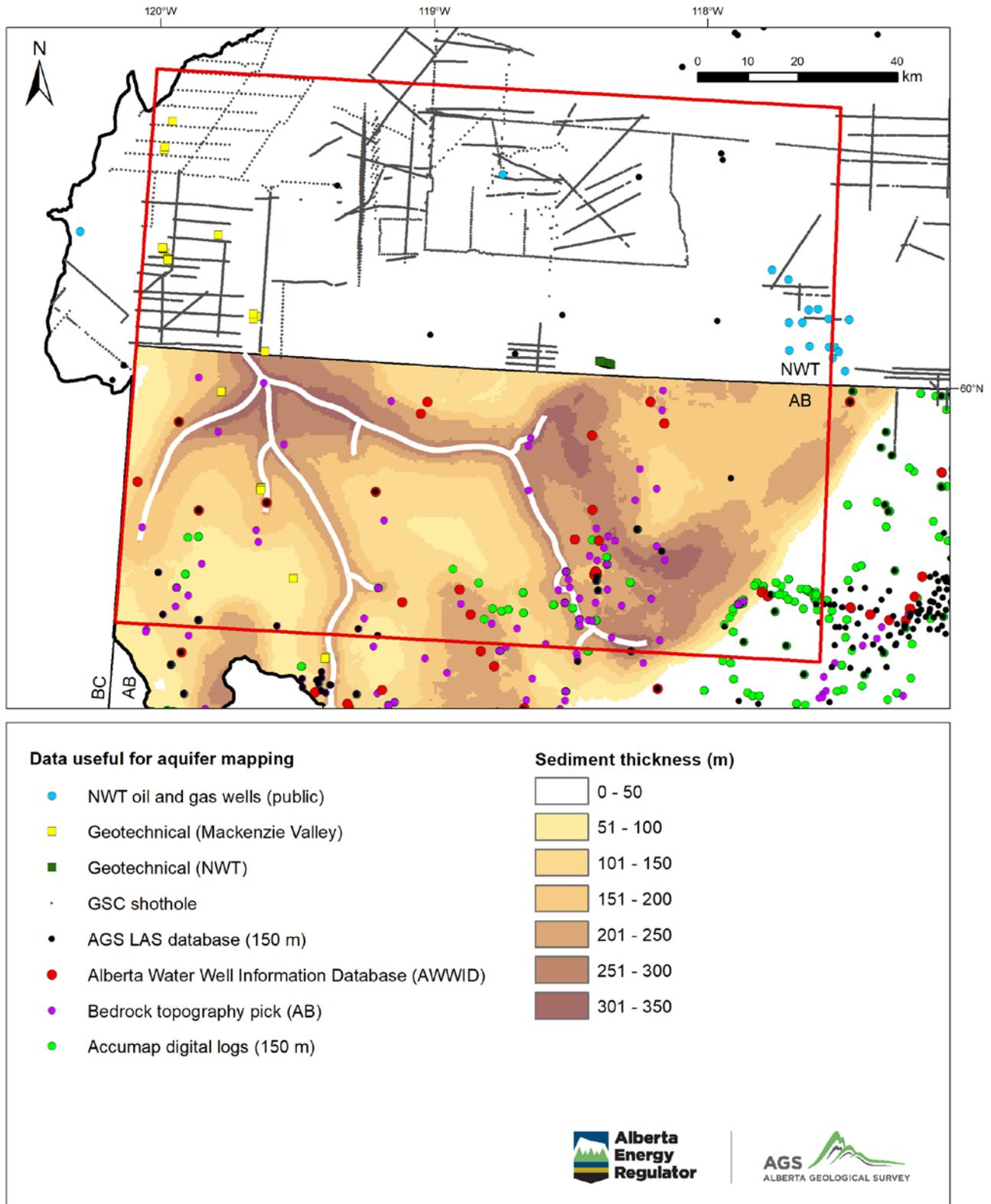
**Figure 8. Detailed view of subsurface information in the Kakisa–Cameron Hills area. Compared to Figure 6, a greater sediment thickness interval is shown to highlight the potential major buried valleys in Alberta.**
