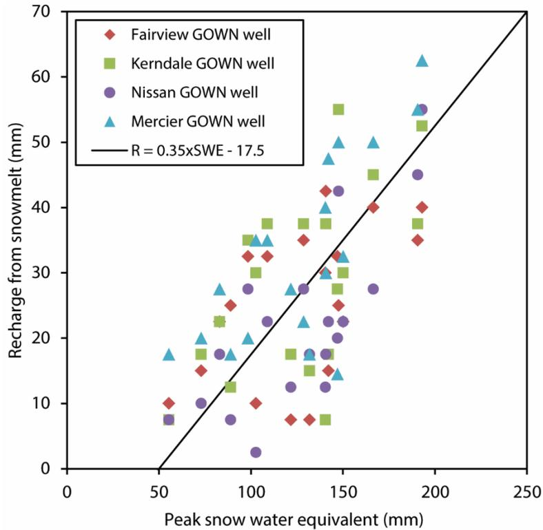
**Figure 6. Summary of groundwater recharge calculated from observed groundwater level rises (Figure 5a) relative to the maximum amount of water contained within the snowpack during the same year.**
