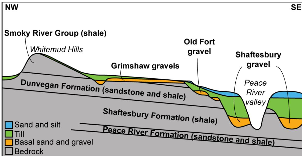
Figure 3. Conceptual geological cross-section identifying the location and elevation of the Grimshaw, Old Fort and Shaftesbury gravels (modified from Slomka et al., 2018).
