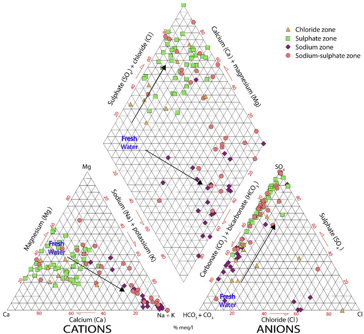
Figure 10. Piper plot illustrating groundwater evolution path showing enrichment in chloride, sulphate, and sodium.
