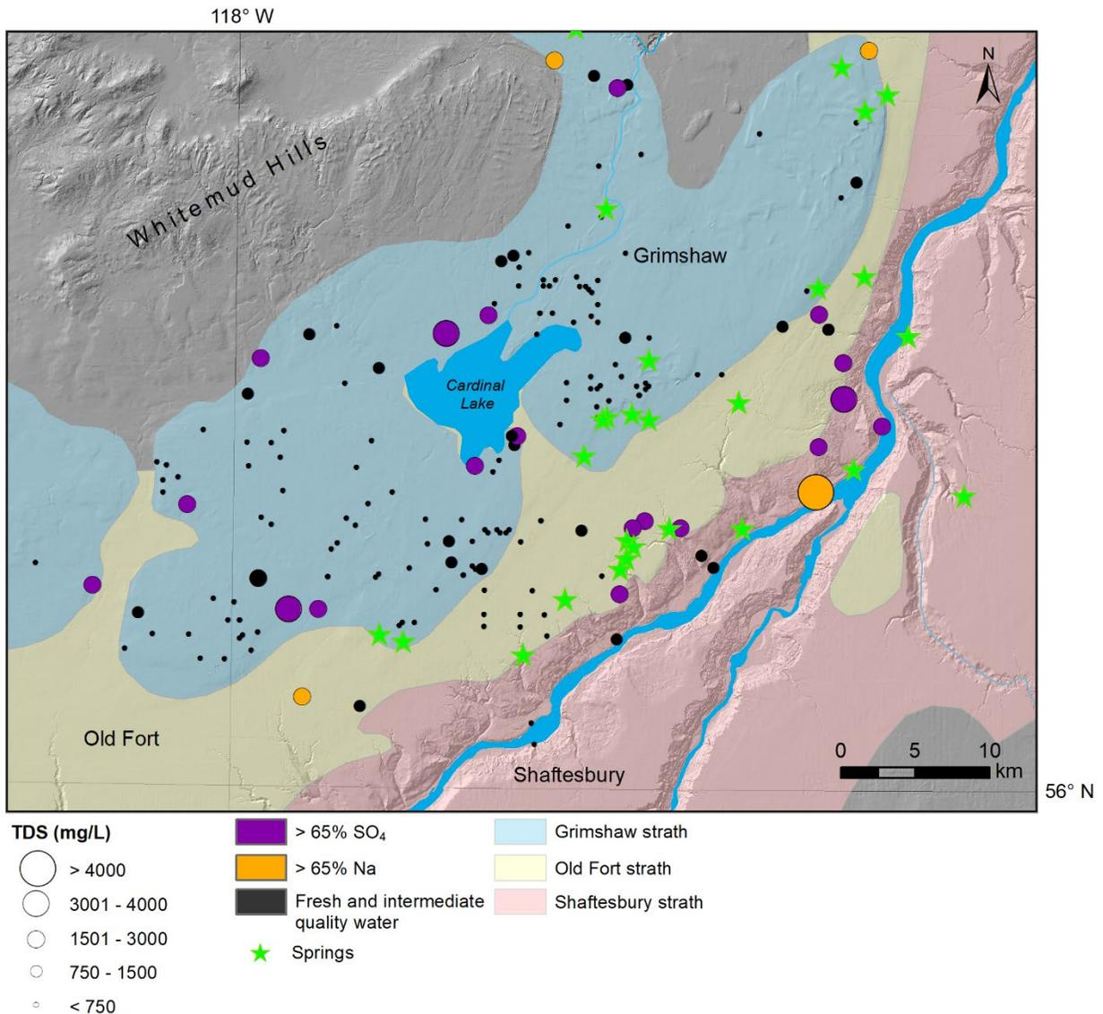
**Figure 7. Groundwater chemistry, including total dissolved solids (TDS), SO<sub>4</sub>, and Na for wells screened in the Grimshaw gravels aquifer, overlain on a hill-shaded DEM of the ground surface. Recharge areas are indicated by black wells with low TDS, and discharge areas are shown by purple and orange with high TDS (modified from Slomka et al., 2018).**
