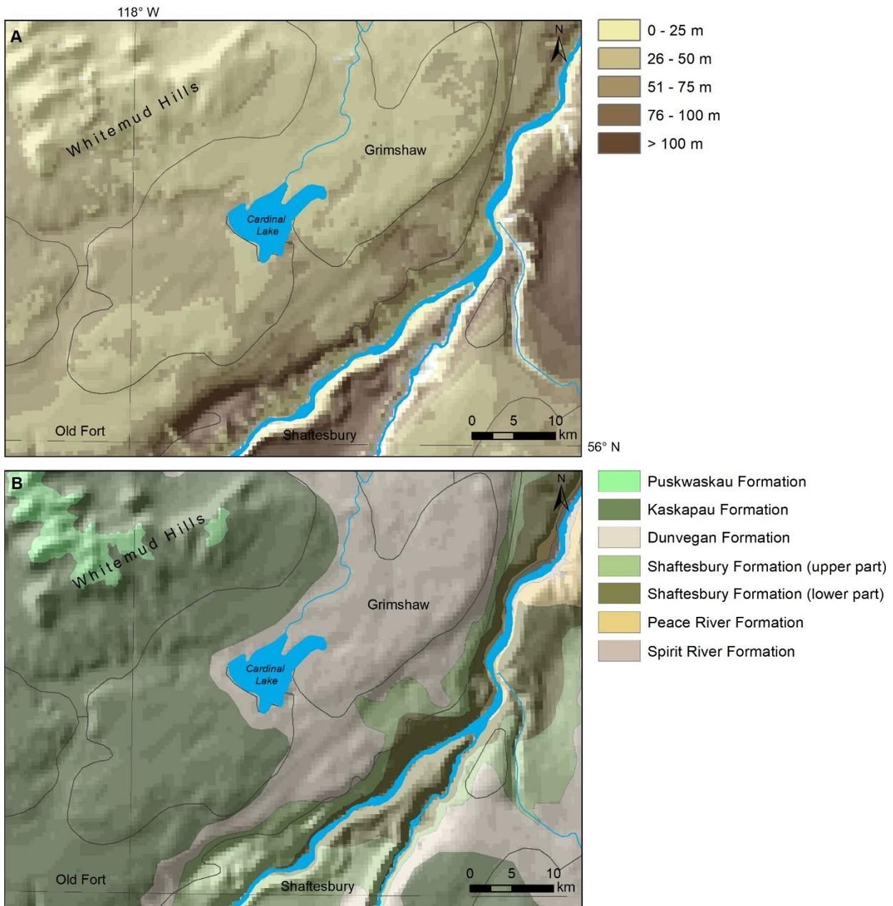
**Figure 2. a) Sediment thickness (AGS, in prep b) (m) and b) bedrock geology (Prior et al., 2013) draped over a hill-shaded DEM of bedrock topography (AGS, in prep a).**
