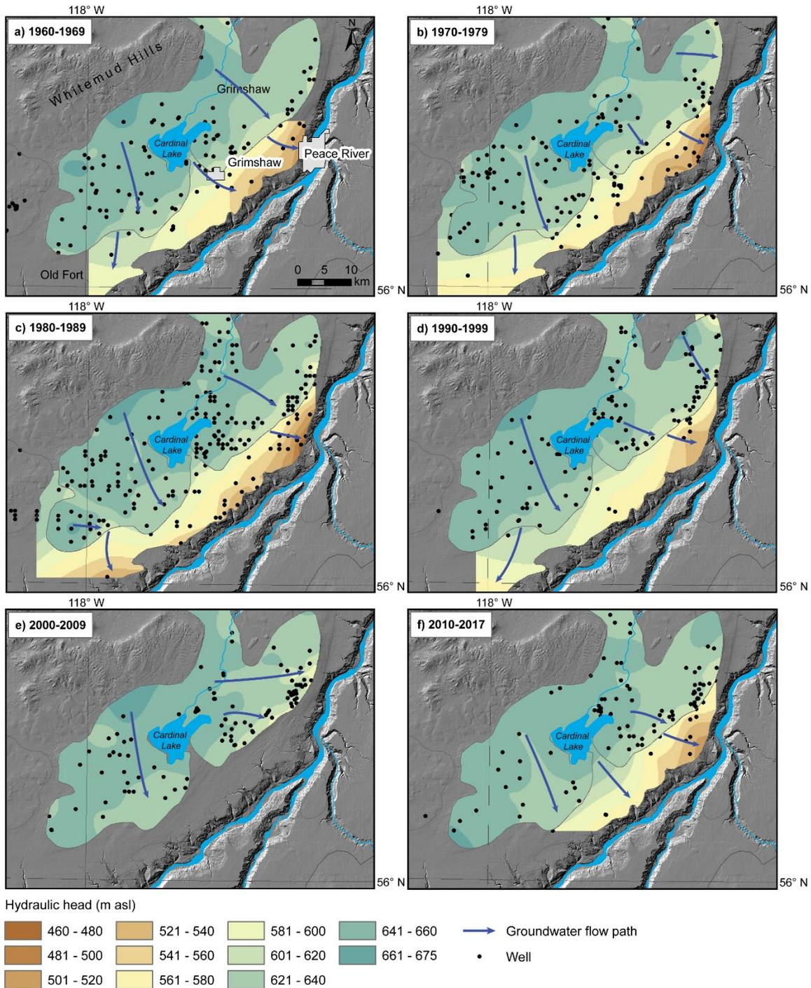
**Figure 4. Maps of the potentiometric surface for Grimshaw and Old Fort gravels organized by decade. Coloured legend indicates ranges of hydraulic head (m asl). Arrows indicate groundwater flow direction. Data limitations prevent mapping of the potentiometric surface within the Old Fort gravel between 2000–2009 (e).**
