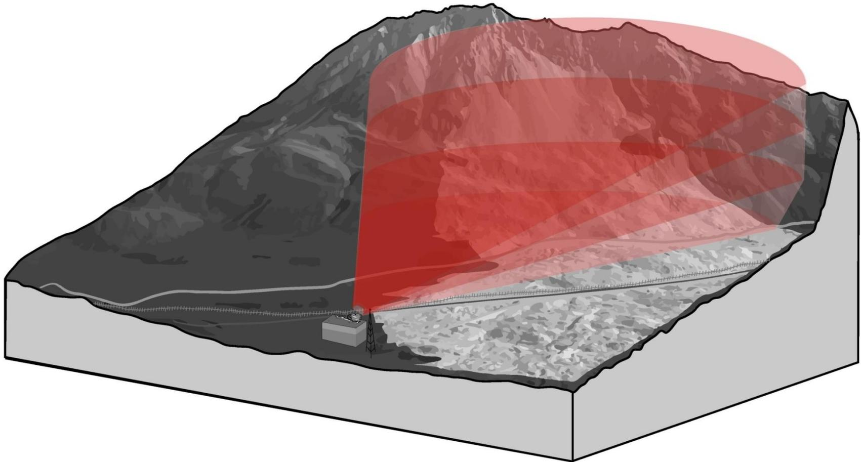
**Figure 2. Overview, as of December 2018, of the primary monitoring equipment. The drawing marks the location of the LiSAMobile system, and the red beam depicts the scanning of the mountain. The light grey area represents the extent of the original 1903 slide. The image is not drawn to scale, and its purpose is to highlight the area LiSAMobile scans.**
