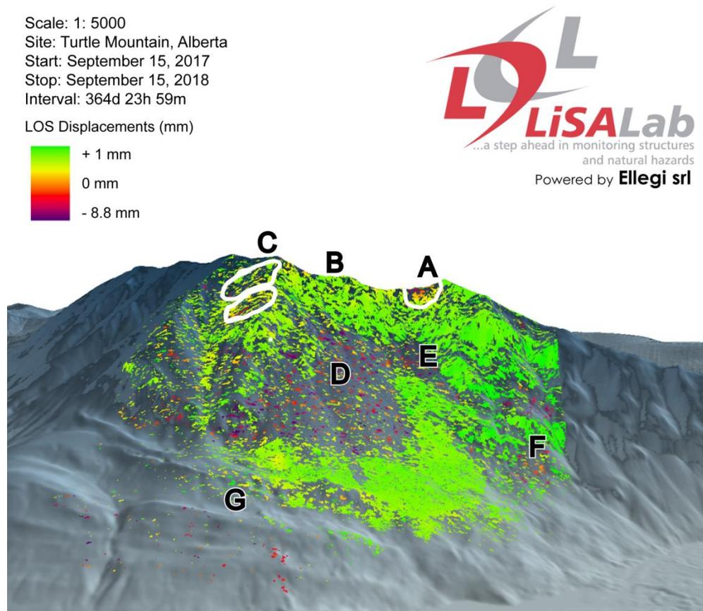
**Figure 7. Annual analysis of large block movements near region A and C, from September 15, 2017, to September 15, 2018 (364d 23h 59m).**
