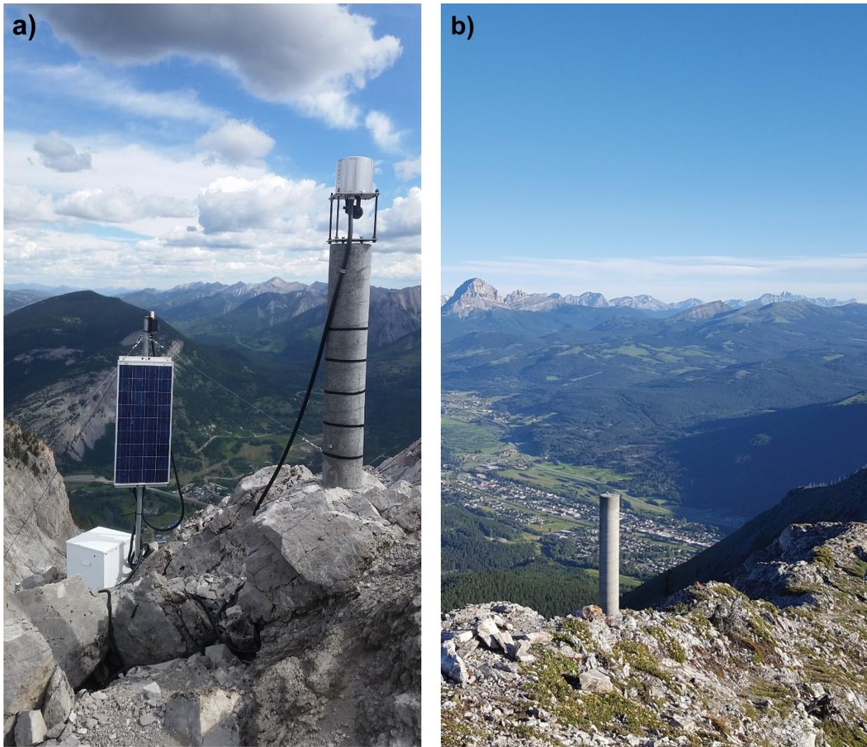
**Figure 7. a) Fully assembled dGPS station in 2016. b) Partially dismantled dGPS station, with only the cement pillar remaining.**
