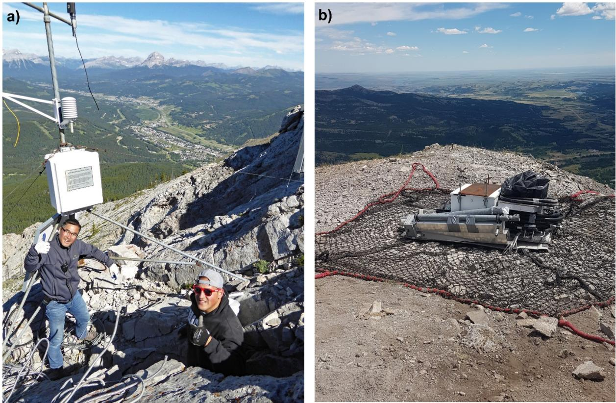
**Figure 3. a) AGS field staff dismantling the weather station electronics and instrumentation. b) Non-operational equipment awaiting removal from Third Peak via helicopter sling.**
