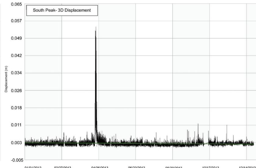
**Figure 7. dGPS station results for Turtle Mountain during 2013. The 3D displacement values are depicted for each corresponding station. The green line indicates the linear trend line.**
