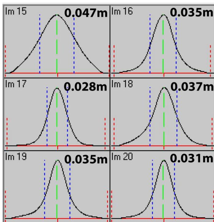
**2013 – control scans piece-wise alignment on 2012 – reference point cloud: histograms and standard deviation.**
