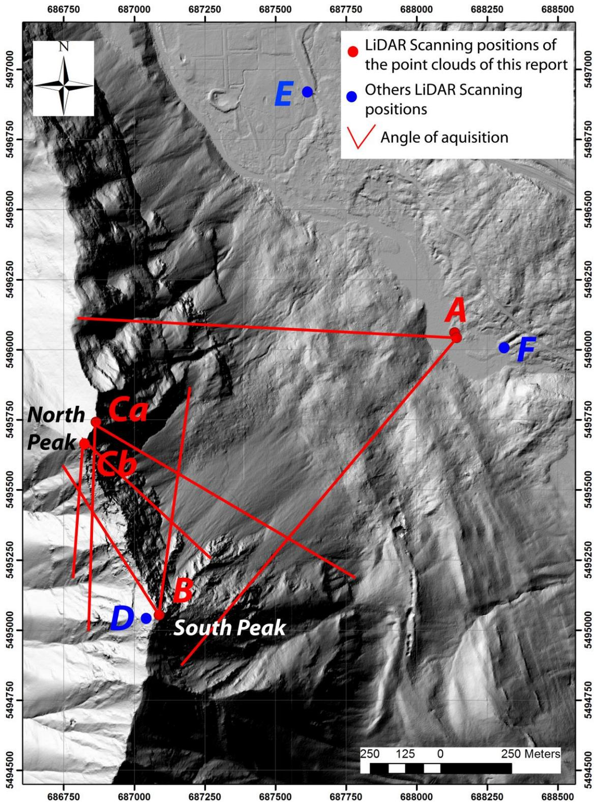
Figure 5: Hillshade map of Turtle Mountain area showing the different GPS position of the LiDAR during acquisitions and indicative acquired area.
