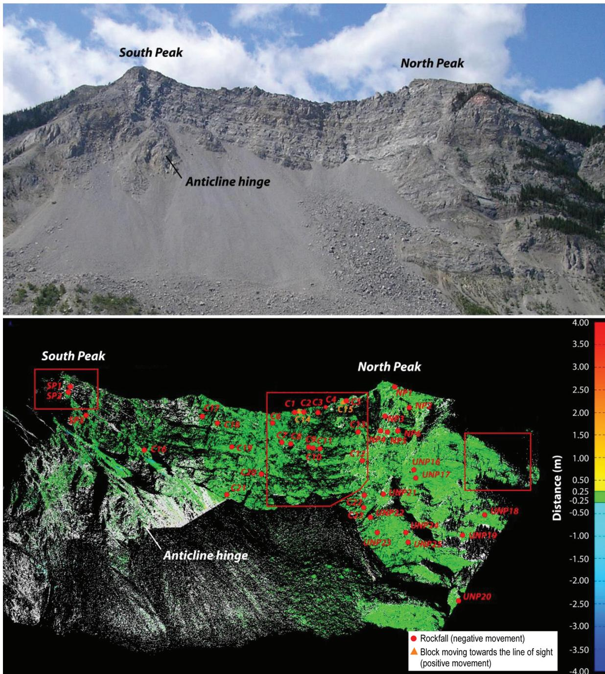
Figure 11. Points, identified as rockfall or block movement, detected during terrestrial LiDAR scanning of the eastern face of Turtle Mountain. The red outlines depict areas of interest further discussed in Appendix 1. Modified from Humair et al. (2013, Figure 9).
