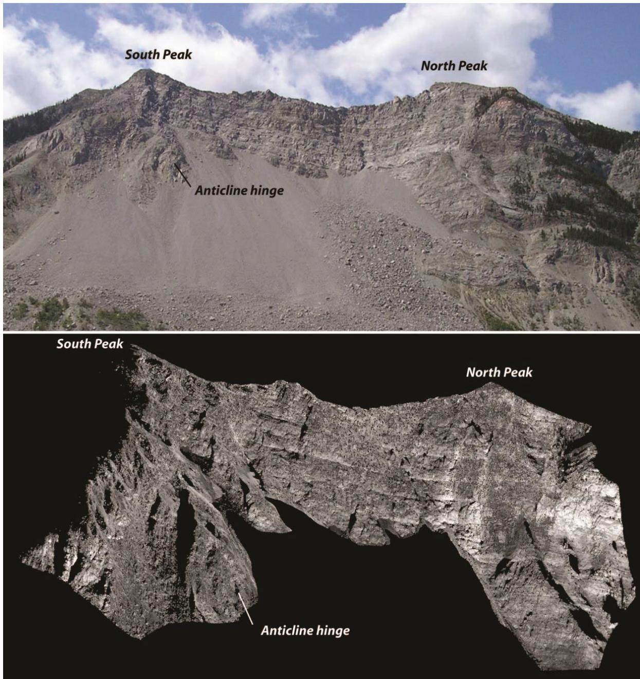
Figure 9. Photo of Turtle Mountain showing the eastern face (top) and corresponding terrestrial LiDAR image (bottom). From Humair et al. (2013, Figure 4).
