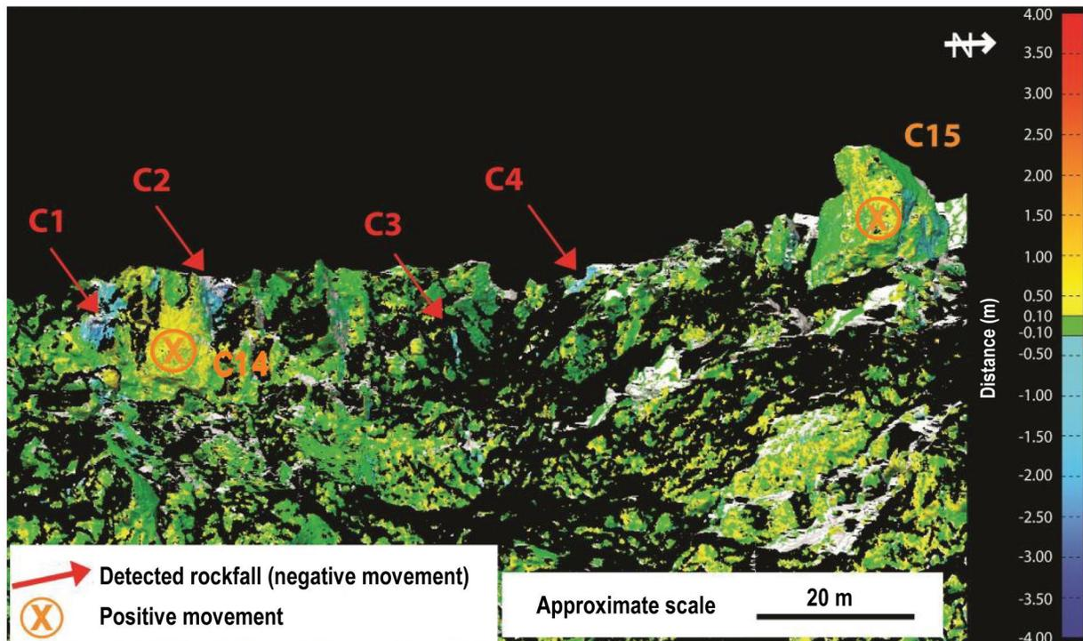
Figure 12. Close-up view of the area of interest of detected rockfalls and positive movements observed on North Peak on Turtle Mountain. Modified from Humair et al.(2013 , Figure 13).
