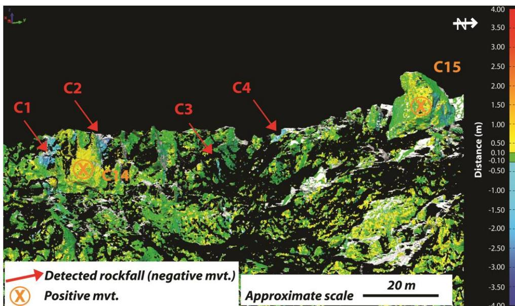
Figure 13: Comparison of the TLS scans focused on the top area of figure 11. The red arrows correspond to the rockfall detected during the 390 days separating both acquisitions (4 rockfalls in this area). The orange crosses correspond to positive movements (block moving forward) detected during the same period (2 blocks in this area).
