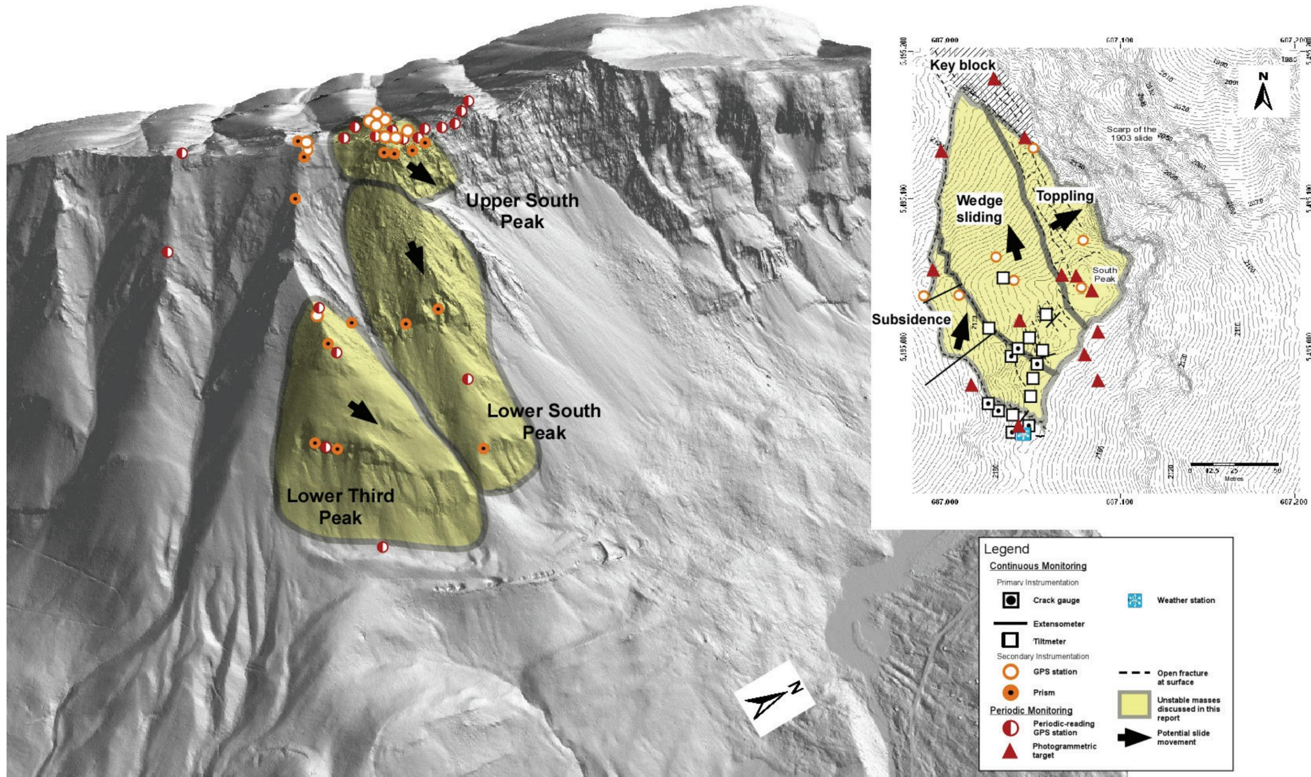
Figure 2. Overview, as of December 2013, of the monitoring network on Turtle Mountain as a whole and South Peak of Turtle Mountain in particular (inset). For readability, primary monitoring instrumentation is shown only on the inset.
