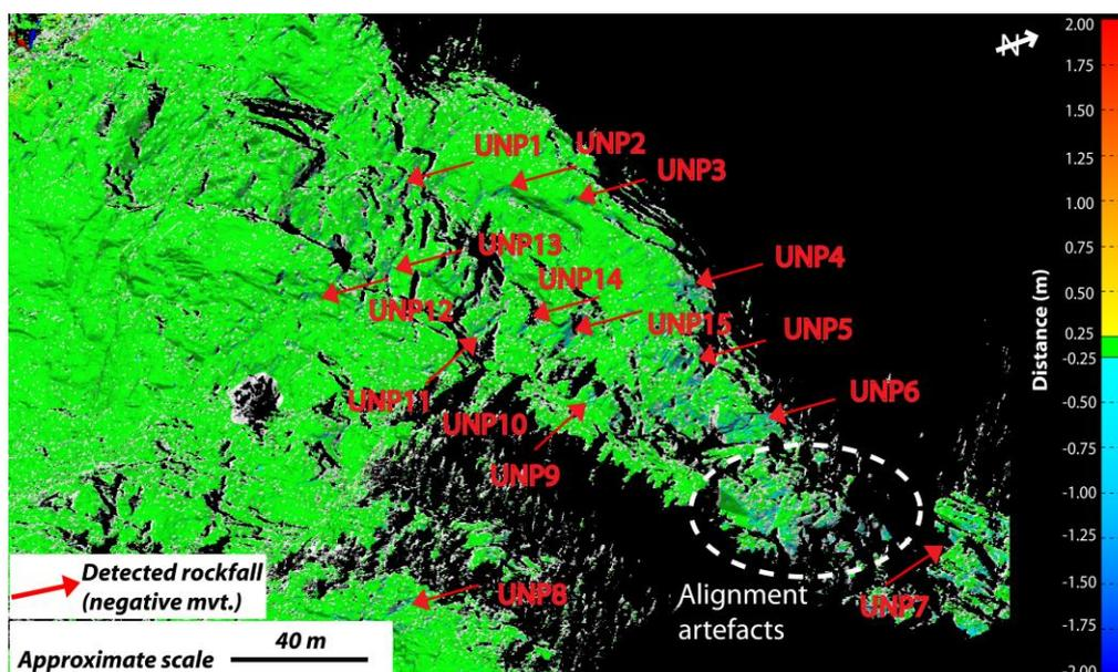
Figure 14: Comparison of the TLS scans focused on the area below North Peak (Figure 9 for location). The red arrows correspond to the rockfall detected during the 390 days separating both acquisitions (15 rockfalls in this area).
