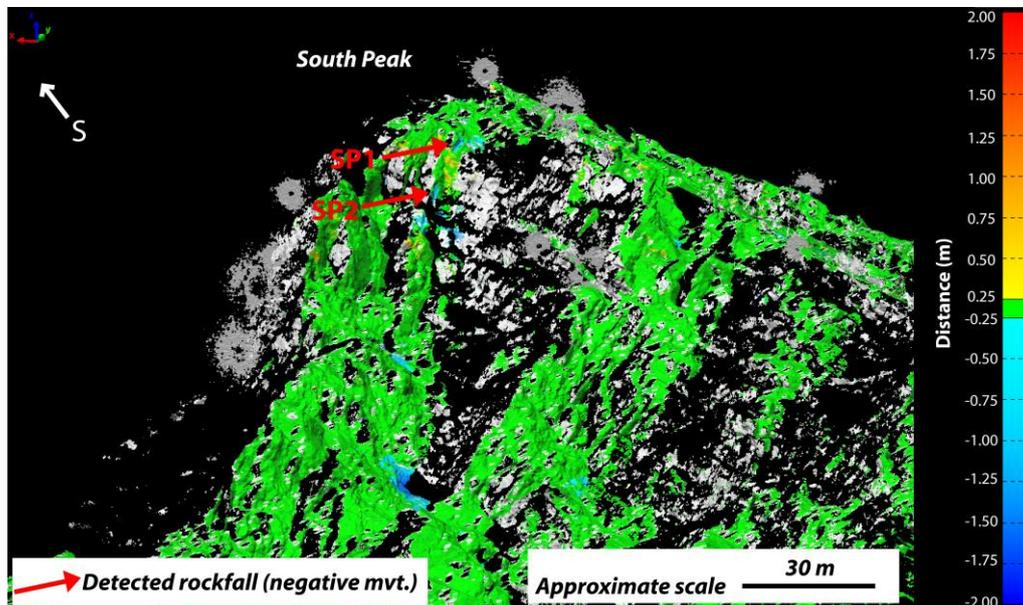
Figure 11: Comparison of the TLS scans focused on South Peak (Figure 9 for location). The red arrows correspond to the rockfall detected during the 390 days separating both acquisitions (2 rockfalls in this area).
