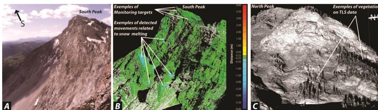
Figure 8: A) and B) Negative movements artefacts due to snow melting between 2012 and 2013 acquisitions. C) Exemple of vegetation (trees) on TLS scan.
