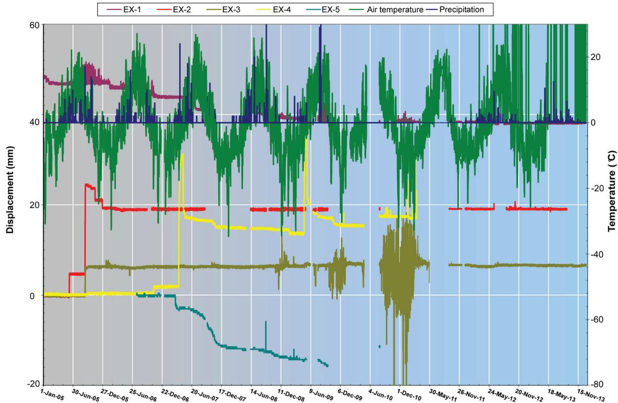
Figure 5. Plot of displacement versus time for extensometers, South Peak, Turtle Mountain.
