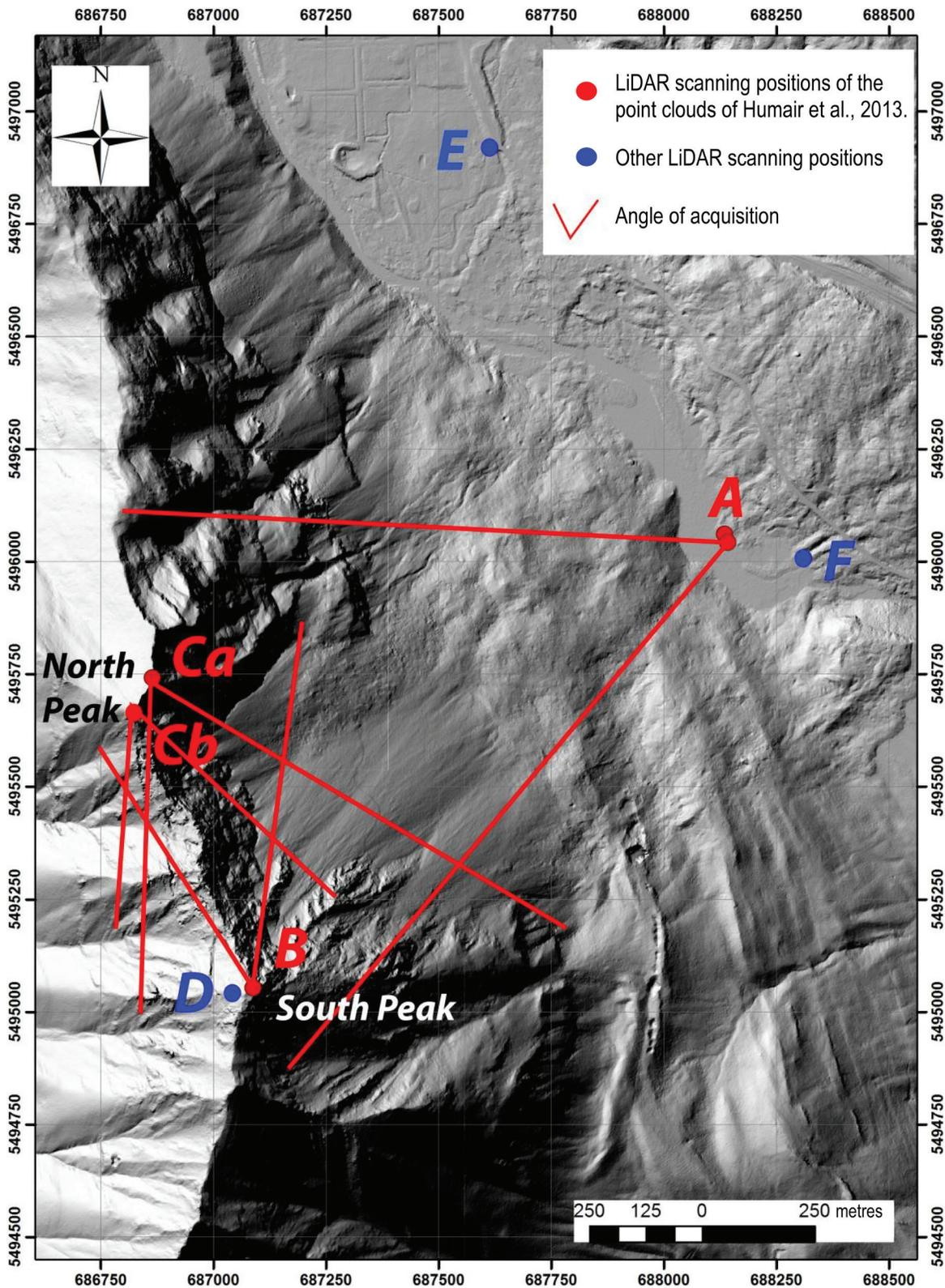
Figure 10. LiDAR map of Turtle Mountain showing locations and acquisition angles of terrestrial LiDAR scanning campaign positions. Modified from Humair et al. (2013, Figure 5).
