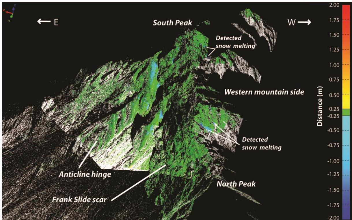
Figure 10: Comparison of the TLS scans focused on the western side of the mountain.
