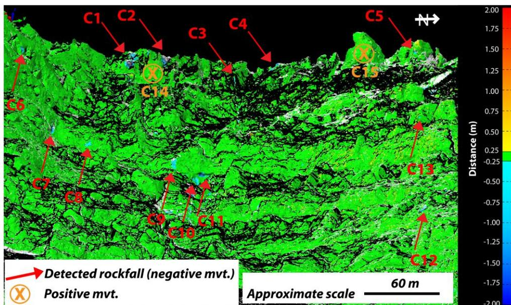
Figure 12: Comparison of the TLS scans focused on the central zone of the Frank Slide scar (Figure 9 for location). The red arrows correspond to the rockfall detected during the 390 days separating both acquisitions (13 rockfalls in this area). The orange crosses correspond to positive movements (block moving forward) detected during the same period (2 blocks in this area).
