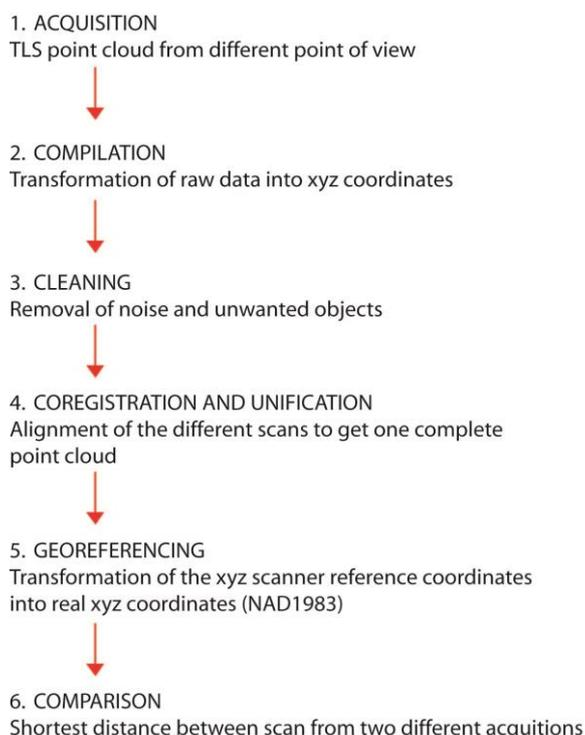
Figure 3: Flowchart of the TLS acquisition and processing methods. Modified after Oppikofer, 2009.
