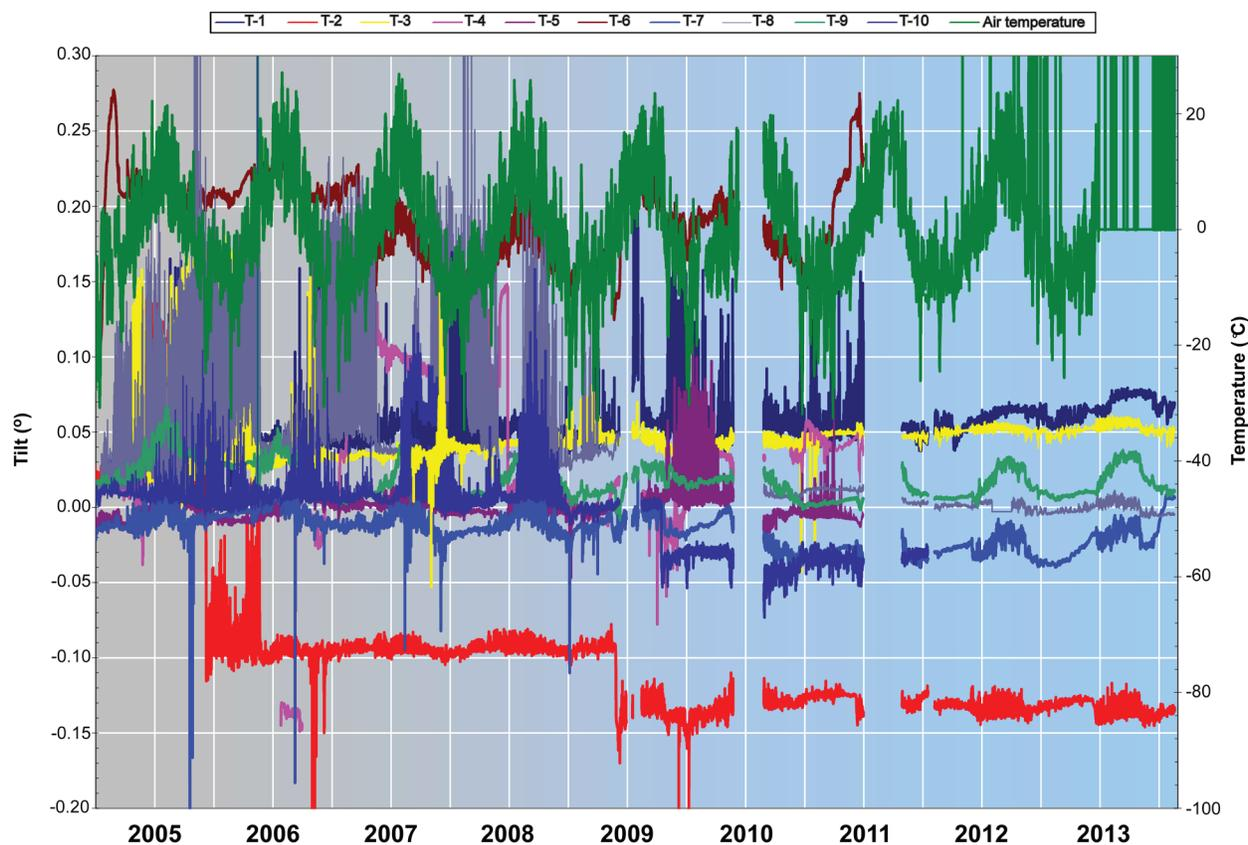
**Figure 4. Plot of tilt versus time for tiltmeters, South Peak, Turtle Mountain.**
