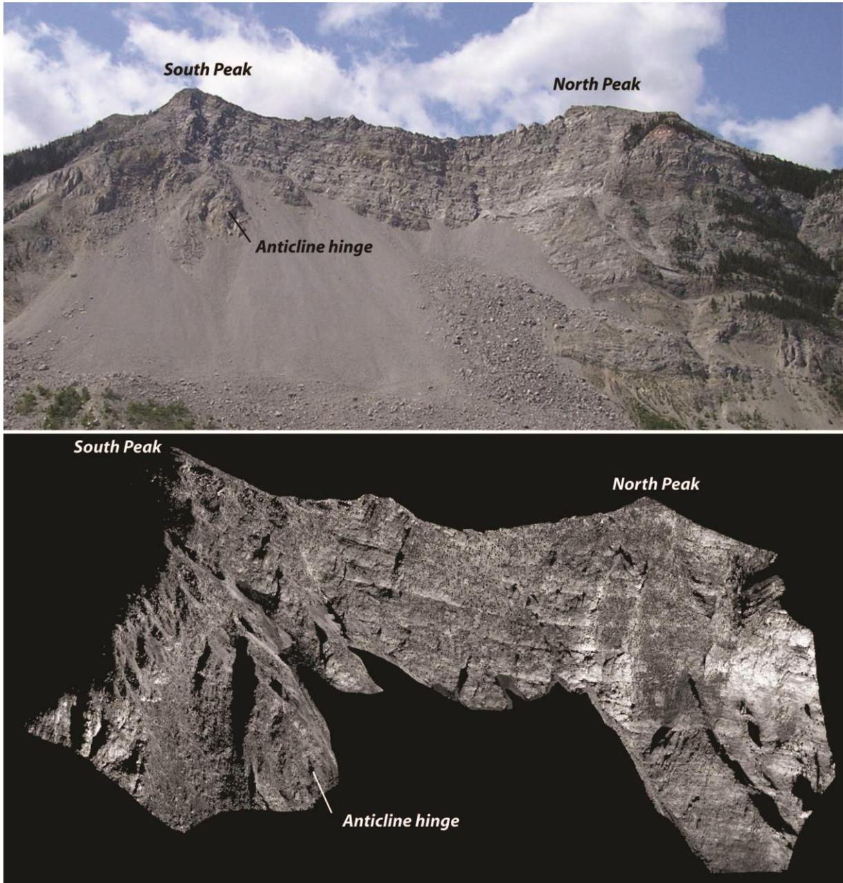
Figure 4: (Above) Picture of the Frank Slide scar, on the eastern face of Turtle Mountain. (Below) Corresponding 2012 point cloud (PolyWorks software).
