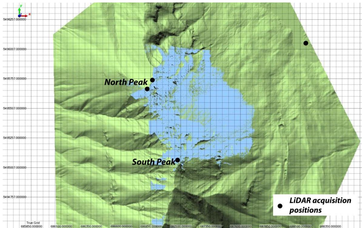
Figure 6: Drapping of the TLS point cloud on the HRDEM showing the area that is covered by the TLS data.
