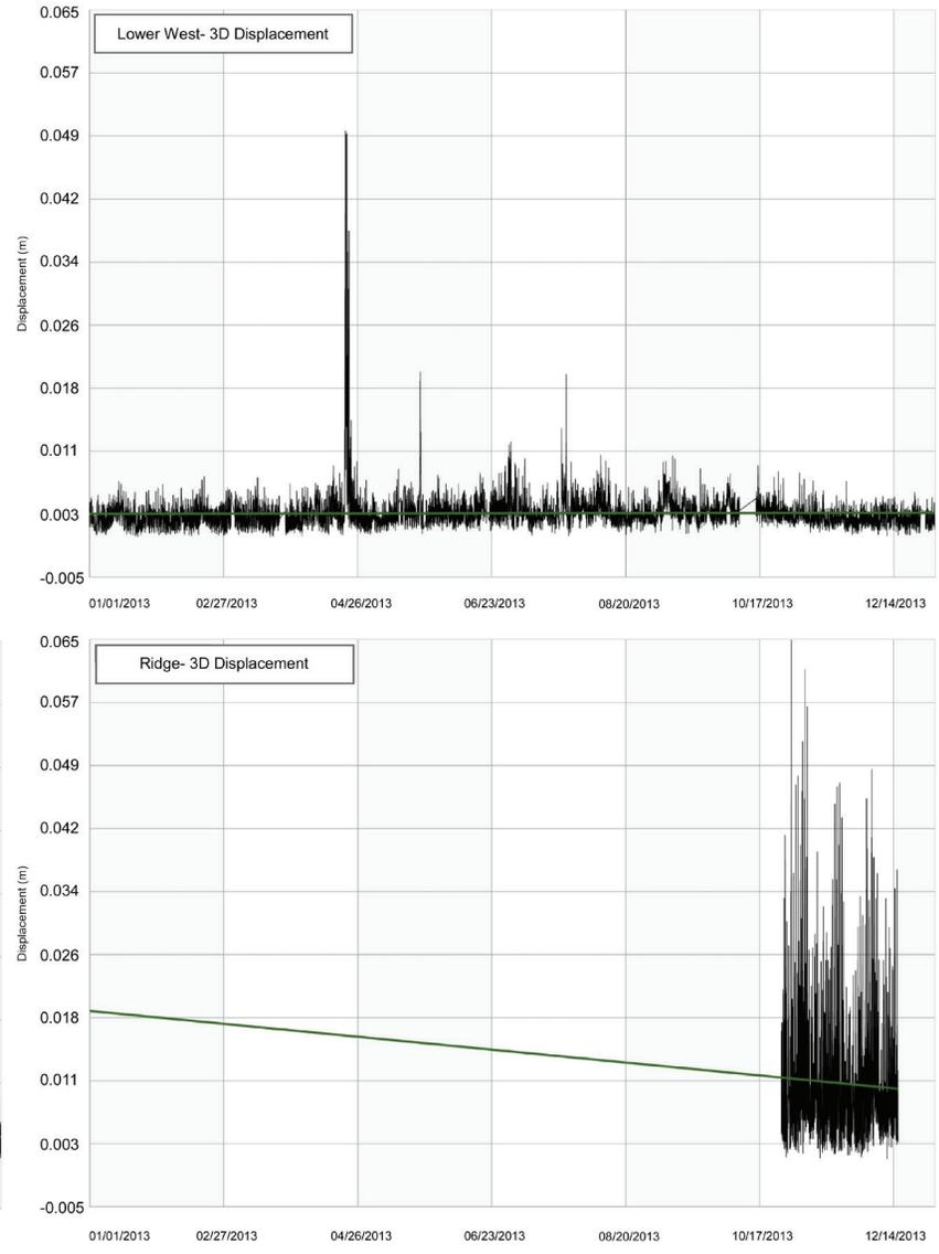
**Figure 6. dGPS station results for Turtle Mountain during 2013. The 3D displacement values are depicted for each corresponding station. The green line indicates the linear trend line.**
