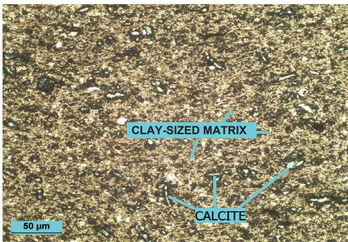
**Plate 5:** plane-polarized light. A high-magnification view of a stained portion of the slide shows ferroan calcite (stained blue) within an unstained clay-sized matrix. Bedding orientation is displayed horizontally in the image.
