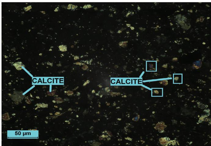
**Plate 6:** cross-polarized light. A high-magnification view shows some calcite as light-coloured grains. Based on the stain, most of the carbonate content is ferroan calcite. Bedding orientation is displayed horizontally in the image.
