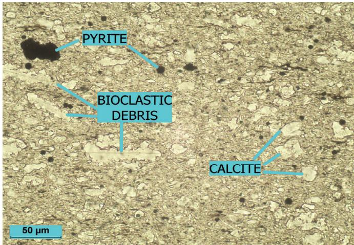
**Plate 4:** plane-polarized light. A high-magnification view of an unstained portion of the slide shows calcite in the form of bioclastic debris and cement. Bedding orientation is displayed horizontally in the image.
