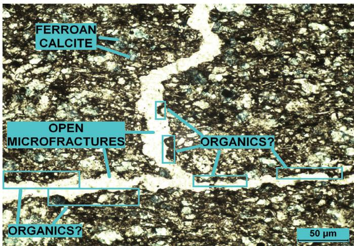
**Plate 6:** plane-polarized light. A high-magnification view shows intersecting open microfractures. As discussed in the description of Plate 5, there appears to be a relationship between the presence of organics and the open microfractures. This image was taken over a stained portion of the slide; ferroan calcite is stained blue. Bedding orientation is displayed horizontally in the image.
