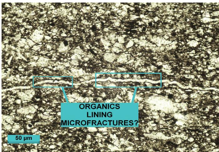
**Plate 5:** plane-polarized light. A high-magnification view shows a very fine, open microfracture that appears to be lined with organic material. The organic matter would have presented a plane of weakness for fracturing during thin-section creation. Bedding orientation is displayed horizontally in the image.
