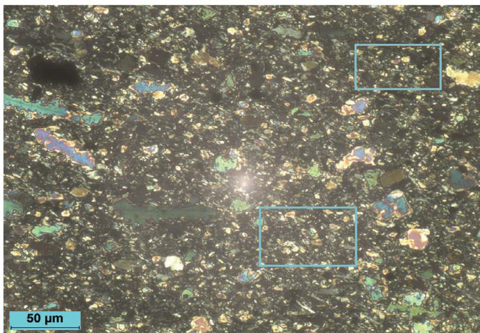
**Plate 6:** cross-polarized light. A high-magnification view shows that many minerals in the matrix have a high birefringence. It appears that this is the ferroan calcite component: the bulk of the clay-sized fraction remains unidentifiable. Bedding orientation is displayed horizontally in the image.
