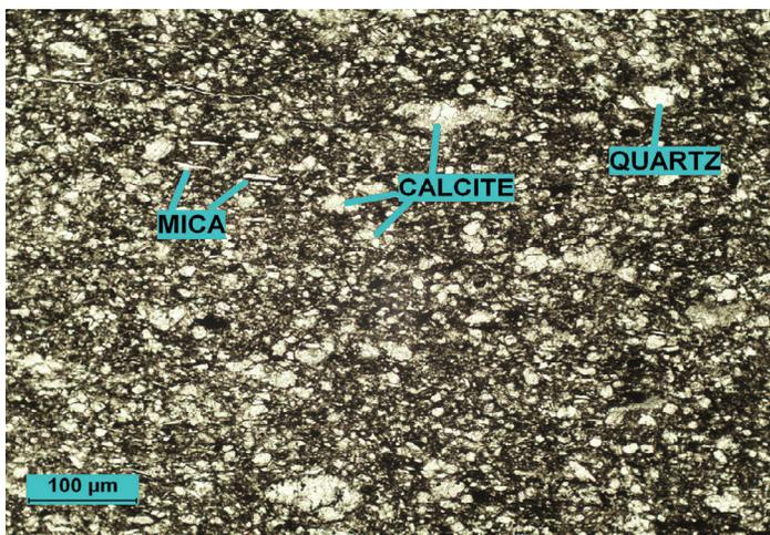
**Plate 2:** plane-polarized light. A medium- to high-magnification view of claystone shows light-coloured calcite and quartz grains. Staining indicates that most of the carbonate minerals are ferroan calcite. Quartz is present as silt- and clay-sized grains. Bedding orientation is displayed horizontally in the image.
