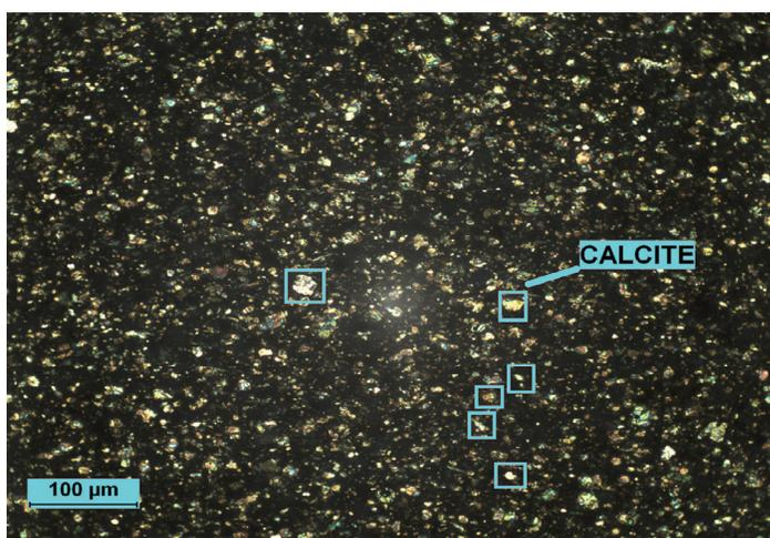
**Plate 5:** cross-polarized light. The same view as Plate 4 under cross-polarized light shows most of the carbonate content as light-coloured grains. Staining indicates that most of the carbonate content is ferroan calcite. Bedding orientation is displayed horizontally in the image.
