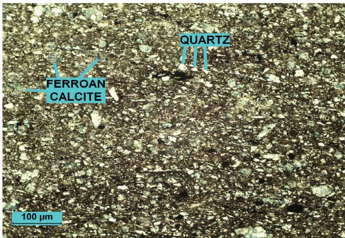
**Plate 3:** plane-polarized light. A medium- to high-magnification view of a stained portion of the slide shows common presence of ferroan calcite, much of which is in the clay-sized fraction. Most of the light-coloured grains are calcite (stained blue), with only minor amounts of quartz grains. Bedding orientation is displayed horizontally in the image.
