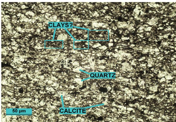
**Plate 3:** plane-polarized light. A high-magnification view shows slightly silty calcareous claystone. The dark brown matrix may be clays intermixed with organic material. Bedding orientation is displayed horizontally in the image.
