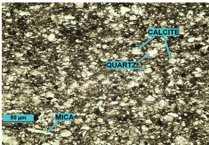
**Plate 6:** plane-polarized light. A high-magnification view of an unstained portion of the slide shows slightly silty claystone. Silt-sized quartz is present, but most of the quartz grains in the sample are clay-sized. Bedding orientation is displayed horizontally in the image.
