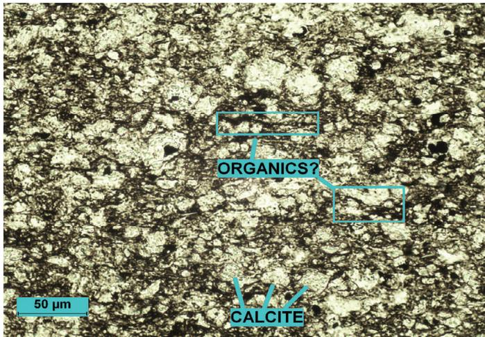
**Plate 4:** plane-polarized light. A high-magnification view shows what appears to be organic material present in the form of wispy plates, although they are too fine to positively identify with a standard petrographic microscope. Bedding orientation is displayed horizontally in the image.
