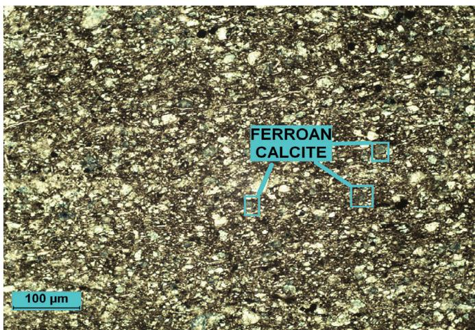
**Plate 2:** plane-polarized light. A medium- to high-magnification view of the stained portion of the slide shows calcareous silty claystone. Staining indicates that most of the carbonate minerals are ferroan calcite. There does appear to be a minor dolomite content as well. Many of the calcite grains are clay-sized. Bedding orientation is displayed horizontally in the image.
