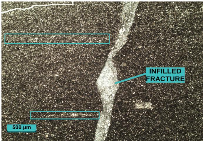
**Plate 1:** plane-polarized light. A low- to medium-magnification overview shows a massive calcareous silty claystone and a calcite-infilled fracture. Areas within the annotated rectangles are alignments of grains that may indicate the horizontal plane, which would suggest that the fracture is almost vertical. The thin section is slightly too thick in this image. Bedding orientation is displayed horizontally in the image.
