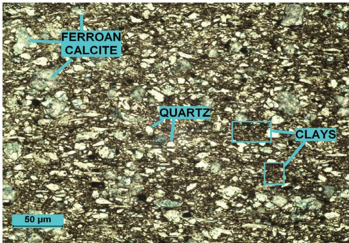
**Plate 4:** plane-polarized light. A high-magnification view of a stained portion of the slide shows ferroan calcite (stained blue) and minor amounts of quartz, within a predominantly clay-sized matrix. There appears to be minor amounts of organic material within the clay-sized matrix. Bedding orientation is displayed horizontally in the image.
