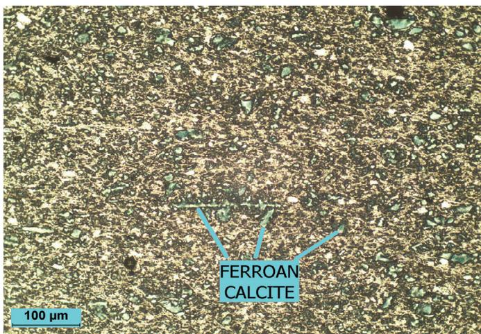
**Plate 3:** plane-polarized light. A medium- to high-magnification view of a stained portion of the slide shows ferroan calcite within a clay-sized matrix. Both detrital and authigenic calcite grains are present. Bedding orientation is displayed horizontally in the image.
