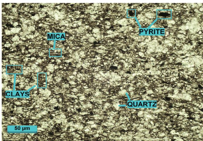
**Plate 5:** plane-polarized light. A high-magnification view shows slightly silty claystone. The dark brown matrix is predominantly clay minerals with trace amounts of organic material intermixed. Bedding orientation is displayed horizontally in the image.
