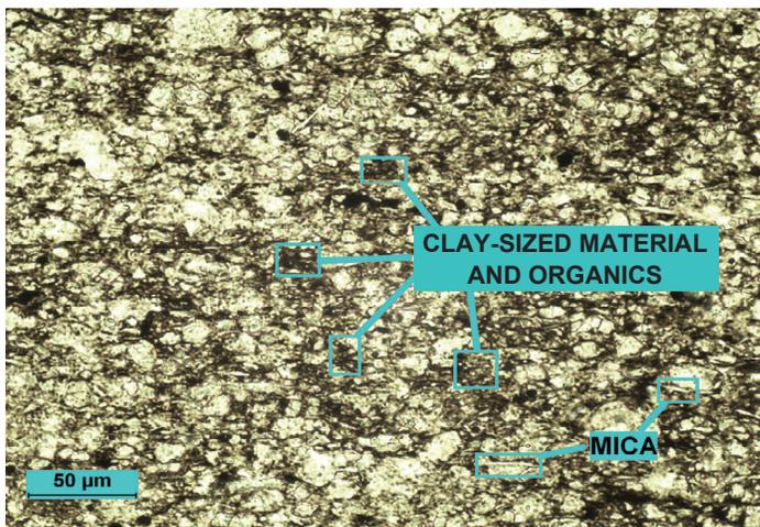
**Plate 3:** plane-polarized light. A high-magnification view shows claystone with trace amounts of mica. Almost all of the light-coloured grains are calcite but, there are clay-sized quartz grains present as well. It appears that there are minor amounts of amorphous organics intermixed with the clay-sized material. Bedding orientation is displayed horizontally in the image.
