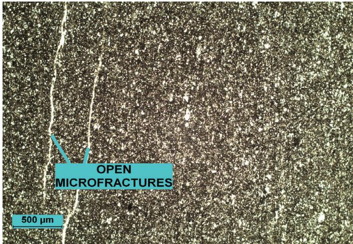
**Plate 1:** plane-polarized light. A low- to medium-magnification view shows calcareous claystone with minor amounts of open microfractures. There are faint indications of bedding, and most of the microfractures are parallel to bedding. Bedding orientation is displayed vertically in the image.
