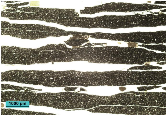
**Plate 1:** plane-polarized light. A low-magnification overview shows the fragmented condition of the slide. The large fractures are a result of thin-section creation. Bedding orientation is displayed horizontally in the image.
