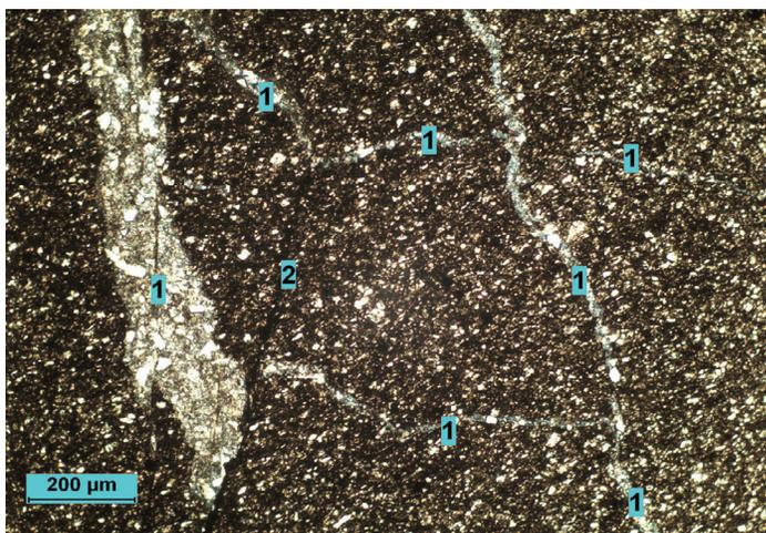
**Plate 2:** plane-polarized light. A medium-magnification view shows a network of infilled fractures, the most prominent (on the left) is present through the length of the slide. Infilled fractures annotated as "1" are infilled with what appears to be ferroan calcite, with trace amounts of quartz crystals within the calcite. The area annotated as "2" is a microfault. The thin section is slightly too thick in this image. Bedding orientation is displayed horizontally in the image.
