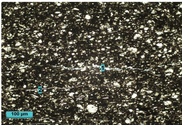
**Plate 3:** plane-polarized light. A medium- to high-magnification view shows a very fine microfracture assumed to be horizontally oriented and filled with ferroan calcite cement (annotated as "1"). Another parallel fracture is open (annotated as "2"). The slide is over-thick where this image was taken. Bedding orientation is displayed horizontally in the image.
