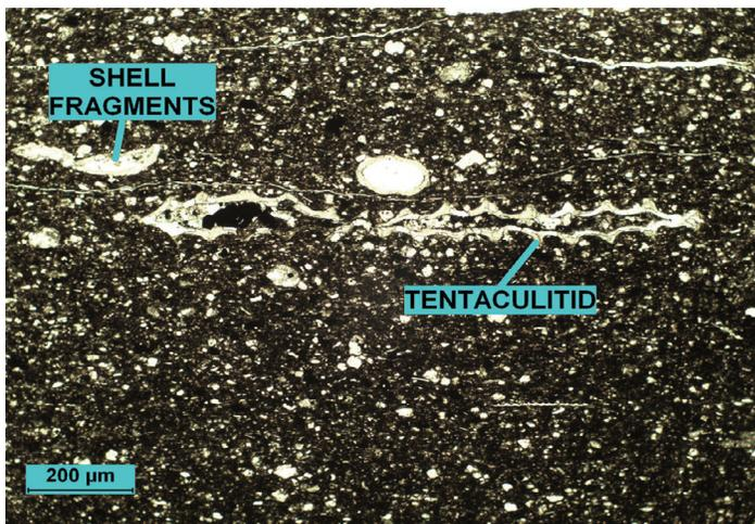
**Plate 2:** plane-polarized light. A medium-magnification view shows claystone with bioclasts, including tentaculitids. Bedding orientation is displayed horizontally in the image.
