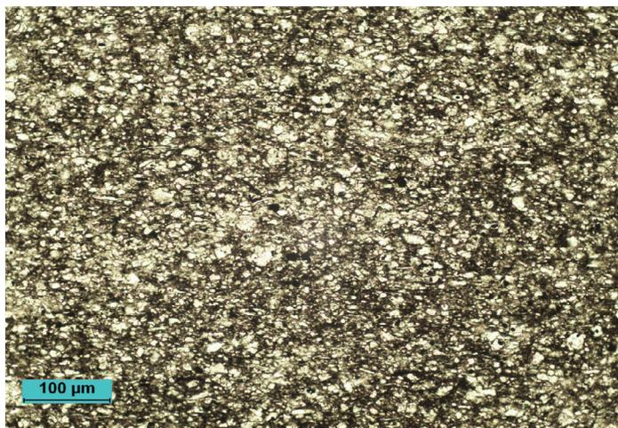
**Plate 4:** plane-polarized light. A medium- to high-magnification view shows calcareous claystone. This is an unstained portion of the slide.
