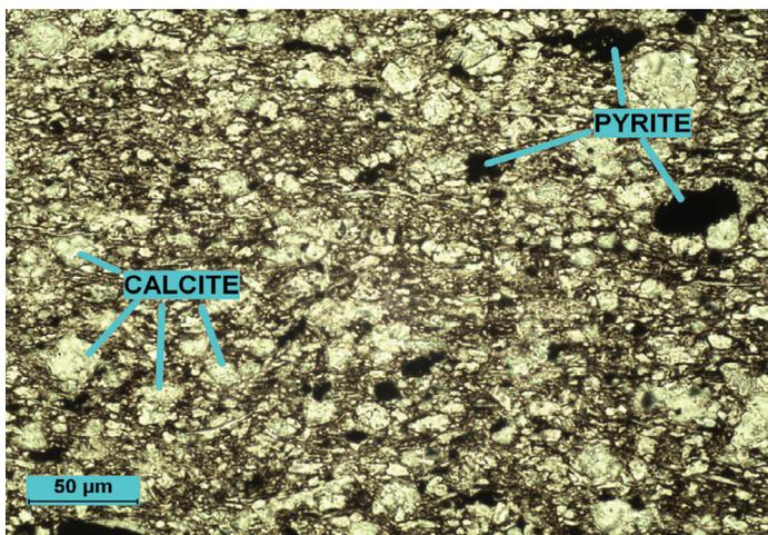
**Plate 5:** plane-polarized light. A high-magnification view shows claystone with calcite cement. Bedding orientation is displayed horizontally in the image.
