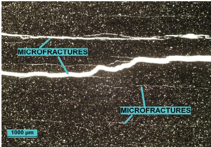
**Plate 1:** plane-polarized light. A low-magnification overview shows predominantly massive claystone with open microfractures. The majority of them are parallel to bedding (horizontal). Fractures are from thin-section creation. Bedding orientation is displayed horizontally in the image.
