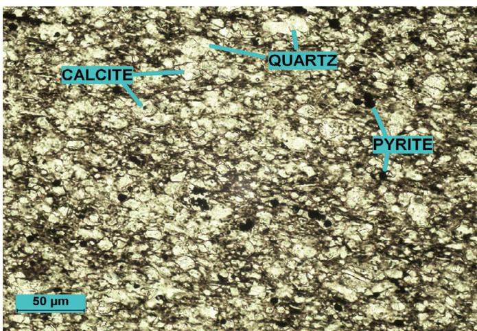
**Plate 6,** plane-polarized light. A high-magnification view shows an unstained portion of the slide. Most of the light-coloured grains in the image are calcite. There are also trace amounts of silt-sized quartz and minor amounts of clay-sized quartz. Bedding orientation is displayed horizontally in the image.
