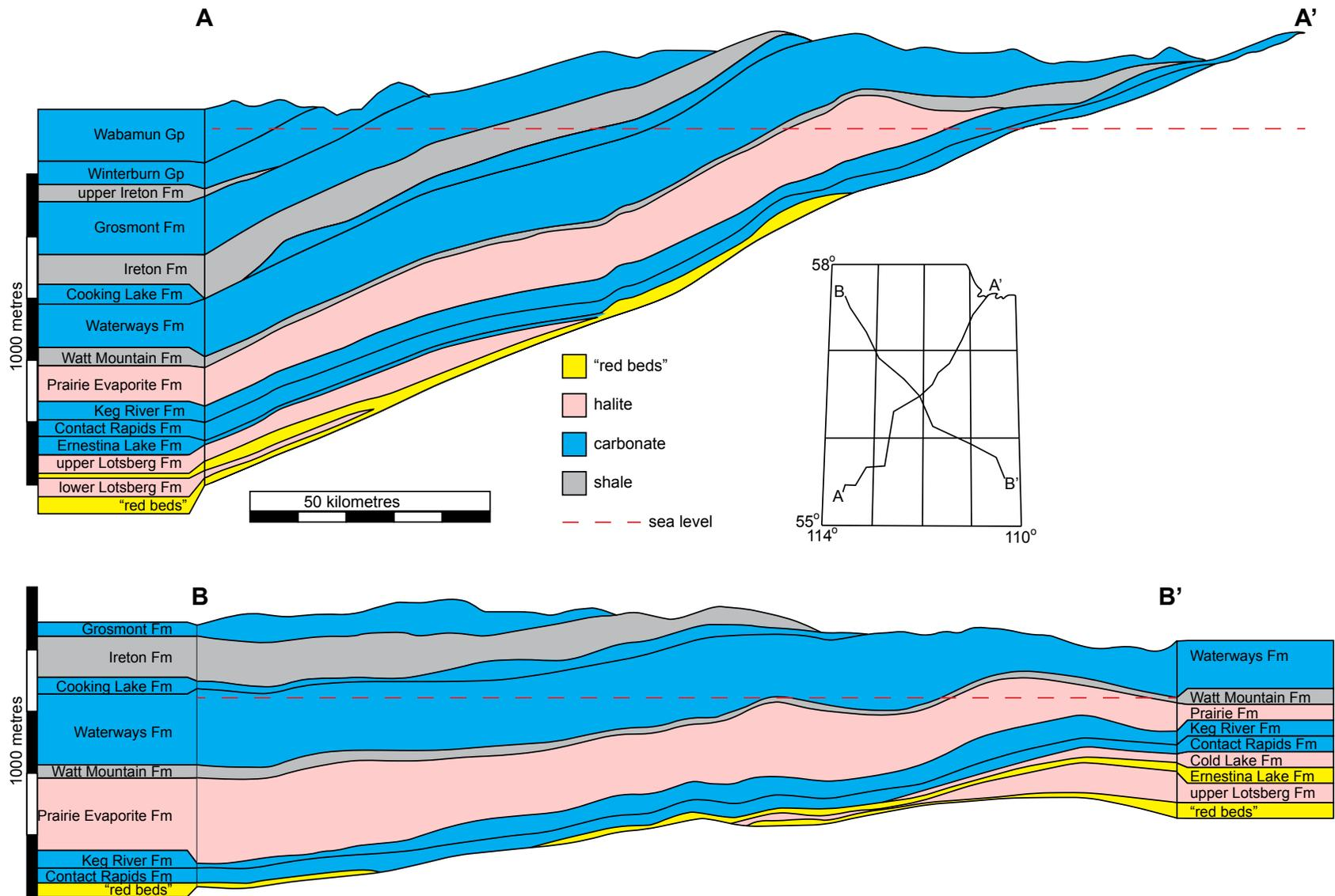
Figure 2. Structural cross-sections through Devonian stratigraphy in northeastern Alberta modified from Bachu et al. (1993). Only the Devonian portions of their cross-sections are presented and nomenclature has been updated.
