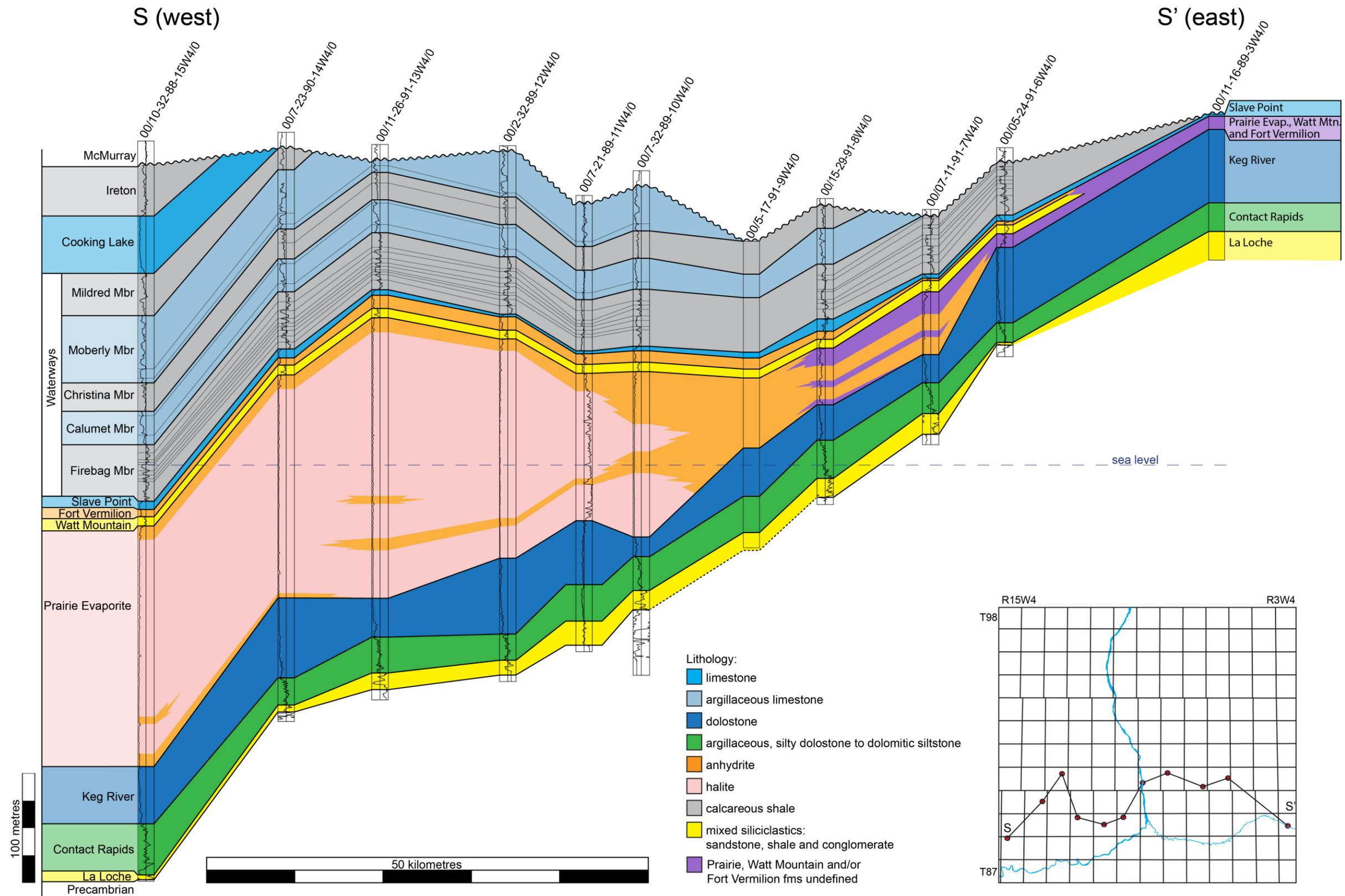
Figure 6. Cross-section of Devonian stratigraphy through the southern portion of the study area.
