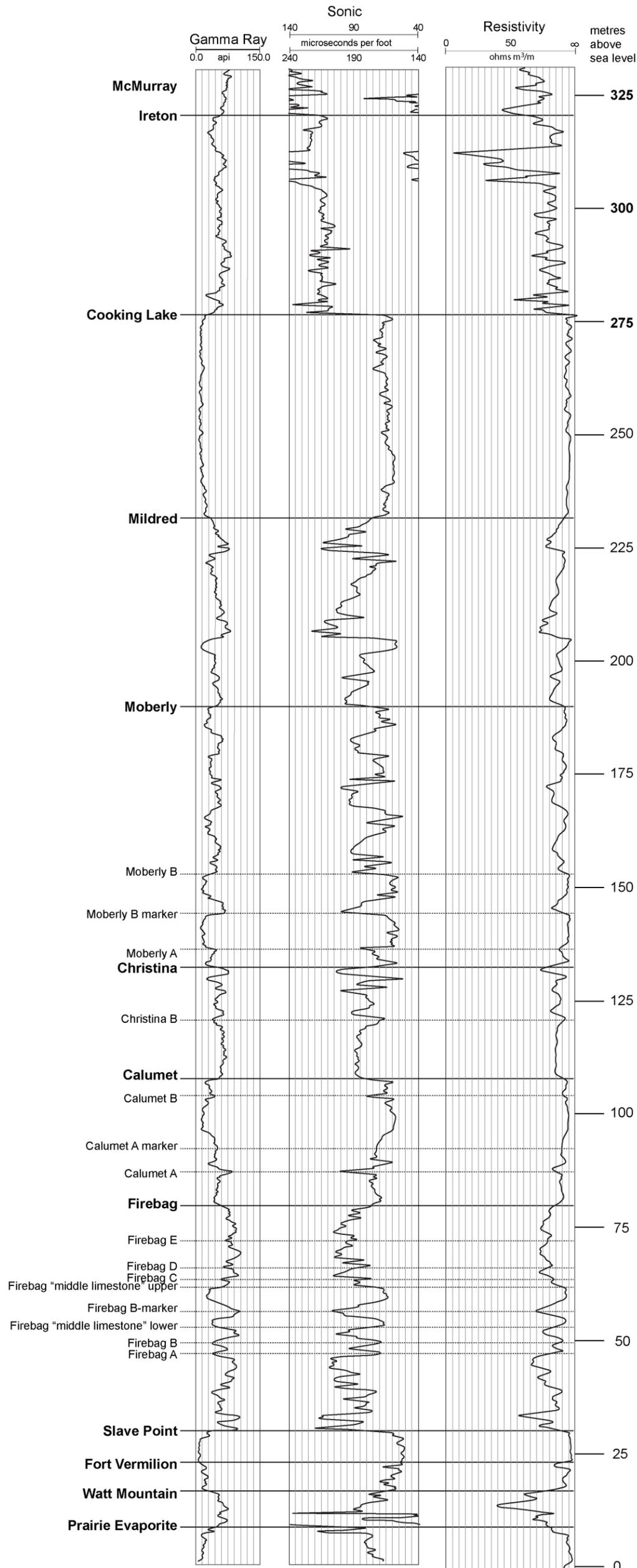
Figure 5. Sample well log of Beaverhill Lake Group and younger strata from the southeasternmost well log in the present study. Formation and member tops are in bold and use solid lines. Marker beds are in smaller, non-bold font and use dotted lines.
