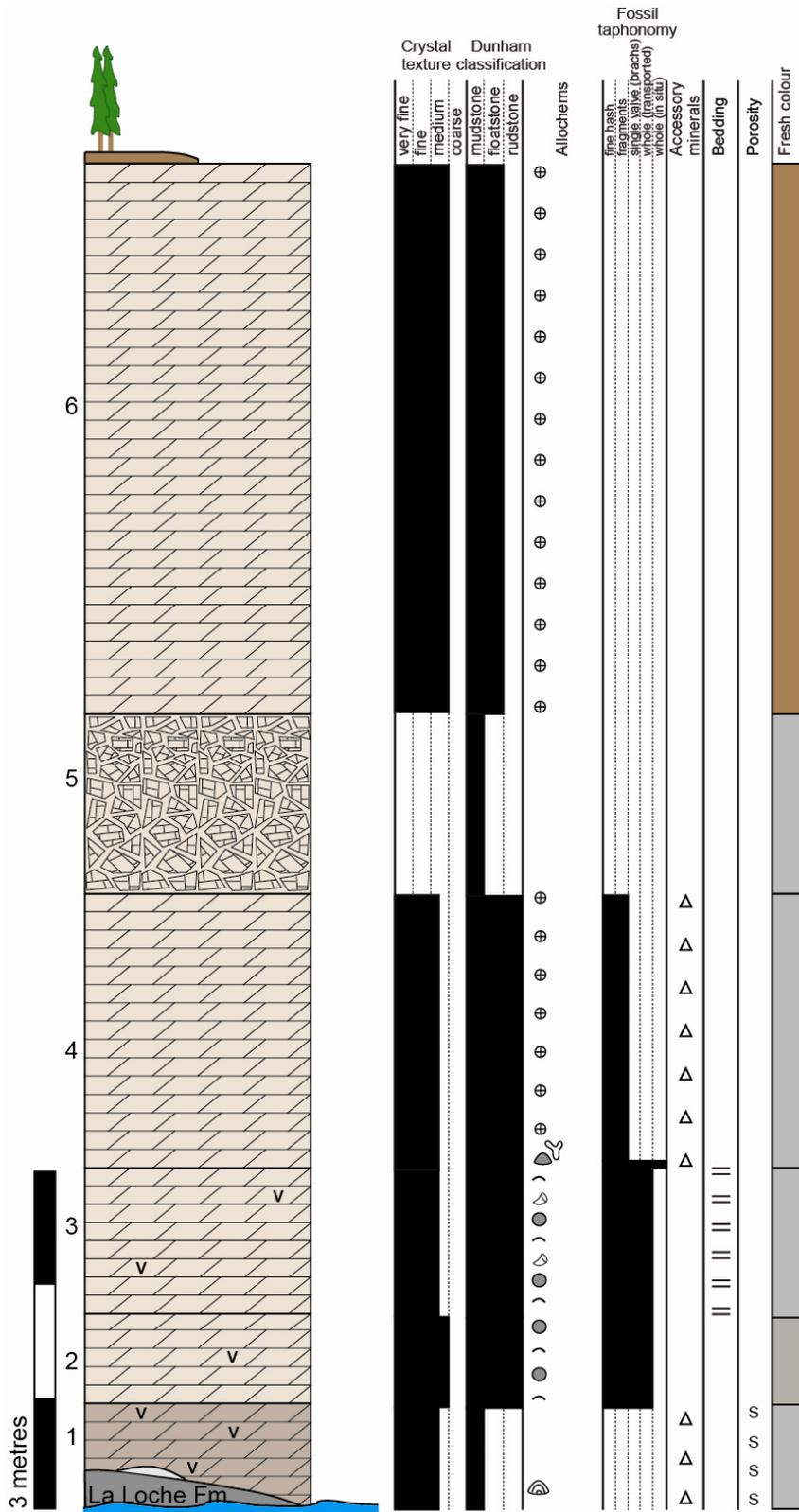
Figure 16. Stratigraphic column of the Keg River Formation at Whitemud Falls. Numbers on the left of the column correspond to Keg River descriptions, not to La Loche–Keg River contact descriptions
