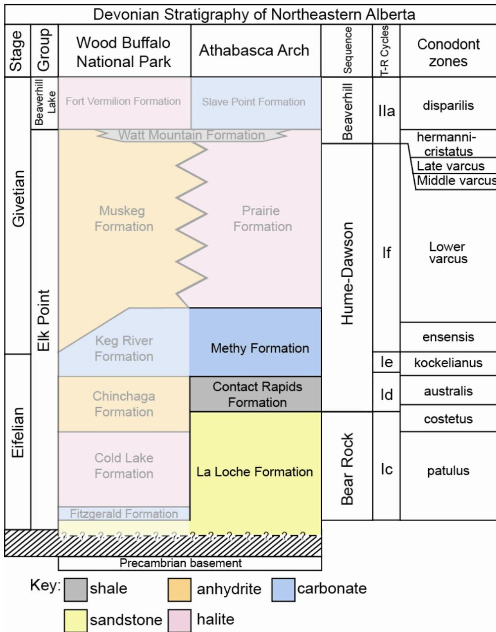
Figure 2. Stratigraphic chart for the Elk Point Group of northeastern Alberta. Units described in this report are highlighted. Sequences are from Moore (1988, 1993). Conodont zones and T-R cycles are from Johnson et al. (1985).
