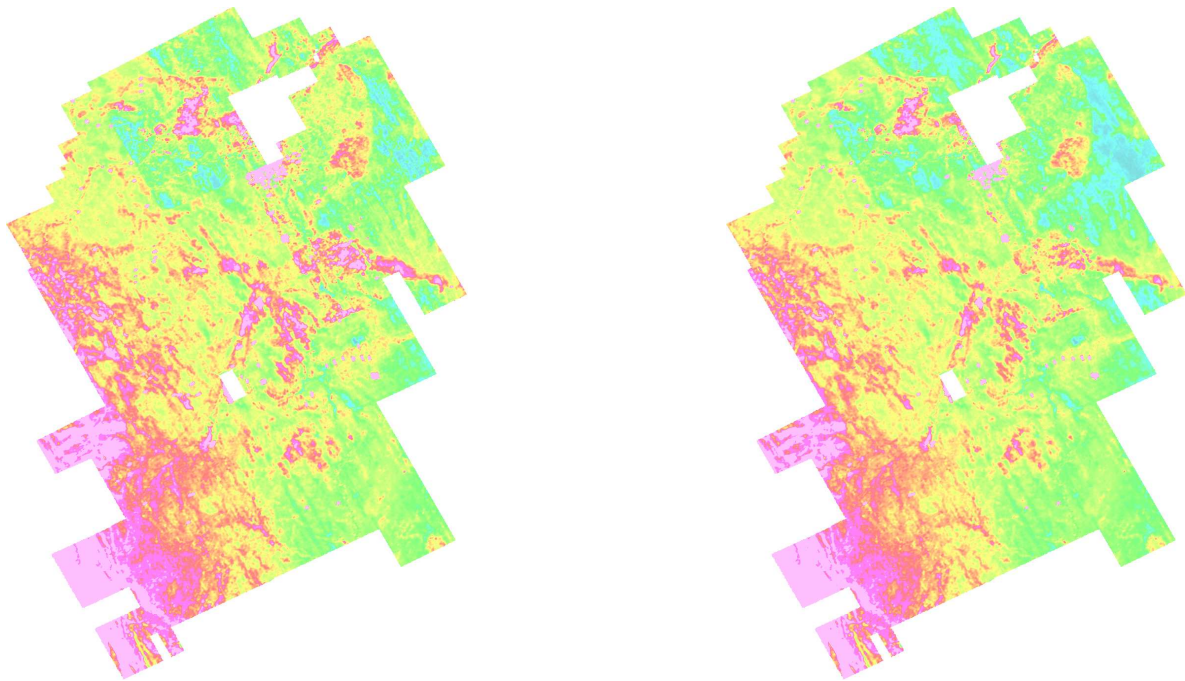
Figure 2. Resistivity Depth Slices at 0 metres (left) and 10 metres (right)
