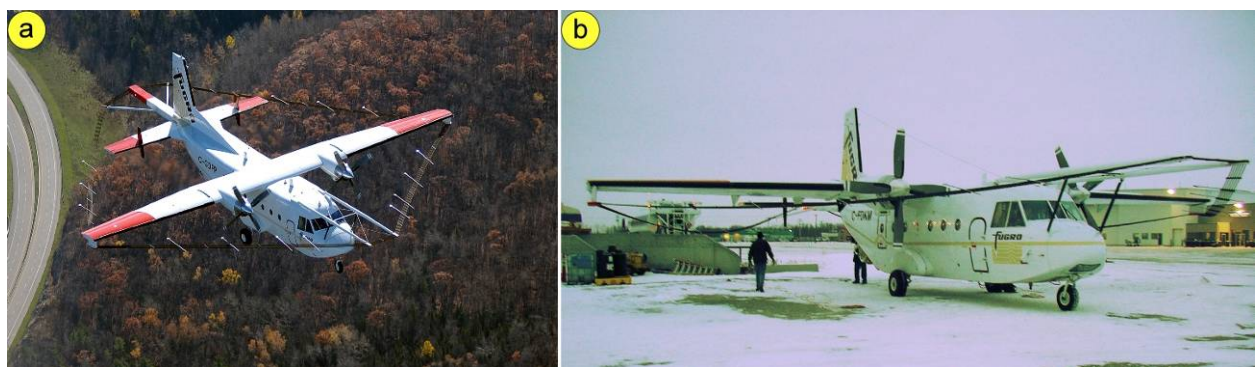
Figure 4. a) The TEMPEST ® survey technique in flight. Note the transmitting loop fixed to the aircraft's nose, tail and wing tips. Primary electromagnetic pulses are created by a series of discontinuous sinusoidal current pulses and transmitted into the transmitting loop. b) Modified Casa 212 aircraft used by Fugro Airborne Surveys in this study.
