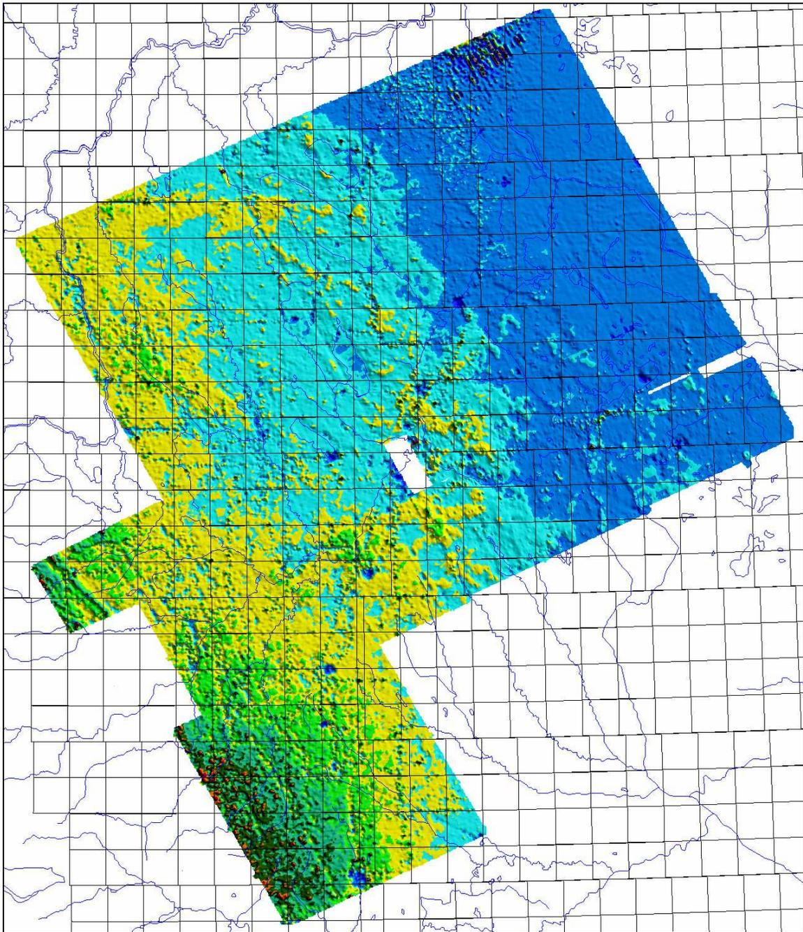
Figure 28: The rnn5, resistivity for fifth layer, merged for the current and previous GEOTEM™ surveys
