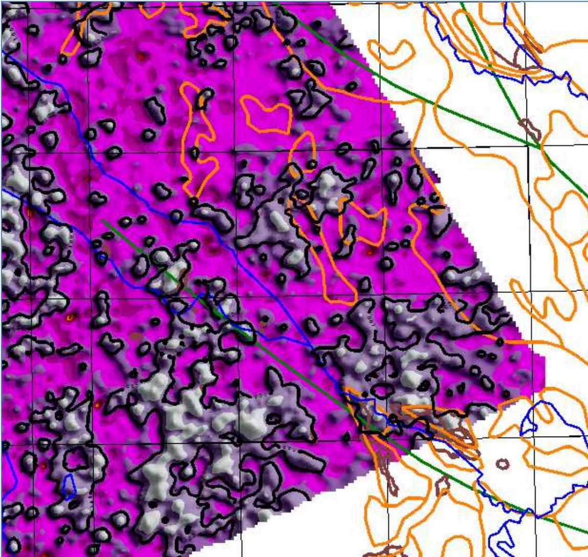
Figure 37: Shaded relief image of the first layer resistivity, mn1, with the AGS features overlain in the SE corner of the survey area. The 100 ohm-m resistivity contours in black lines overlain.
