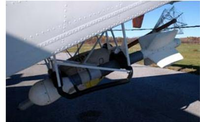
Figure 3: Mag and GEOTEM® Receivers
