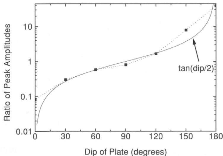
Fig. 6. The ratio of the peak amplitudes of the normalized z-component response (left/right) plotted with solid squares. The ratio plots very close to the tangent of half the dip angle  $\theta$  of the plate.
