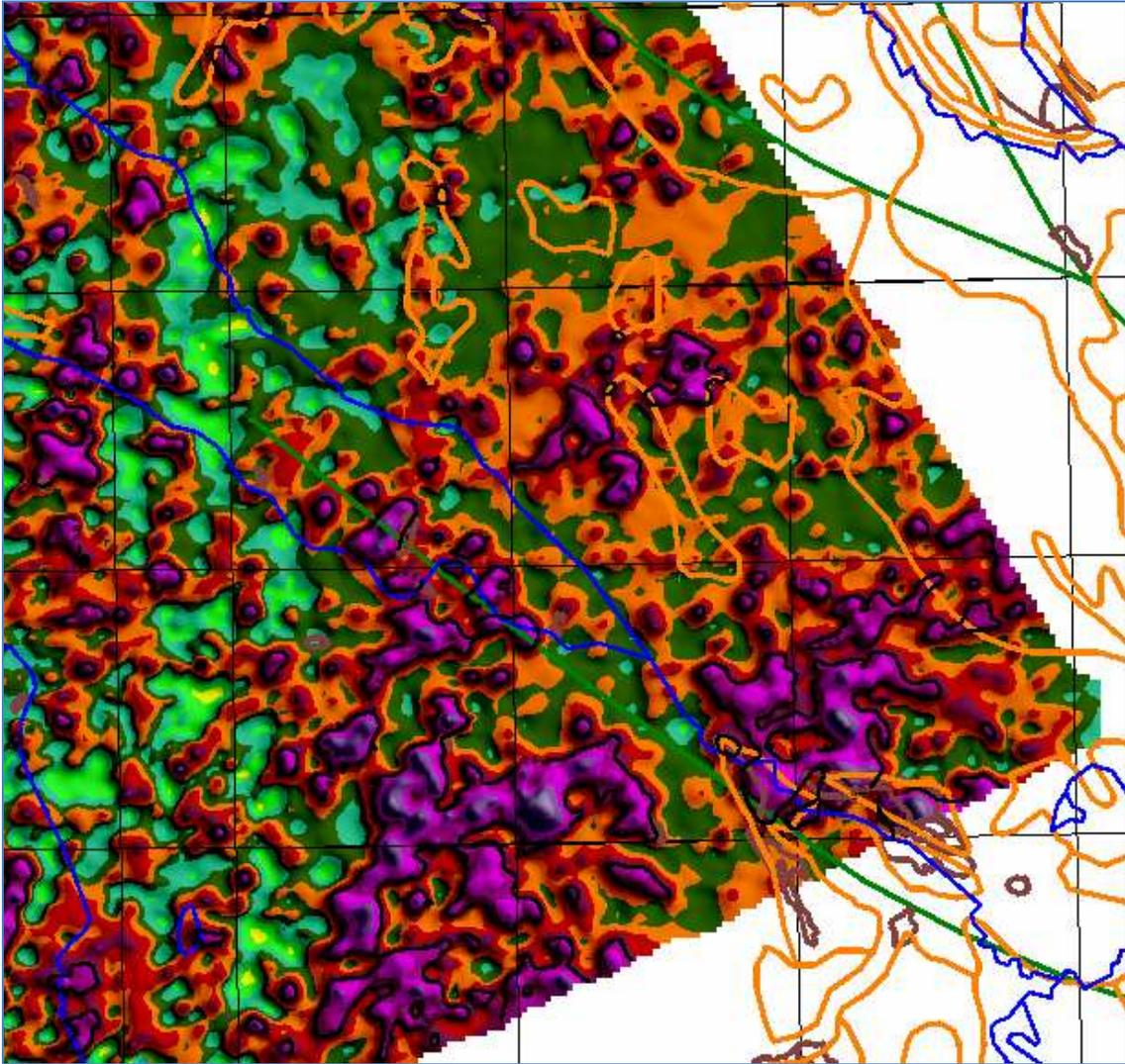
Figure 41: Shaded relief image of the second layer resistivity with the AGS features are overlain for the SE corner of the survey area. Black resistivity contours are overlain at a 50 ohm-m level.
