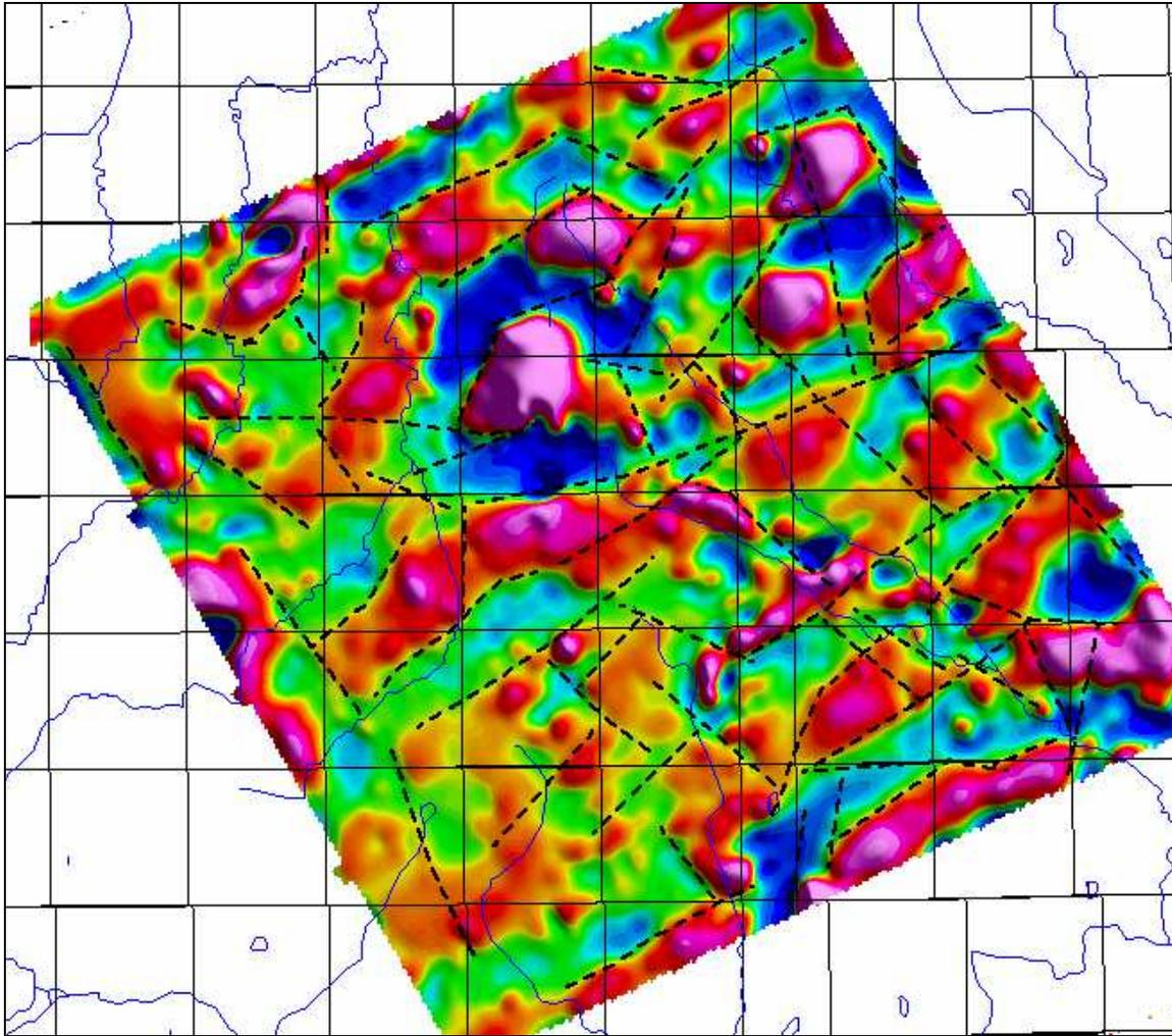
Figure 45c: Band pass filter of the total magnetic field reduced to the pole 2 km to 10km (Bp 1: 2-10k).
