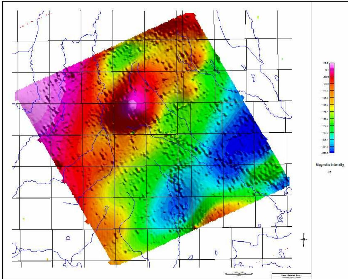
Figure 45a: Shaded relief image of the total magnetic field reduced to the pole.
