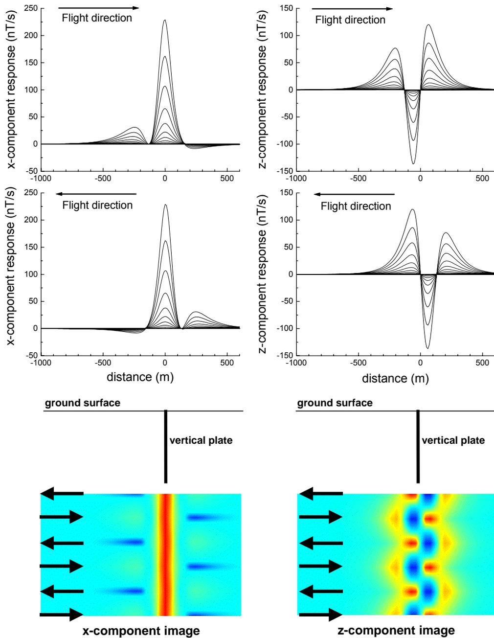
Figure 2. The response over a vertical plate. The left panels show the x-component, the right panels the z-component. The top is flying left to right, the middle is right to left, the bottom is a plan image with the alternating flight directions shown with arrows.
