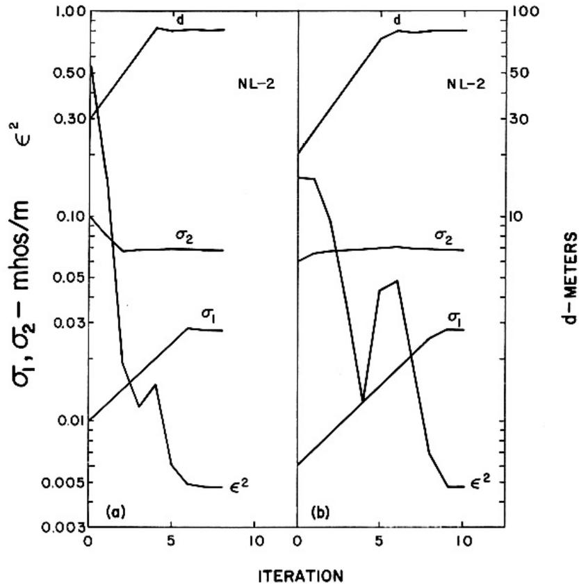
Figure 6: Figure shows the changing conductivity,  $\sigma$ , (inverse of resistivity) and first layer thickness,  $d$ , with iteration for a two layer model. The least square error,  $\epsilon$ , is also shown. The left and right views show the iterative process converge to nearly identical models starting with different starting values for the two layer conductivities and the first layer thickness (After Glenn et al., 1973).
