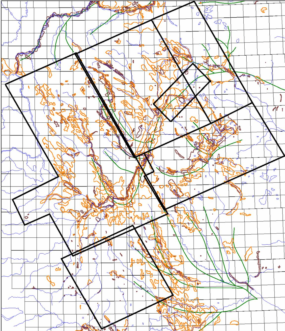
Figure 33a: Map of AGS data: Red color is buried channels, Green color is aggregate, Orange color is coarse sediments. Black lines outline the the survey areas with the current survey in the extreme south west. The small rectangle along the south west border of the south east survey is a data gap over the city of Red Deer. The small inset survey is the RESOLVE™ survey.
