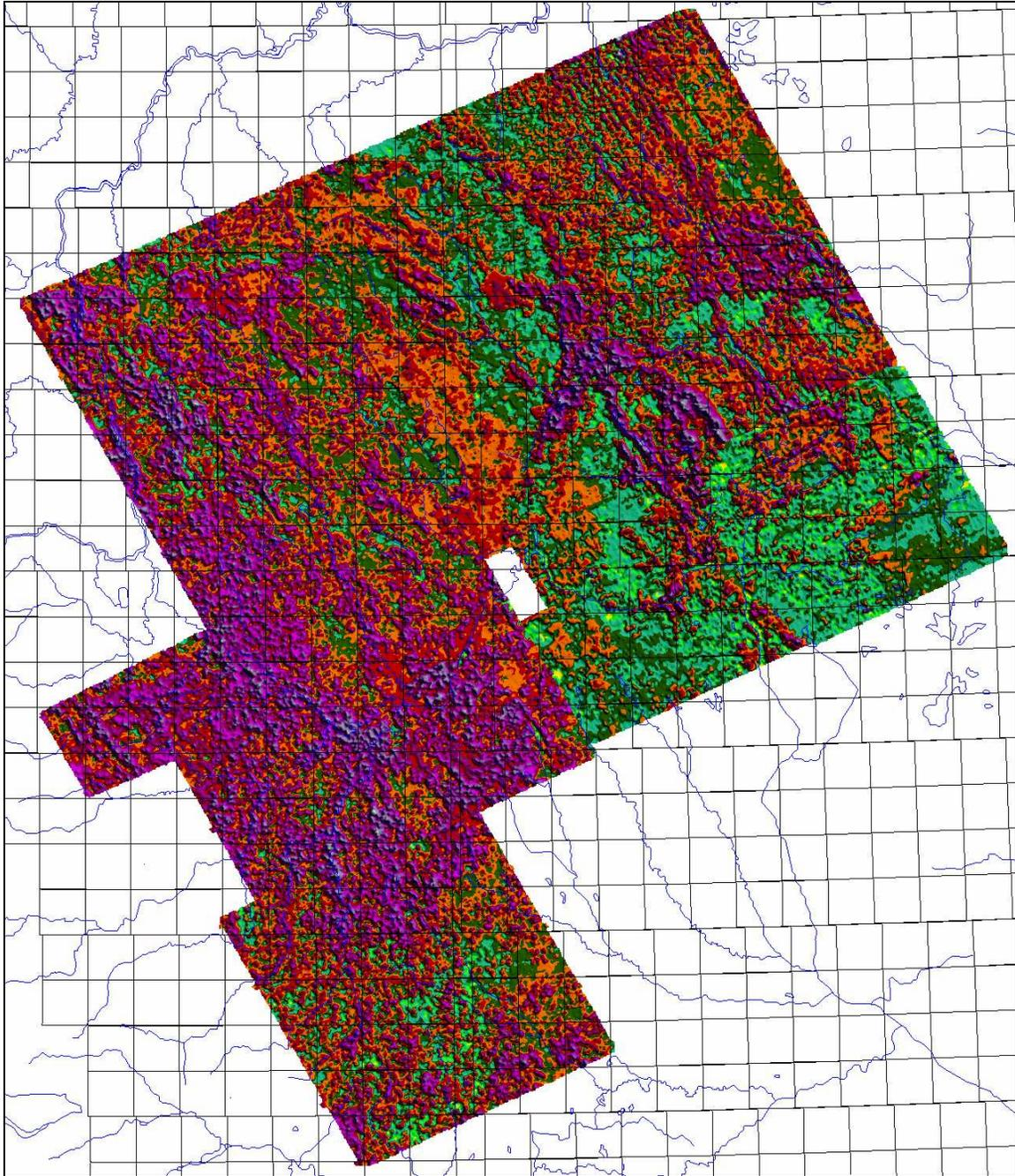
Figure 25: The rnn2, second layer resistivity, merged for the current and previous GEOTEM™ surveys.
