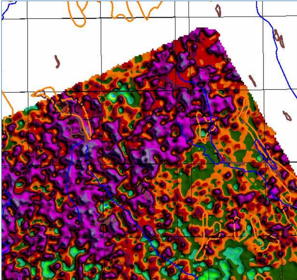
Figure 40: Shaded relief image of the second layer resistivity with the AGS features overlain for the NE corner of the survey area. Black resistivity contours are overlain at 50 ohm-m level.
