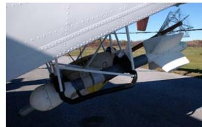
Figure 3: Mag and GEOTEM® Receivers
