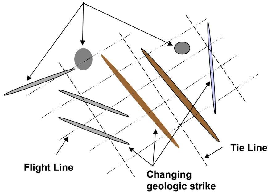
Figure 11: Illustration of aliasing due to flight line spacing
