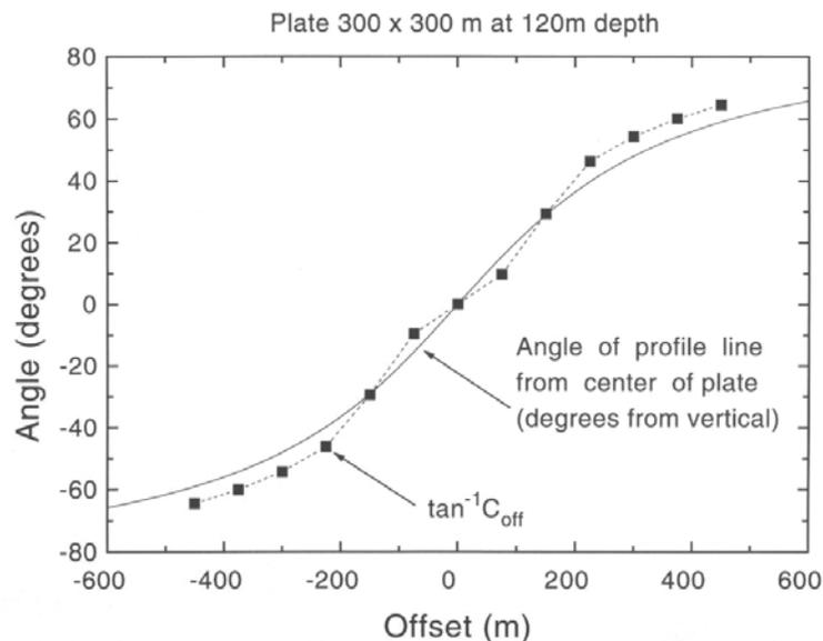
Fig. 15. The arctangent of  $C_{off} = V_y/V_z$ , plotted as a function of varying offset (solid squares). There is good agreement between this quantity and the angle  $\phi$  between a vertical line and the line from the center of the top edge of the plate to the profile line.
