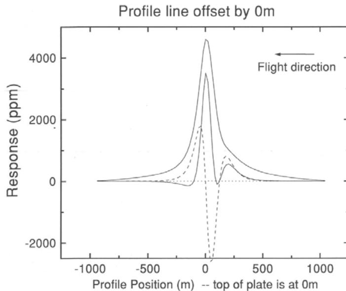
Fig. 9 The response of a 300 by 300 m plate traversed by a profile line crossing the center of the plate in a direction perpendicular to the strike of the plate (the strike angle  $\zeta$  of the plate with respect to the profile line is  $90^\circ$ ).
