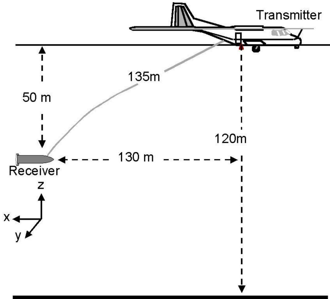
Figure 1. Nominal geometry of the MEGATEM/GEOTEM system.
