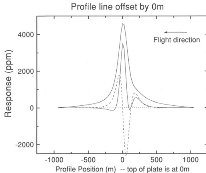
Fig. 9 The response of a 300 by 300 m plate traversed by a profile line crossing the center of the plate in a direction perpendicular to the strike of the plate (the strike angle  $\zeta$  of the plate with respect to the profile line is  $90^\circ$ ).
