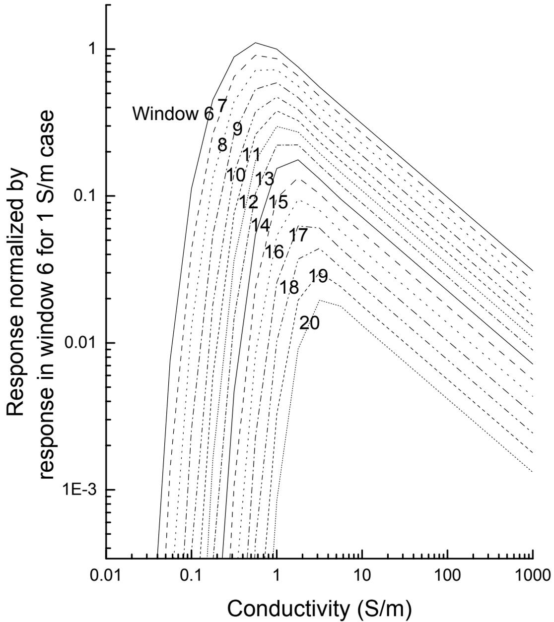
Figure 16. Nomogram for windows 6-20 normalized to a response from a 1 Siemen conductor in window 6.
