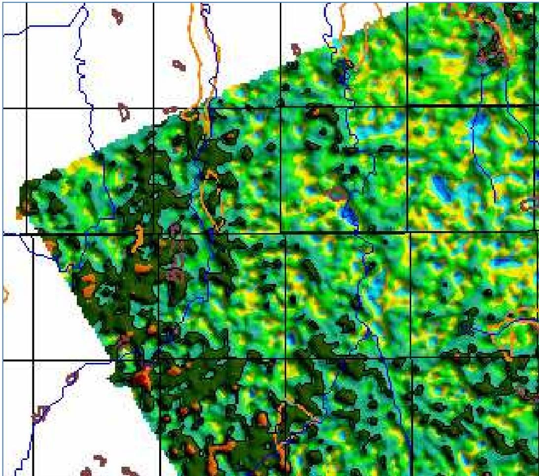
Figure 42a: Shaded relief image of the third layer resistivity with the AGS features overlain in the NW corner of the survey area. Black contours are overlain at a 30 ohm-m level.
