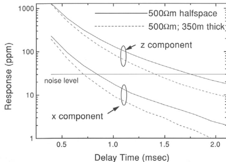
Fig. 2. The response for a  $500 \Omega\cdot\text{m}$  half-space (solid line) and a  $500 \Omega\cdot\text{m}$  layer of thickness  $350 \text{ m}$  overlying a resistive half-space (dashed line). The  $z$ -component responses are the two curves with the larger amplitudes and the two  $x$ -component response curves are 6 to 10 times smaller than the corresponding  $z$  component. A noise level of 30 ppm is considered to be typical of both components in the absence of strong spherics.
