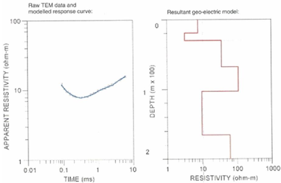
Figure 9: Layered earth inversion of a time domain decay curve, left, using a 6 layered model, right (from Associated Geosciences). The measured points are small boxes in the left figure and the model result is the smooth curve through these points. These data are from a ground survey.
