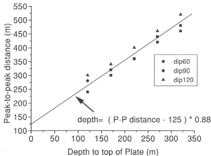
Fig. 8. The peak-to-peak distance as a function of plate depth for three different dip angles  $\theta$ . A variation in dip of  $\pm 30^\circ$  does not result in a large change in the peak to peak distance.
