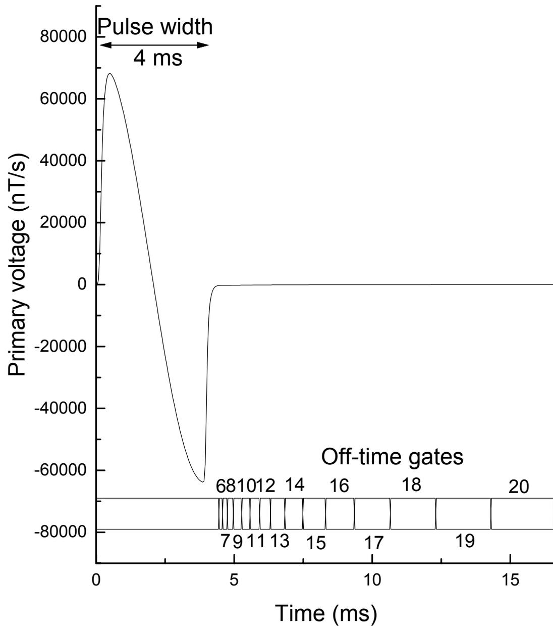
Figure 2. Theoretical transmitter waveform response in the receiver.
