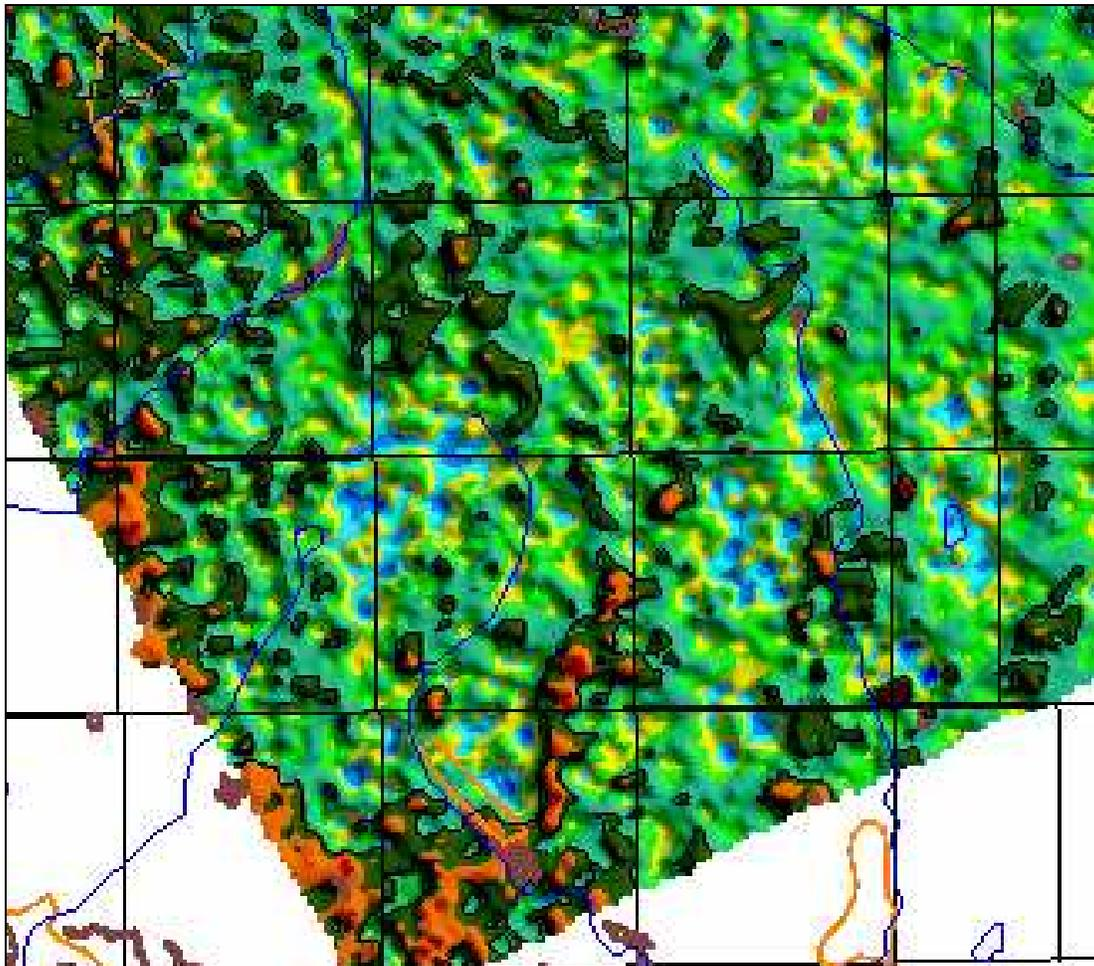
Figure 42b: Shaded relief image of the third layer resistivity with the AGS features overlain in the SW corner of the survey area. Black contours are overlain at a 30 ohm-m level.
