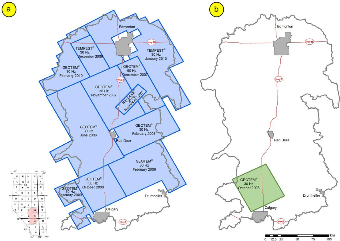
**Figure 2. a) Location of the 11 geophysical survey blocks in the Edmonton–Calgary Corridor, Alberta. The type of geophysical survey completed and when it was completed are provided on each survey block. b) Location of the survey block north of Calgary, Alberta. Inset depicts the location of the ECC, Alberta.**
