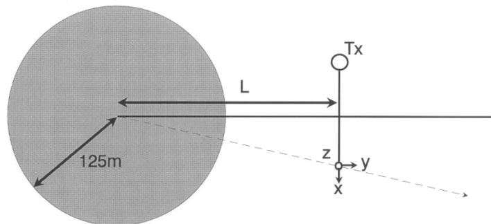
Fig. 16. Plan view of a flat-lying conductor (a circular loop with a radius of 125 m). The AEM system is offset a distance  $L$  from the center of the conductor in a direction perpendicular to the traverse direction. The traverse direction of the system is from the bottom to the top of the figure.
