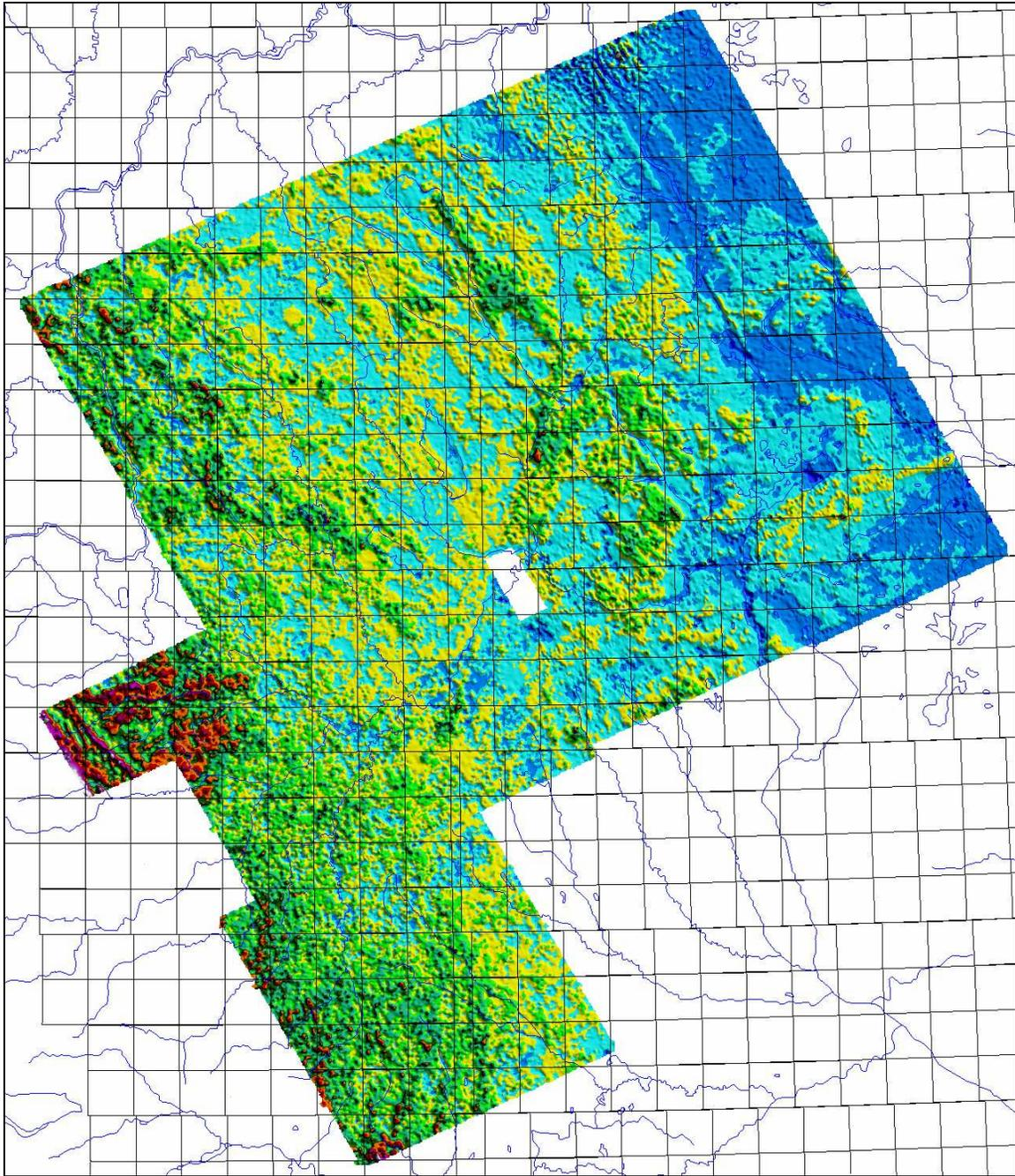
Figure 31: The Thnn3, thickness for third layer, merged for the current and previous GEOTEM™ surveys
