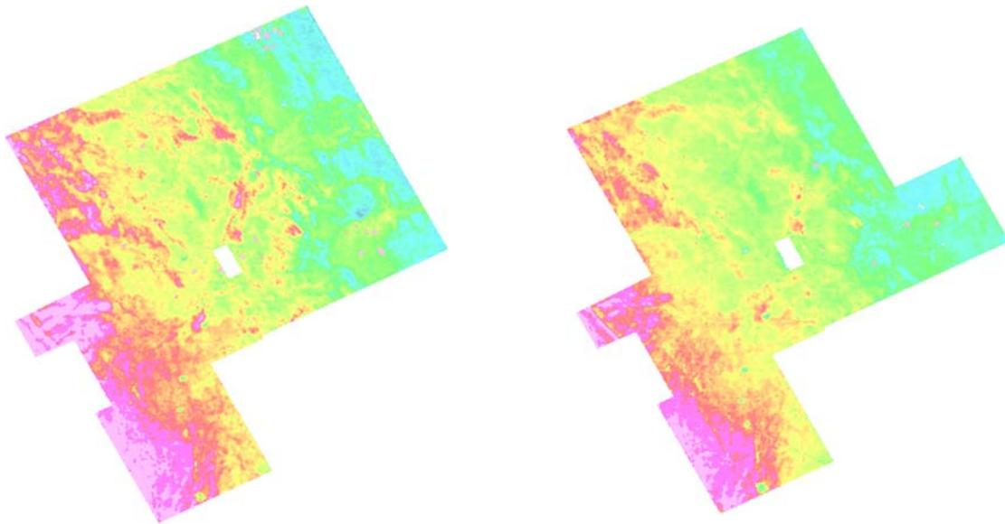
Figure 3. Resistivity Depth Slices at 60 metres (left) and 120 metres (right)
