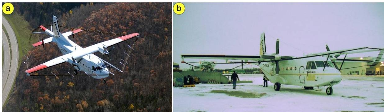
Figure 4. a) The GEOTEM<sup>®</sup> survey technique in flight. Note the transmitting loop fixed to the aircraft's nose, tail and wing tips. Primary electromagnetic pulses are created by a series of discontinuous sinusoidal current pulses and transmitted into the transmitting loop. b) Modified Casa 212 aircraft used by Fugro Airborne Surveys in this study.
