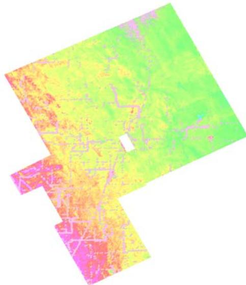
Figure 4. Apparent Resistivity Derived from Z Coil Channels 1 to 20
