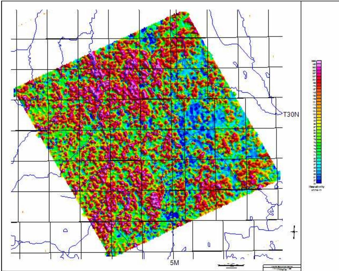
Figure 13b: The first layer resistivity shaded relief image, rnn1 using a rainbow, histogram equalization palette.
