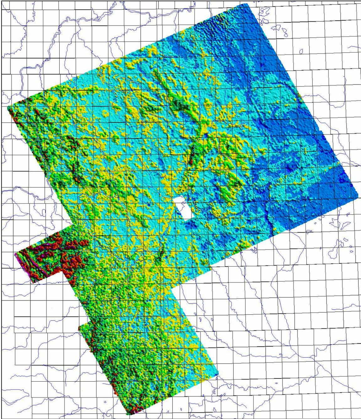
Figure 30: The Thnn2, thickness for second layer, merged for the current and previous GEOTEM™ surveys
