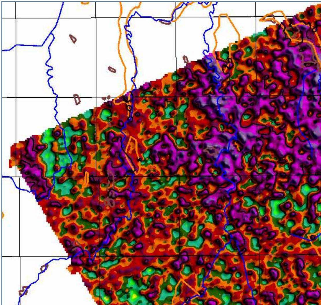
Figure 39: Shaded relief image of the second layer resistivity with the AGS features overlain in the NW corner of the area. Black resistivity contours are overlain at 50 ohm-m levels.
