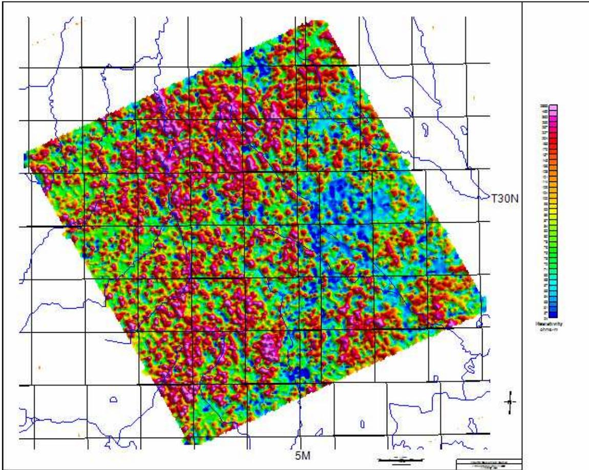
Figure 13b: The first layer resistivity shaded relief image, rnn1 using a rainbow, histogram equalization palette.
