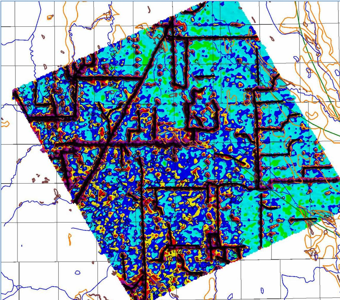
Figure 34b: The per cent error image with the high resistivity features highlighted by black lines. Features are likely cultural affects such as pipelines.
