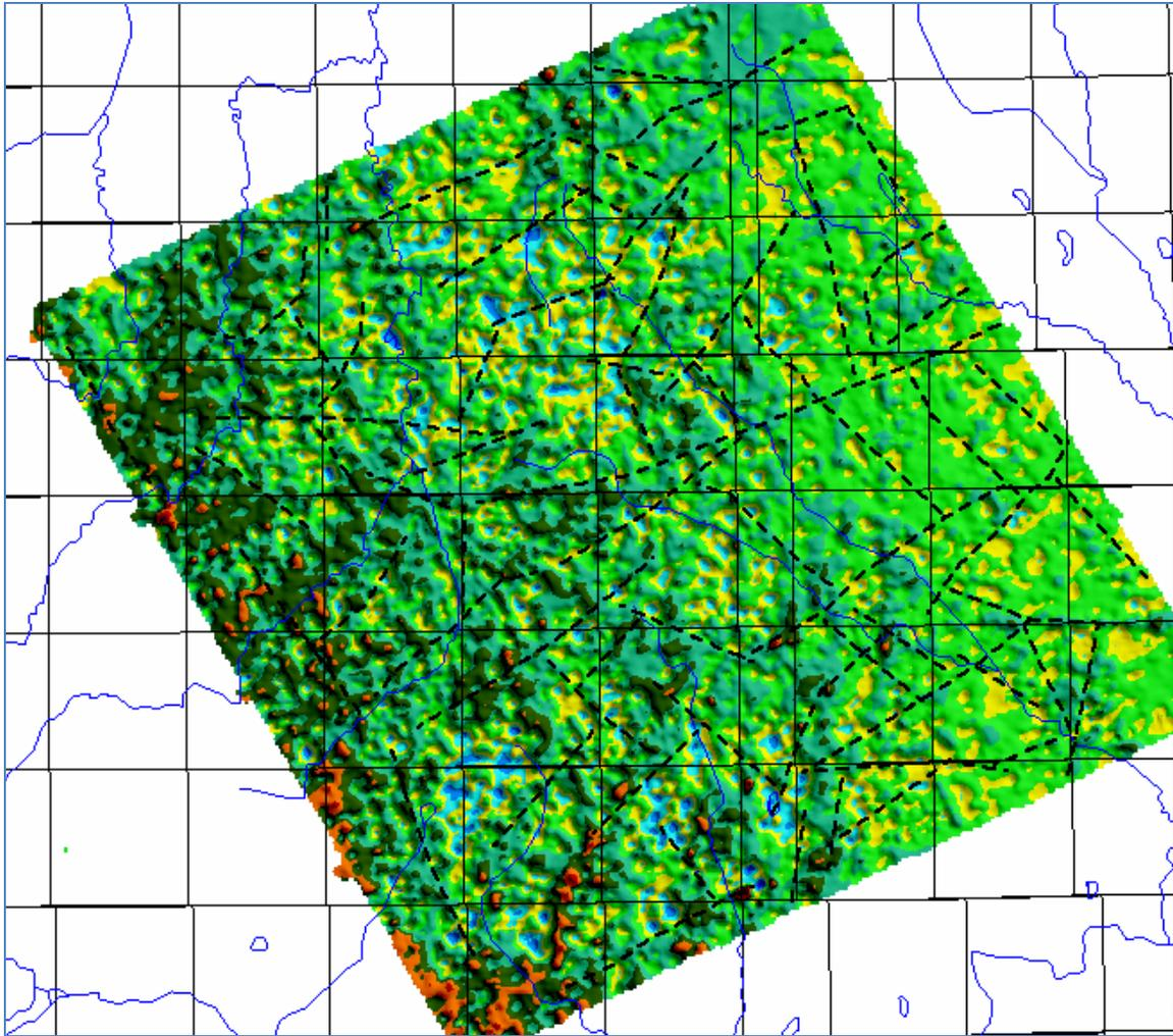
Figure 46: The third layer resistivity,  $R_{nn3}$ , with the interpreted magnetic lineaments overlain
