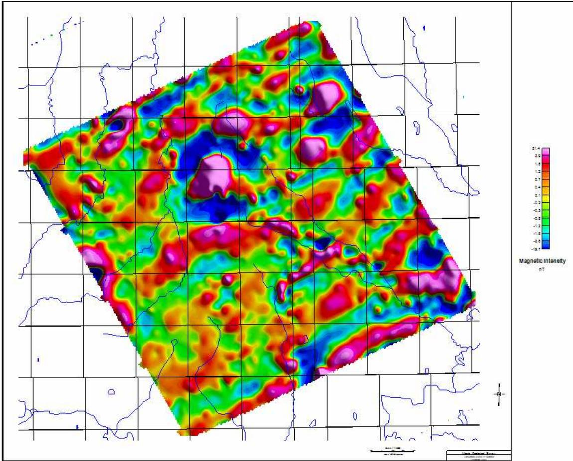
Figure 45b: Band pass filter of the total magnetic field reduced to the pole 2 km to 10km (Bp 1: 2-10k).
