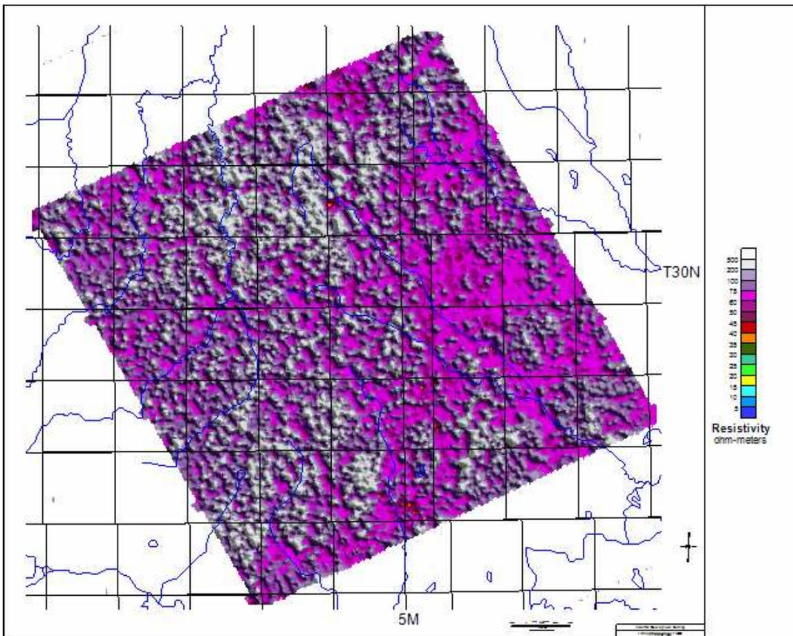
Figure 13a: The first layer resistivity shaded relief image, *rnn1*
