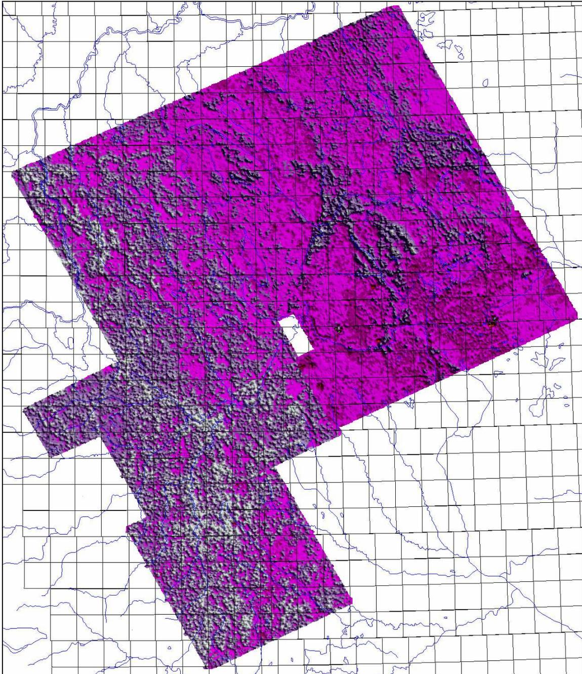
Figure 24: The rnn1, first layer resistivity, merged for the current and previous GEOTEM™ surveys.
