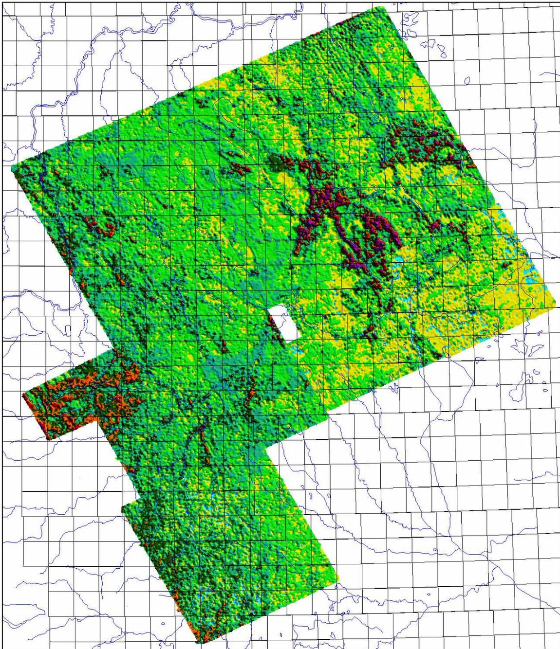
Figure 26: The mn3, third layer resistivity, merged for the current and previous GEOTEM™ surveys
