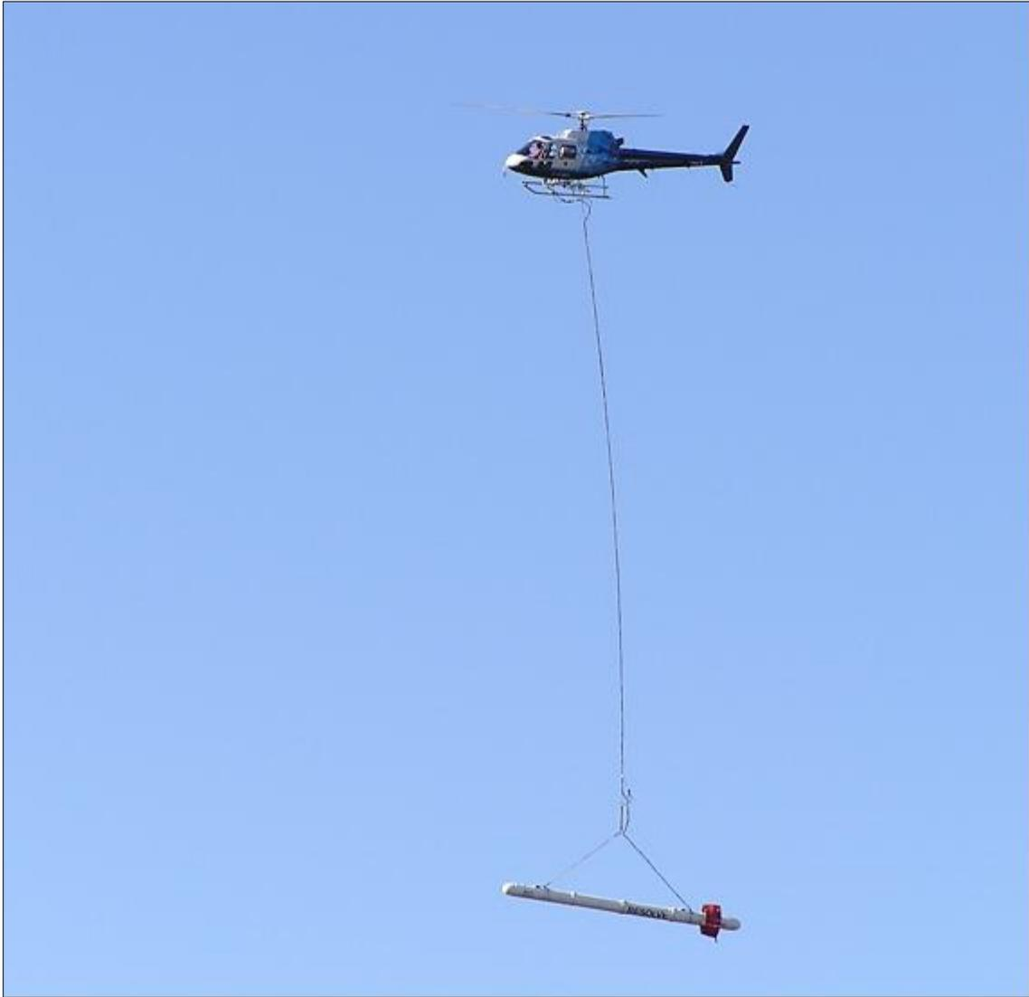
Figure 1: Fugro Airborne Surveys RESOLVE EM bird
