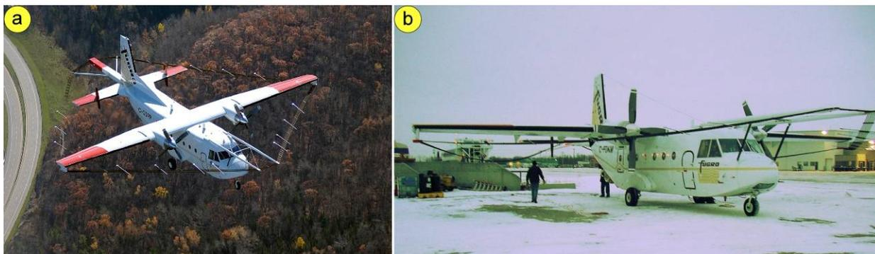
Figure 5. a) The GEOTEM<sup>®</sup> survey technique in flight. Note the transmitting loop fixed to the aircraft's nose, tail and wing tips. Primary electromagnetic pulses are created by a series of discontinuous, sinusoidal current pulses and transmitted into the transmitting loop. b) Modified Casa 212 aircraft used by Fugro Airborne Surveys in this study.
