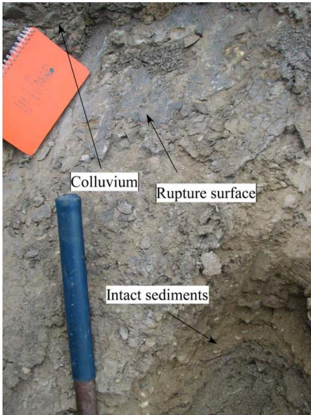
Figure 22. Rupture surface of landslide shown in Figure 21 showing colluvial material on top of intact Quaternary sediments. Location: east side of the Heart River, Peace River Alberta, left flank of landslide (483425E, 6231130N, UTM Zone 11, NAD83).
