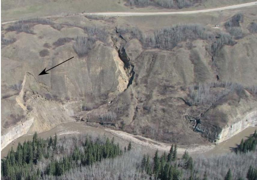
Figure 21. Oblique aerial photo of a landslide seated in colluvium along the east side of the Heart River. Debris can be seen spilling over the Peace River Formation sandstone into the river. Location: Peace River, Alberta (483520E, 6231090N, UTM Zone 11, NAD83).
