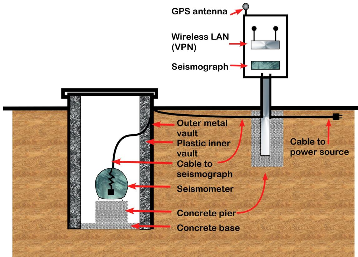
Figure 46. Schematic cross-section of an Alberta Telemetered Seismograph Network (ATSN) station installation. Abbreviations: LAN, local area network; VPN, virtual private network.
