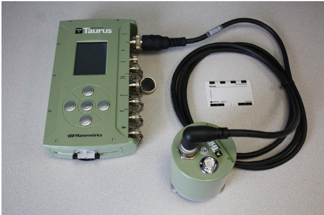
Figure 48. Compact seismometer and digitizer similar to the equipment deployed in the Strachan temporary array.
