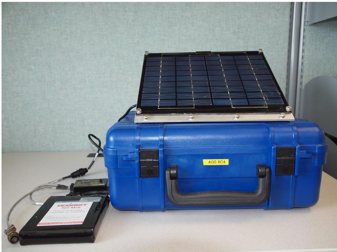
Figure 49. Transport and deployment case for temporary seismic stations. The battery shown on the left is normally inside the protective case.
