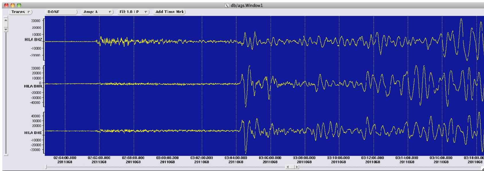
Figure 10. Seismogram from seismic station HILA, showing the 7.2 Mw event near the east coast of Honshu, Japan on March 9, 2011 at 02:45:18 Co-ordinated Universal Time (UTC).
