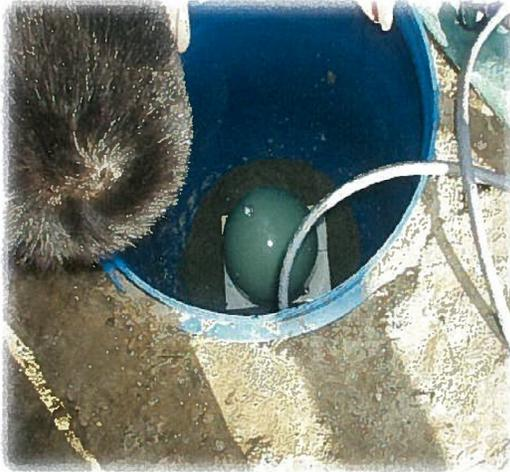
The seismometer is placed below the surface on a concrete pad, to minimize the effects of surface vibrations and wind noise. The instrument is capable of detecting earthquakes from around the world.
