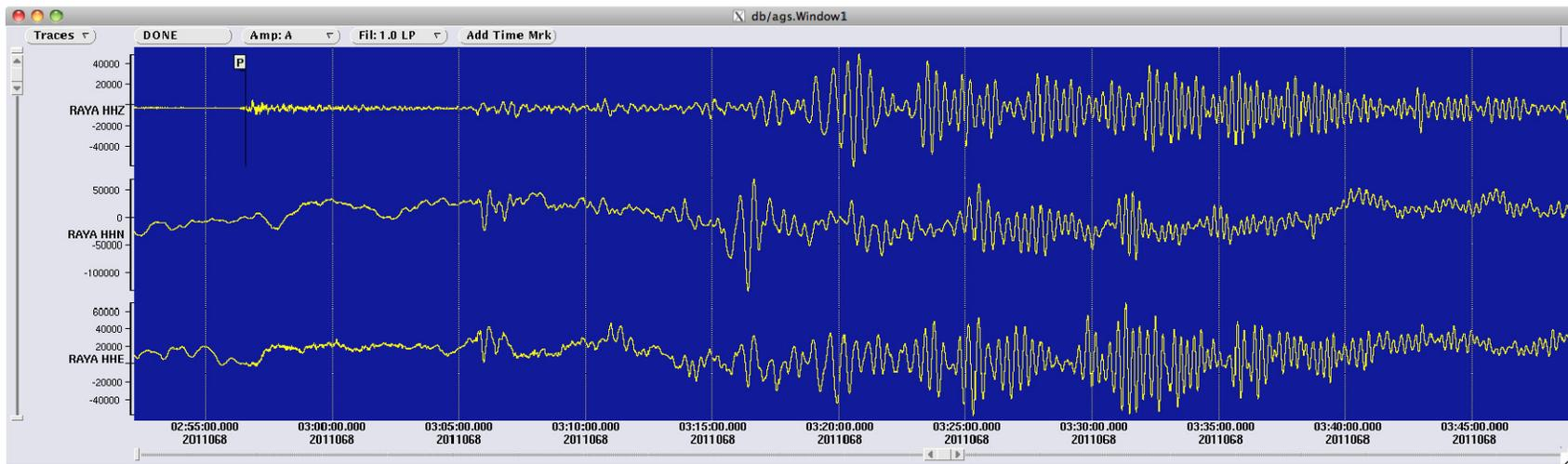
Figure 18. Seismogram from seismic station RAYA, showing the 7.2 Mw event near the east coast of Honshu, Japan on March 9, 2011 at 02:45:18 Co-ordinated Universal Time (UTC). The flag marked 'P' is the p-arrival pick from an automated detection and association algorithm.
