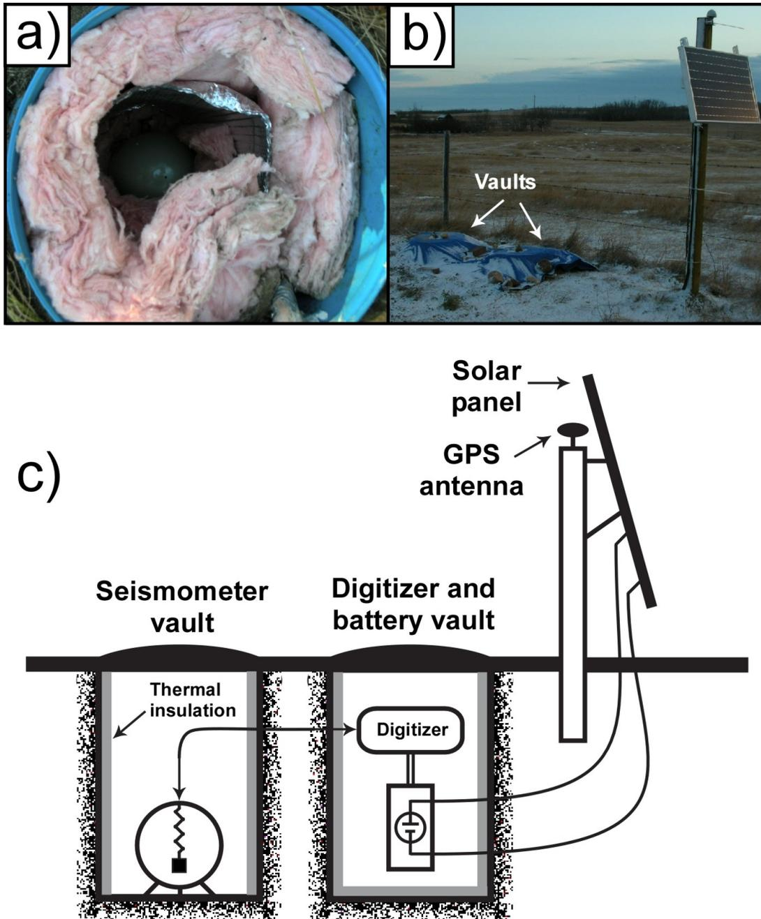
Figure 47. Configuration of Canadian Rockies and Alberta Network (CRANE) stations: a) view looking into vault from above, b) surface view of installed vaults and solar panel, and c) schematic cross-section of buried vaults (photo courtesy of J. Gu).
