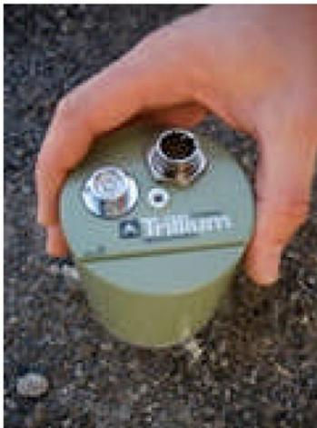
The temporary seismometer is about the size of an oil filter. It is placed 30 cm below the surface on a patio stone, to minimize the effects of surface vibrations and wind noise. The instrument is covered with a protective insulated housing and covered with soil.
