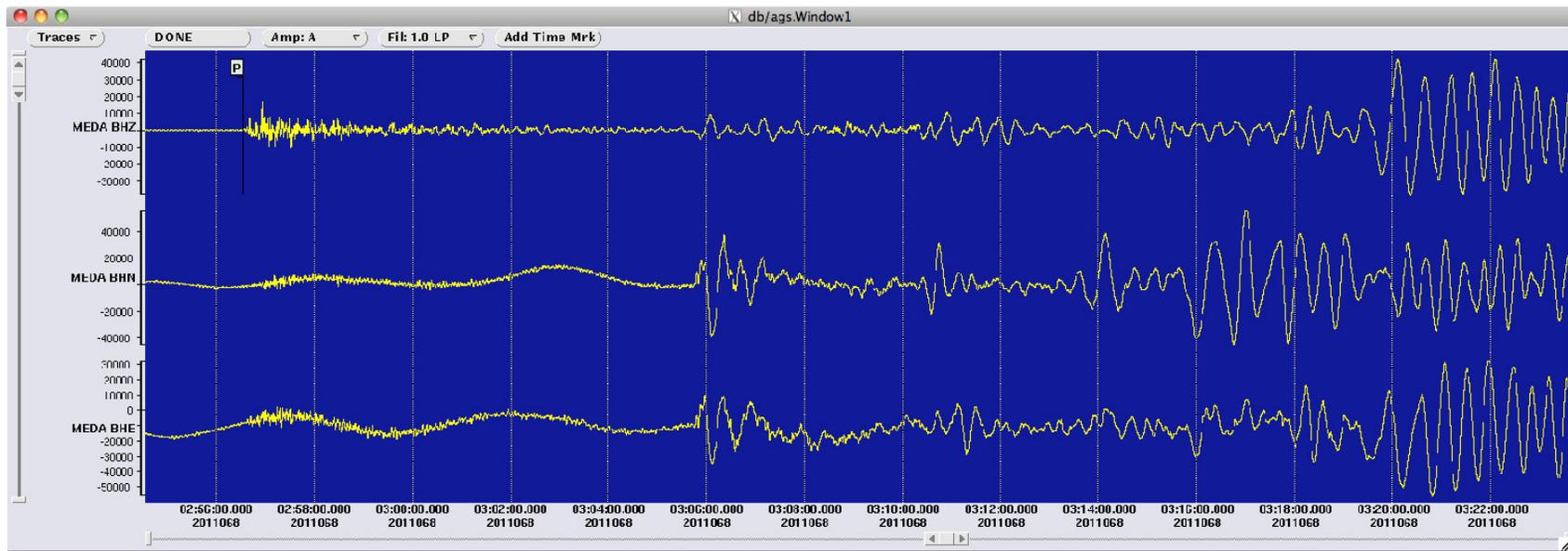
Figure 15. Seismogram from seismic station MEDA, showing the 7.2 Mw event near the east coast of Honshu, Japan on March 9, 2011 at 02:45:18 Co-ordinated Universal Time (UTC). The flag marked 'P' is the p-arrival pick from an automated detection and association algorithm.
