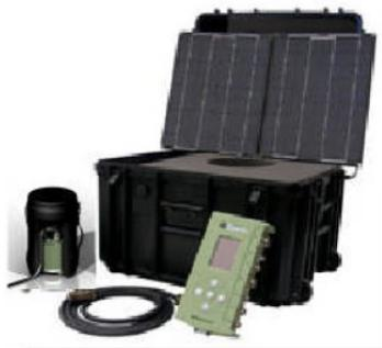
Components of a temporary seismograph station. Seismometer (right); electronics and solar panel (left) which remains above ground.
