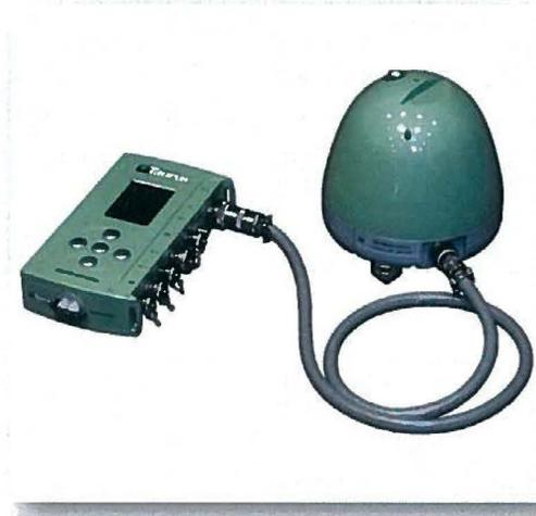
Components of a seismograph station: seismometer (right); digital seismograph (left). The seismometer is about the same size as a bowling ball.
