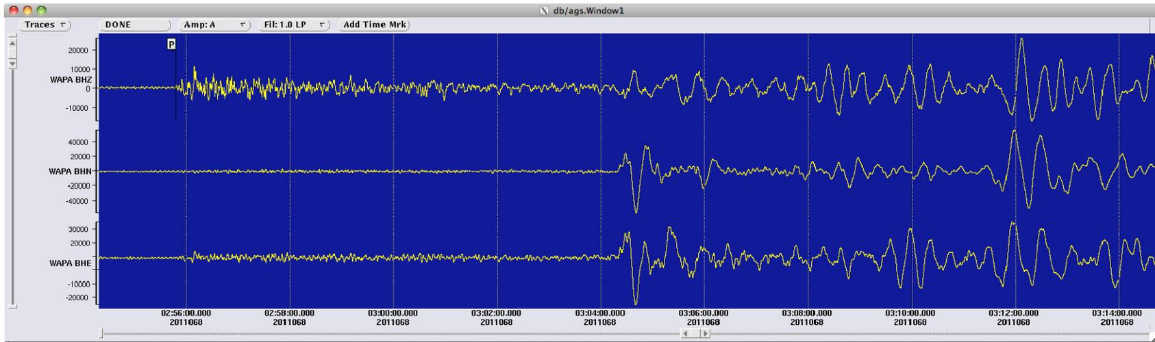
Figure 24. Seismogram from WAPA, showing the 7.2 Mw event near the east coast of Honshu, Japan on March 9, 2011 at 02:45:18 Co-ordinated Universal Time (UTC). The flag marked 'P' is the p-arrival pick from an automated detection and association algorithm.
