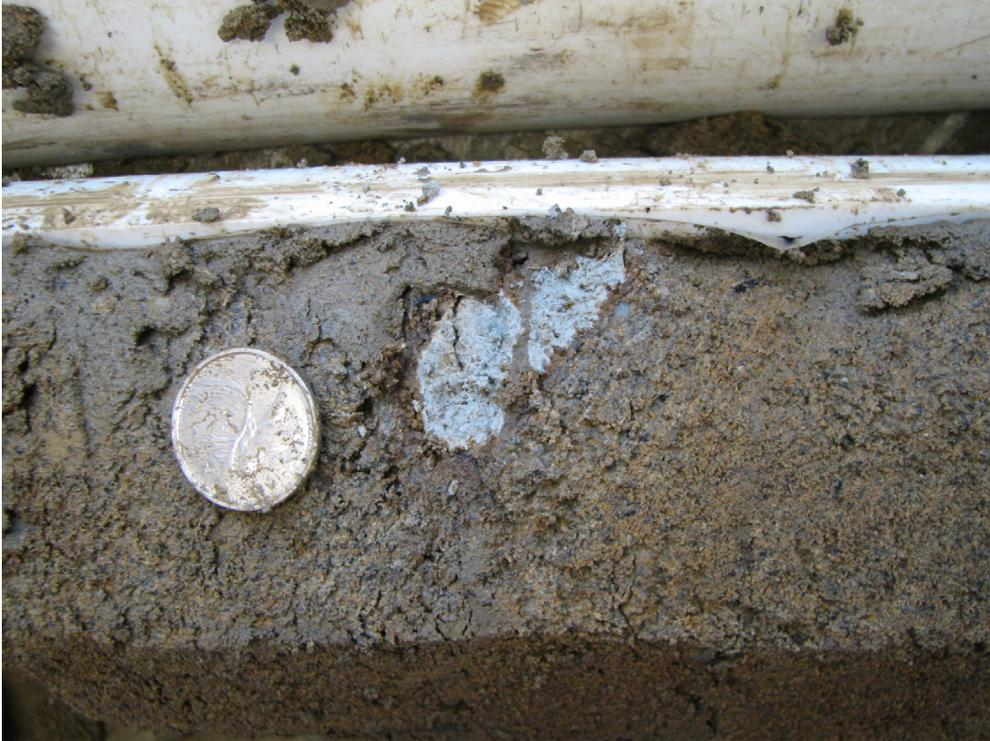
Figure 103. Carbonate interclast (right of coin) in medium-grained sands (PR08-5; 99.1–100.1 m; 439.3–438.3 m asl).
