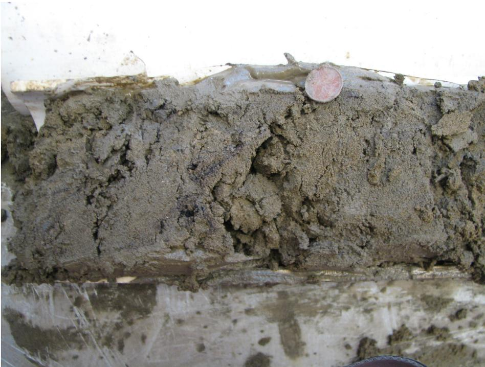
Figure 96. Silty, fine- to medium-grained sand; sample lost downhole and re-recovered (PR08-5; 91.4–91.8 m; 446.9–446.5 m asl).
