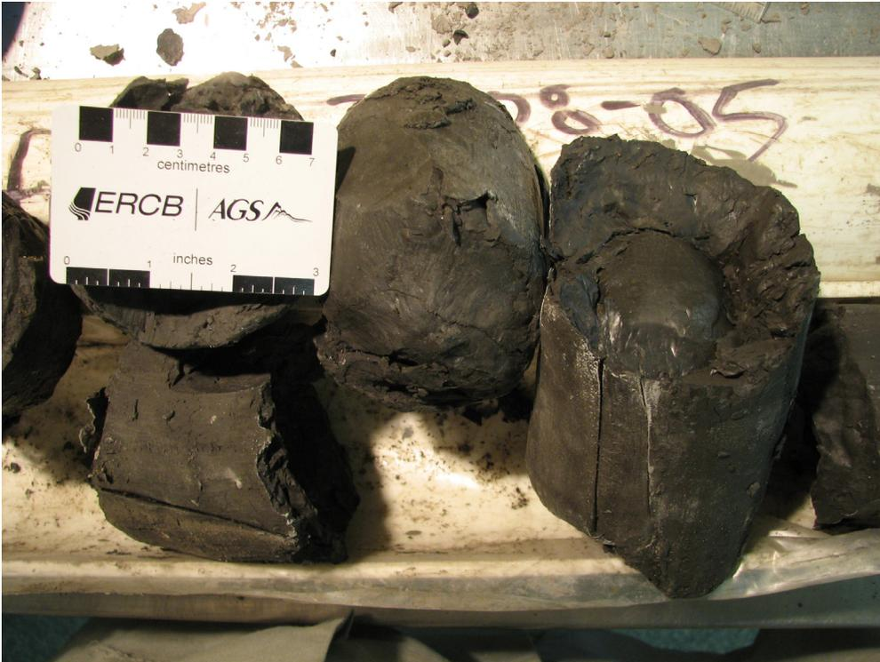
Figure 82. Slickensides in silty clay to clayey silt (Note: Slickensides appear to be drill-induced), (PR08-5; 79.2–80.8 m; 459.1–457.6 m asl).
