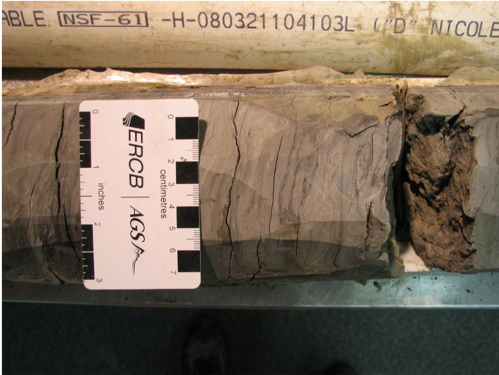
Figure 107. Clayey silt to silty clay, wisps of silty, very fine sand throughout (PR08-5; 101.3–102.1 m; 437.1–436.2 m asl).
