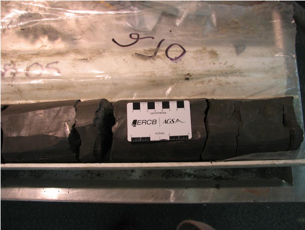
Figure 84. Slickensides within clayey silt to silty clay (Note: Slickensides appear to be drill-induced), (PR08-5; 80.8–82.3 m; 457.6–456.1 m asl).
