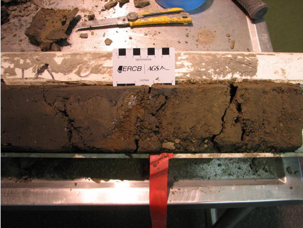
Figure 57. Erosional contact between silty sand (right of flagging tape) and overlying clayey sandy silt to silty sand, stony diamicton (left of flagging tape; 28.8–29 m; 509.6–509.4 m asl).
