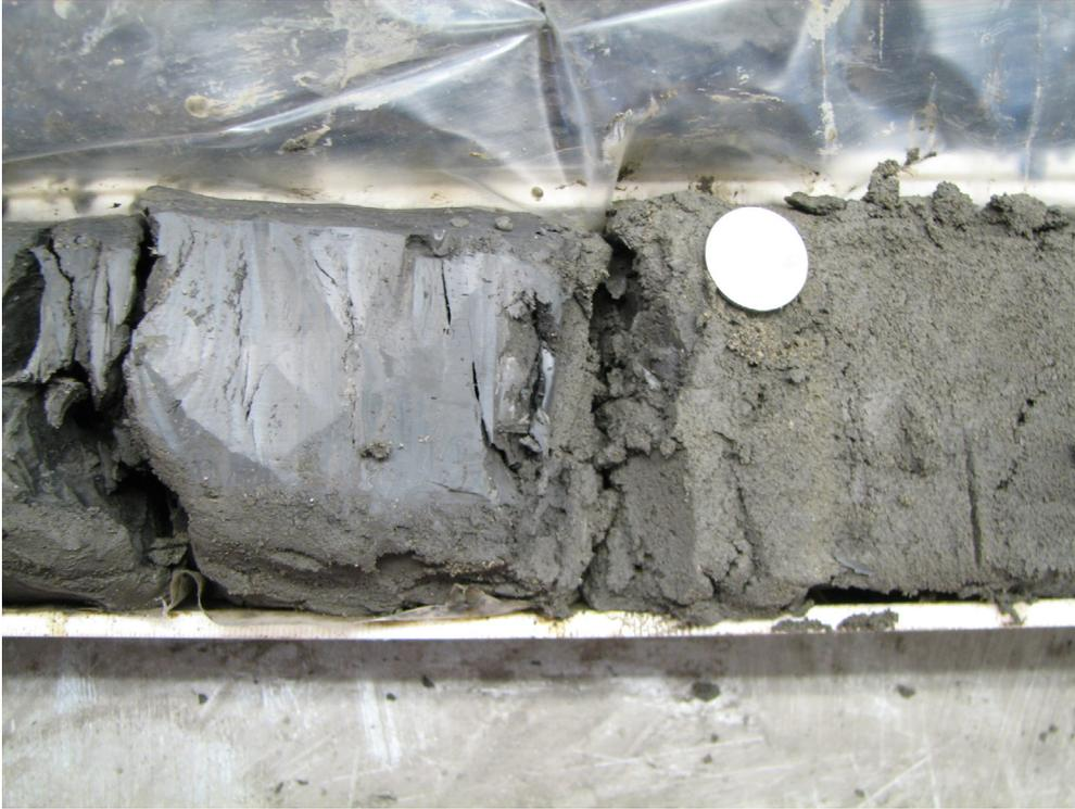
Figure 85. Gradational contact between silty clay to clayey silt and fine- to medium-grained sand (PR08-5; 84.1 m; 454.3 m asl).
