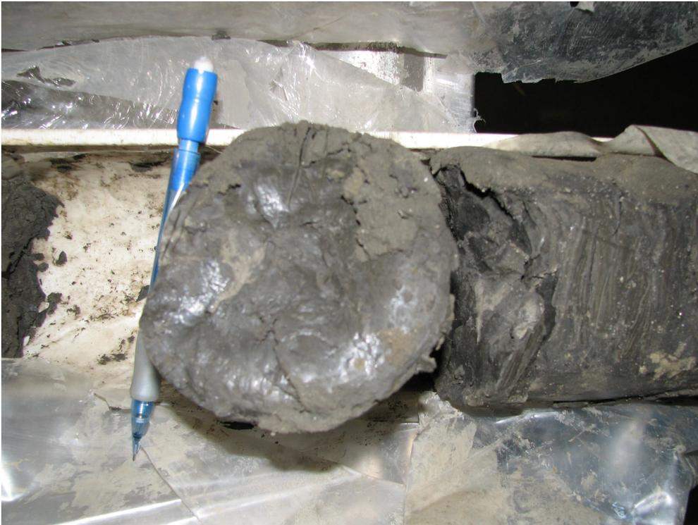
Figure 86. Slickenside within silty clay to clayey silt (PR08-5; 83.8–84.1 m; 454.5–454.2 m asl).
