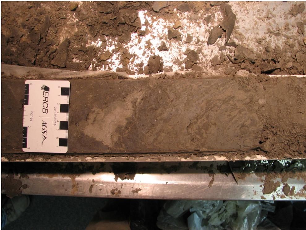
Figure 60. Interclasts of very fine grained sand (PR08-5; right of scale card) in clayey sandy silt to silty sand, stony diamicton (PR08-5; 44.2–45.7 m; 494.2–492.6 m asl).
