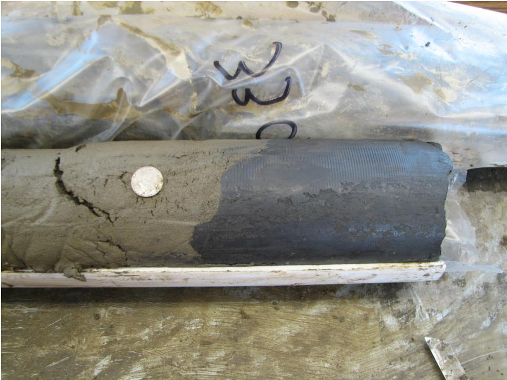
Figure 104. Erosive contact between silty fine sand and silty clay (PR08-5; 100.4–100.6 m; 438–437.8 m asl).
