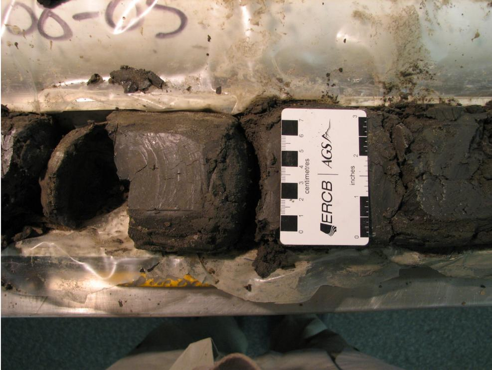
Figure 91. Clayey silt to silty clay, laminated, with horizontal slickenside surfaces (PR08-5; 87.8–88.2 m; 450.5–450.1 m asl).
