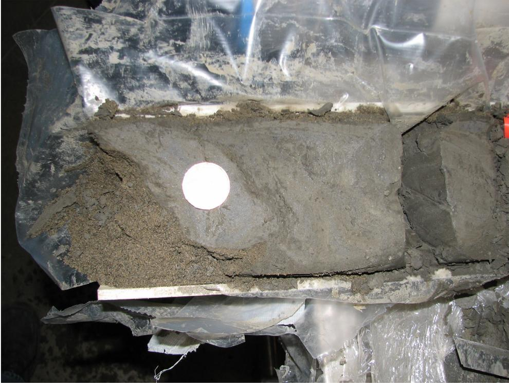
Figure 89. Erosive contact between fine- to medium-grained silty sand and silty clay to clayey silt (PR08-5; 85.3–85.6 m; 453–452.7 m asl).
