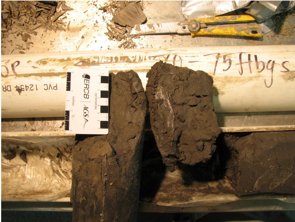
Figure 55. Fractures (jointing?) in silt-rich diamicton; surface mostly obscured by drilling mud (PR08-5; 21.3–22.9 m; 517–515.5 m asl).
