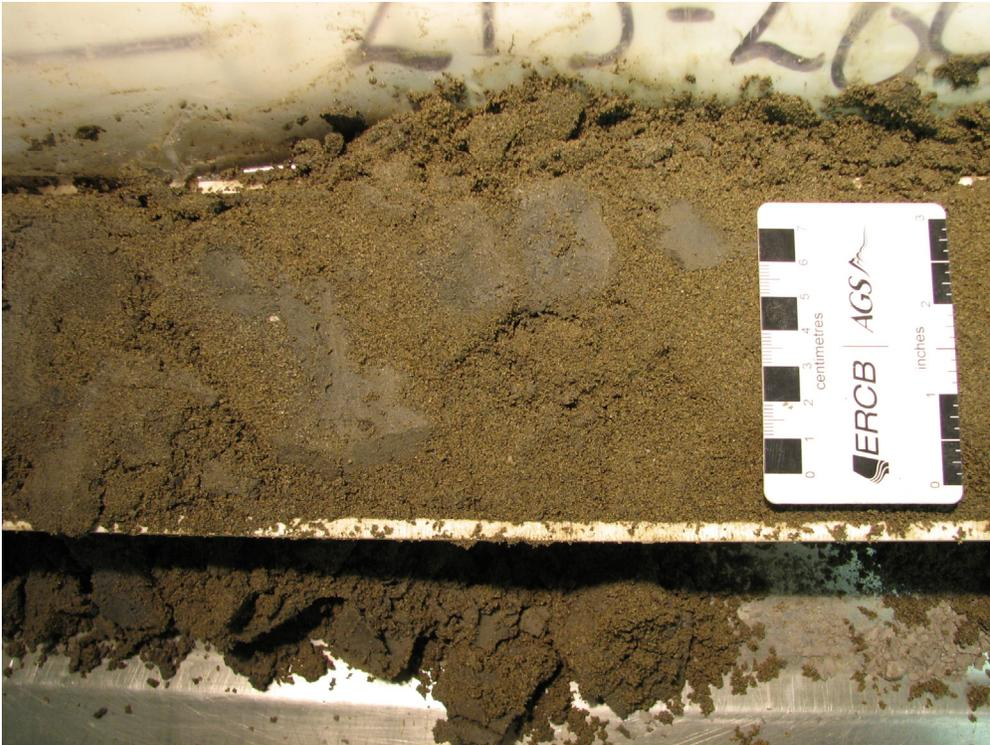
Figure 88. Medium- to coarse-grained silty sand with interclasts of clayey silt (PR08-5; 84.2–84.6 m; 454.2–453.8 m asl).
