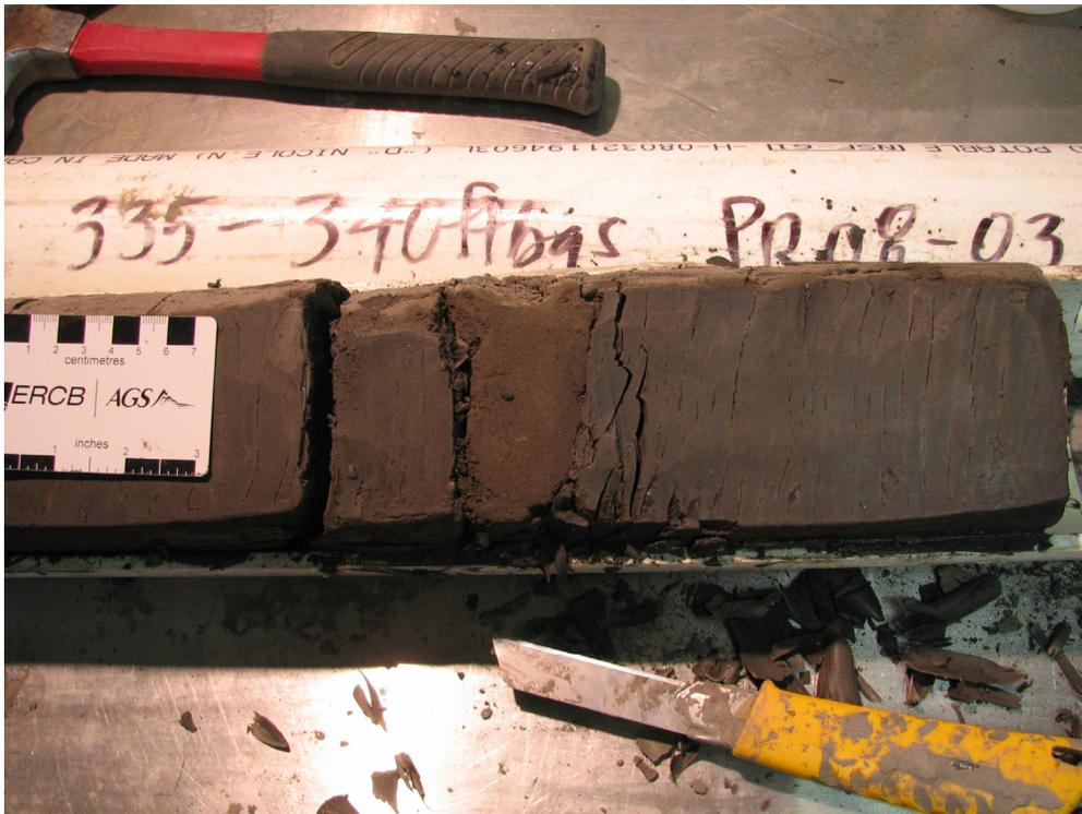
Figure 36. Rhythmically bedded silty sand, silt and clay (PR08-3; 103.4 m; 341.9 m asl).
