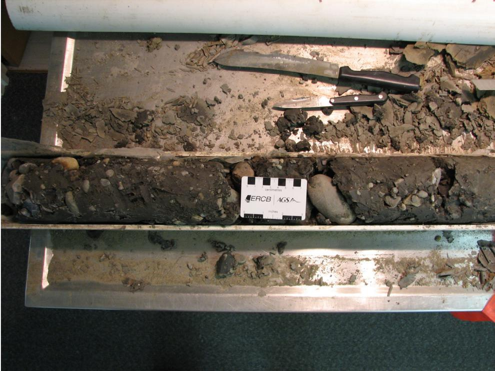
Figure 69. Clayey sandy silt to silty sand, stony diamicton; clast size ranges between small pebble and cobble grade (PR08-5; 54.2–54.9 m; 484.2–483.5 m asl).
