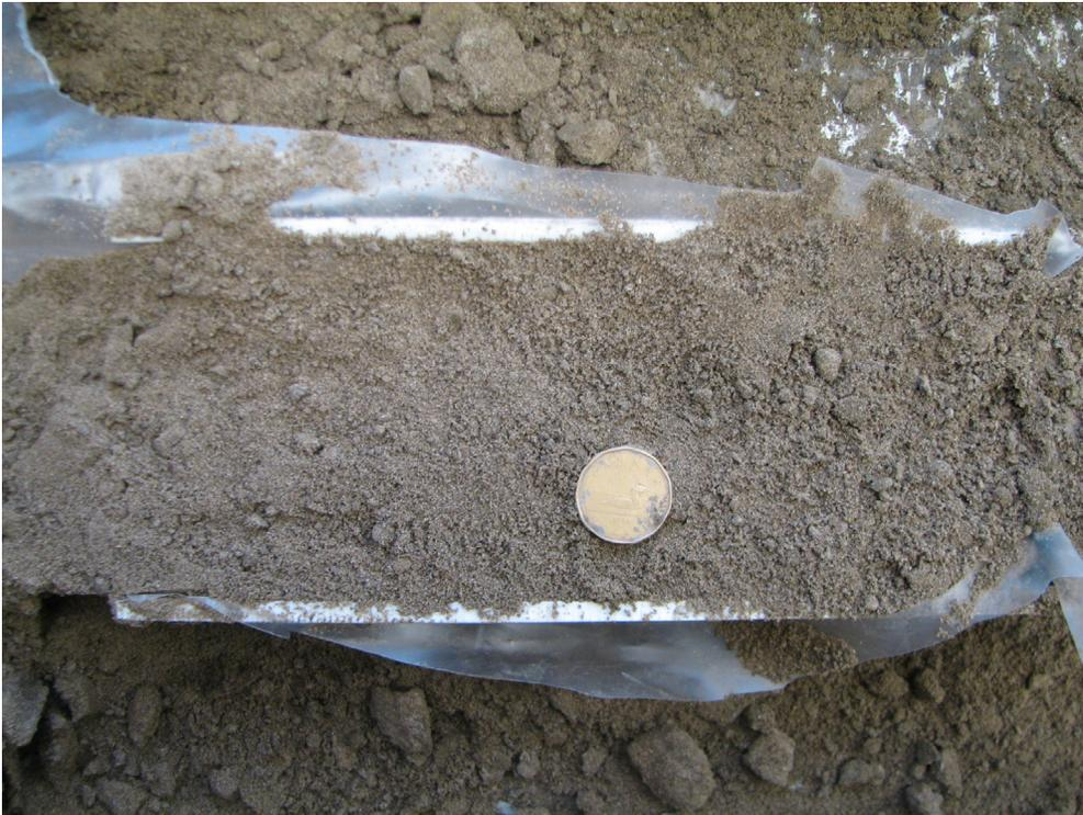
Figure 52. Fine- to medium-grained sand (PR08-5; 17.7–18.3 m; 520.7–520.1 m asl).
