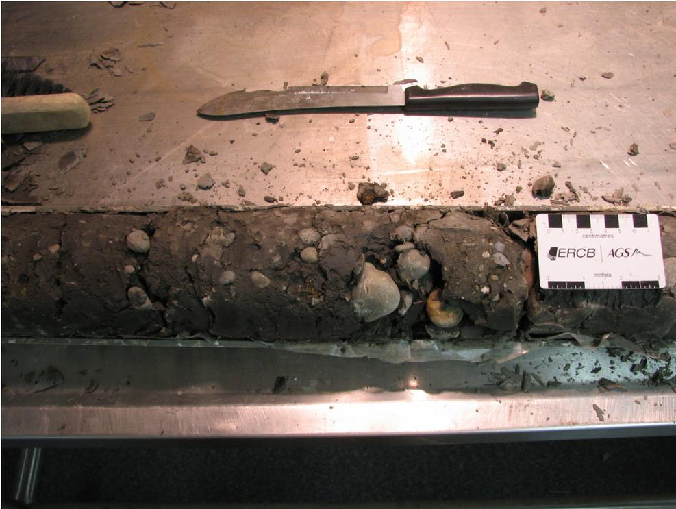
Figure 76. Clayey sandy silt to silty sand, stony diamicton; clast size ranges between small pebble and cobble grade (PR08-5; 56.4–57.9 m; 482.4–481.9 m asl).
