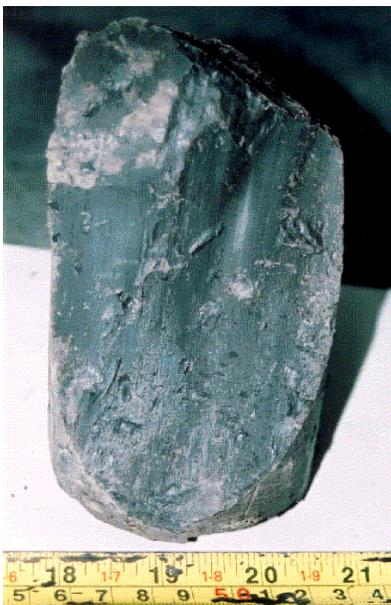
Figure 122. Discontinuity example: continuous, semi-undulose, striated, moderately shiny (7.6 cm [3 inch] diameter core sample).
