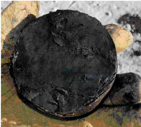
Figure 118. Discontinuity example: continuous, planar, slightly rough, dull. Scale indicated by gloved hand holding the 7.6 cm (3 inch) diameter core sample.
