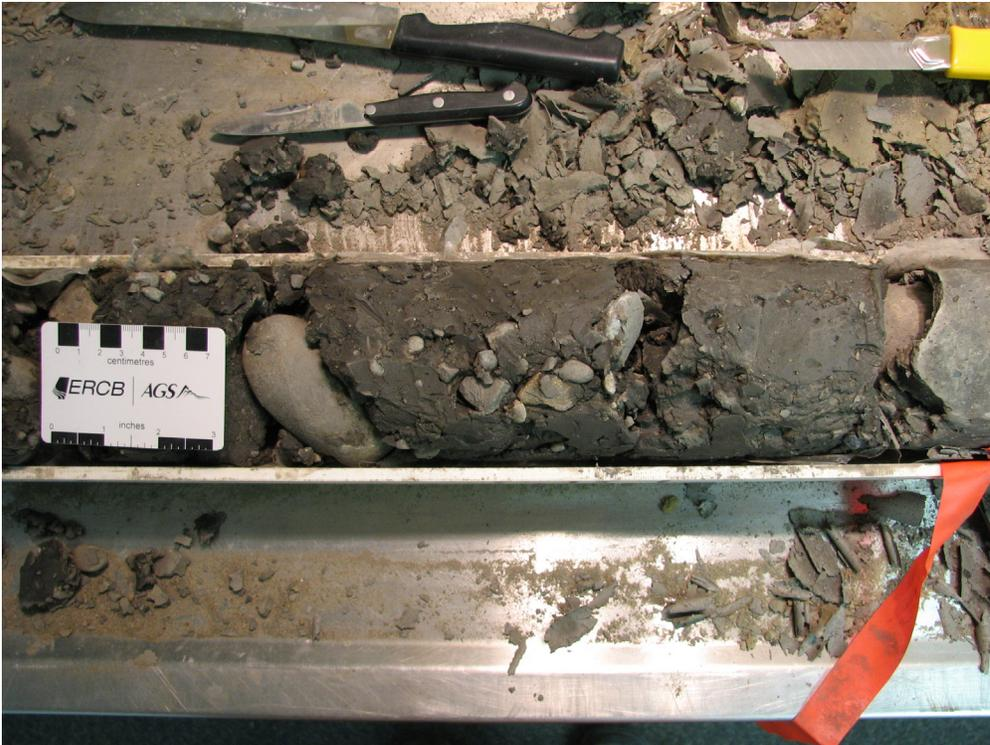
Figure 70. Clayey sandy silt to silty sand, stony diamicton; clast size ranges between small pebble and cobble grade (PR08-5; 54.2–54.9 m; 484.2–483.5 m asl).
