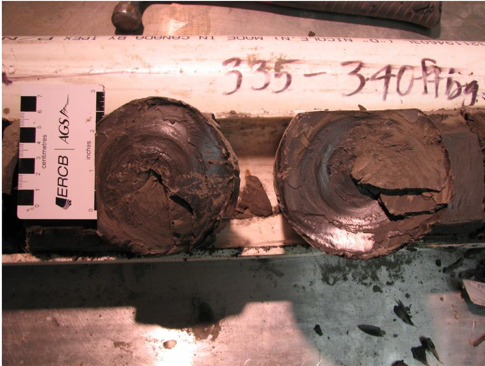
Figure 37. Slickensides parallel to bedding in silty clay to clayey silt (Note: slickensides appear to be drill induced), (PR08-3; 102.7–103.4 m; 342.6–341.9 m asl).
