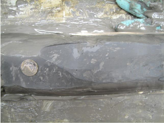
Figure 113. Silt and clay with very fine grained sand stringers and blebs (PR08-5; interclasts; 110–110.9 m; 428.4–427.5 m asl).
