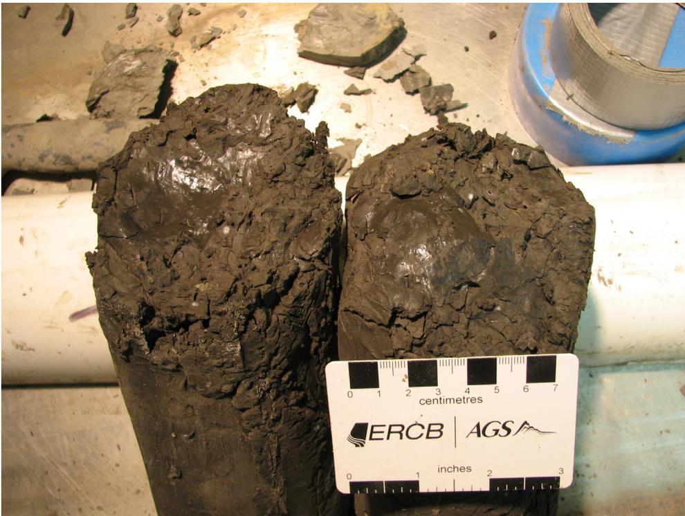
Figure 112. Slickensides in silty clay to clayey silt (PR08-5; 104.9–105.2 m; 433.5–433.2 m asl).
