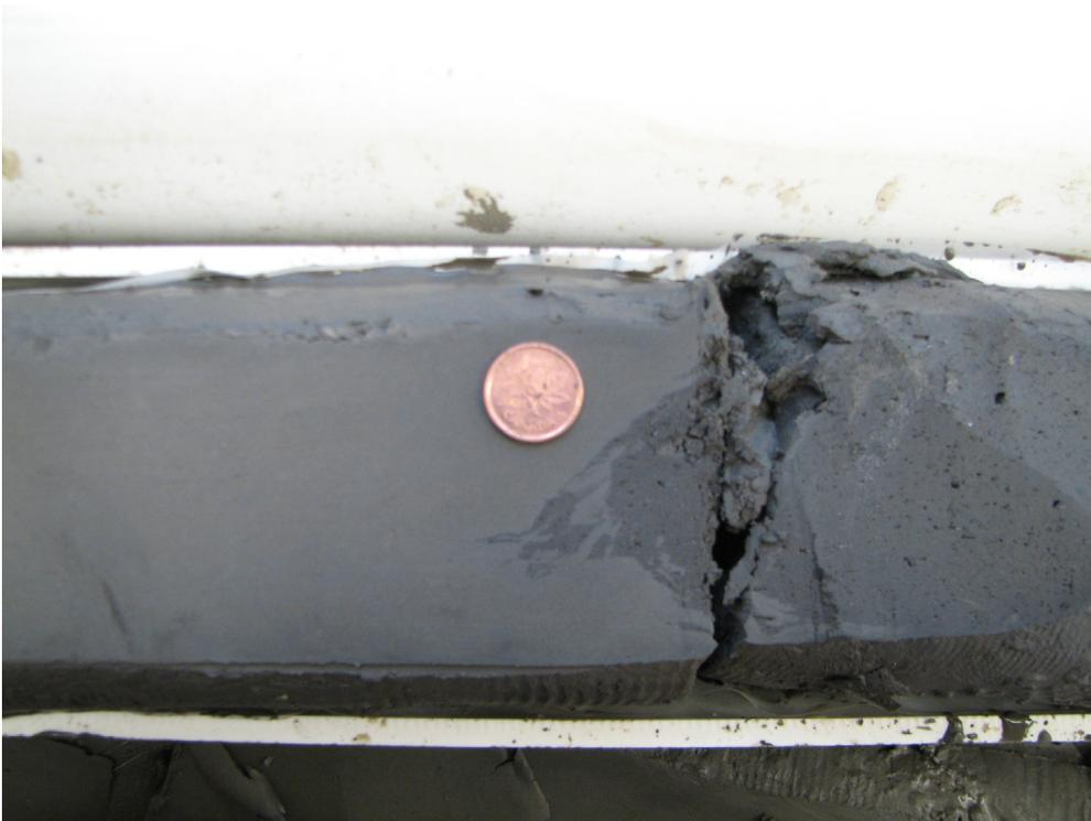
Figure 66. Contact between sandy silt and clayey sandy silt to silty sand, stony diamicton; note load structure immediately below coin (PR08-5; 50.3–50.8 m; 488.1–487.6 m asl).
