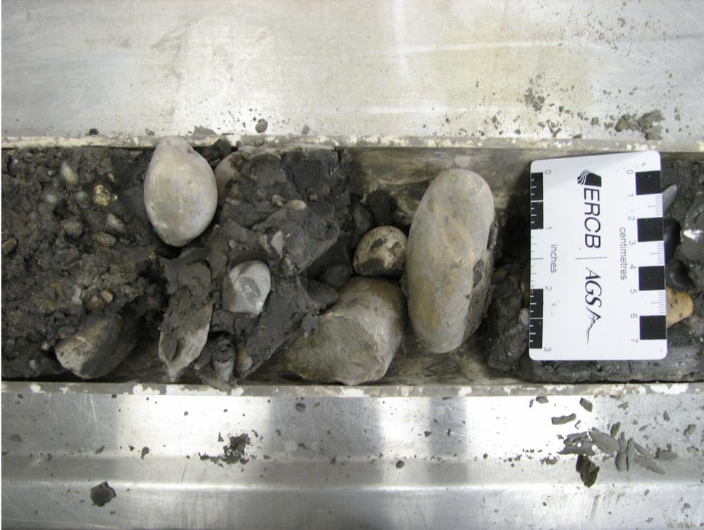
Figure 75. Clayey sandy silt to silty sand, stony diamicton; clast size ranges between small pebble and cobble grade; note cobble lag below scale card (PR08-5; 56.4–57.9 m; 482.4–481.9 m asl).
