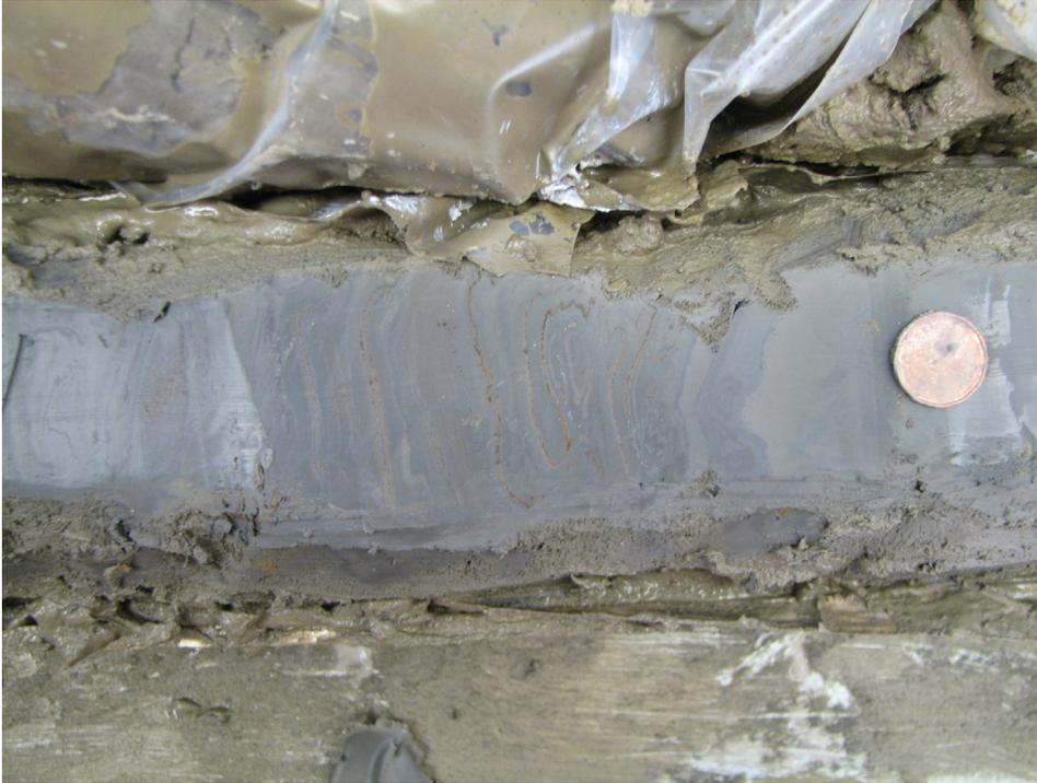
Figure 93. Rhythmically bedded deposits of clayey silt, silty clay and very fine to fine-grained sand; sample lost downhole and re-recovered (PR08-5; 90.8–91.4 m; 447.5–446.9 m asl).
