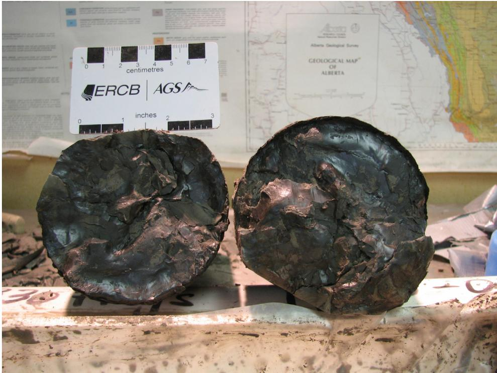
Figure 33. Rhythmically bedded deposits of very fine sandy silt and silty clay; slickensides noted in silty clay (PR08-3; 99.1–100.6 m; 346.2–344.7 m asl).
