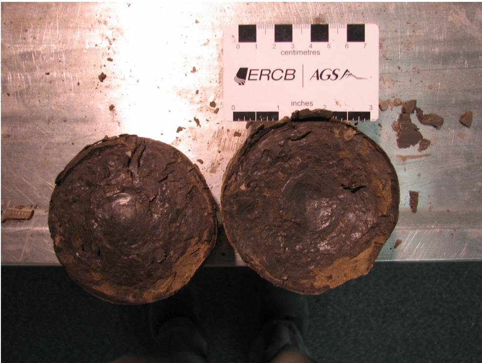
Figure 46. Slickensides within silt and clay rhythmite (Note: Slickensides appear to be drill-induced), (PR08-5; 9.1–10.6 m; 529.2–527.7 m asl).
