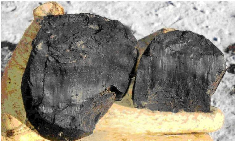
Figure 119. Discontinuity Example: Smooth, undulating, polished, continuous, intersecting. Scale indicated by gloved hand holding the 7.6 cm (3 inch) diameter core sample.
