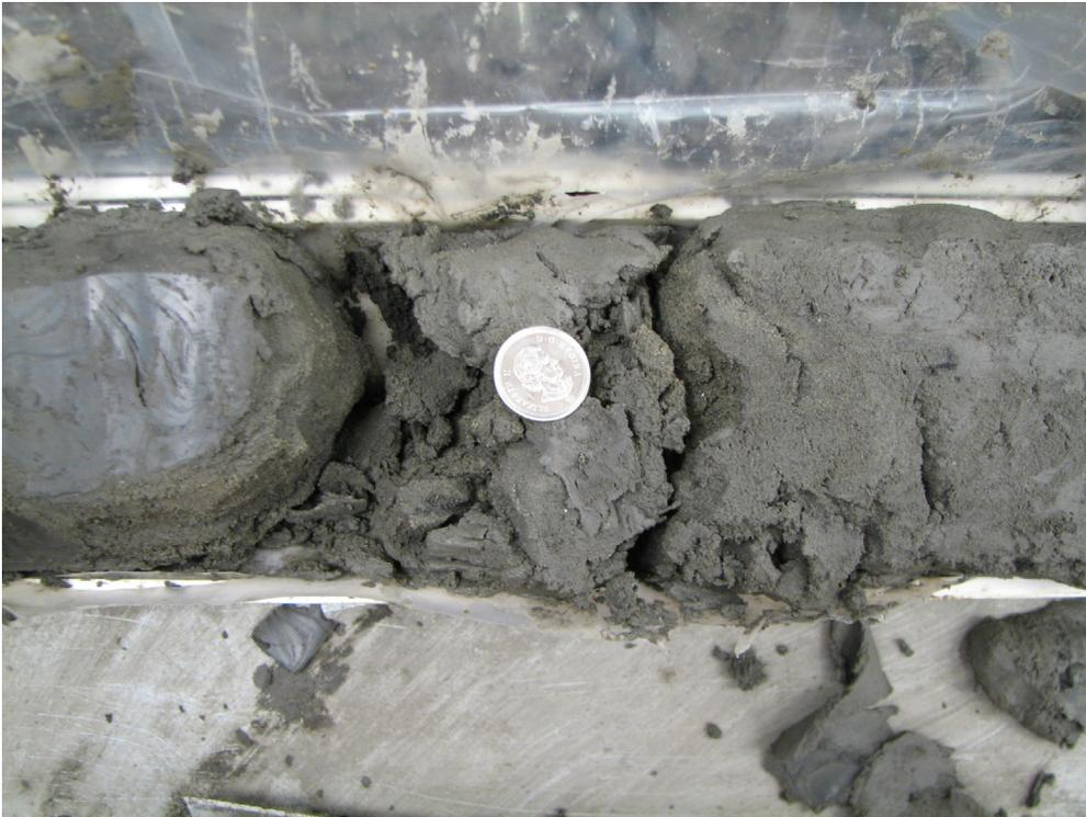
Figure 90. Clayey silt to silty clay interbedded with silty, fine- to medium-grained sand (PR08-5; 85.6–86.9 m; 452.7–451.5 m asl).
