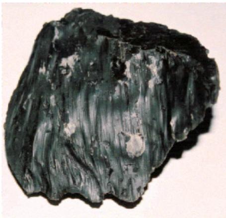
Figure 121. Discontinuity example: continuous, striated, slightly rough, intersecting (7.6 cm [3 inch] diameter core sample).
