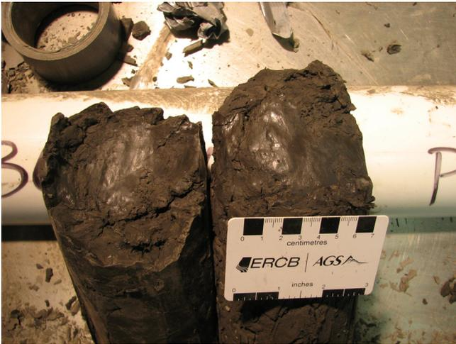
Figure 114. Slickensides in silt and clay (PR08-5; 110–110.9 m; 428.4–427.5 m asl).
