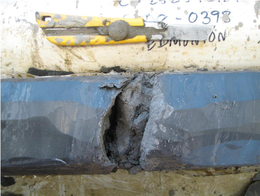
Figure 105. Clayey silt to silty clay interbedded with silty sand; note 2.5 cm thick bed of silty sand (PR08-5; 100.6–101.3 m; 437.8–437.1 m asl).
