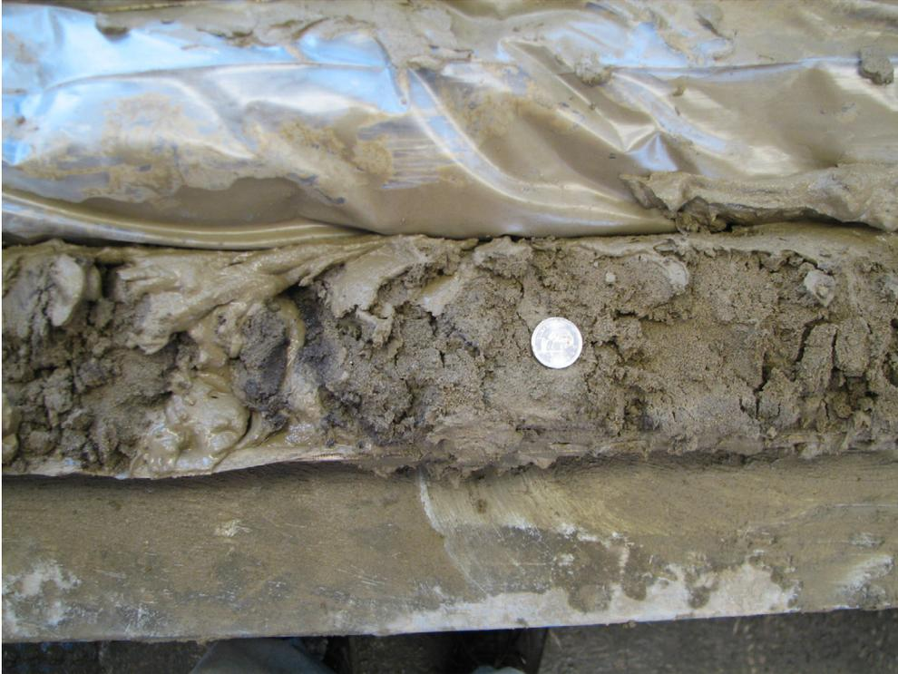
Figure 101. Medium-grained silty sand (PR08-5; 96–97.5 m; 442.3–440.8 m asl).
