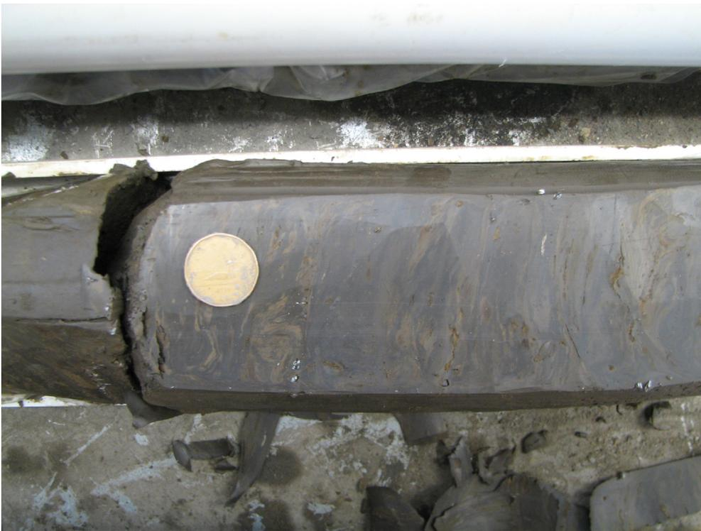
Figure 47. Deformed, rhythmically bedded deposits of silty clay to clayey silt (PR08-5; 12.3–14 m; 526.1–524.3 m asl).
