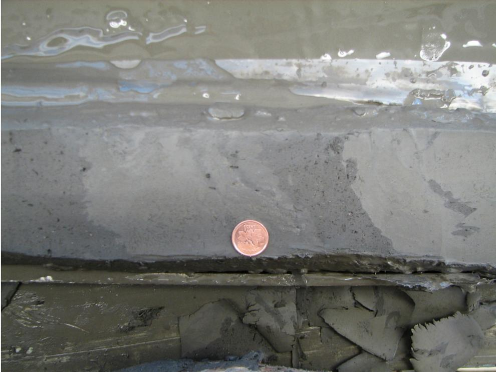
Figure 65. Beds of sandy silt and silty sand, blocks of dislocated clayey sandy silt to silty sand, stony diamicton (PR08-5; 48.8–50.3; 489.6–488.1 m asl).
