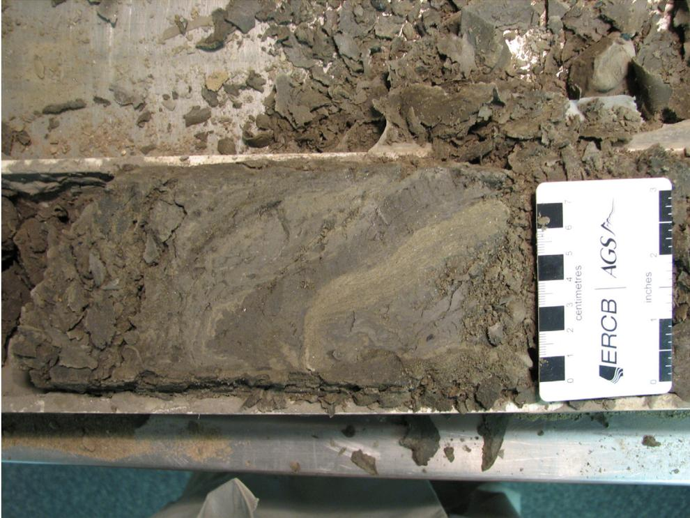
Figure 61. Beds of silty, very fine to fine-grained sand in clayey sandy silt to silty sand, stony diamicton (PR08-5; 44.2–45.7 m; 494.2–492.6 m asl).
