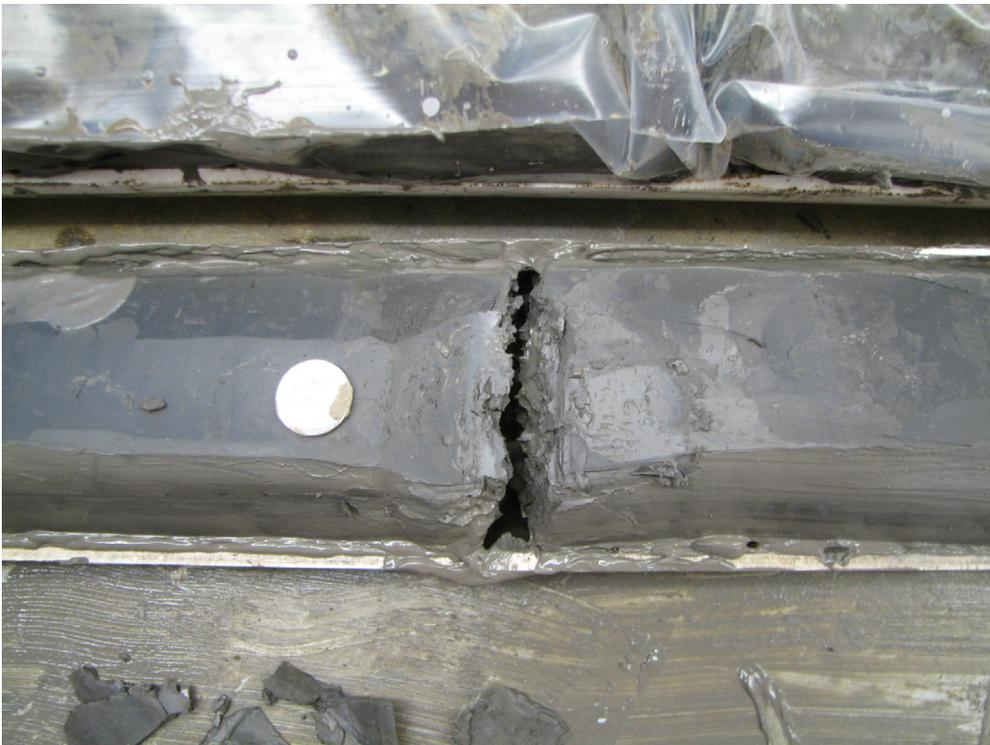
Figure 110. Silt-rich lens in clayey silt to silty clay (PR08-5; 104.3 m; 434.1 m asl).
