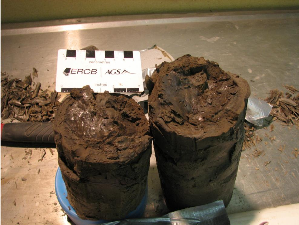
Figure 45. Slickensides within silt and clay rhythmites (Note: Slickensides appear to be drill-induced), (PR08-5; 7.6–9.1 m; 530.7–529.2 m asl).
