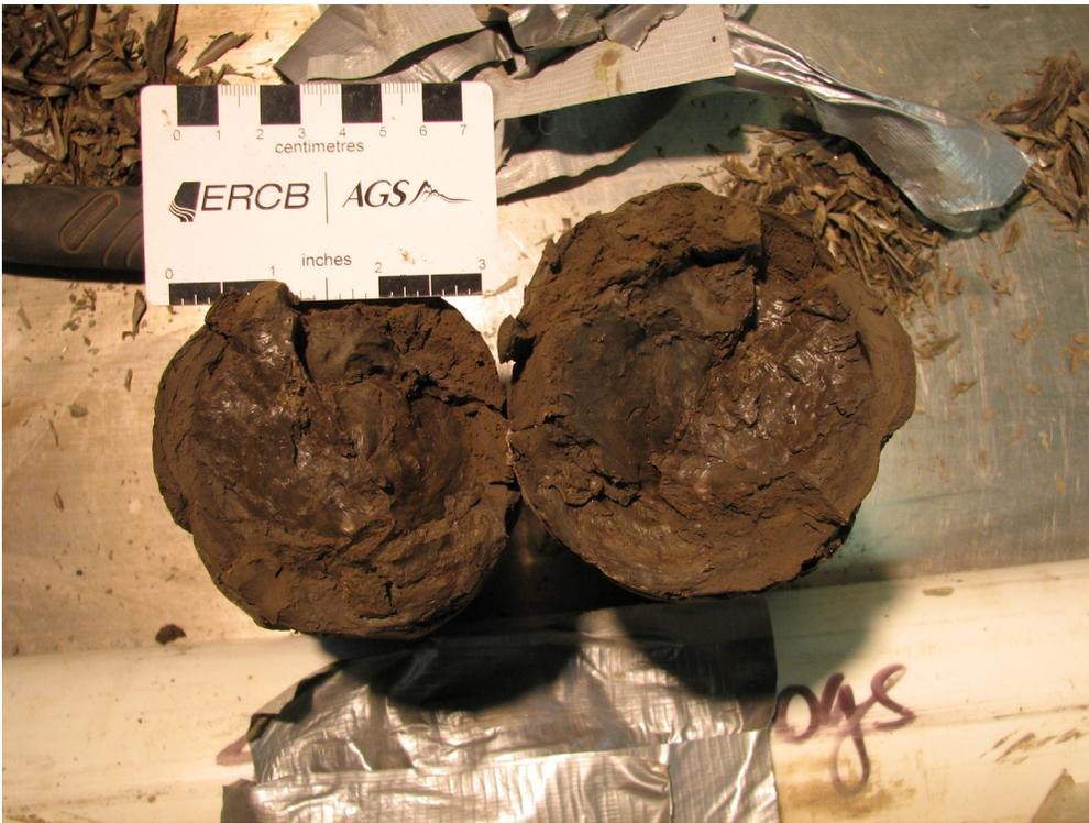
Figure 44. Slickensides within silt and clay rhythmities (Note: Slickensides appear to be drill-induced), (PR08-5; 7.6–9.1 m; 530.7–529.2 m asl).
