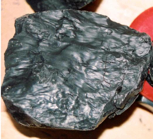
Figure 123. Discontinuity example: continuous, semi-undulose, very shiny, striated, intersecting (7.6 cm [3 inch] diameter core sample).
