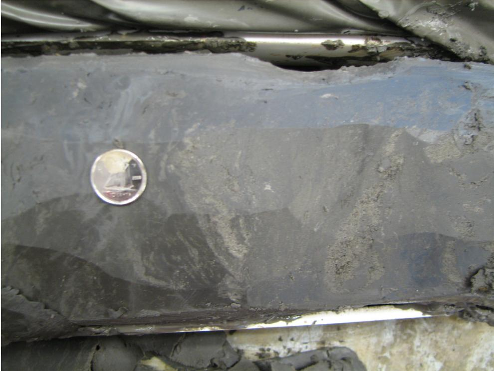
Figure 109. Clayey silt to silty clay, note wisps of silty, very fine sands (PR08-5; 102.1–103.6 m; 436.2–434.7 m asl).
