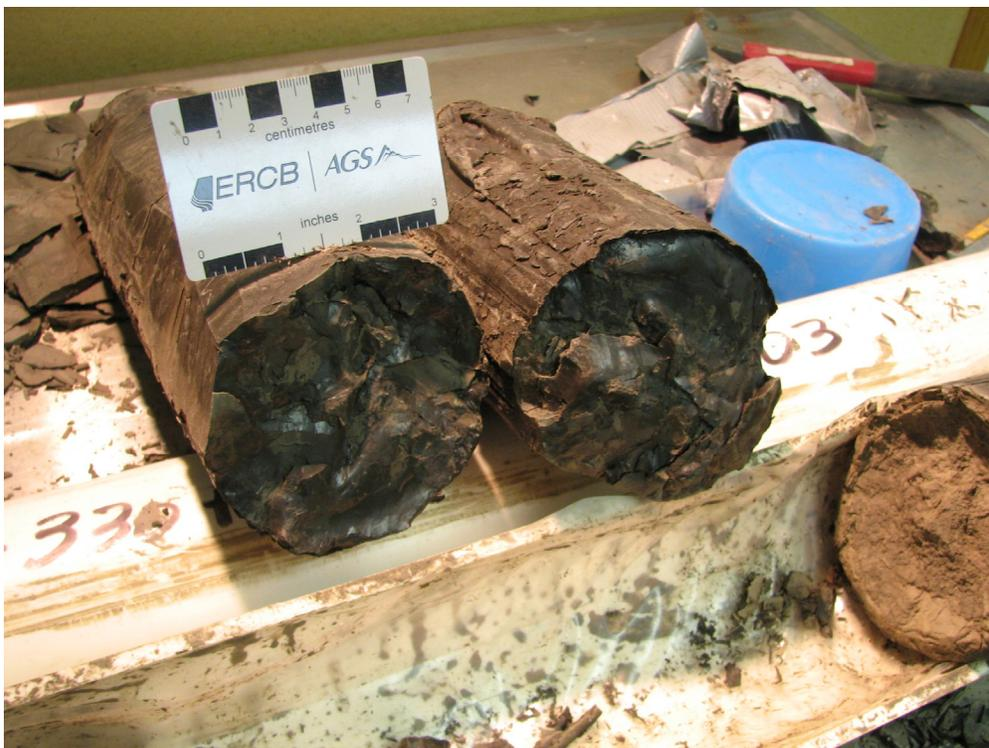
Figure 34. Rhythmically bedded deposits of very fine sandy silt and silty clay; slickensides noted in silty clay (PR08-3; 99.1–100.6 m; 346.2–344.7 m asl).
