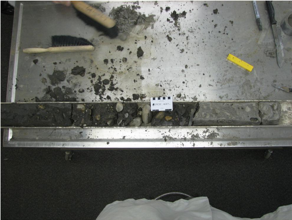
Figure 74. Clayey sandy silt to silty sand, stony diamicton; clast size ranges between small pebble and cobble grade; note cobble lag below scale card (PR08-5; 56.4–57.9 m; 482.4–481.9 m asl).
