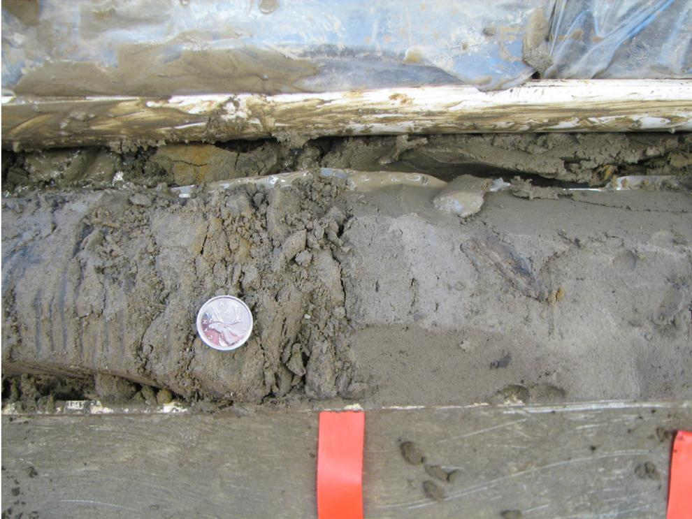
Figure 97. Fine- to medium-grained sand, discontinuous beds (laminae) of silty sand to sandy silt (PR08-5; 94.1–94.3 m; 444.2–444.1 m asl).
