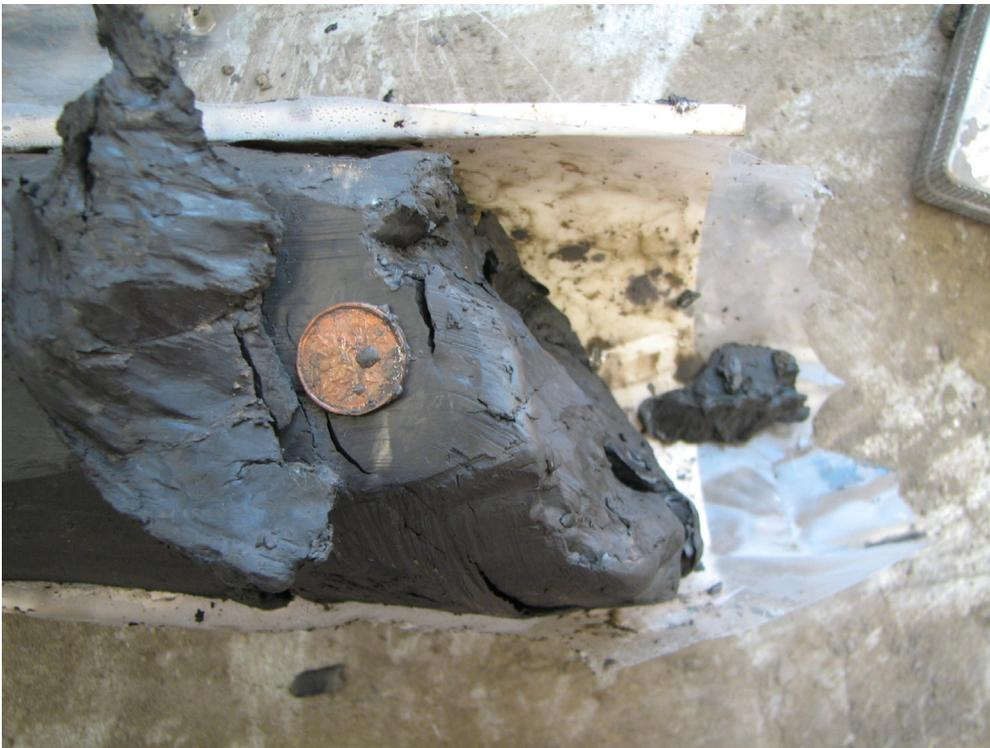
Figure 80. 45° slickenside in silty clay to clayey silt (PR08-5; 80.8 m; 457.6 m asl).
