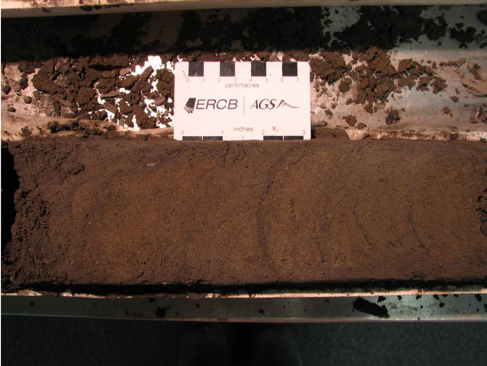
Figure 35. Planar-bedded, silty, fine- to medium-grained sand (PR08-3; 101.6–101.7 m; 343.7–343.6 m asl).
