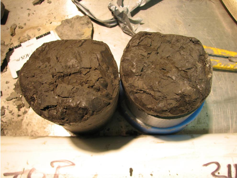
Figure 111. Slickensides in silty clay to clayey silt (PR08-5; 104.9–105.2 m; 433.5–433.2 m asl).
