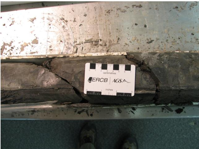
Figure 115. Slickensides in silt and clay (PR08-5; 110–110.9 m; 428.4–427.5 m asl).
