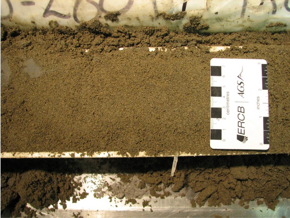
Figure 87. Medium- to coarse-grained silty sand with interclasts of clayey silt (PR08-5; 84.2–84.6 m; 454.2–453.8 m asl).
