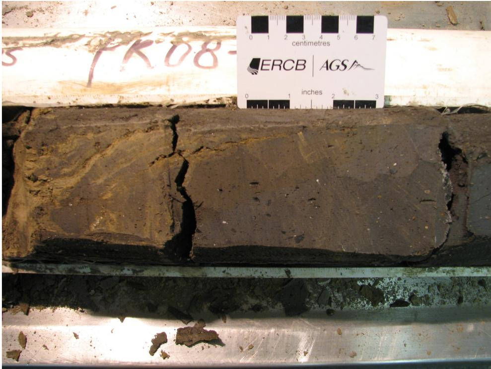
Figure 59. Fine- to medium-grained sand with interbeds of till; ripple drift in sand, contorted and overturned; contact with diamicton shown (PR08-5; 32.5–33.2 m; 505.8–505.1 m asl).
