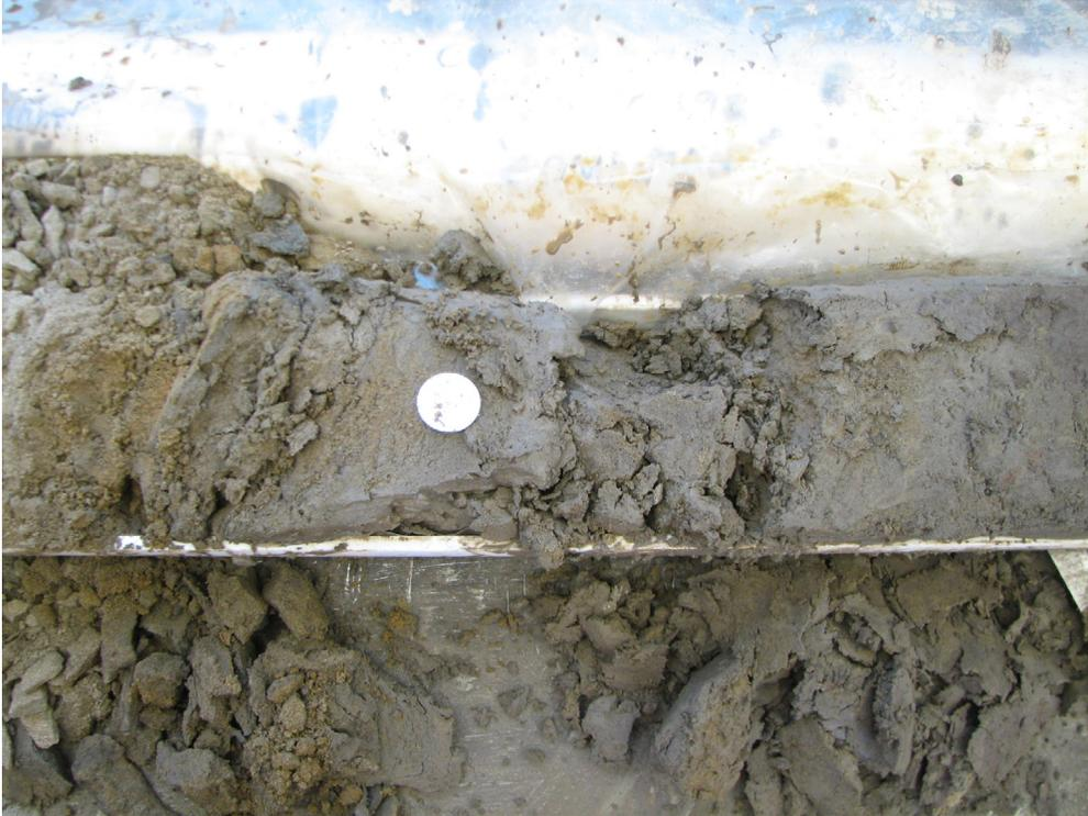
Figure 99. Very fine to fine-grained silty sand (PR08-5; 95.1–95.6 m; 443.2–442.8 m asl).
