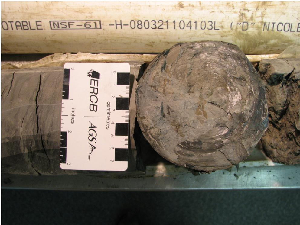
Figure 108. Clayey silt to silty clay, wisps of silty, very fine sand throughout; slickensides in clay (Note: Slickensides appear to be drill-induced), (PR08-5; 101.3–102.1 m; 437.1–436.2 m asl).
