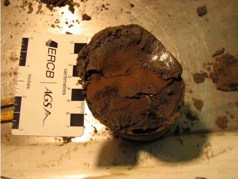
Figure 95. Rhythmically bedded deposits of clayey silt, silty clay and very fine to fine-grained sand; slickensides in clay-rich sediments; sample lost downhole and re-recovered (PR08-5; 90.8–91.4 m; 447.5–446.9 m asl).
