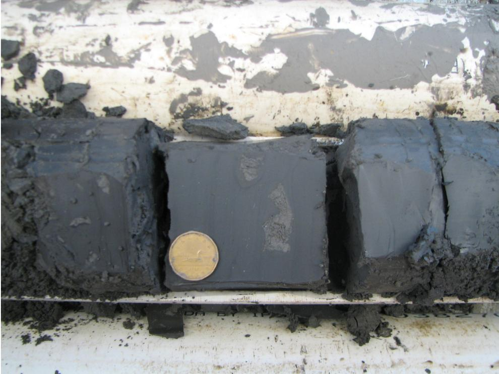
Figure 41. Rhythmically bedded deposits of silty clay to clayey silt; note silt-rich interclasts adjacent to coin (PR08-3; 105.3–106.7 m; 340–338.6 m asl).
