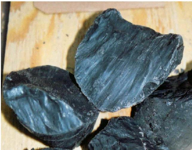
Figure 124. Discontinuity example: continuous, semi-undulose, striated, polished, intersecting (7.6 cm [3 inch] diameter core sample).
