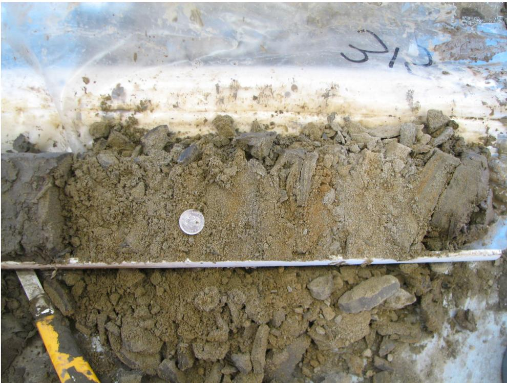
Figure 100. Medium- to coarse-grained sand with interbeds of silt (PR08-5; 95.6–96 m; 442.8–442.3 m asl).
