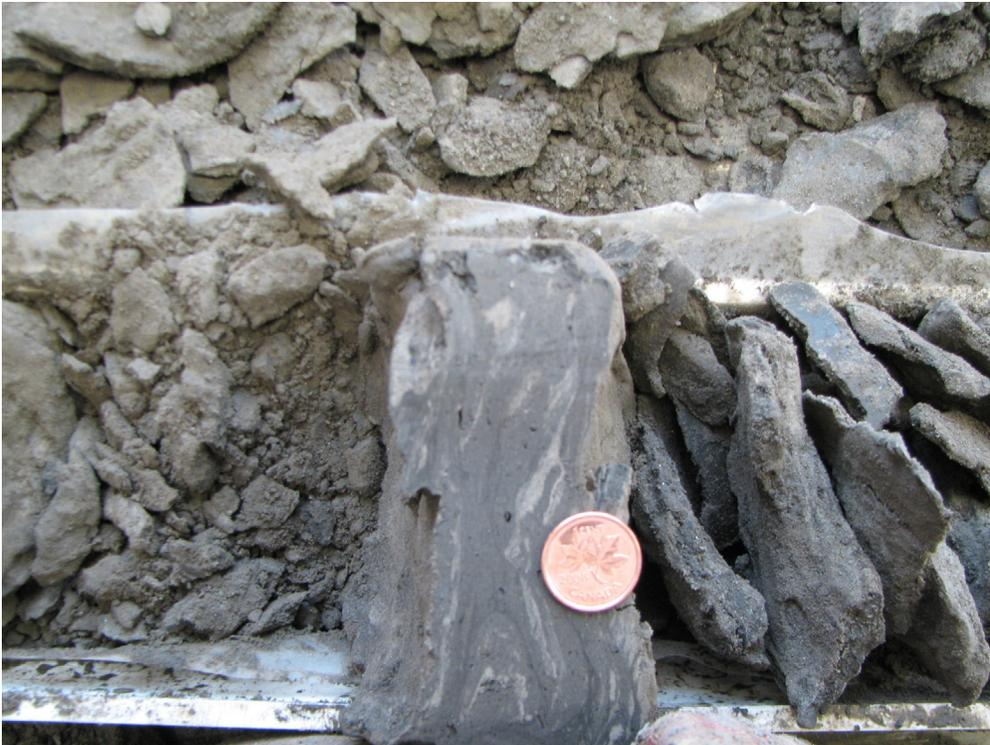
Figure 62. Planar bedded deposits of silty fine sand and silt (PR08-5; 45.7–46.3 m; 492.6–492 m asl).
