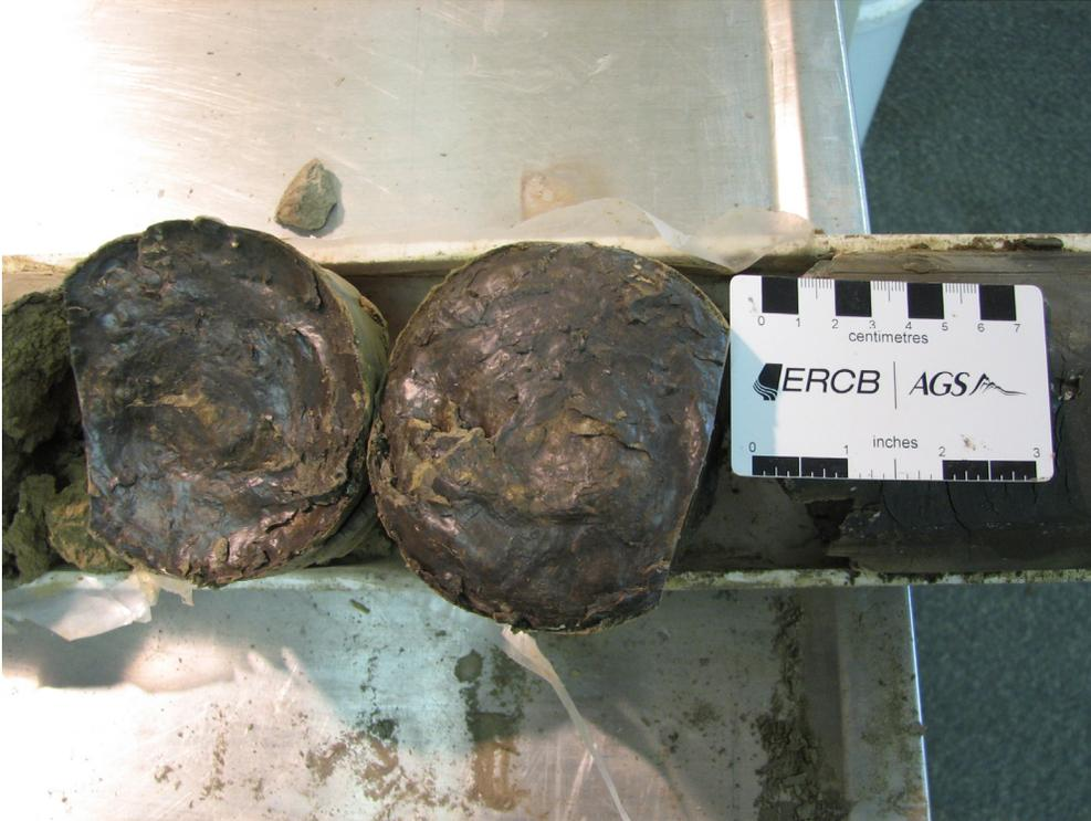
Figure 51. Slickenside in silty clay (Note: Slickensides appear to be drill-induced), (PR08-5; 14–15.2 m; 524.3–523.1 m asl).
