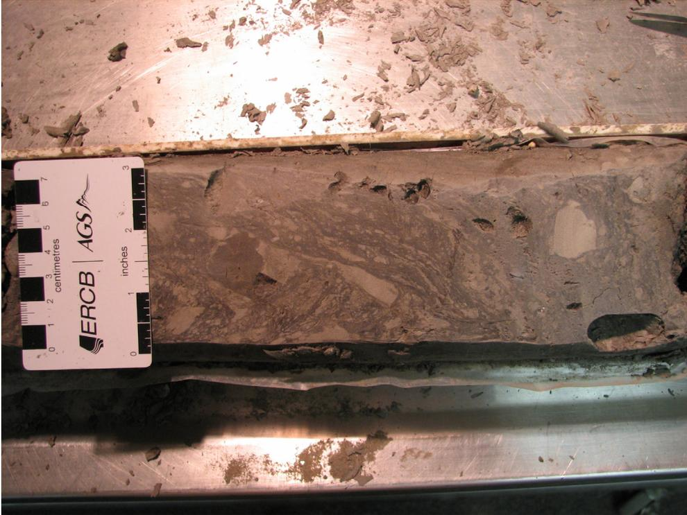
Figure 77. Clayey sandy silt to silty sand, stony diamicton; note interclasts of silty sand to sandy silt (PR08-5; 56.4–57.9 m; 482.4–481.9 m asl).
