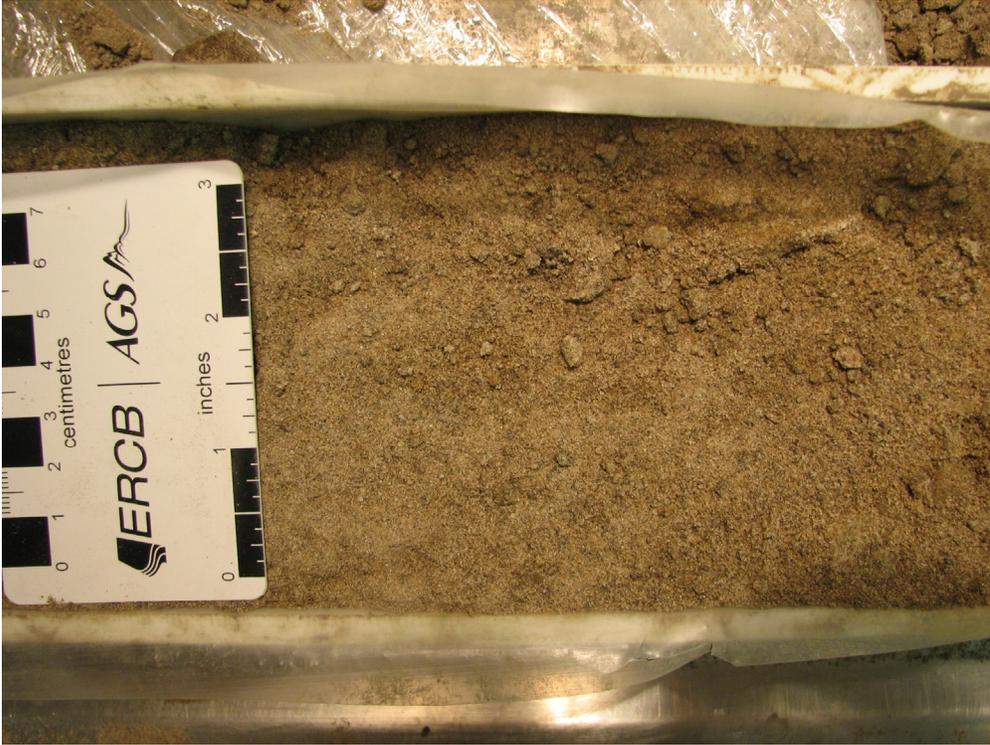
Figure 53. Fine- to medium-grained sand (PR08-5; 18.3–19.5 m; 520.1–518.8 m asl).
