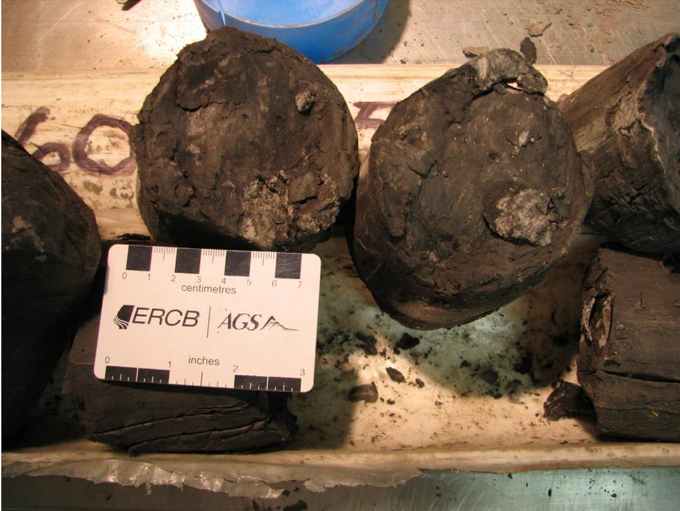
Figure 81. Slickensides in silty clay to clayey silt (Note: Slickensides appear to be drill-induced), (PR08-5; 79.2–80.8 m; 459.1–457.6 m asl).
