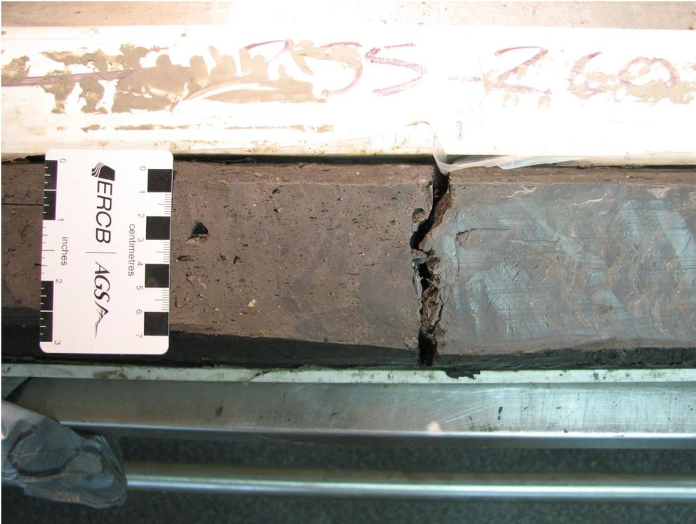
Figure 78. Erosive contact between clayey sandy silt to silty sand, stony diamicton and underlying silt and clay (PR08-5; 77.7–78.7 m; 460.6–459.7 m asl).
