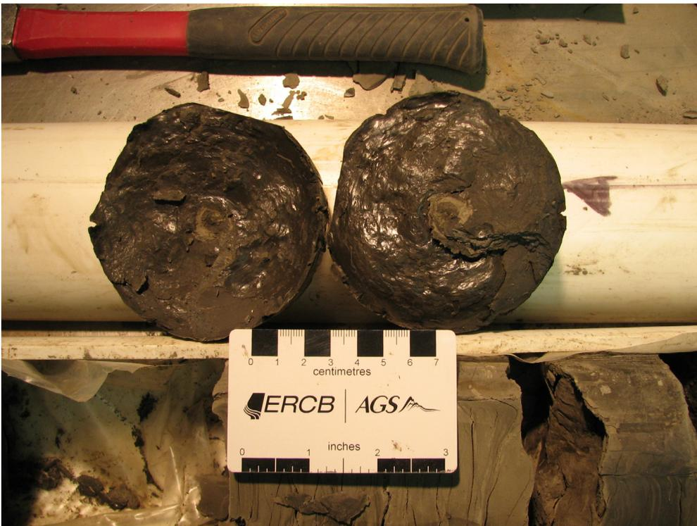
Figure 42. Slickensides parallel to bedding in rhythmically bedded deposits of silty clay to clayey silt (Note: slickensides appear to be drill-induced), (PR08-3; 105.3–106.7 m; 340–338.6 m asl).
