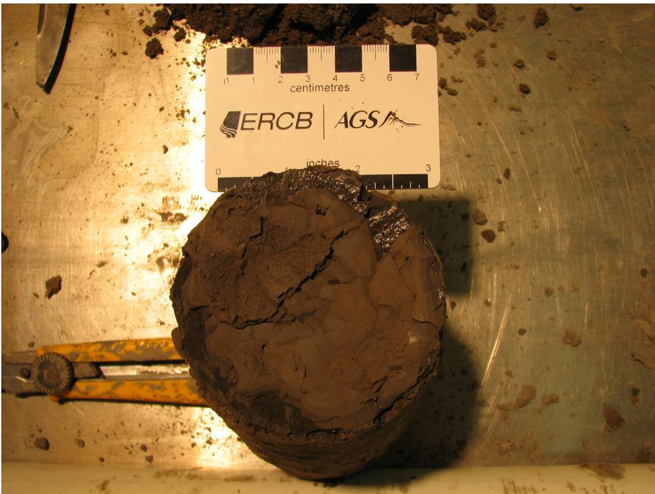
Figure 94. Rhythmically bedded deposits of clayey silt, silty clay and very fine to fine-grained sand; slickensides in clay-rich sediments; sample lost downhole and re-recovered (PR08-5; 90.8–91.4 m; 447.5–446.9 m asl).
