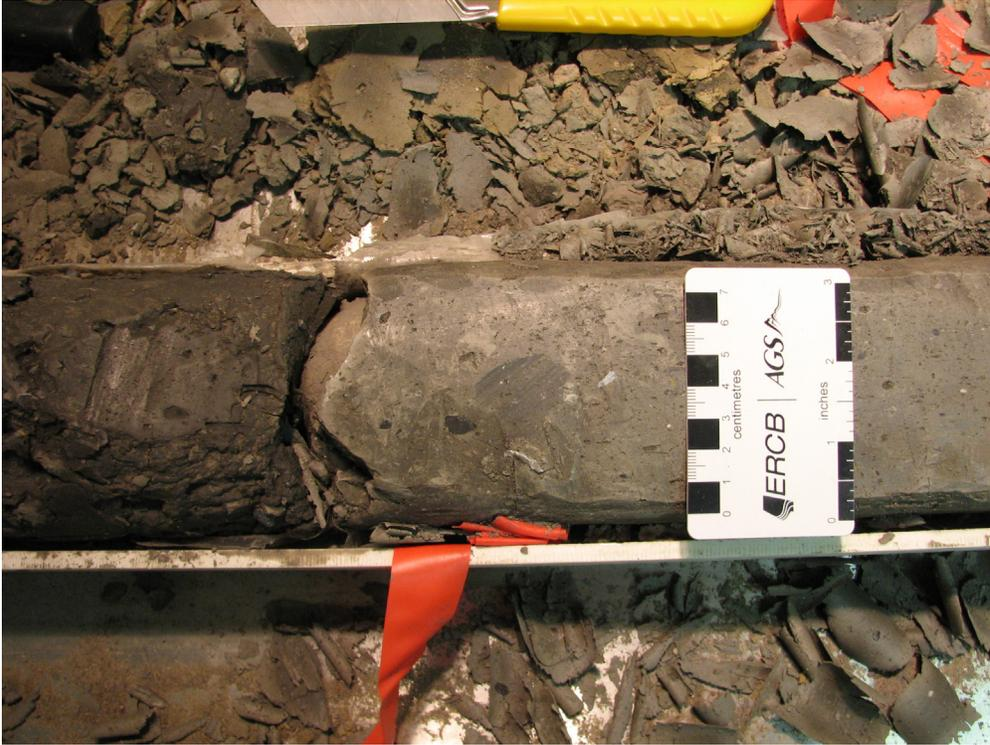
Figure 71. Clayey sandy silt to silty sand, stony diamict; clast size ranges between small pebble and cobble grade (PR08-5; 54.2–54.9 m; 484.2–483.5 m asl).
