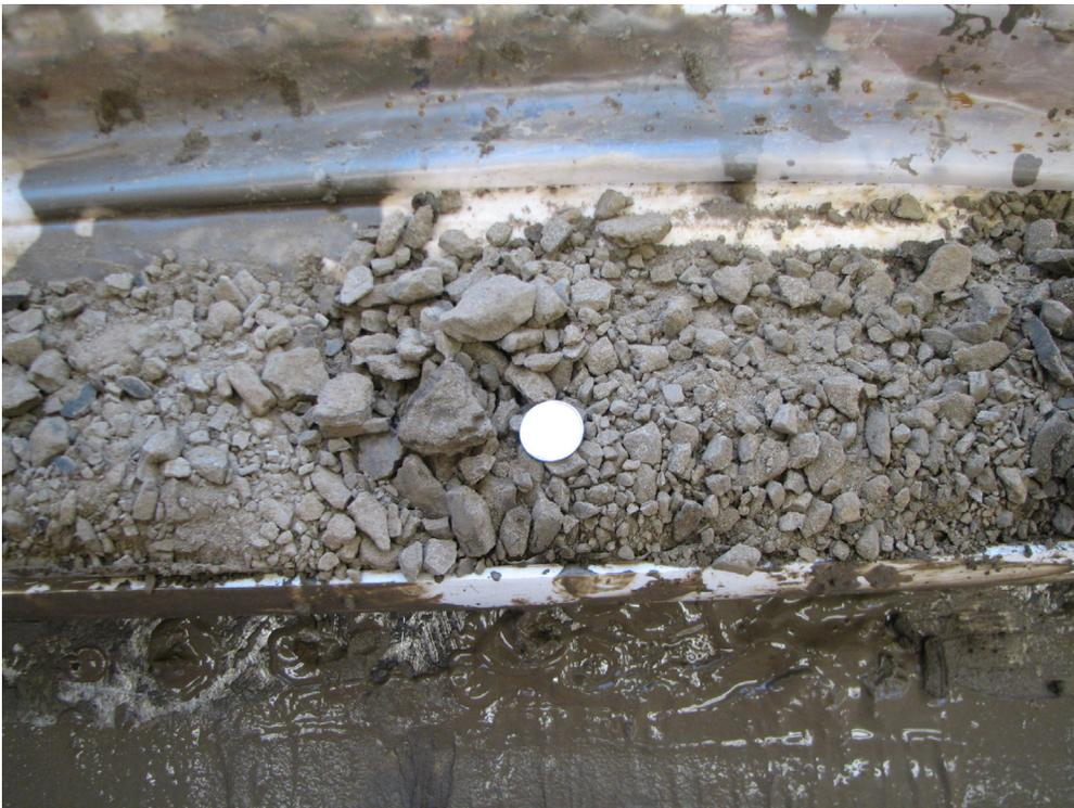
Figure 98. Fine- to medium-grained sand with silty interbeds, weakly cemented and fractured (PR08-5; 94.5–95.1 m; 443.9–443.2 m asl).
