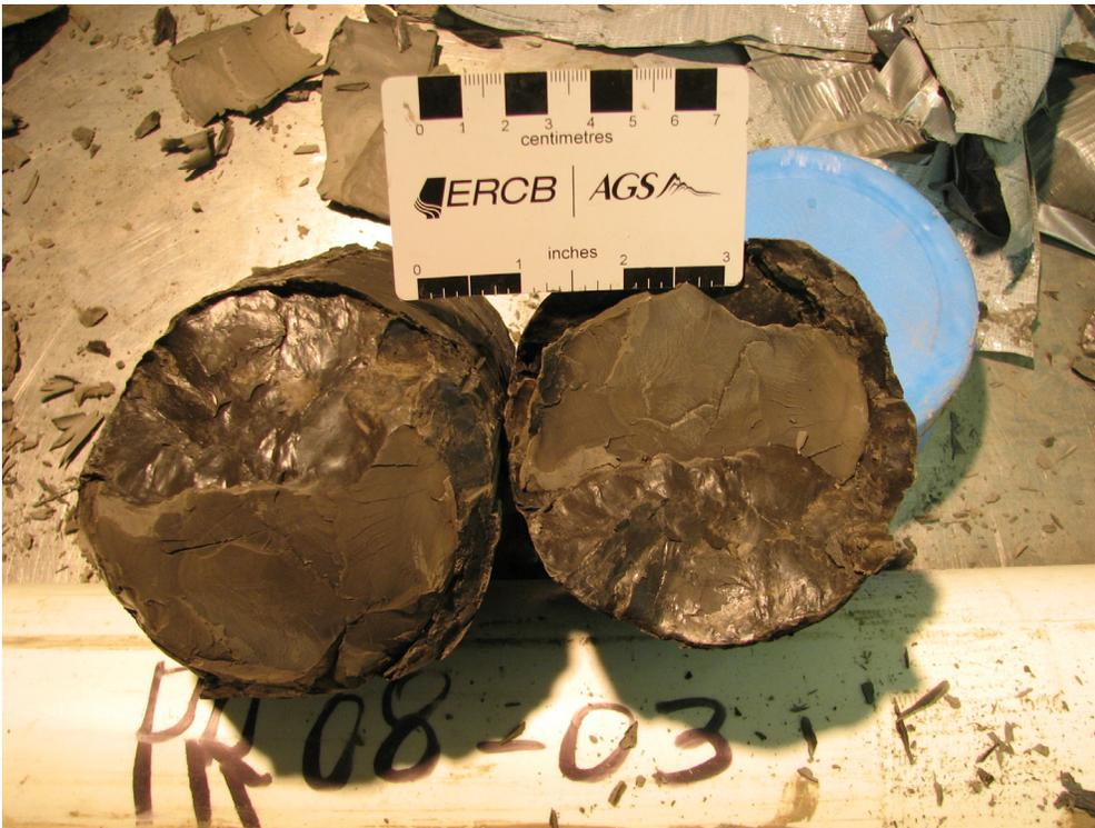
Figure 32. Rhythmically bedded deposits of very fine sandy silt and silty clay; slickensides noted in silty clay (PR08-3; 99.1–100.6 m; 346.2–344.7 m asl).
