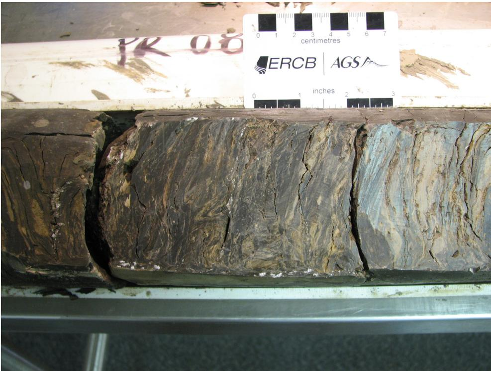
Figure 48. Deformed, rhythmically bedded deposits of silty clay to clayey silt (PR08-5; 12.3–14 m; 526.1–524.3 m asl).
