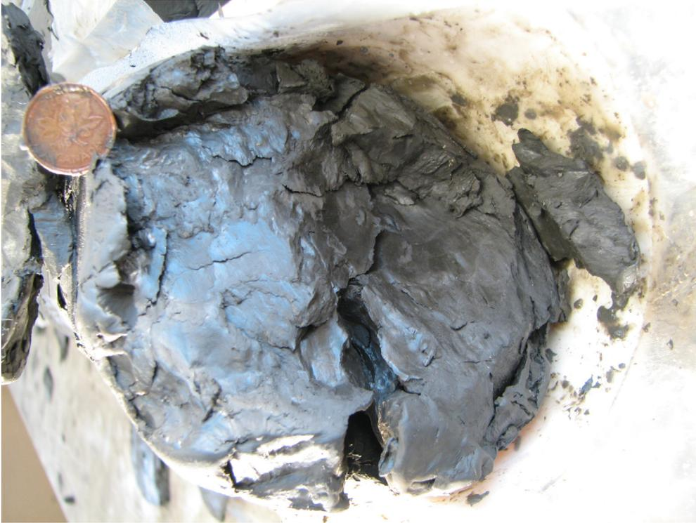
Figure 79. 45° slickenside in silty clay to clayey silt (PR08-5; 80.8 m; 457.6 m asl).
