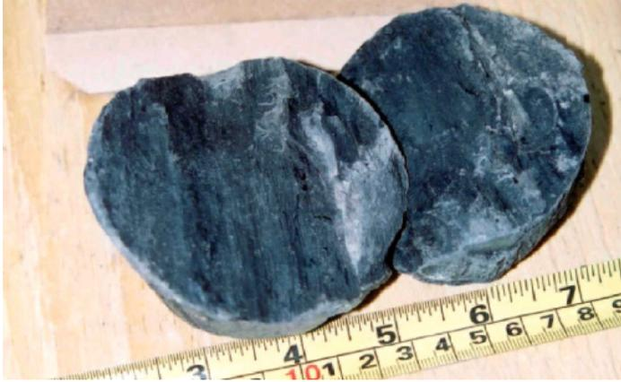
Figure 120. Discontinuity example: continuous, curved, striated, polished.
