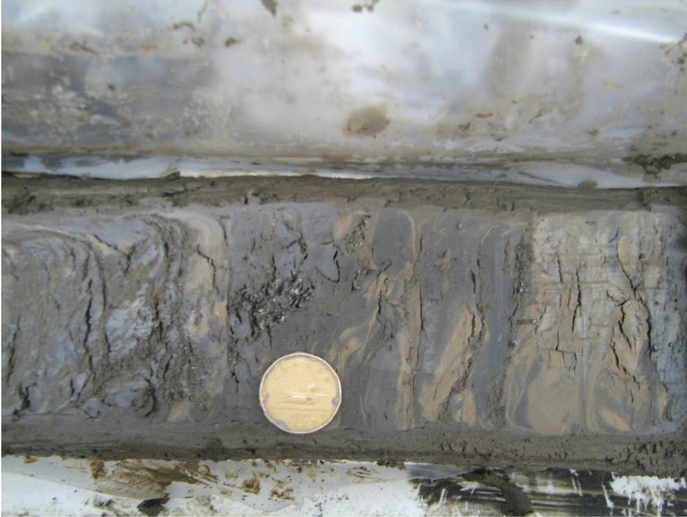
Figure 43. Rhythmically bedded deposits of silt and clay (PR08-5; 1.5–4.6 m; 536.8–535.3 m asl).
