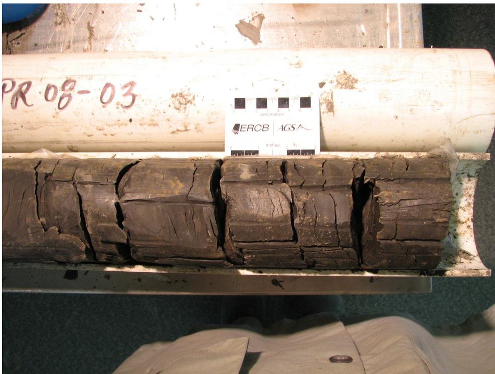
Figure 40. Slickensides parallel to bedding in rhythmically bedded deposits of silty clay to clayey silt (Note: slickensides appear to be drill-induced), (PR08-3; 103.6–105.2 m; 341.7–340.1 m asl).
