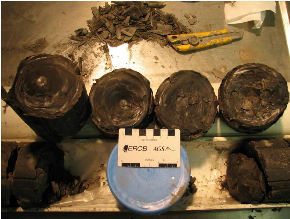
Figure 38. Slickensides parallel to bedding in silty clay to clayey silt (Note: slickensides appear to be drill-induced), (PR08-3; 103.6–105.2 m; 341.7–340.1 m asl).
