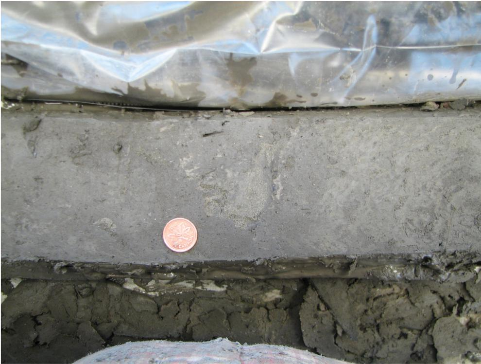
Figure 64. Contorted beds of sandy silt and silty sand (PR08-5; 47.2–48.8 m; 491.1–489.6 m asl).
