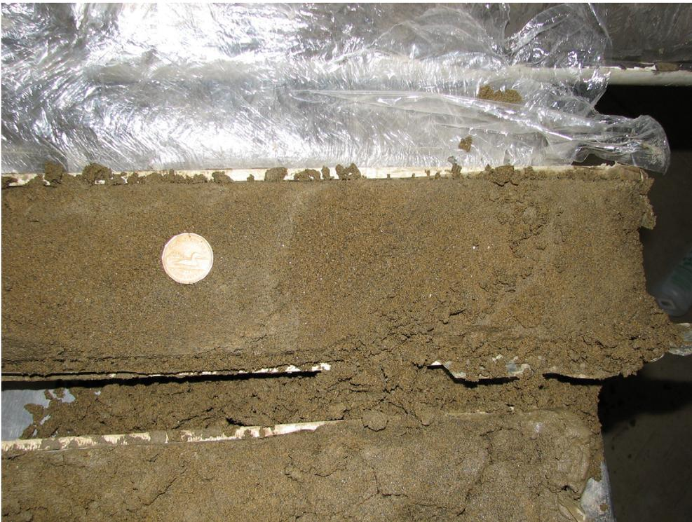
Figure 92. Medium- to coarse-grained sand (PR08-5; 88.4–89.9 m; 450–448.4 m asl).
