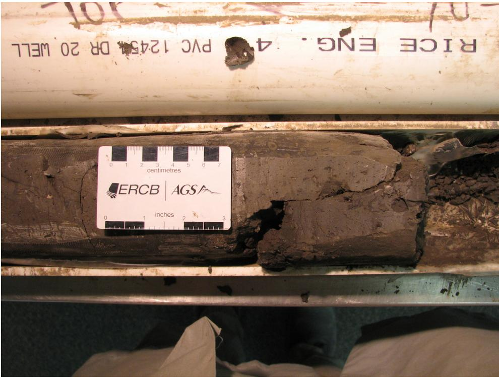
Figure 54. Fractures (jointing?) in silt-rich diamicton (PR08-5; 21.3–22.9 m; 517–515.5 m asl).
