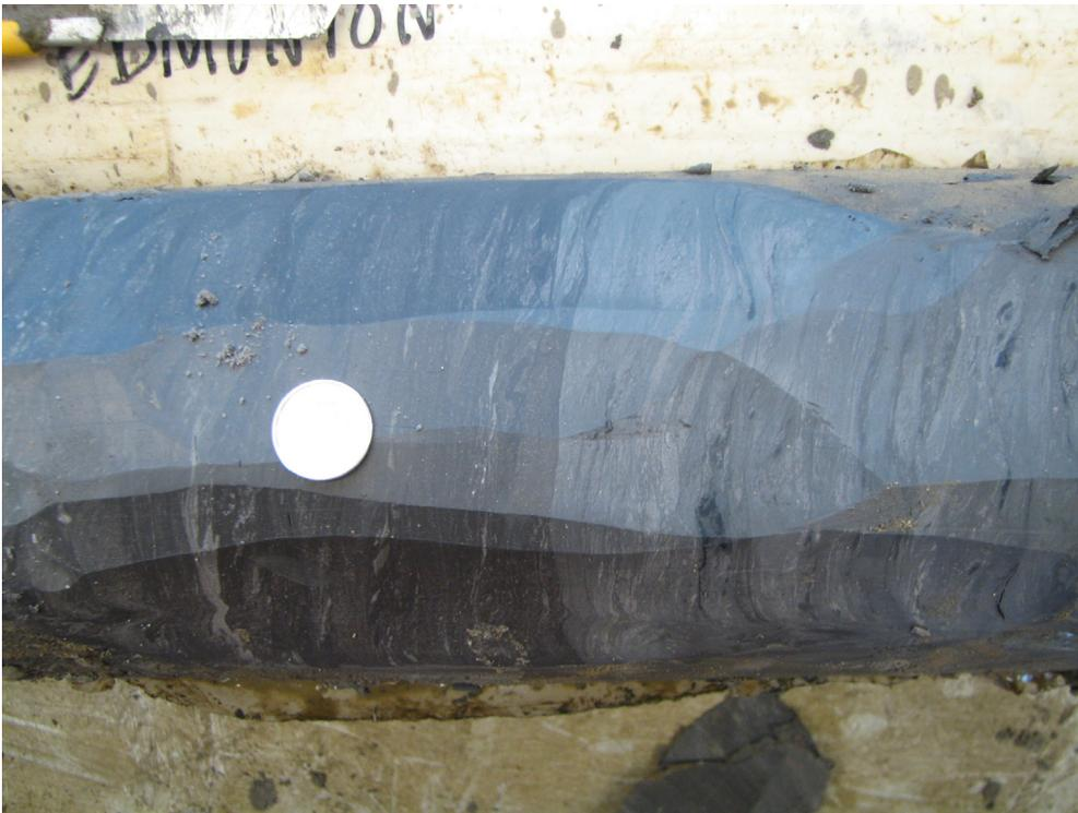
Figure 106. Clayey silt to silty clay, wisps of silty, very fine sands throughout (PR08-5; 101.3–102.1 m; 437.1–436.2 m asl).
