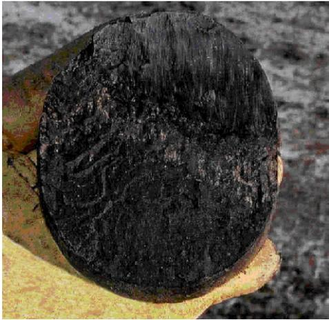
Figure 117. Discontinuity example: continuous, planar, moderately shiny, striated. Scale indicated by gloved hand holding the 7.6 cm (3 inch) diameter core sample.
