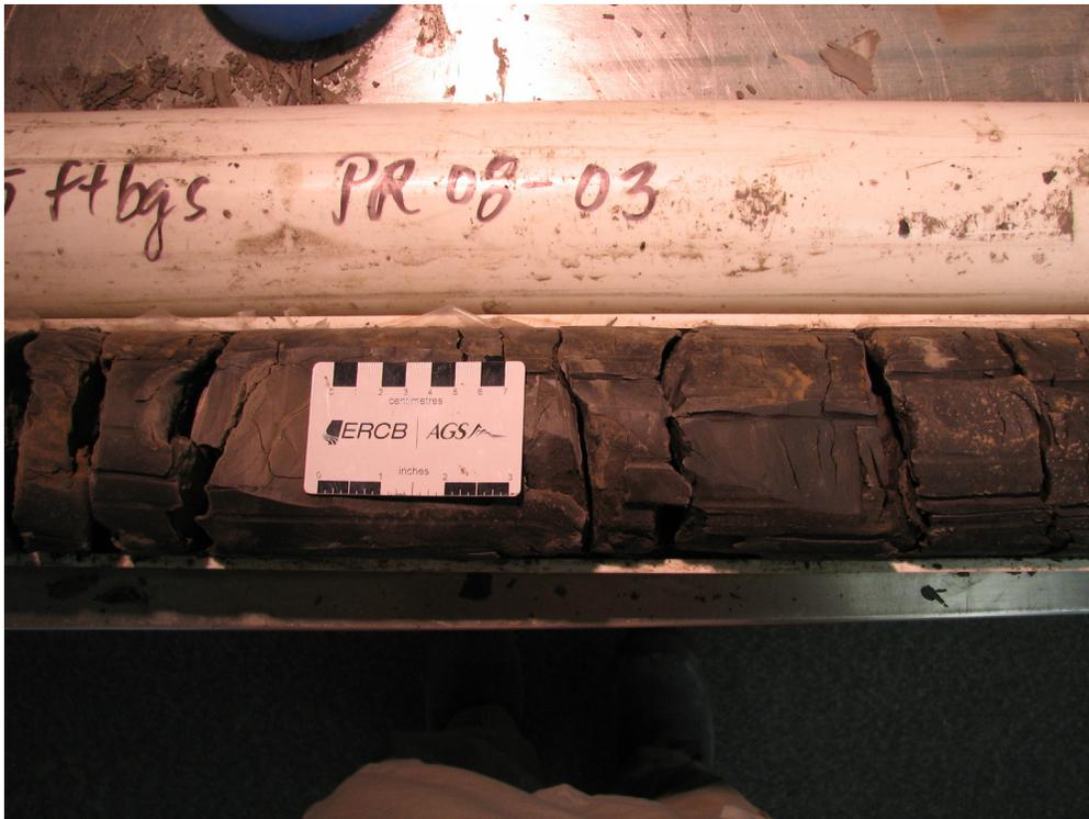
Figure 39. Slickensides parallel to bedding in rhythmically bedded deposits of silty clay to clayey silt (Note: slickensides appear to be drill-induced), (PR08-3; 103.6–105.2 m; 341.7–340.1 m asl).
