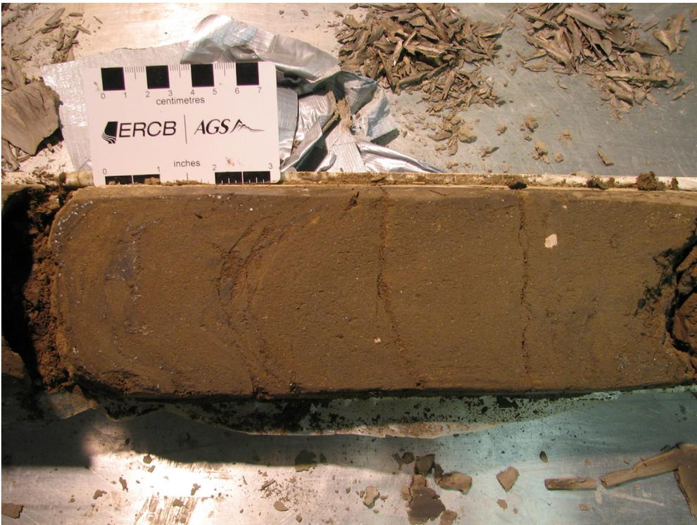
Figure 50. Silty sand with interbeds of silty clay (PR08-5; 14–15.2 m; 524.3–523.1 m asl).
