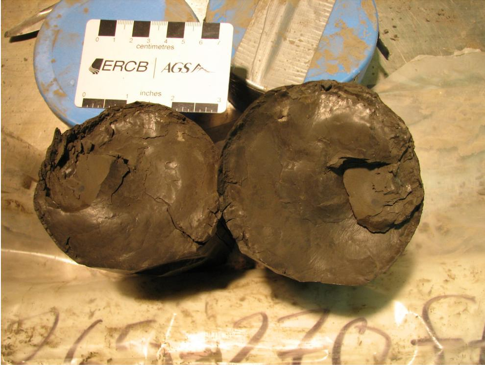
Figure 83. Slickensides within clayey silt to silty clay (Note: Slickensides appear to be drill-induced), (PR08-5; 80.8–82.3 m; 457.6–456.1 m asl).
