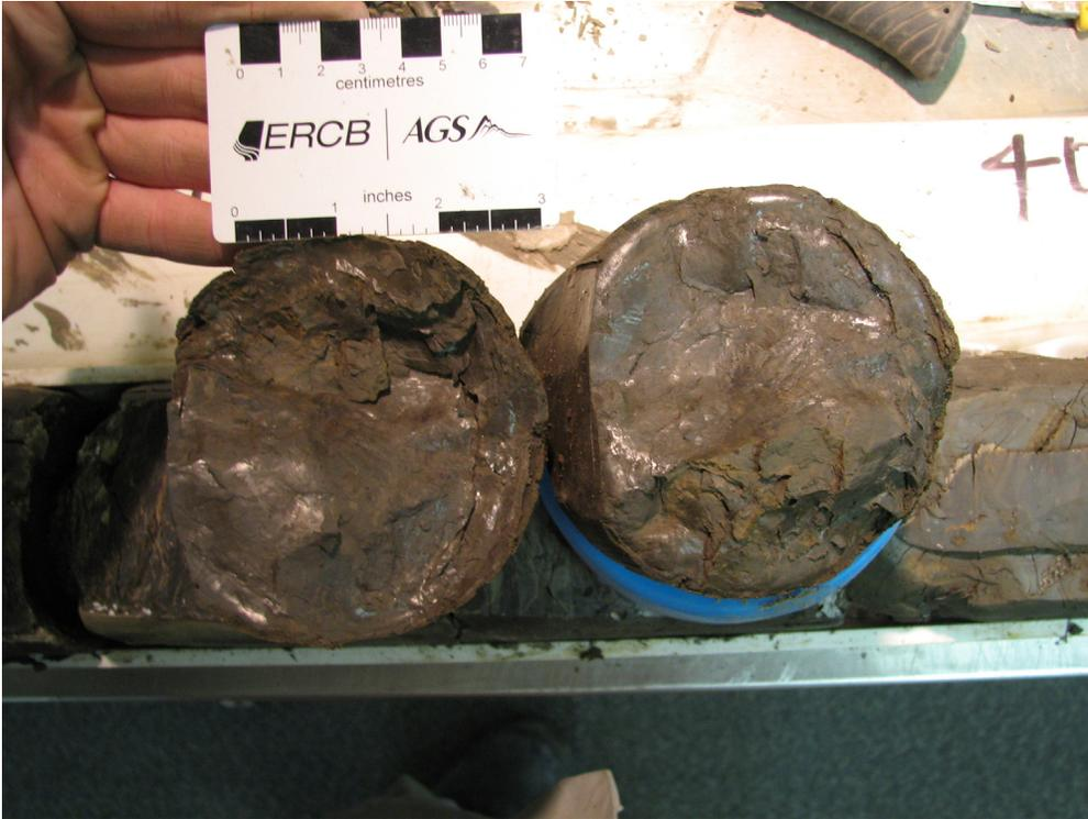
Figure 49. Slickenside in slit and clay rhythmite (PR08-5; 12.3–14 m; 526.1–524.3 m asl).
