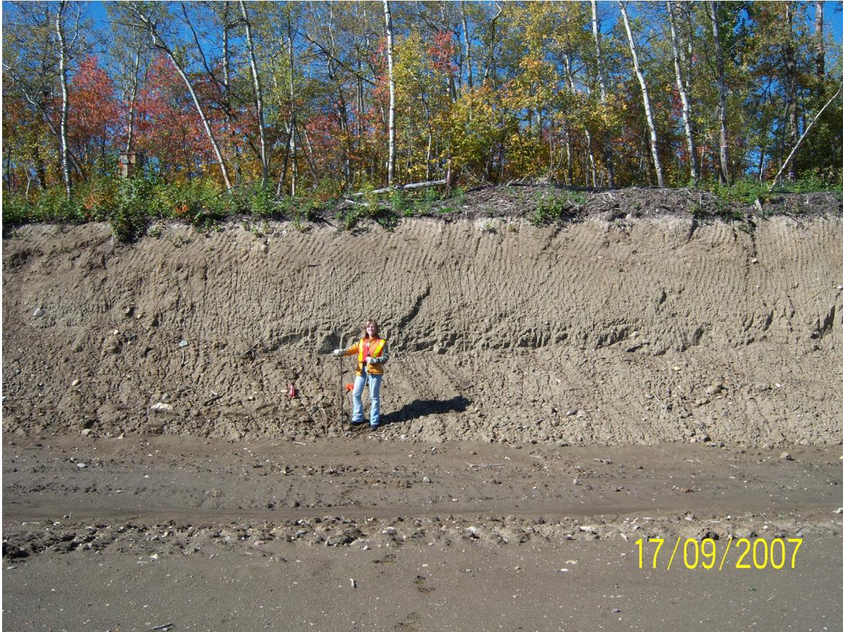
**Figure 4. Surficial-material sample site TC-07-4 (Appendix 1) provided an unweathered till sample from a depth of 4.5–4.75 m.**
