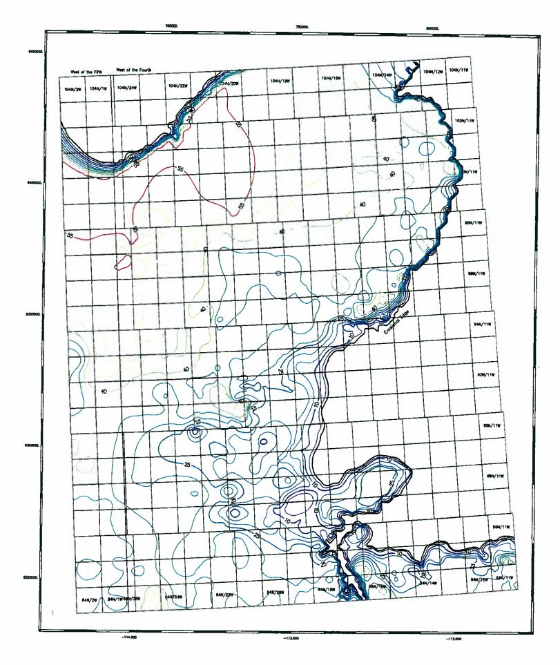
Figure 14. Lower Stratigraphic Interval, Pelican Formation to Base Fish Scales isopach
