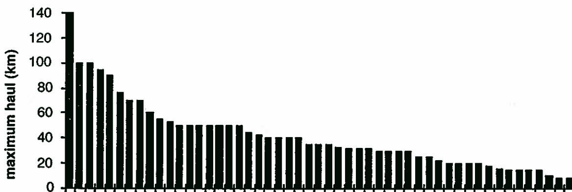
Figure 5. Maximum haul distance (km.) for sand or gravel for each of 51 regional municipalities.
