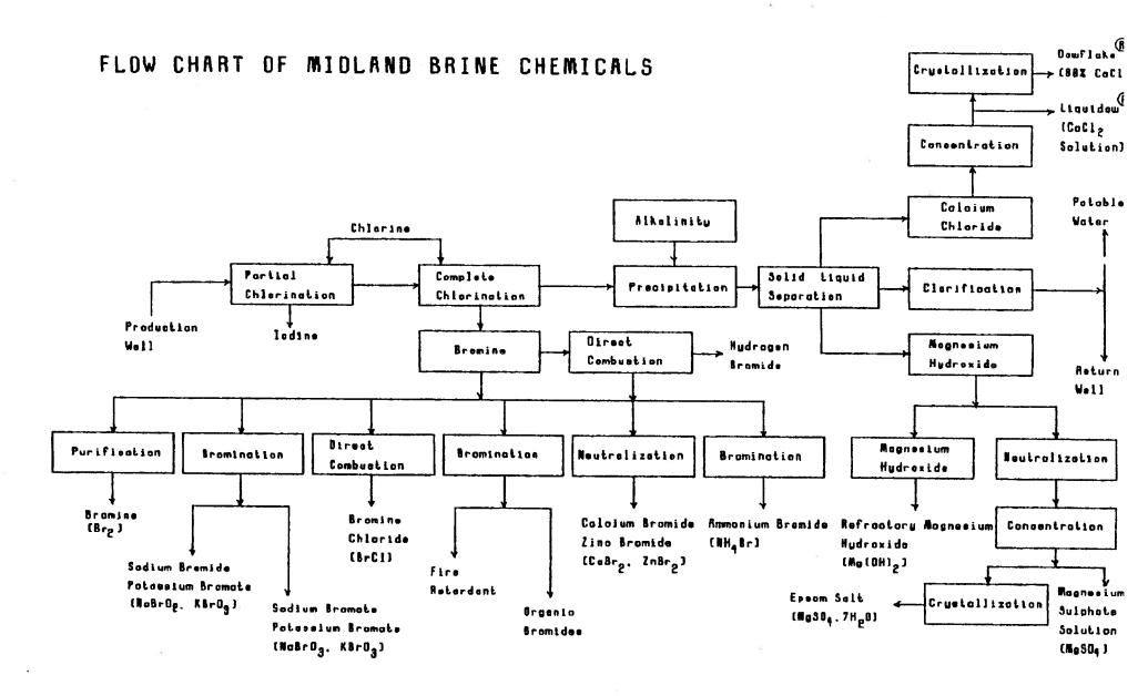
Figure 2 . Example of an integrated brine abemicals faaility using brine from the Sylvania formation
