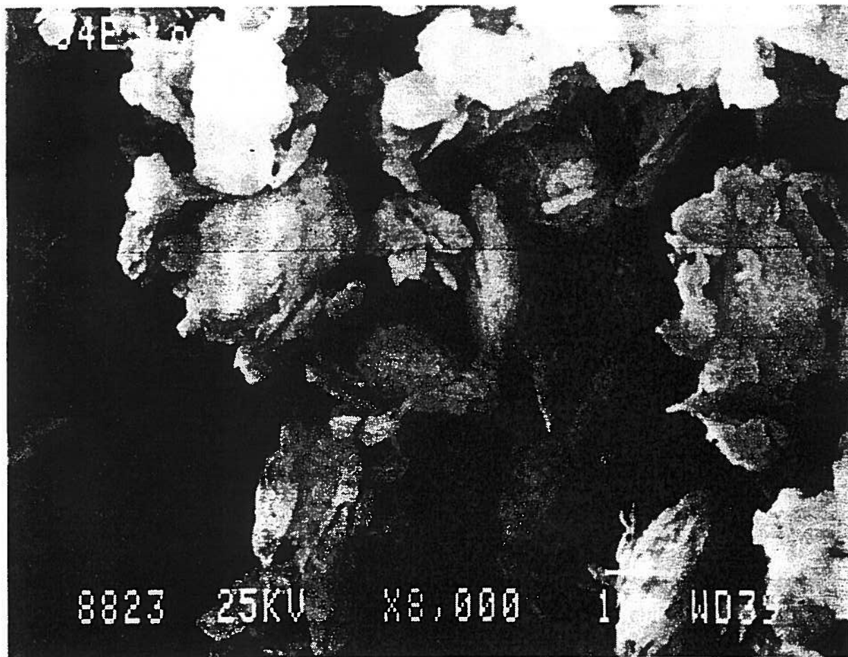
Figure 7. Scanning electron micrograph, -2\mu\text{m} fraction, sample 34E-Top. Agglomerates of kaolinite flakes are the only minerals seen in this size fraction from Whitemud kaolinitic sand.
