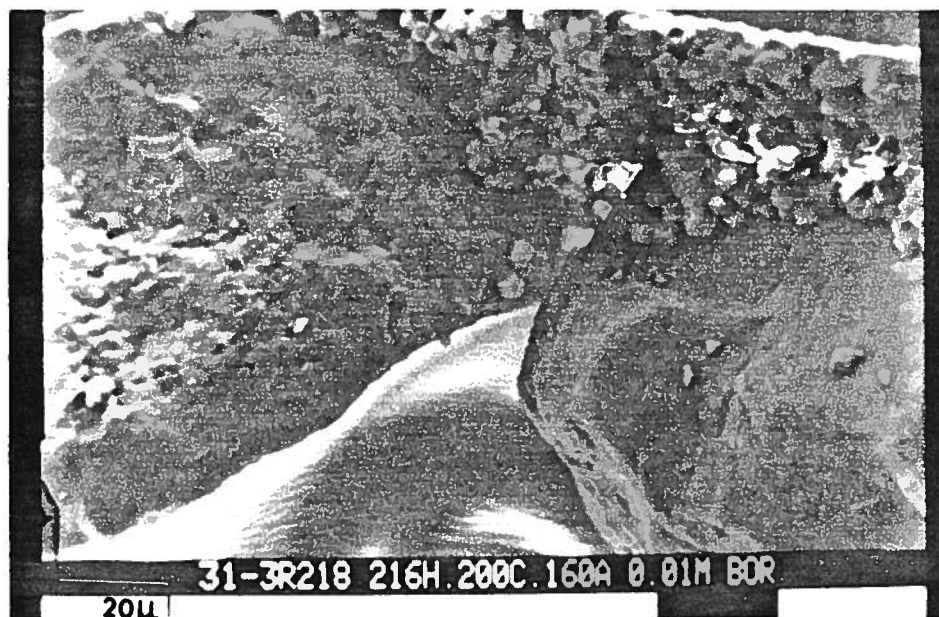
PLATE 11: Extensive analcime growth closing off a pore. Bitumen-free Athabasca oil sand, reacted with 0.01 M borax at 200°C for 216 hours.
