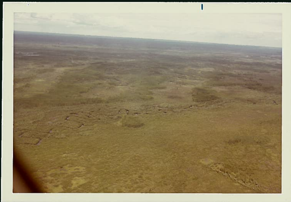
Photo 6. Tributary stream meandering across flat terrain of the in situ area. Note the absence of an erosional valley and hence the lack of a damsite.
