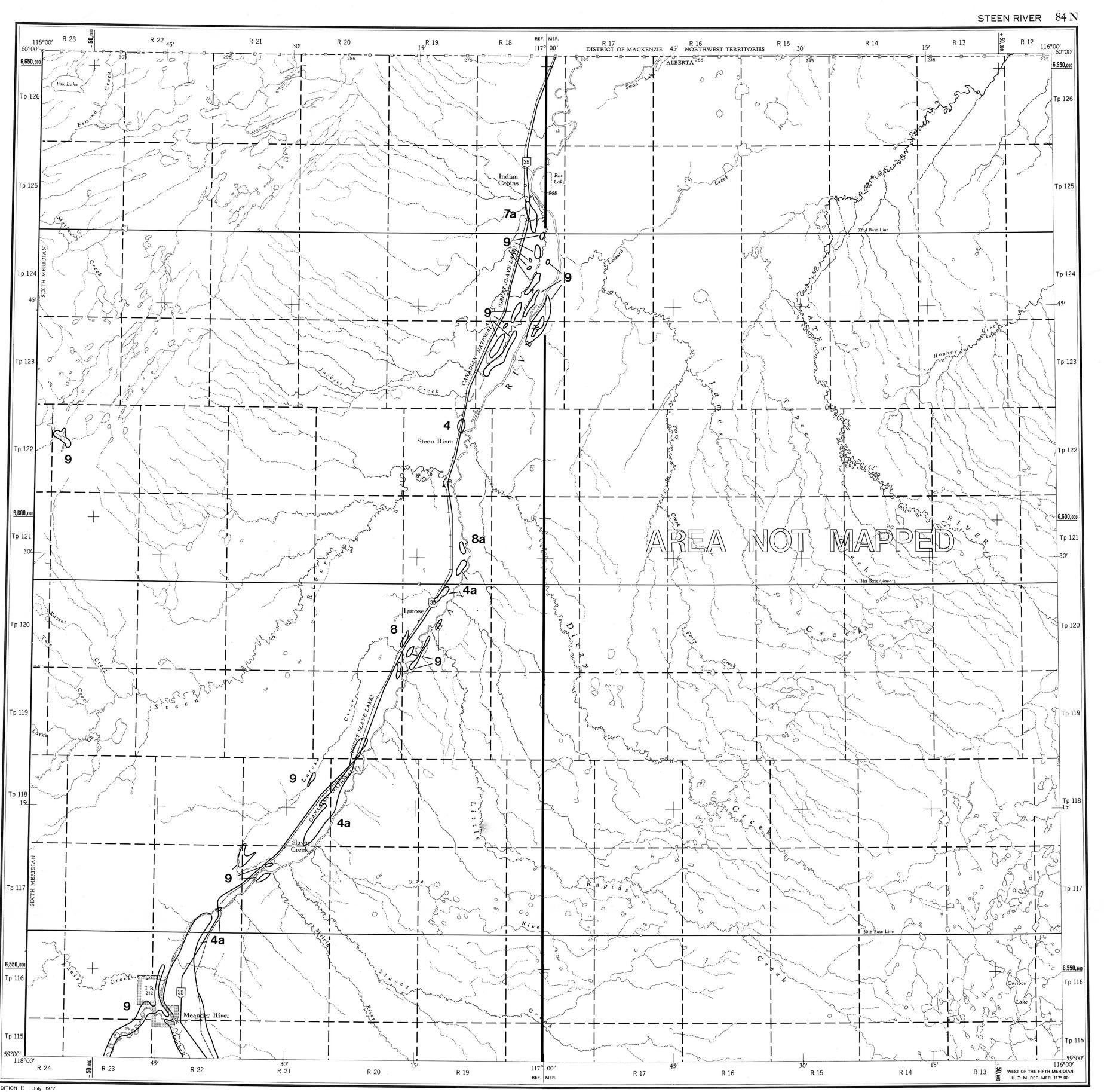
This reconnaissance-level, aggregate potential map is derived from published information, aerial photograph interpretation and limited field checking. As such, deposit outlines are assumed and material descriptions are either assumed or approximate. The sources of information used to produce this map are listed below and terms used in the legend are defined in the ternary diagram.
