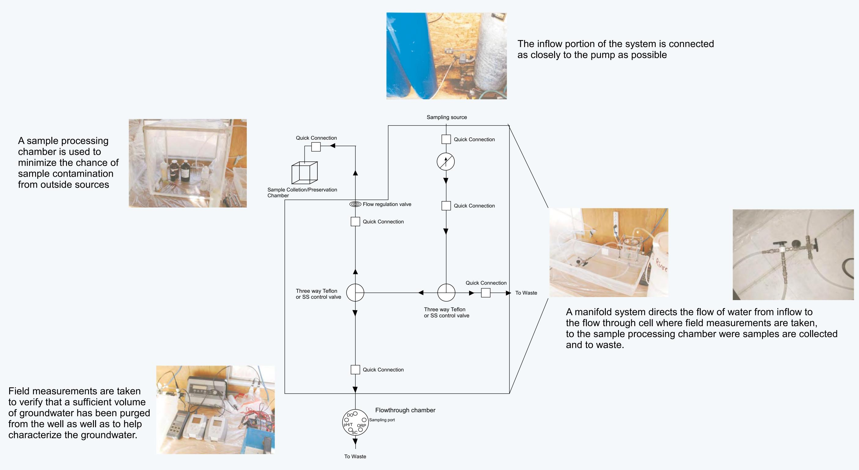
Groundwater Field Sampling Setup (modified from Koterba and others, 1995)
