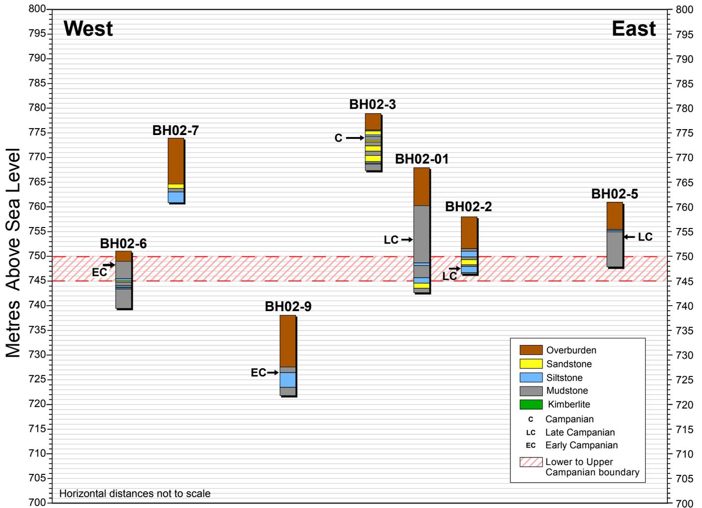
Figure 7: Section showing auger core-holes that intersect bedrock and palynological ages determined from core.
