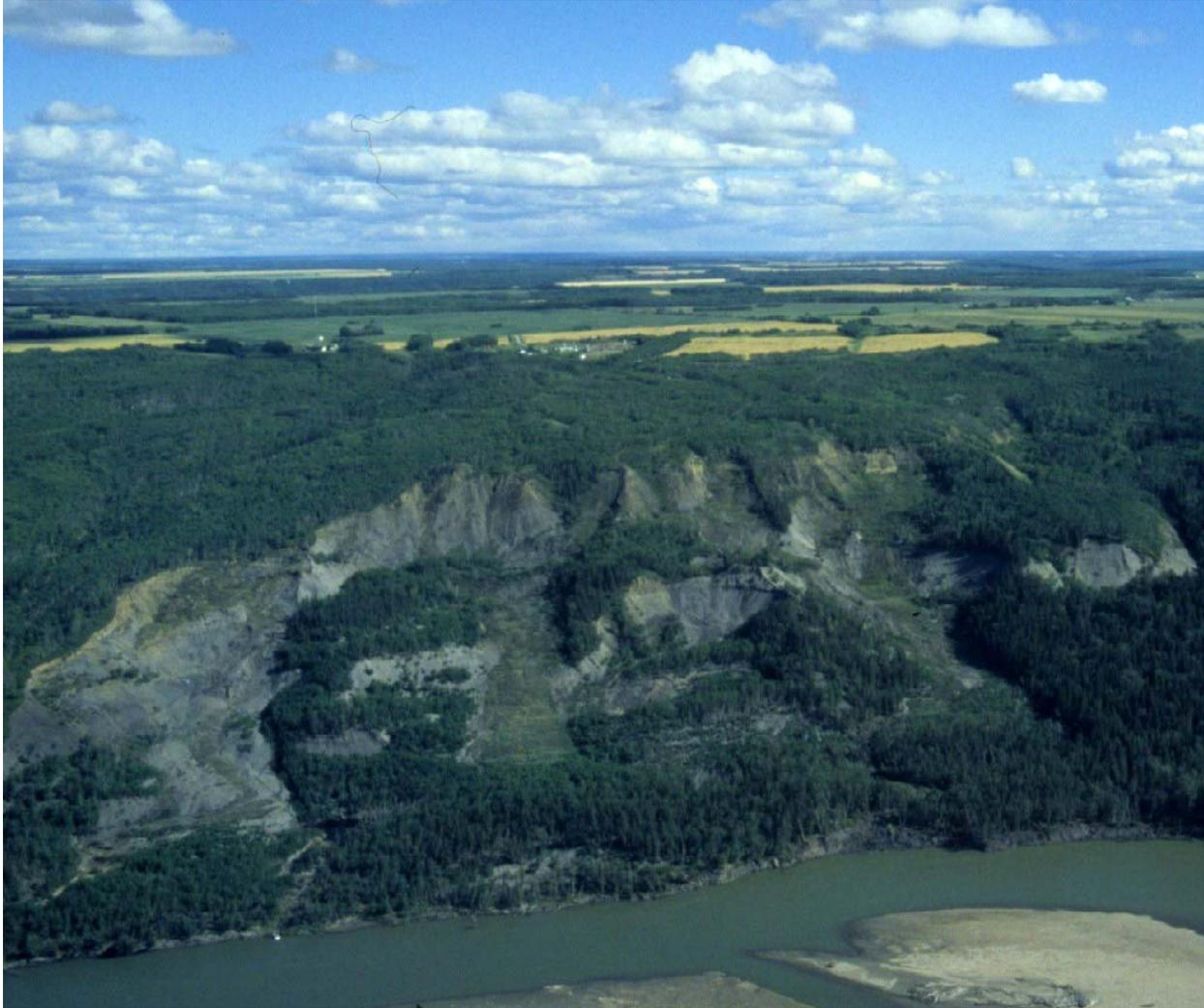
Figure 11. A recent landslide on the Smoky River occurring in Shaftesbury Formation shale.
