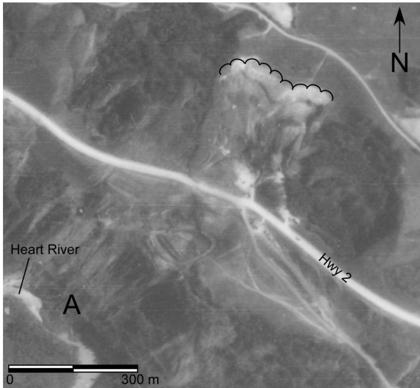
Figure 8. The 1984 earth flow above the Heart River along Highway 2 (inventory slide number 86) provides an example of a slide feature classified as active. Note the original slide topography and slopes that are bare of vegetation (see also Figure 4). The slide debris deposited in the Heart River is visible (A) (Air Photograph 84-102P LN 83 3056 36, 1:60 000, ©Alberta Sustainable Resource Development, Air Photo Distribution).
