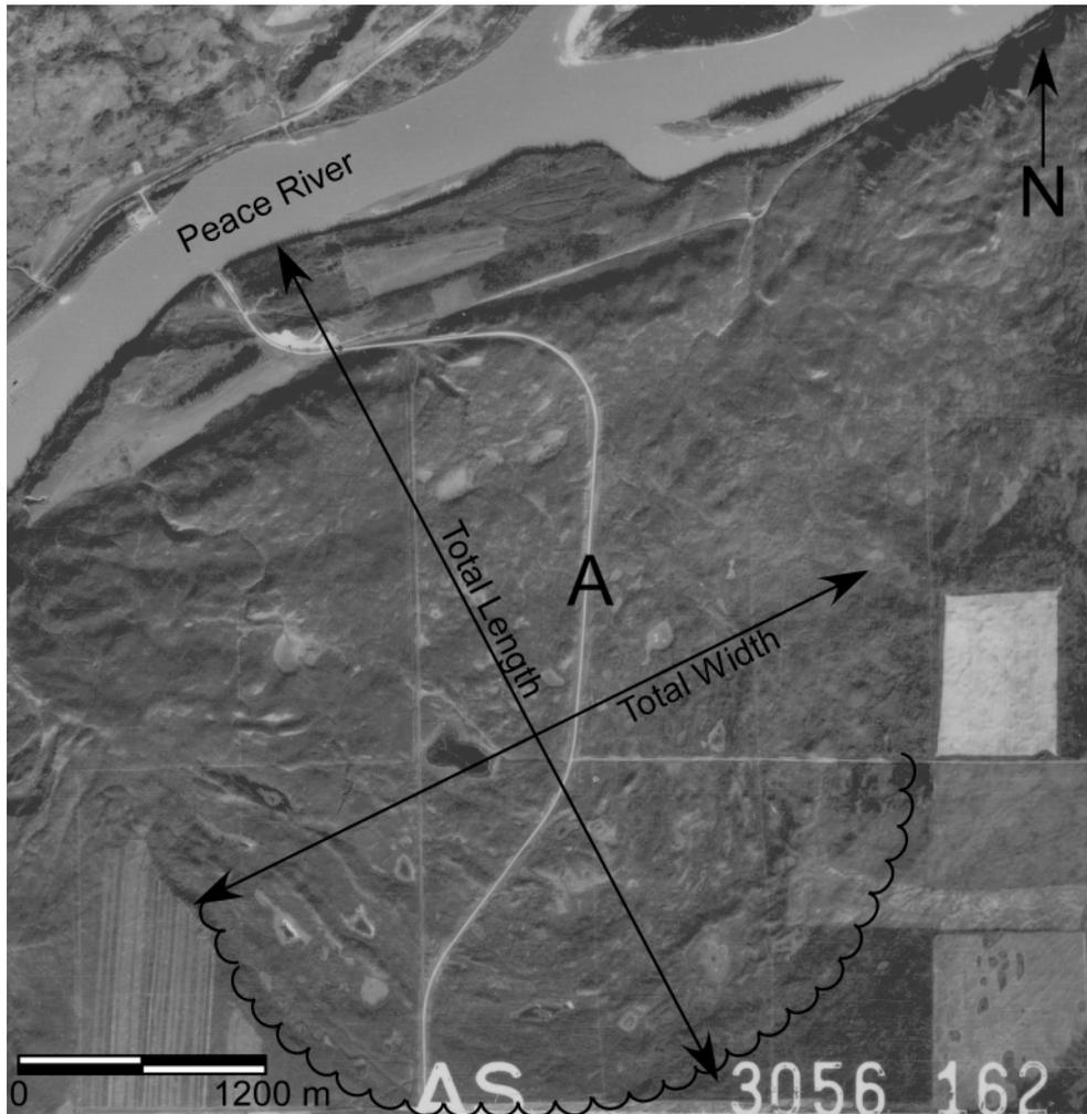
Figure 7. Example of an inactive-old earth flow. A bowl shaped depression (A) formed when the material flowed as a viscous fluid. The Peace River has shifted toward the opposite side of the valley and drainage is established on the slide mass, common features of slide described as Inactive-Old. Length and width measurements are shown. (Air Photograph 84-102P LN 82 3056 162 1:60000, ©Alberta Sustainable Resource Development, Air Photo Distribution).
