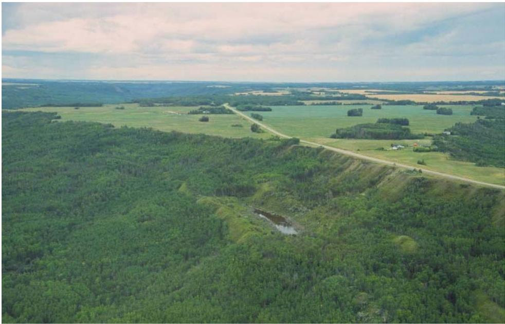
Figure 6. Sag pond developed near the scarp of a landslide. Highway 744 can be seen to the south.
