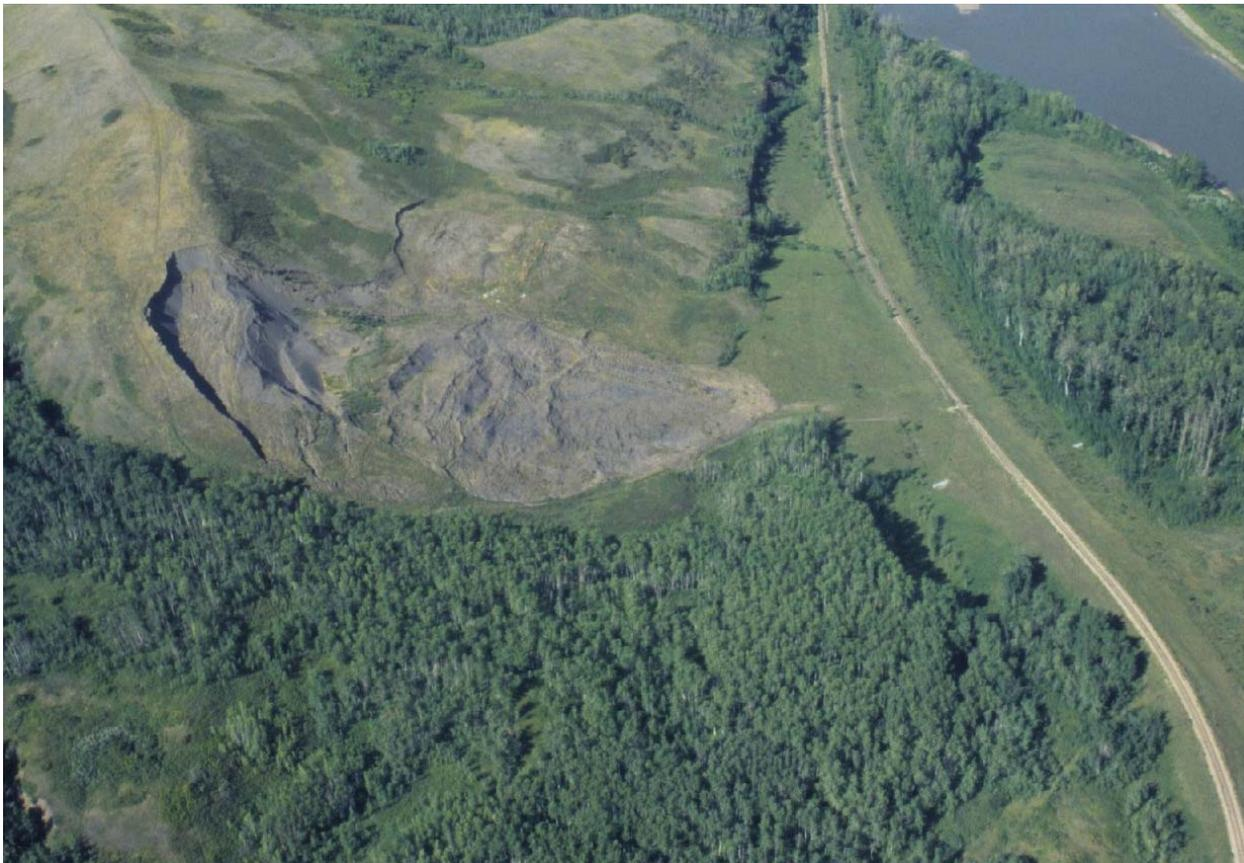
Figure 10. A recent landslide in glacial Lake Peace sediments.
