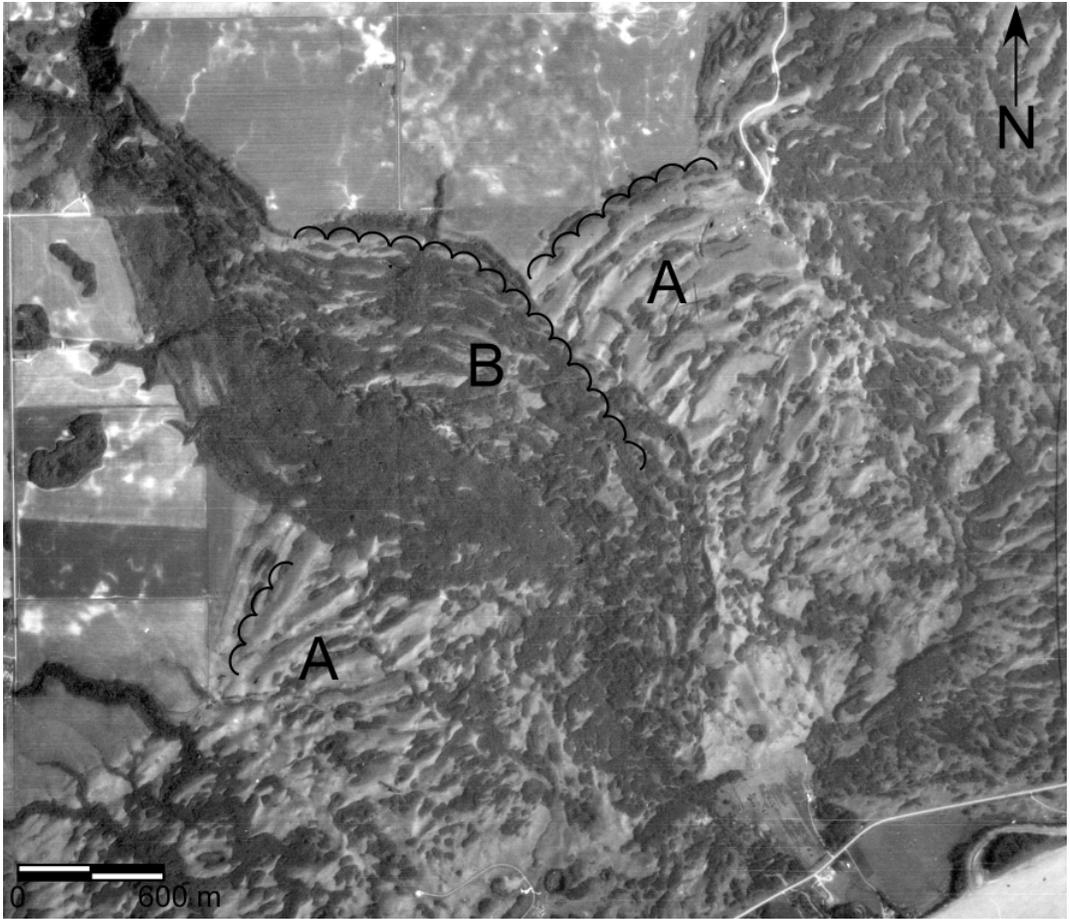
Figure 5. Example of a rotational slide (A) dissected by more recent sliding (B). Note backward tilted displaced material (Air Photograph 84-102P LN 83 3057 32, 1:60 000, ©Alberta Sustainable Resource Development, Air Photo Distribution).
