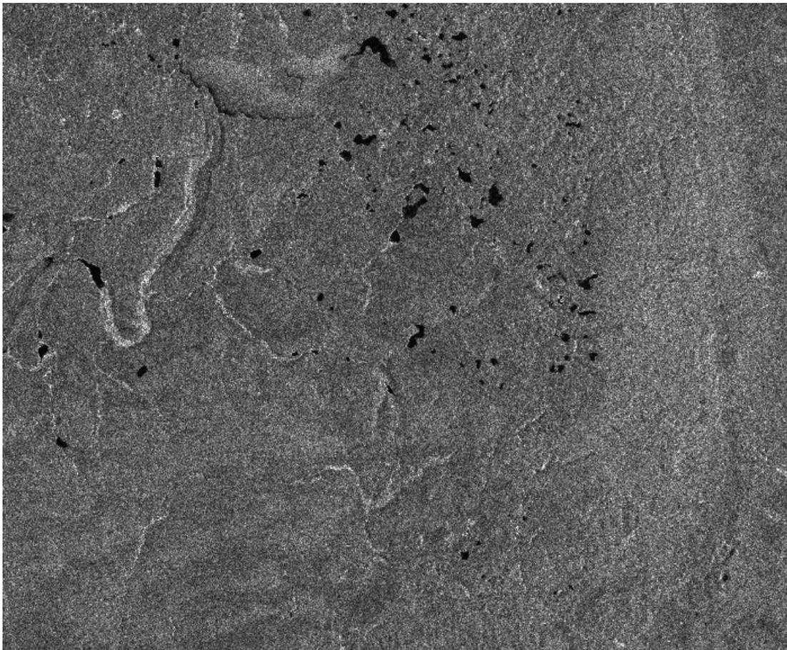
Figure 4a. S1 ascending RADARSAT-1 imagery – orthorectified and unfiltered. There is considerable speckle in the image and ground features are obscured.
