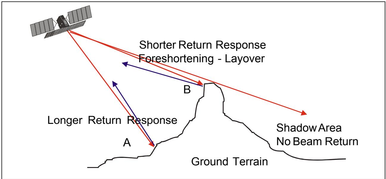
Figure 3. Terrain effects on radar response. Areas of high relief result in responses that are time dependent. These different responses result in layover. Also, the back side of the topographic feature will provide no return at all, resulting in a null image.
