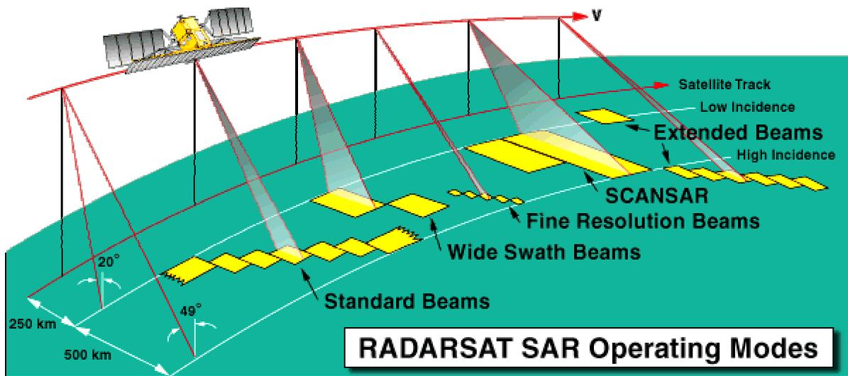
Figure 1. Operating modes for RADARSAT-1. Variable beam widths and angles are available with RADARSAT-1.
