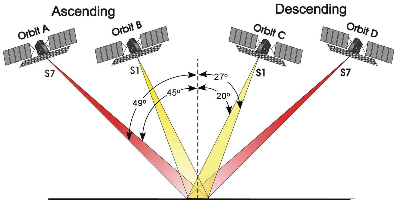
Figure 2. Configuration of the use of multi-beam imagery for the terrain mapping program at the Alberta Geological Survey.
