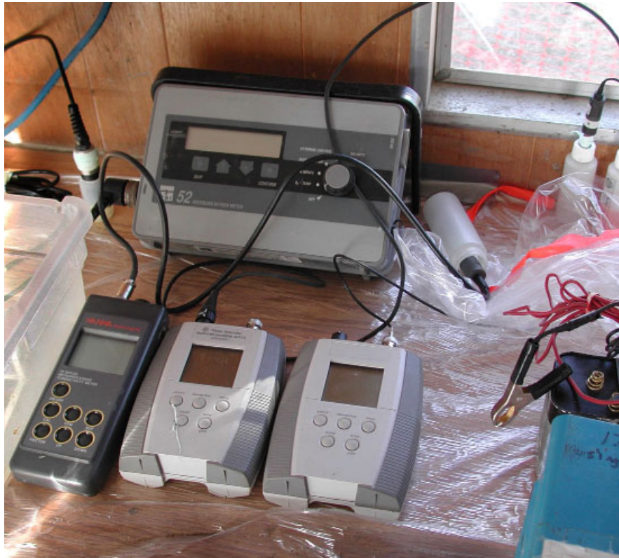
Figure 5. Field parameter measurement equipment (front from left to right: conductivity meter, pH-temperature meter and oxidation-reduction potential meter; rear: dissolved oxygen meter).
