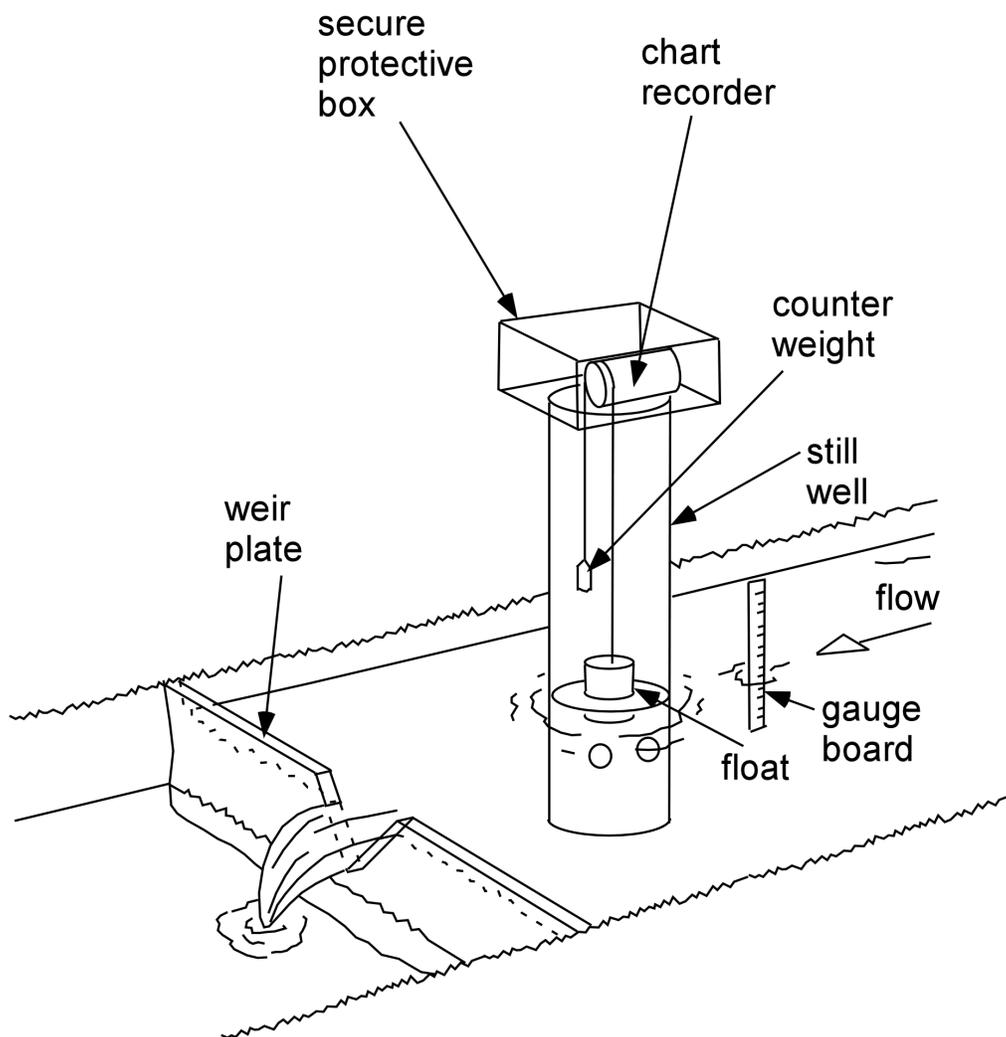
Figure 3. Weir and Still Well setup (not to scale).
