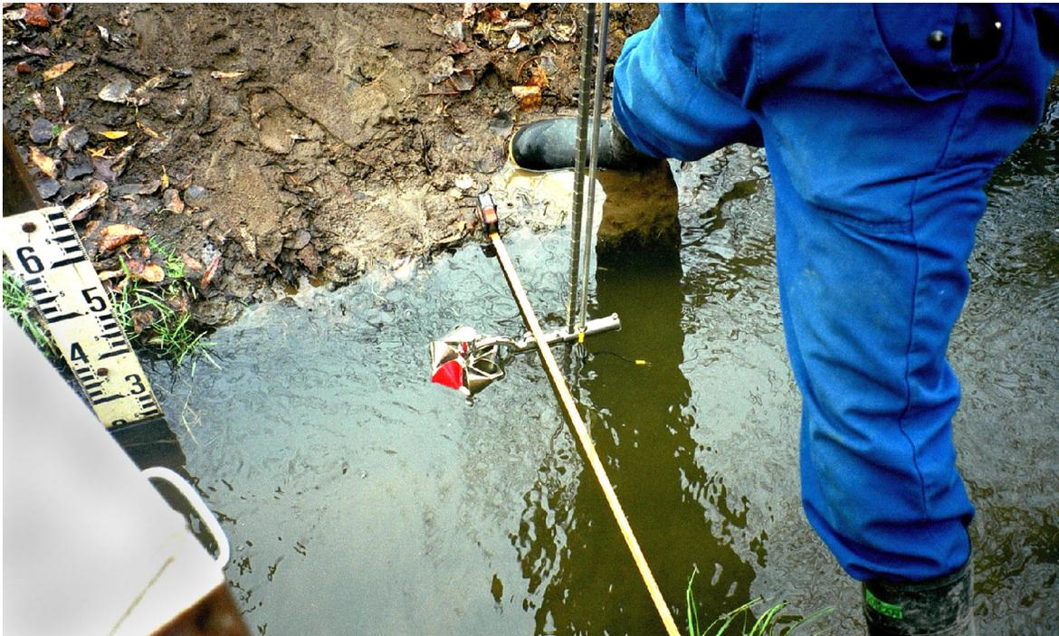
Figure 4. Flowmeter and wading rod.
