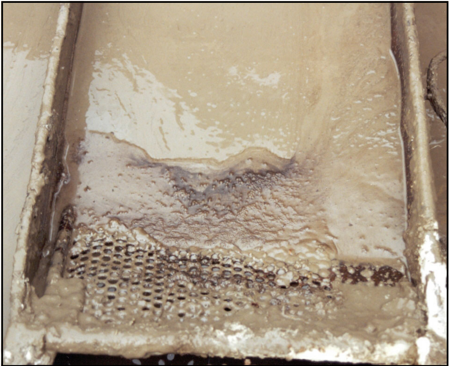
Figure 4. Oily emulsion in drill-mud tank, core hole WEPAA00-1. The emulsion was first observed when drilling in till at a depth of about 32.5 m, and was visible in the drill mud over the next four days, until the hole was abandoned at a depth of 173.5 m.
