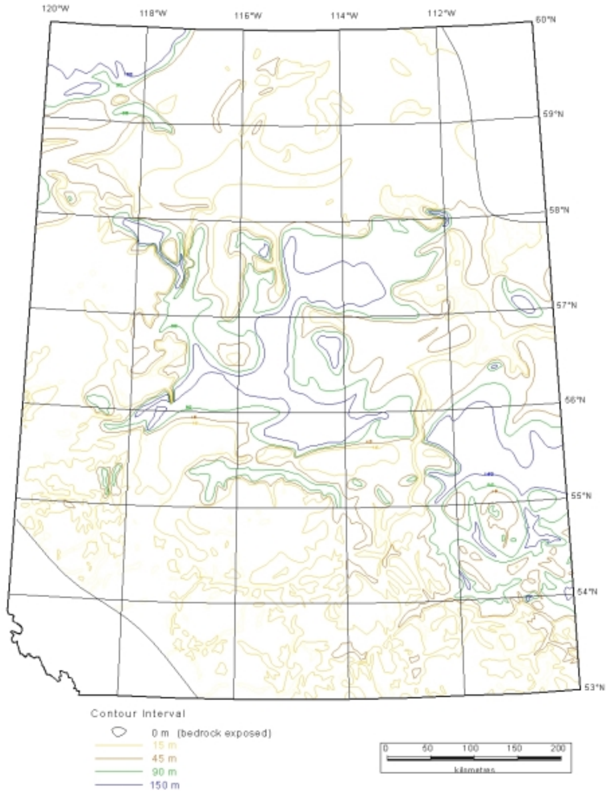
Figure 3. Drift thickness map, reduced from Pawlowicz and Fenton 1995. Northern half of the map based on very limited data.
