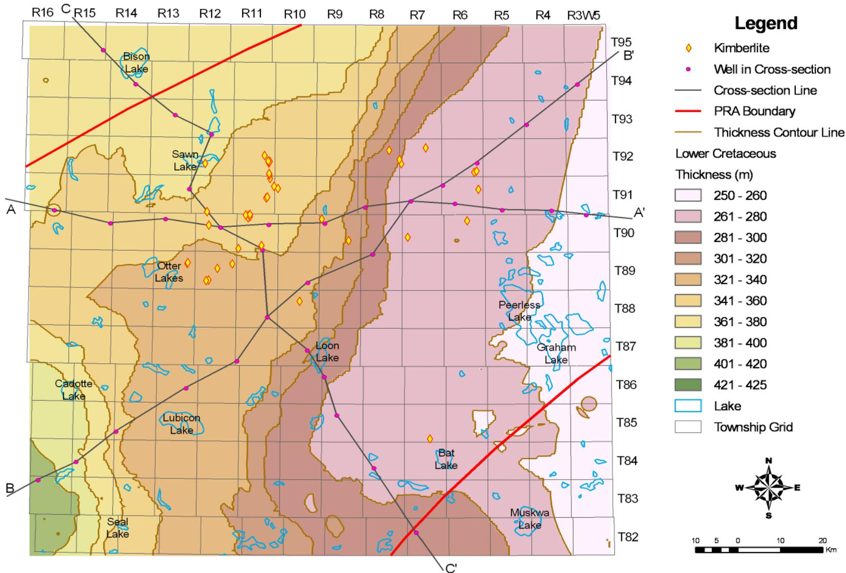
Figure 10. Isopach map of Lower Cretaceous formations for the Buffalo Head Hills—Peerless Lake region, representing the thickness of the strata from the base of the Gething and/or Bluesky Formation to the base of the Fish Scales Formation. The Peace River Arch (PRA) boundaries were digitally compiled by Pana et al. (2001) from O'Connell et al. (1990).
