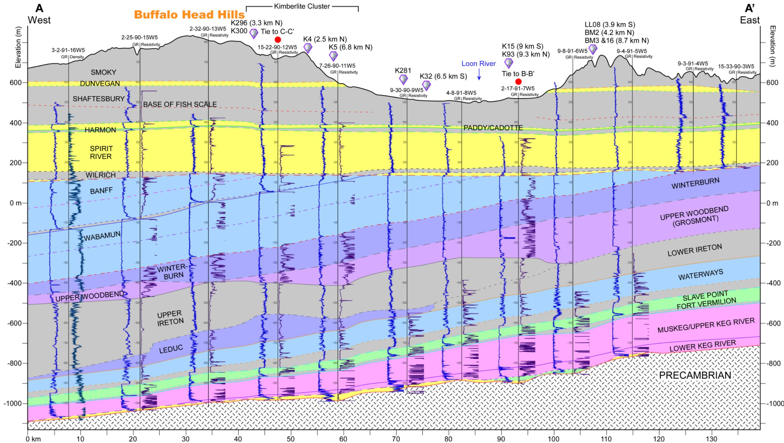
Figure 4. East-trending cross-section A-A'. Vertical scale 1:10,000; horizontal scale 1:380,000 (horizontal versus vertical scale, 1:38). The geophysical logs for selected oil/gas wells are shown. Refer to Figure 1 for the cross-section location and Figure 7 for a legend. Note that glacial deposits are not differentiated from bedrock in this cross-section.
