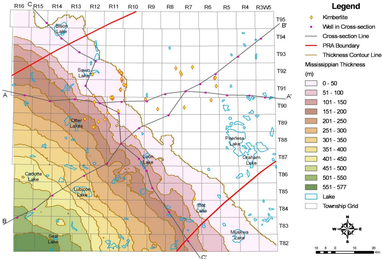
Figure 9. Isopach map of Mississippian formations for the Buffalo Head Hills—Peerless Lake region, representing the thickness of the strata from the Exshaw Formation base to the Rundle Group top erosional surface. The Mississippian strata were truncated to the northeast and is overlain by the Lower Cretaceous units. The Peace River Arch (PRA) boundaries were digitally compiled by Pana et al. (2001) from O'Connell et al. (1990).
