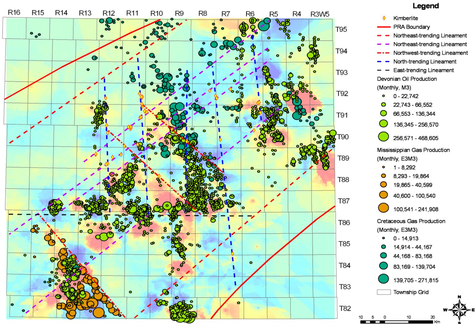
Figure 16. Distribution of oil and gas pools and production in the Buffalo Head Hills—Peerless Lake region, showing strong impact by the basement topography and lineaments. The pools are seemingly preferentially distributed along and around basement highs and confined by the lineaments inferred by this study. The Peace River Arch (PRA) boundaries were digitally compiled by Pana et al. (2001) from O'Connell et al. (1990). Figure 15 for lineament names and Precambrian top residuals.
