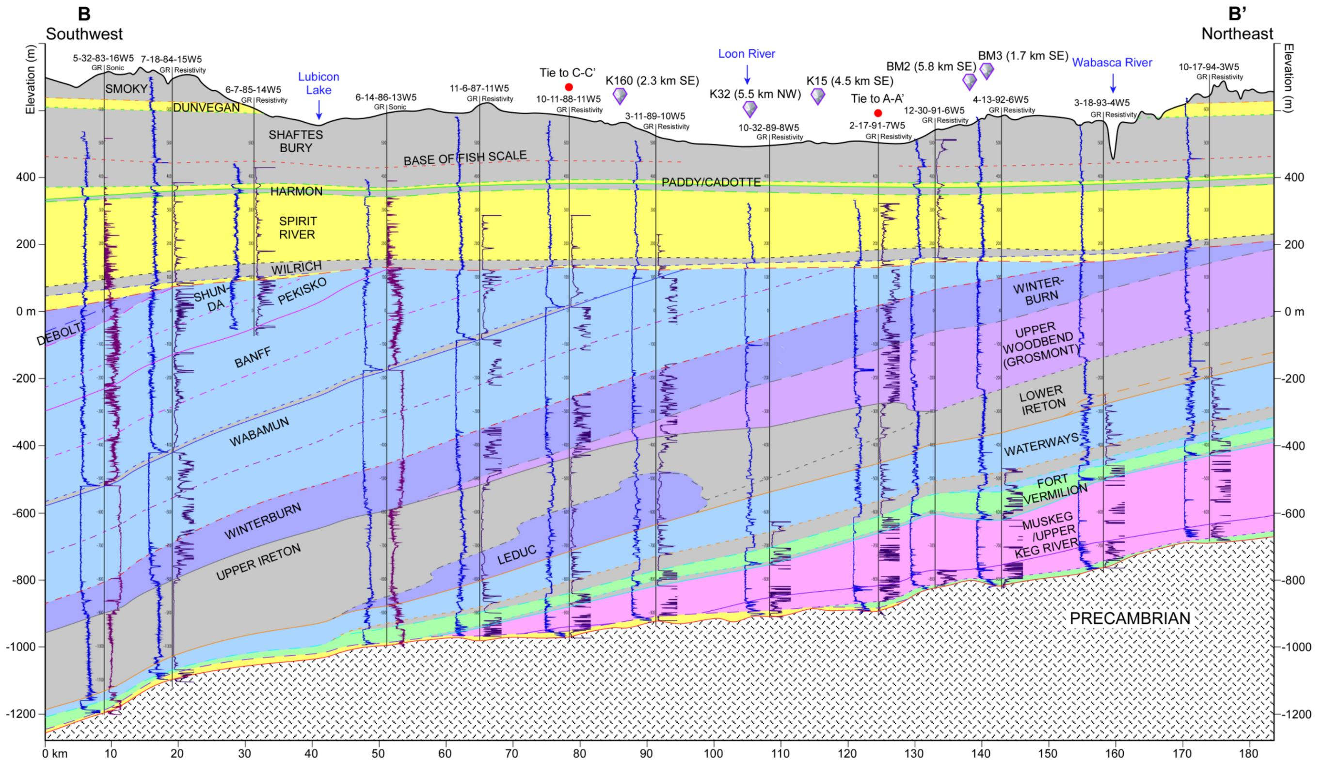
Figure 5. Northeast-trending cross-section B-B'. Vertical scale 1:10,000; horizontal scale 1:500,000 (horizontal versus vertical scale, 1:50). The geophysical logs for selected oil/gas wells are shown. Refer to Figure 1 for the cross-section location and Figure 7 for a legend. Note that glacial deposits are not differentiated from bedrock in this cross-section.
