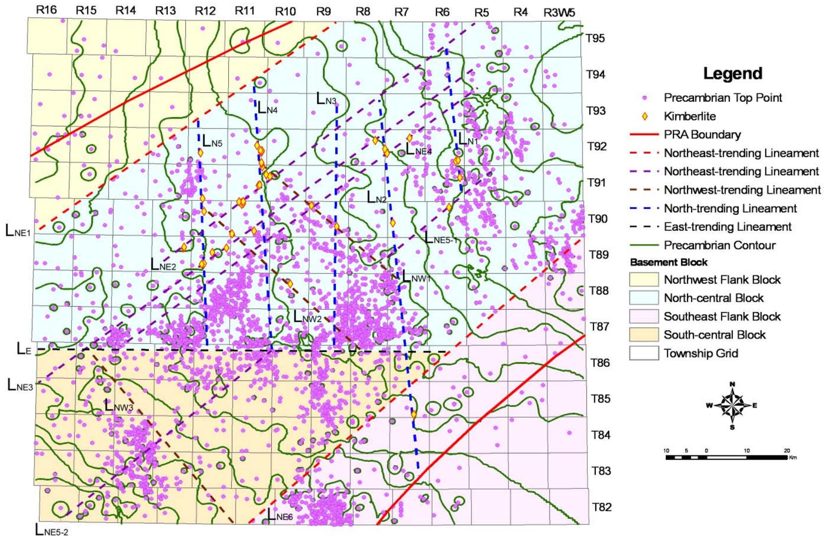
Figure 14. Basement subdivisions and locations of the wells with the Precambrian basement top identified in the Buffalo Head Hills—Peerless Lake region. There are 3230 mapping control points (pink-filled purple circles) for the maps in Figures 13 and 15. The region can be divided into four large blocks based on the change of the overall contour line strikes and patterns. The Peace River Arch (PRA) boundaries were digitally compiled by Pana et al. (2001) from O'Connell et al. (1990).
