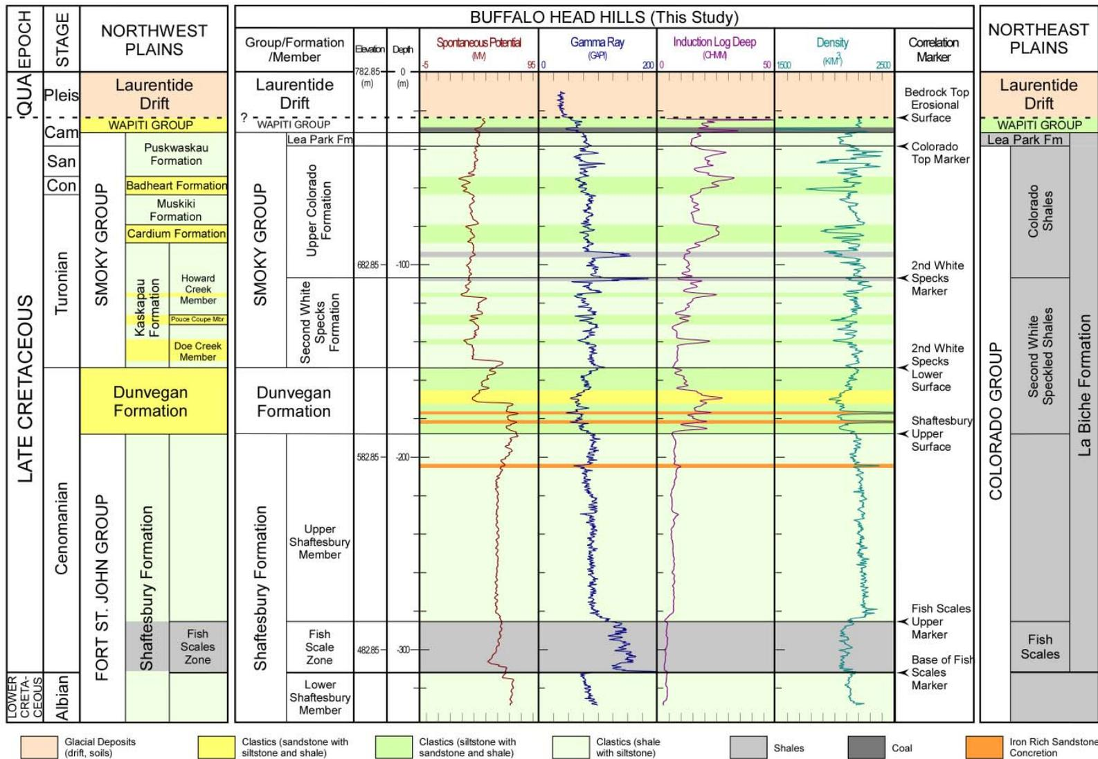
Figure 3. Stratigraphic features and nomenclature of the upper Cretaceous in the Buffalo Head Hills area (this study) and equivalent strata in northern Alberta (modified from Stott, 1982, 1984; Cotterill and Berhane, 1996). The reference logs are from well 9-4-93-12W5, with a kelly bushing (KB) elevation of 782.85 m above sea level. Abbreviations: QUA, Quaternary; Con, Coniacian; San, Santonian; Cam, Campanian; Pleis, Pleistocene; Fm, Formation; Mbr, Member.
