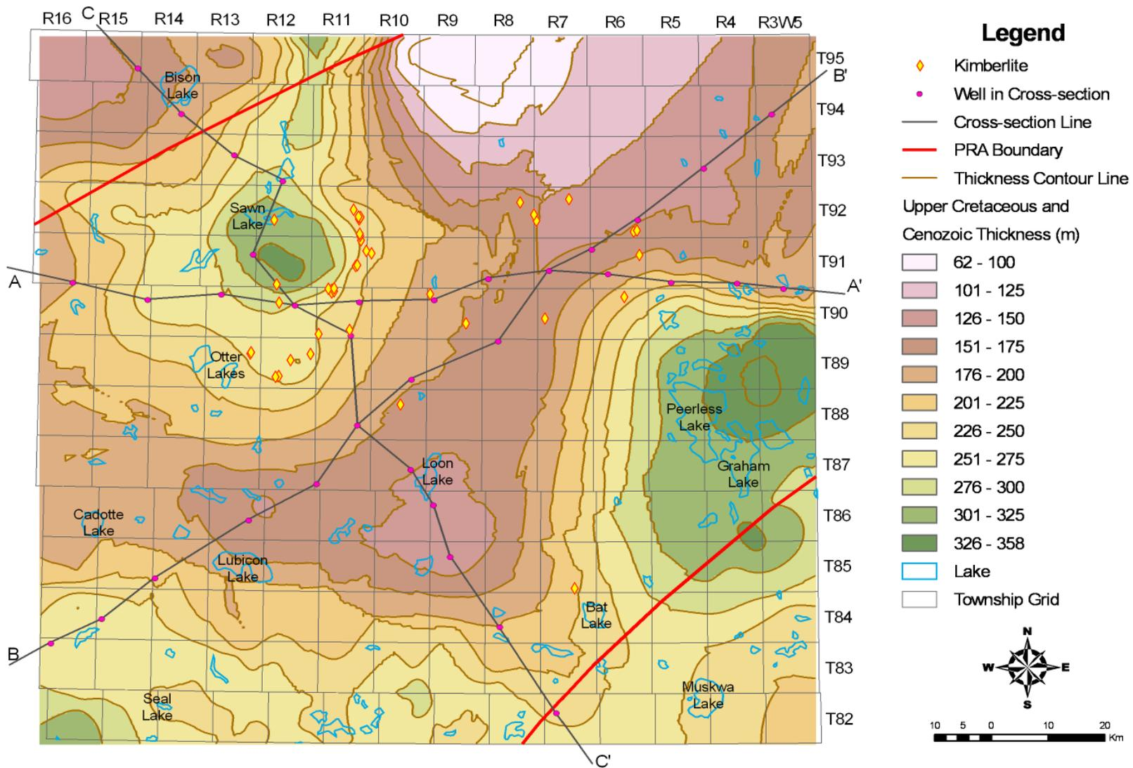
Figure 11. Isopach map of Upper Cretaceous and Cenozoic formations for the Buffalo Head Hills—Peerless Lake region, representing the thickness of the strata from the base of the Fish Scales Formation to the ground surface. Note that the pattern of this isopach map is very similar to that of the ground surface topography in Figure 12. The Peace River Arch (PRA) boundaries were digitally compiled by Pana et al. (2001) from O'Connell et al. (1990).
