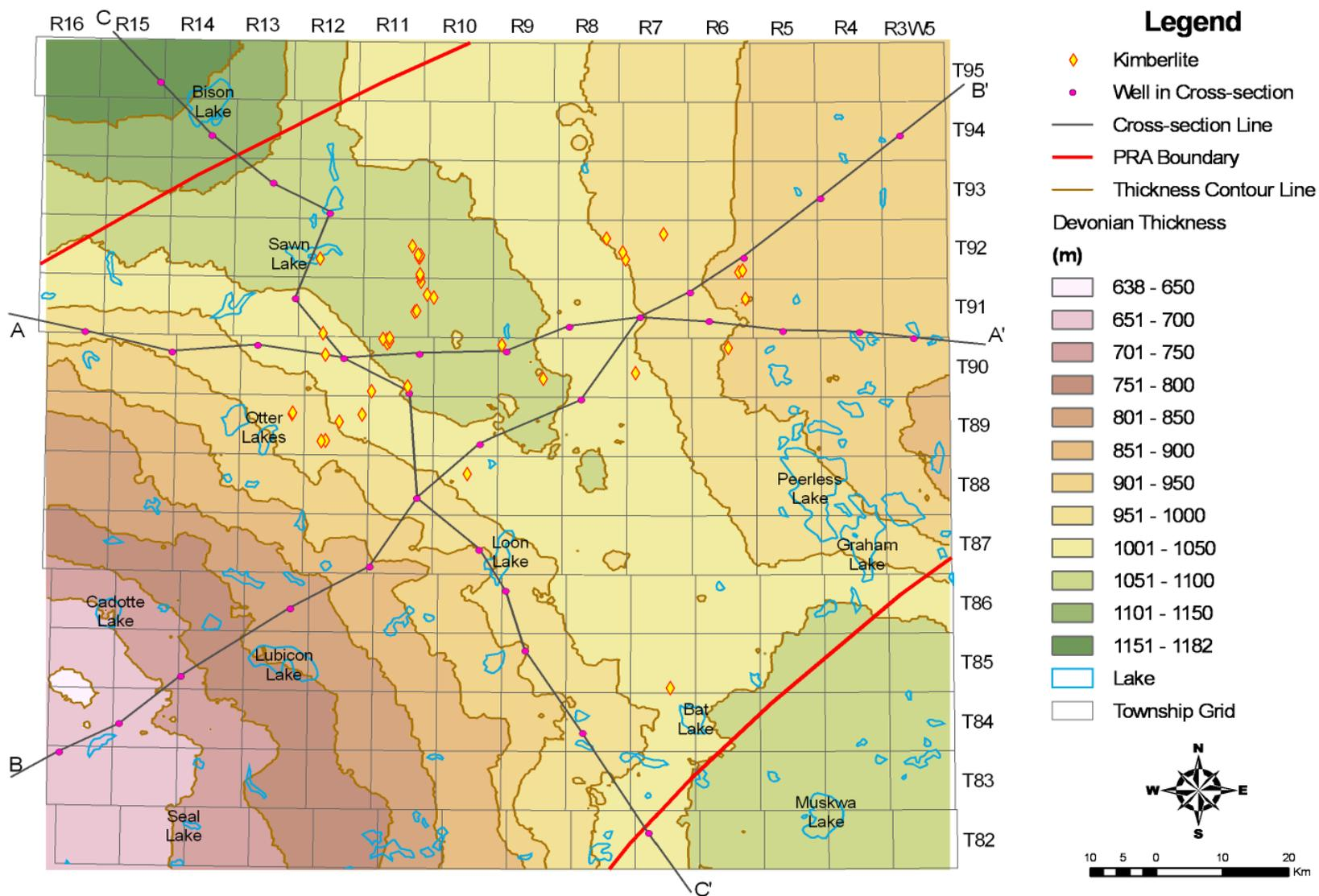
Figure 8. Isopach map of Devonian formations in the Buffalo Head Hills—Peerless Lake region, representing the thickness of the strata from the Granite Wash litho-zone base to the Wabamun Group top. Note that the Wabamun top is truncated by Cretaceous formations in the northeast of the area. The Peace River Arch (PRA) boundaries were digitally compiled by Pana et al. (2001) from O’Connell et al. (1990).
